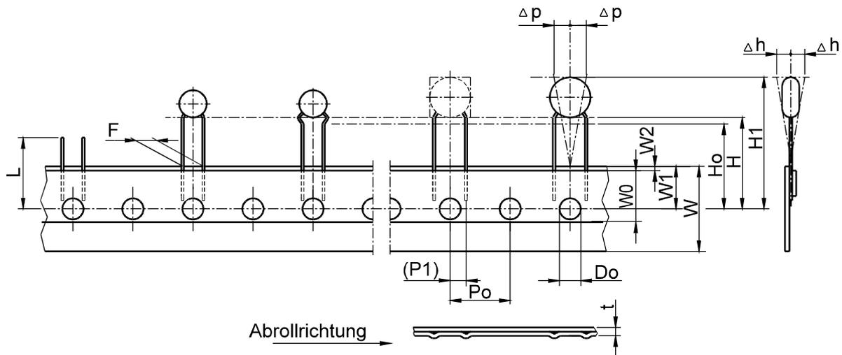
**Tape dimensions, in Millimeters (mm):**
