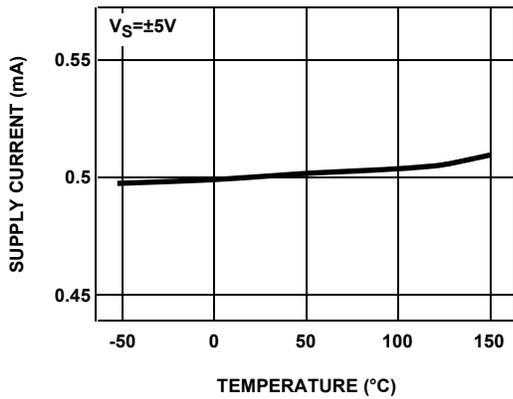
FIGURE 9. SUPPLY CURRENT PER CHANNEL vs TEMPERATURE
