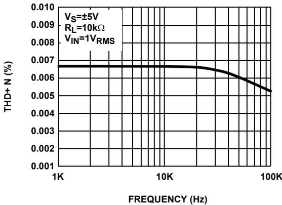
FIGURE 17. TOTAL HARMONIC DISTORTION + NOISE vs FREQUENCY
