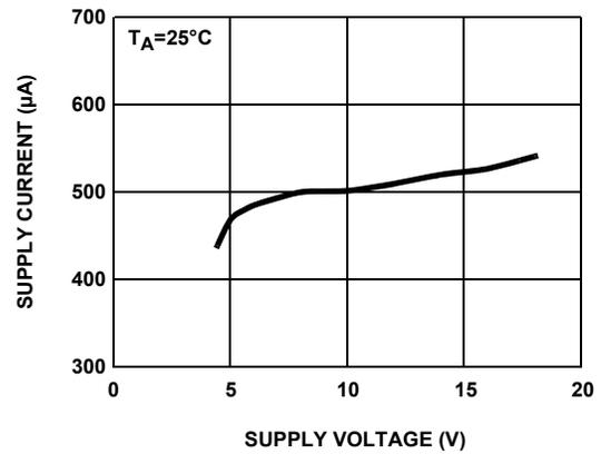
FIGURE 10. SUPPLY CURRENT PER CHANNEL vs SUPPLY VOLTAGE
