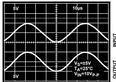
FIGURE 23. OPERATION WITH RAIL-TO-RAIL INPUT AND OUTPUT
