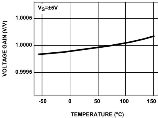
FIGURE 7. VOLTAGE GAIN vs TEMPERATURE
