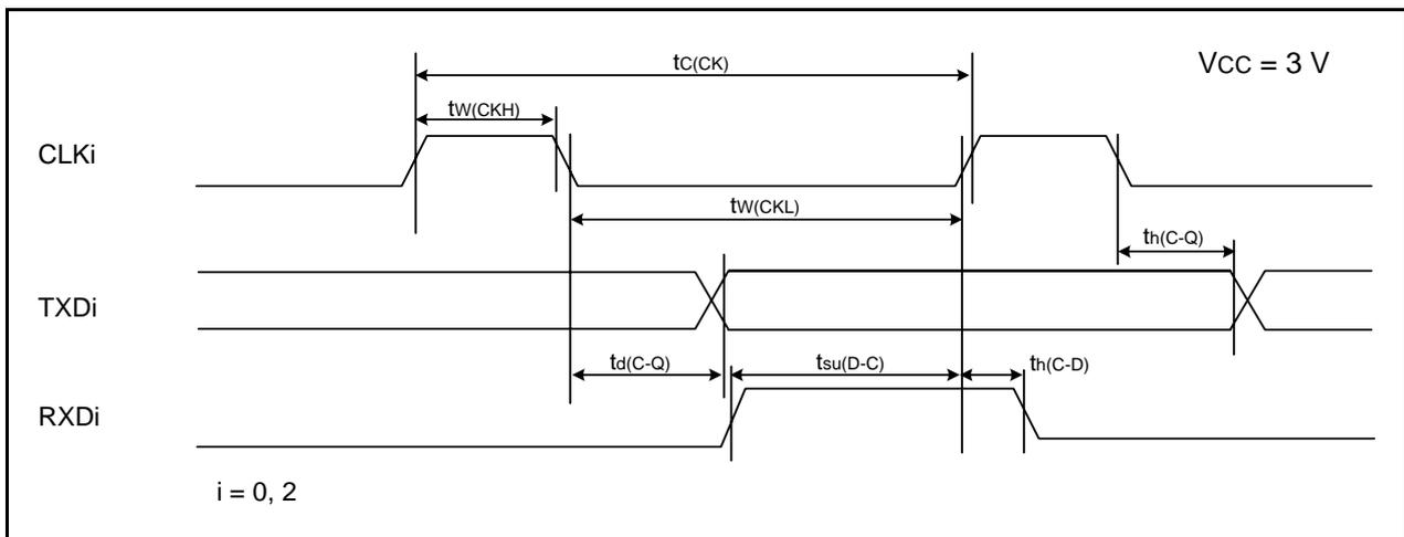
**Figure 31.14 Serial Interface Timing Diagram when Vcc = 3 V**
