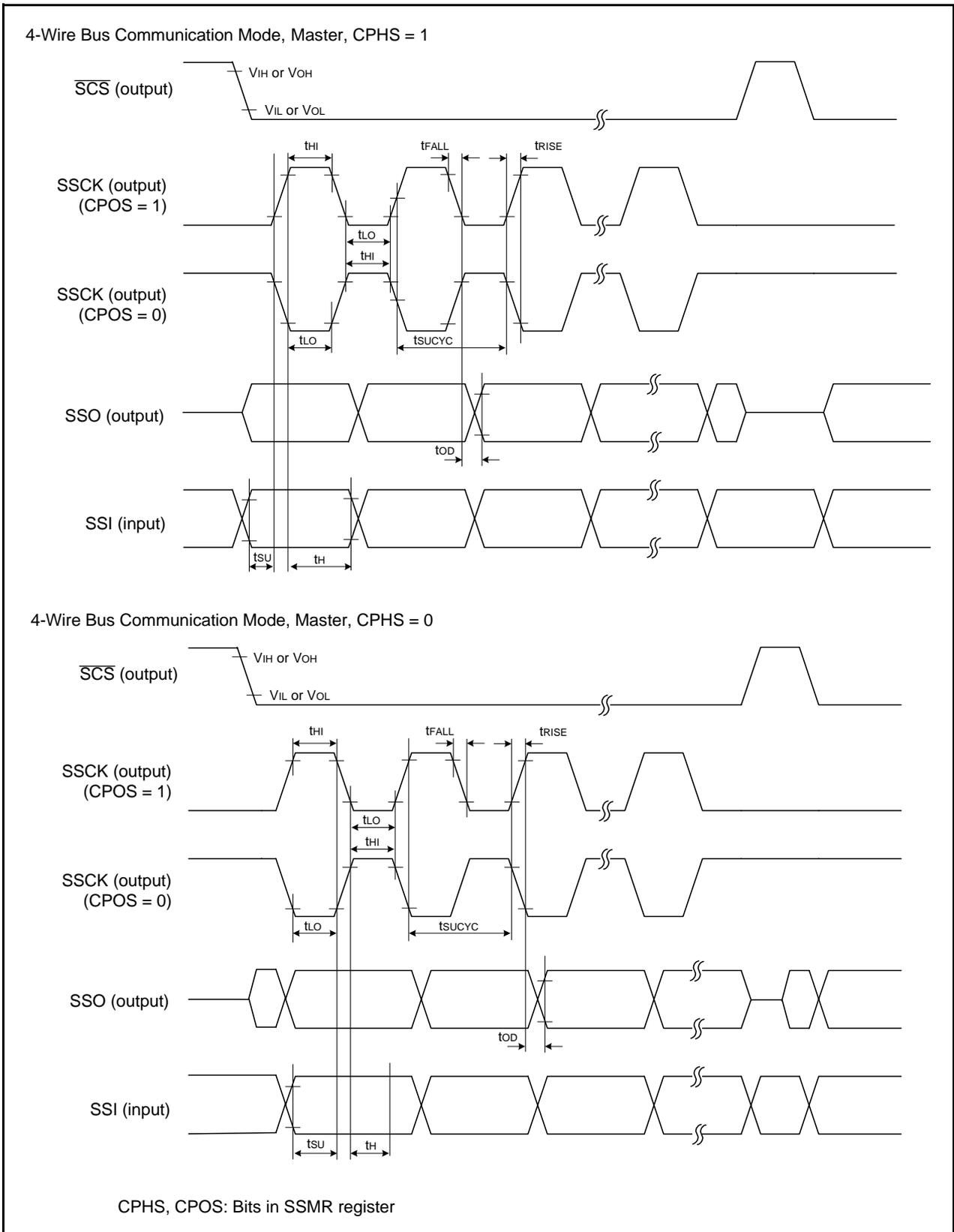
Figure 31.4 I/O Timing of Synchronous Serial Communication Unit (SSU) (Master)
