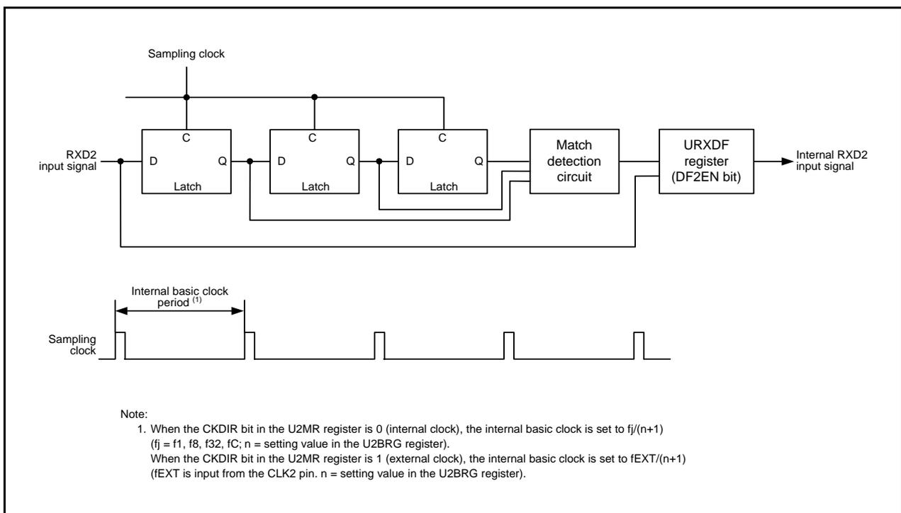
Figure 22.12 Block Diagram of RXD2 Digital Filter Circuit
