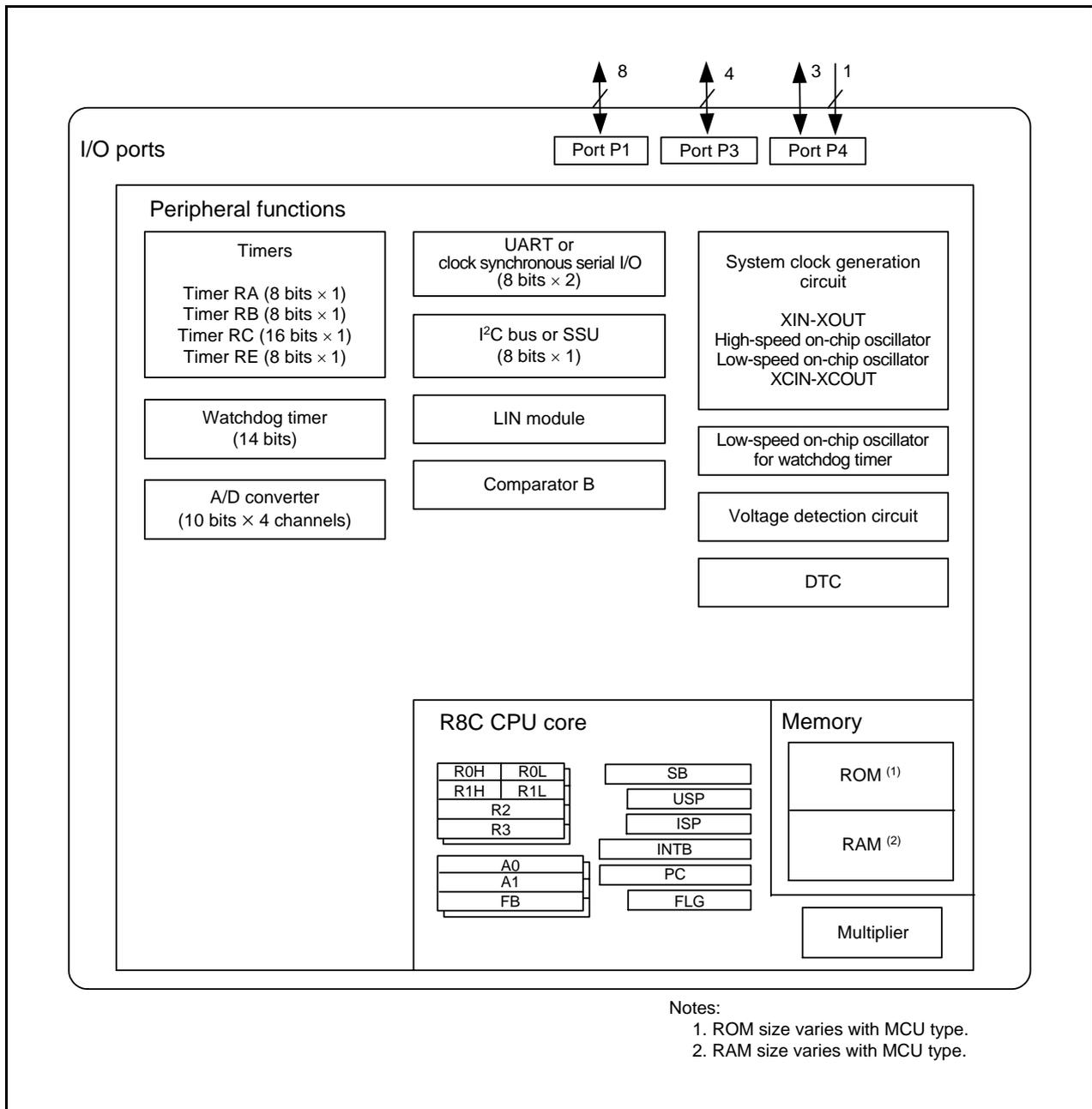
Figure 1.2 Block Diagram
