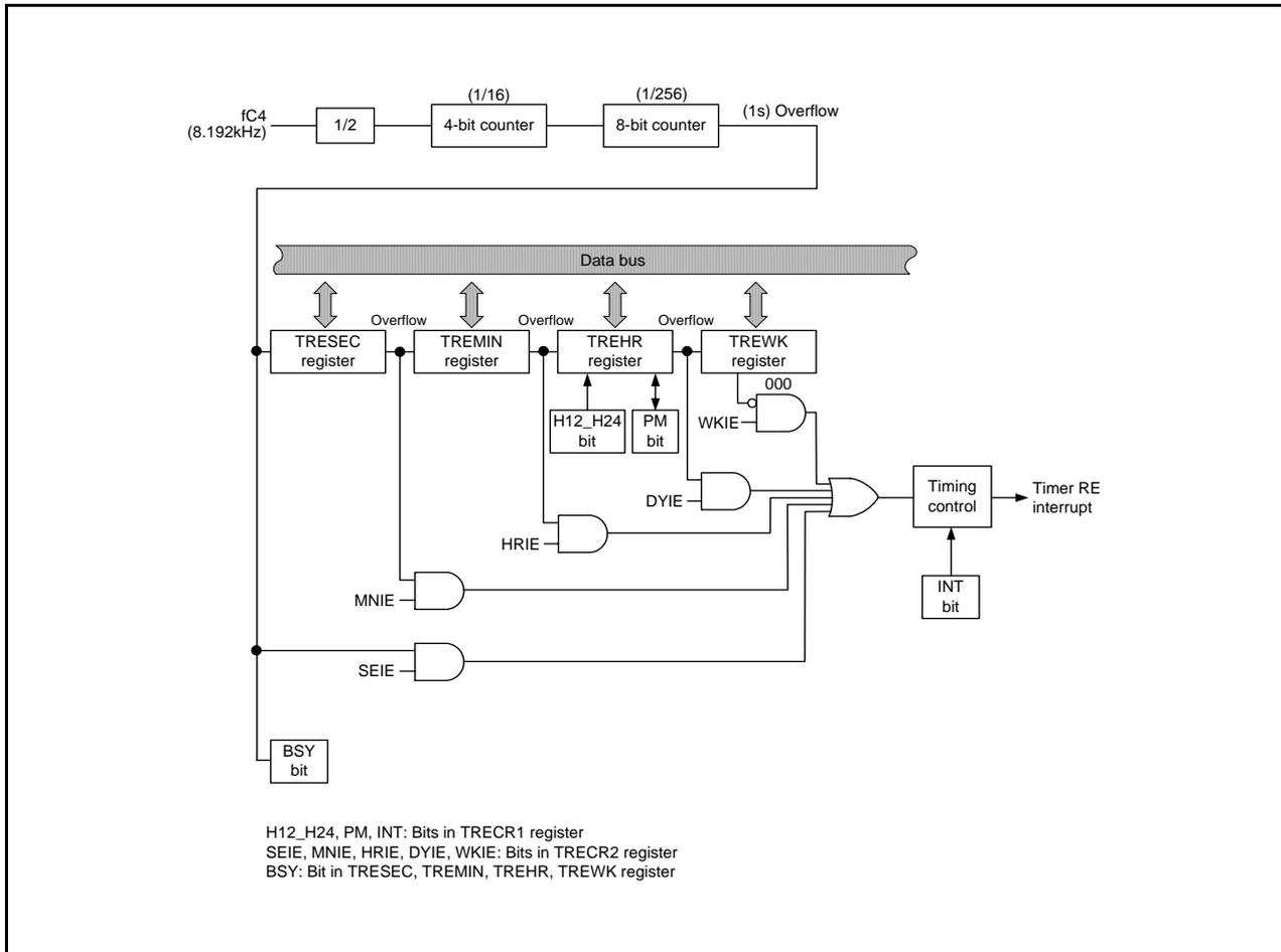
Figure 20.1 Block Diagram of Real-Time Clock Mode
