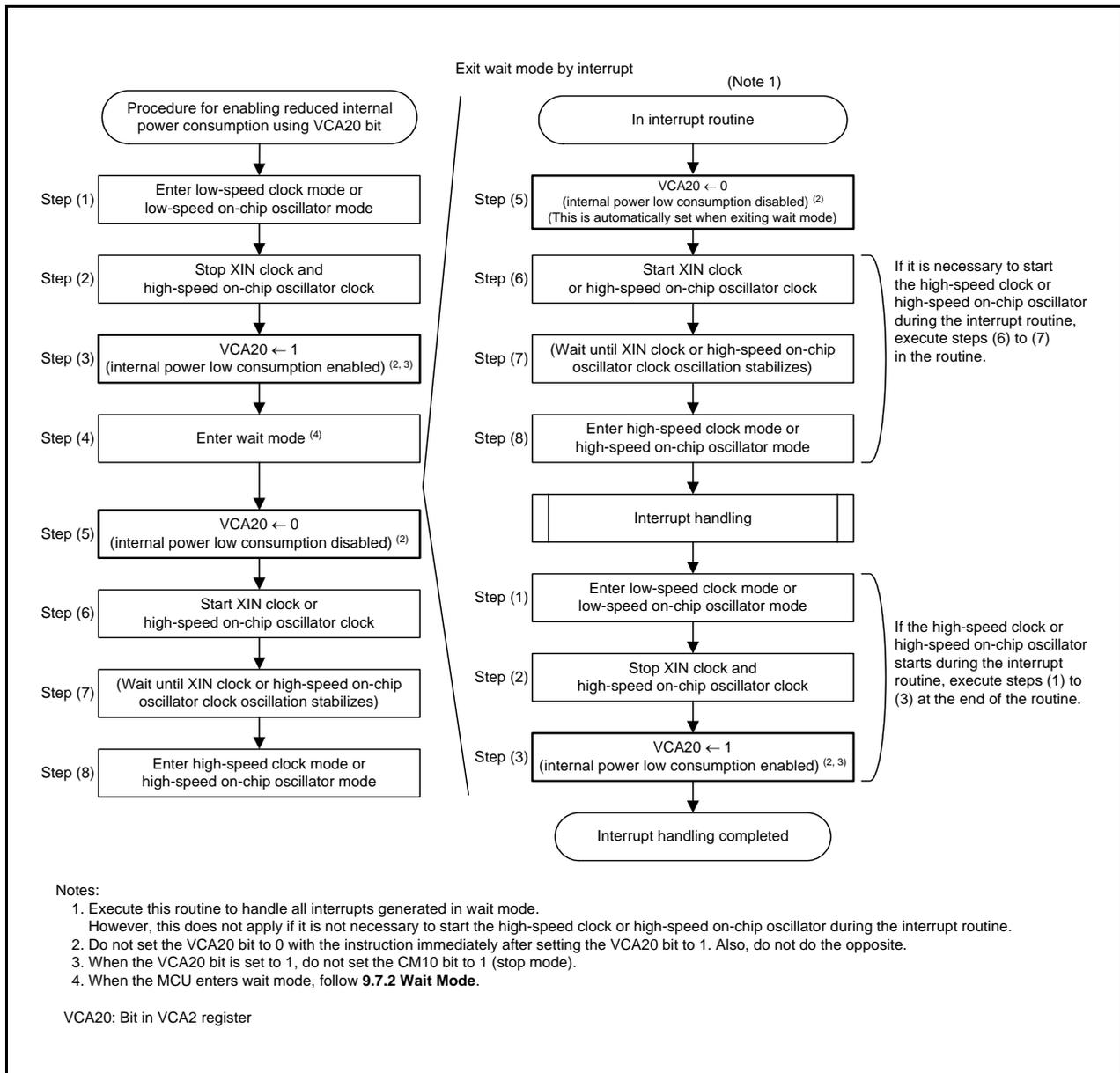
**Figure 30.1 Handling Procedure for Reducing Internal Power Consumption Using VCA20 Bit**
