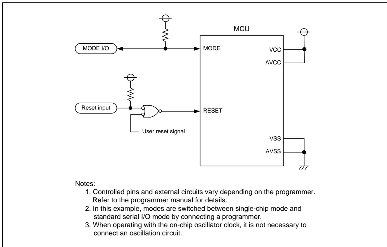
**Figure 29.18 Pin Handling in Standard Serial I/O Mode 3**
