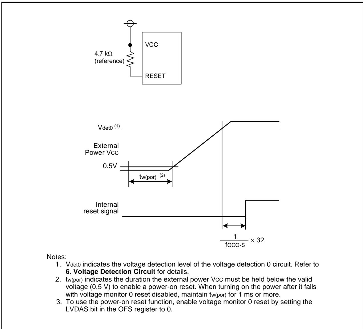
Figure 5.6 Example of Power-On Reset Circuit and Operation
