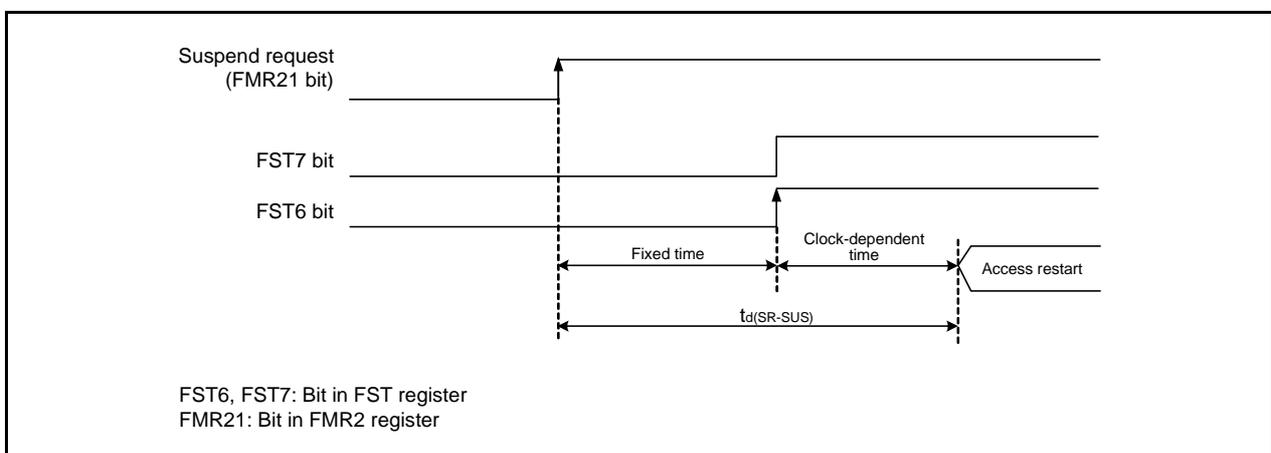
**Figure 31.2 Time delay until Suspend**
