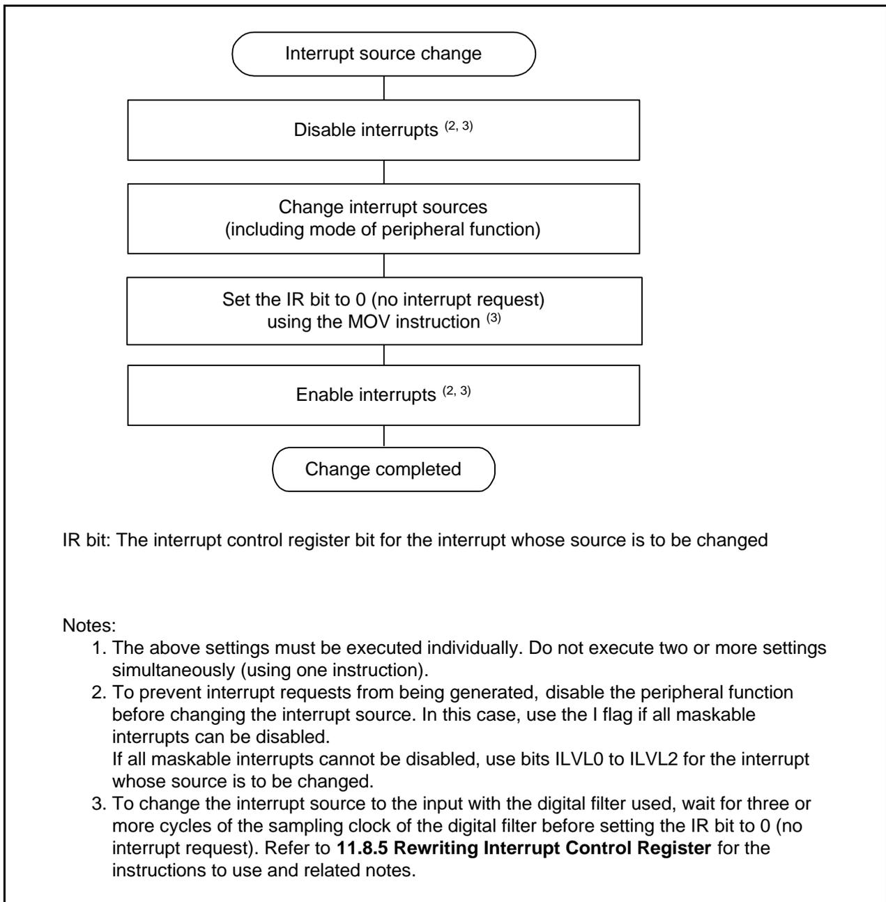
Figure 32.1 Procedure Example for Changing Interrupt Sources
