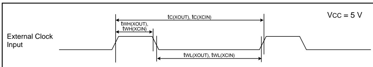
**Figure 31.8 External Clock Input Timing Diagram when  $V_{CC} = 5\text{ V}$** **Table 31.19 TRAI0 Input**
