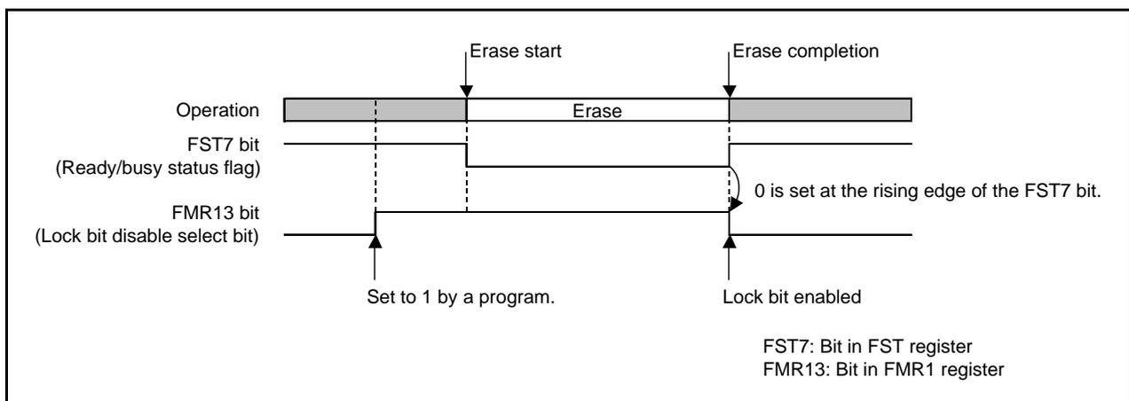
**Figure 29.7 FMR13 Bit Operation Timing**
