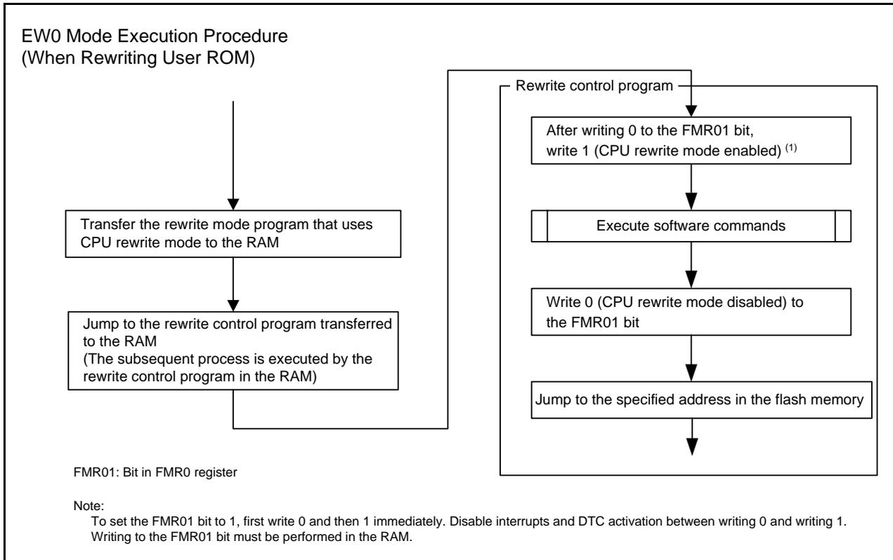
**Figure 29.4 How to Set and Exit EW0 Mode**
