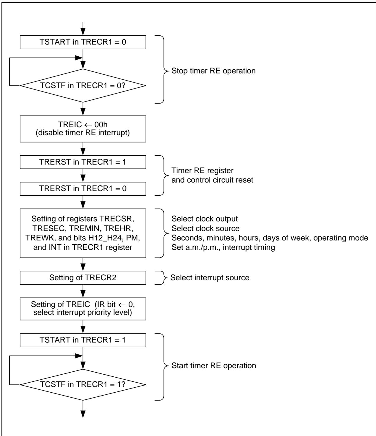
Figure 20.6 Setting Example in Real-Time Clock Mode
