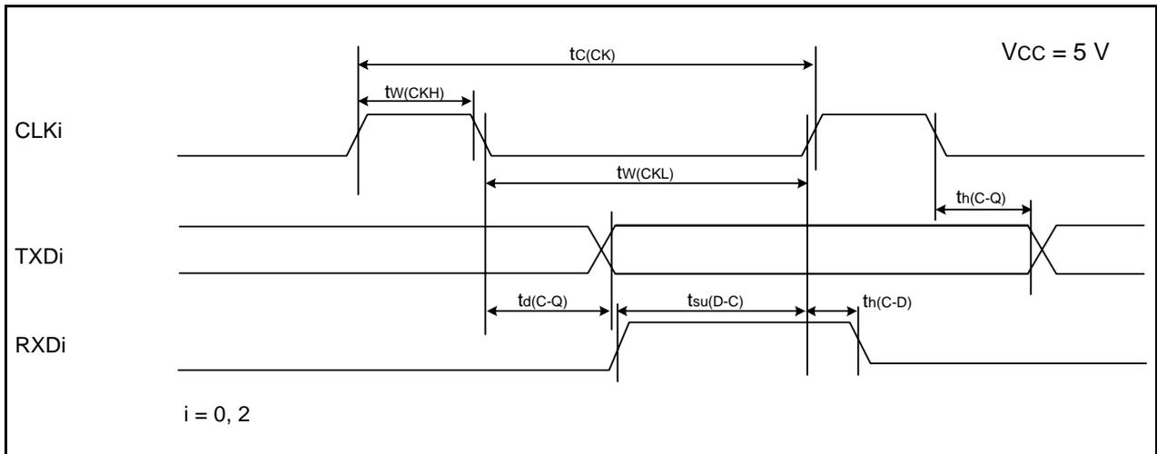
**Figure 31.10 Serial Interface Timing Diagram when  $V_{CC} = 5 V$**
