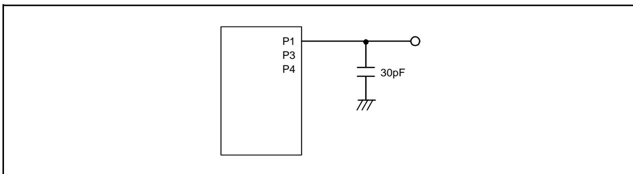
Figure 31.1 Ports P1, P3, P4 Timing Measurement Circuit
