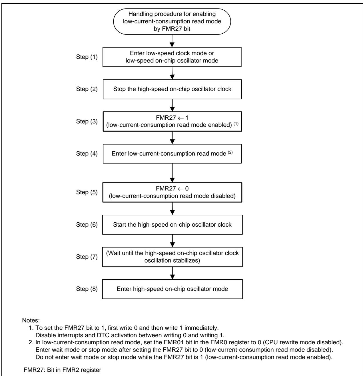
**Figure 30.3 Handling Procedure Example of Low-Current-Consumption Read Mode**
