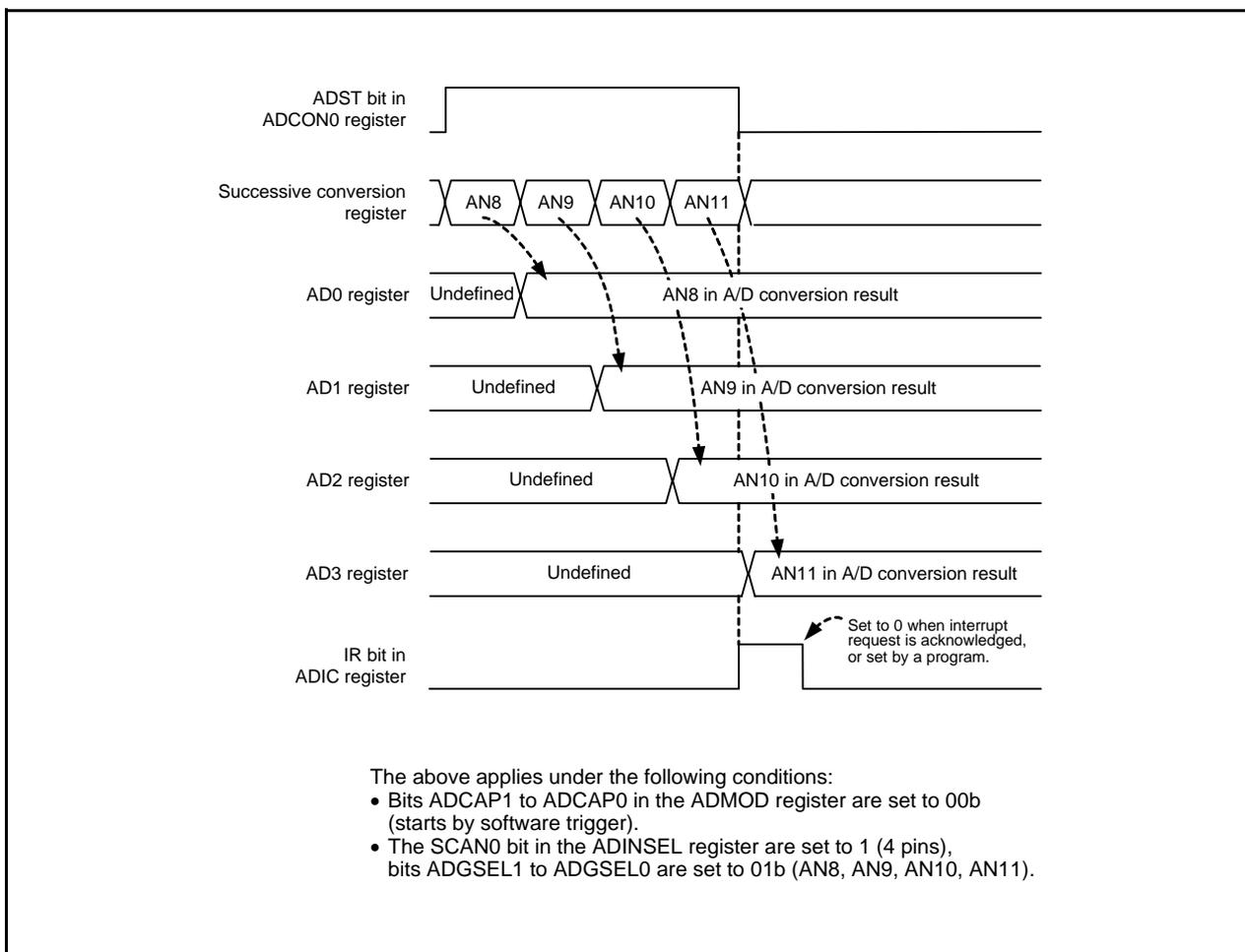
**Figure 27.8** Operating Example of Single Sweep Mode
