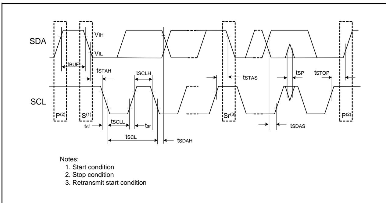
**Figure 31.7 I/O Timing of I<sup>2</sup>C bus Interface**
