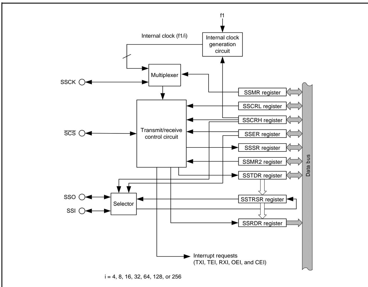
Figure 24.1 Block Diagram of Synchronous Serial Communication Unit
