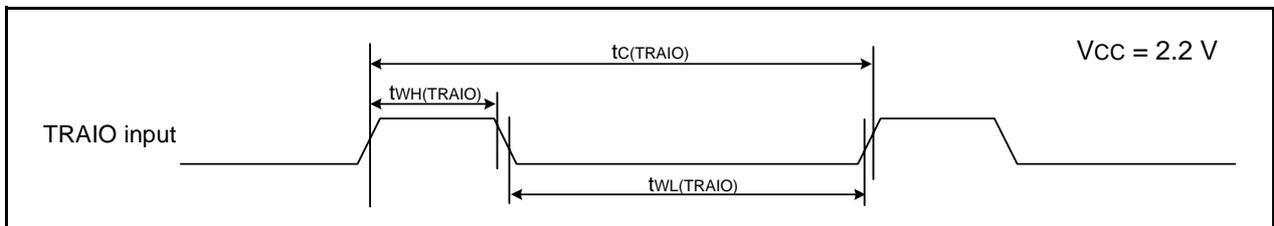
**Figure 31.17 TRAI0 Input Timing Diagram when  $V_{CC} = 2.2\text{ V}$**
