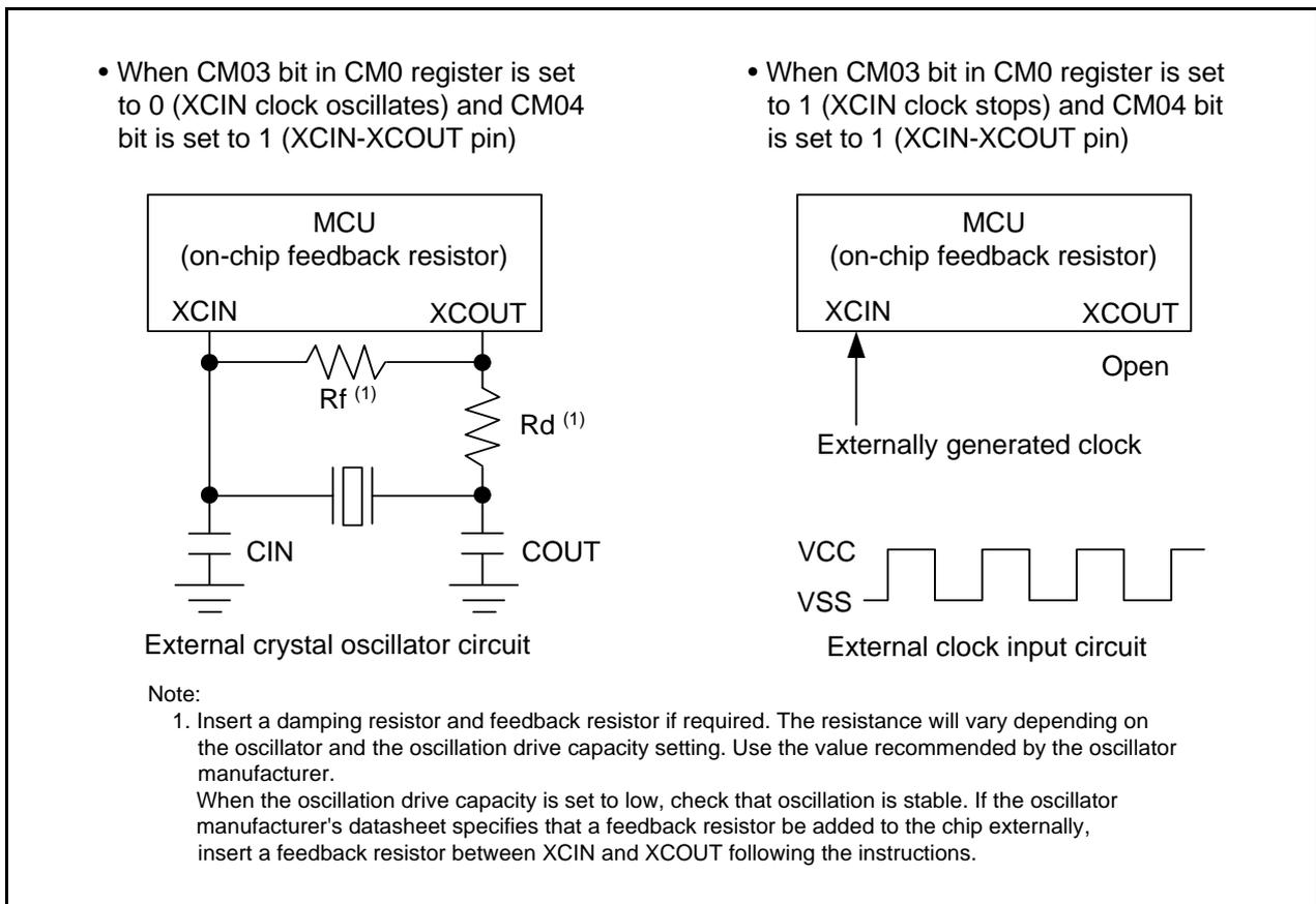
Figure 9.5 Examples of XCIN Clock Connection Circuits
