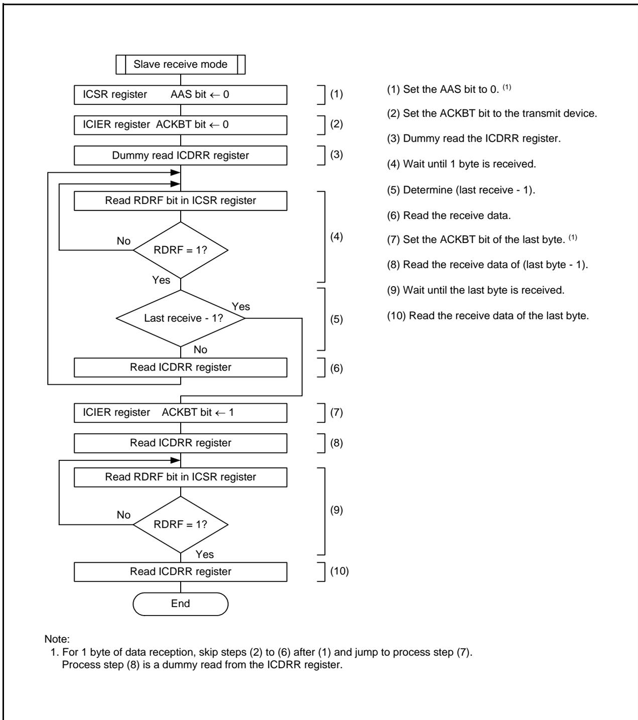
**Figure 25.19 Register Setting Example in Slave Receive Mode (I<sup>2</sup>C bus Interface Mode)**
