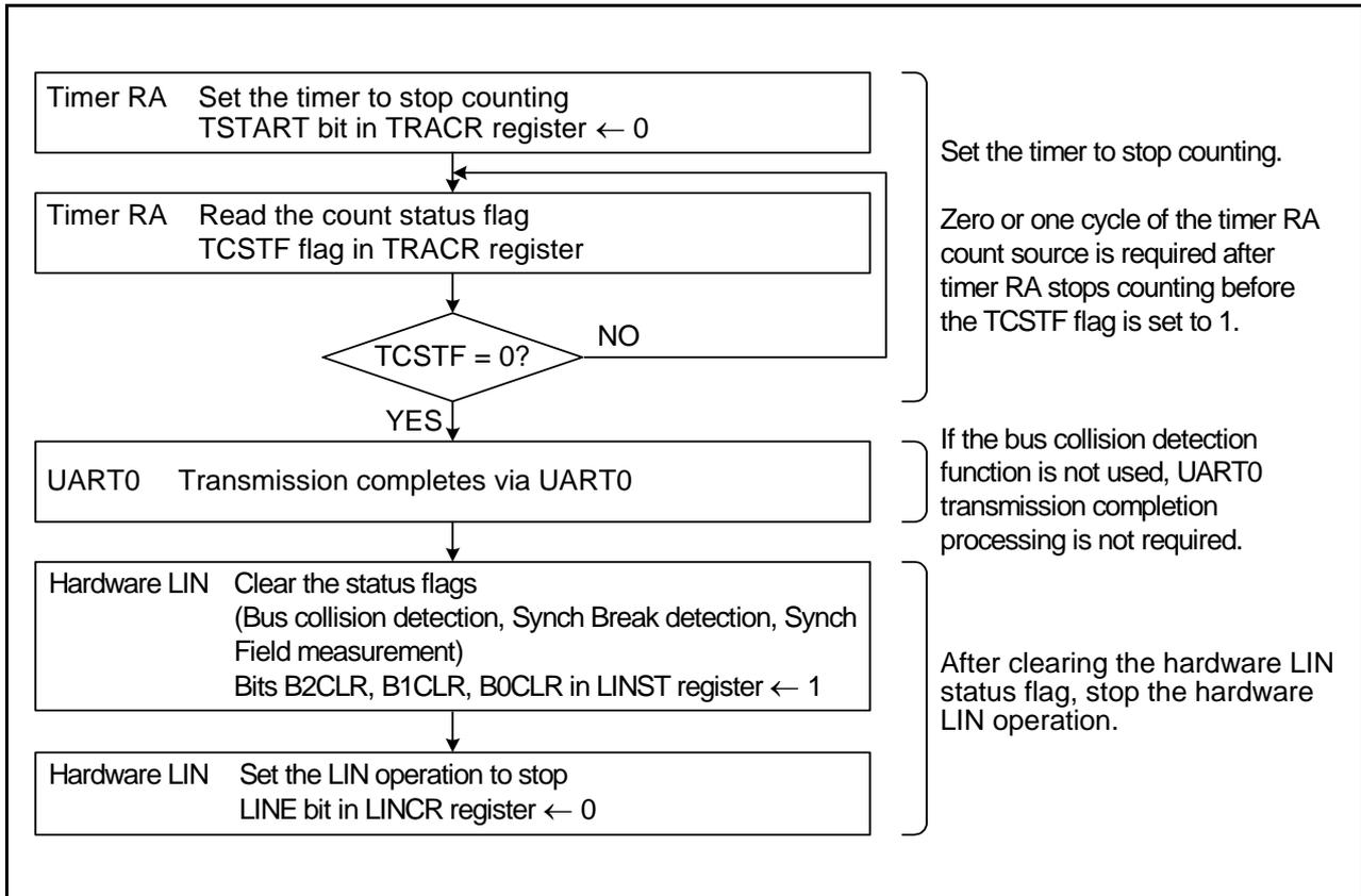
Figure 26.10 Example of Hardware LIN Communication Completion Flowchart
