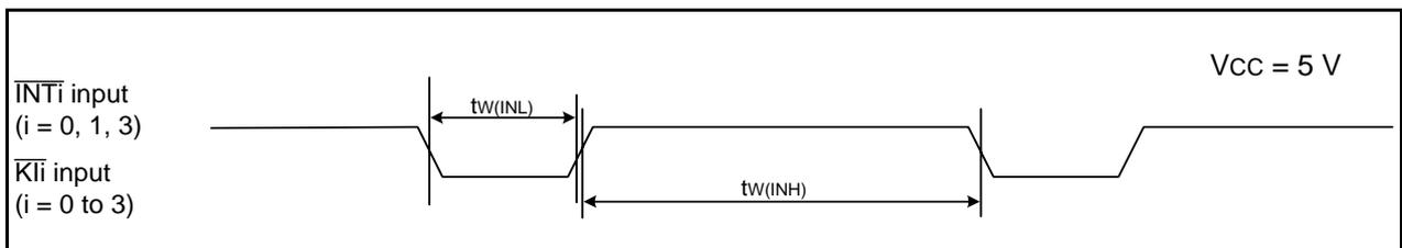
**Figure 31.11 Input Timing Diagram for External Interrupt  $\overline{INT}_i$  and Key Input Interrupt  $\overline{K}_i$  when  $V_{CC} = 5 V$**
