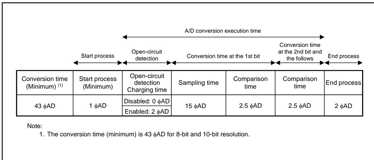
Figure 27.3 A/D Conversion Cycles ( $\phi_{AD} = f_{AD}$ )
