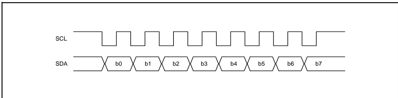
**Figure 25.13** Transfer Format of Clock Synchronous Serial Format
