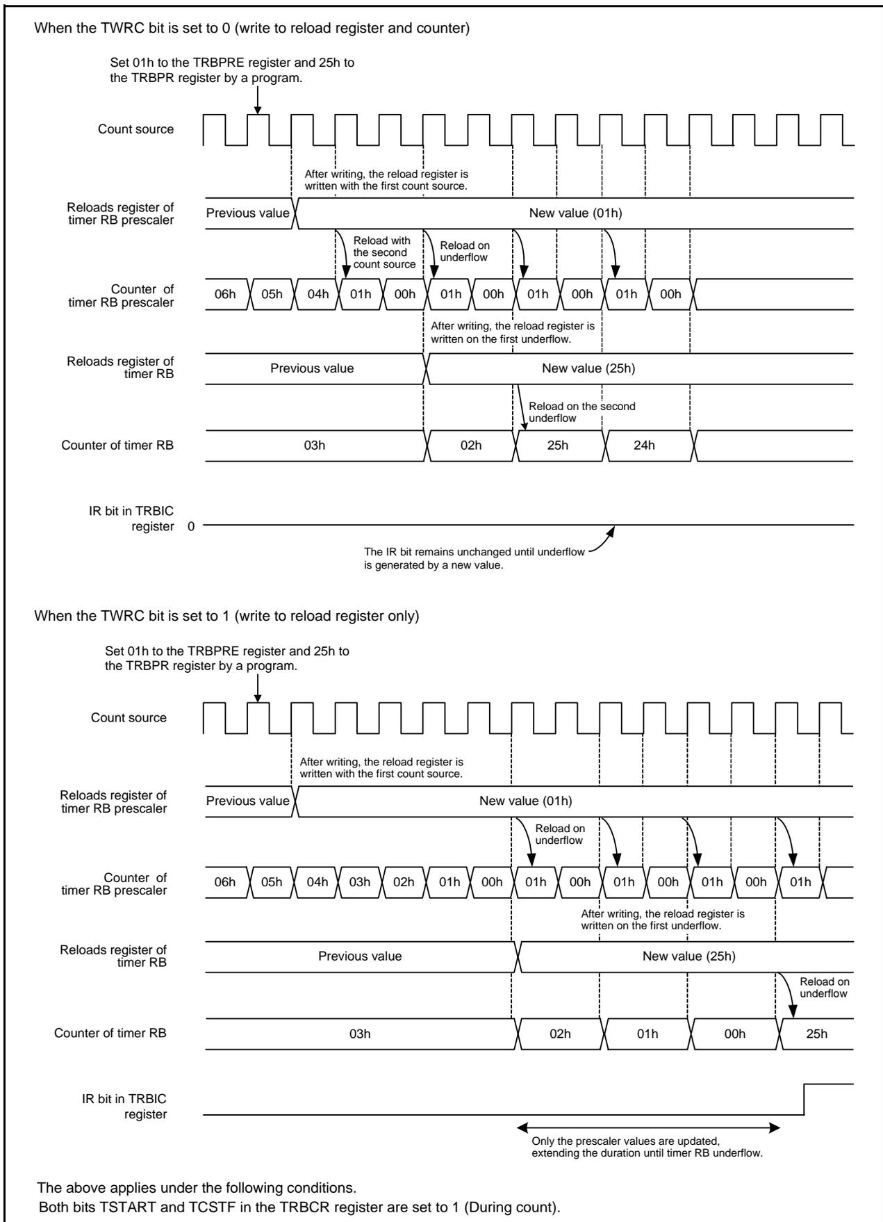
**Figure 18.2 Operating Example of Timer RB when Counter Value is Rewritten during Count Operation**
