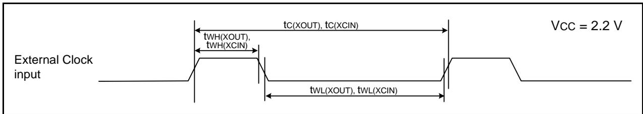
**Figure 31.16 External Clock Input Timing Diagram when  $V_{CC} = 2.2\text{ V}$** **Table 31.31 TRAI0 Input**
