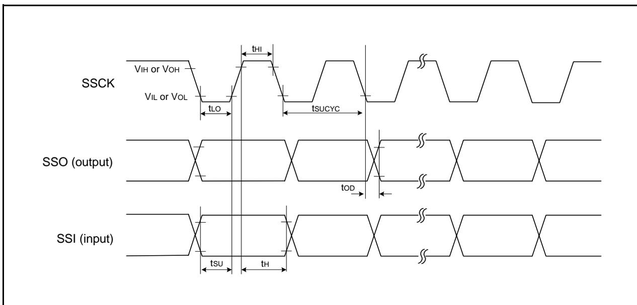
**Figure 31.6 I/O Timing of Synchronous Serial Communication Unit (SSU) (Clock Synchronous Communication Mode)**
