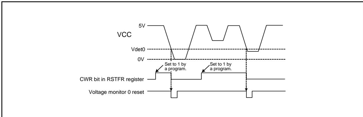
Figure 5.8 Operating Example of Cold Start-Up/Warm Start-Up Function
