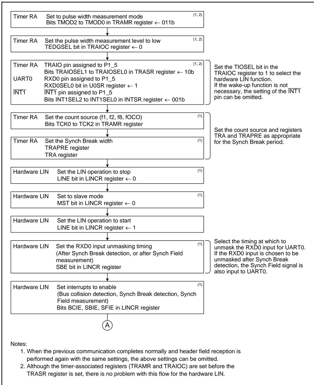
Figure 26.6 Header Field Reception Flowchart Example (1)
