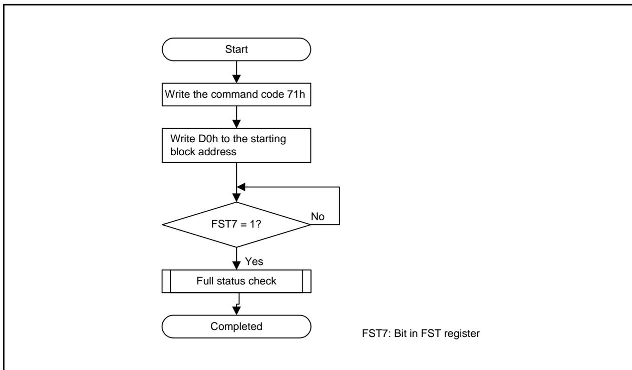
Figure 29.14 Read Lock Bit Status Flowchart
