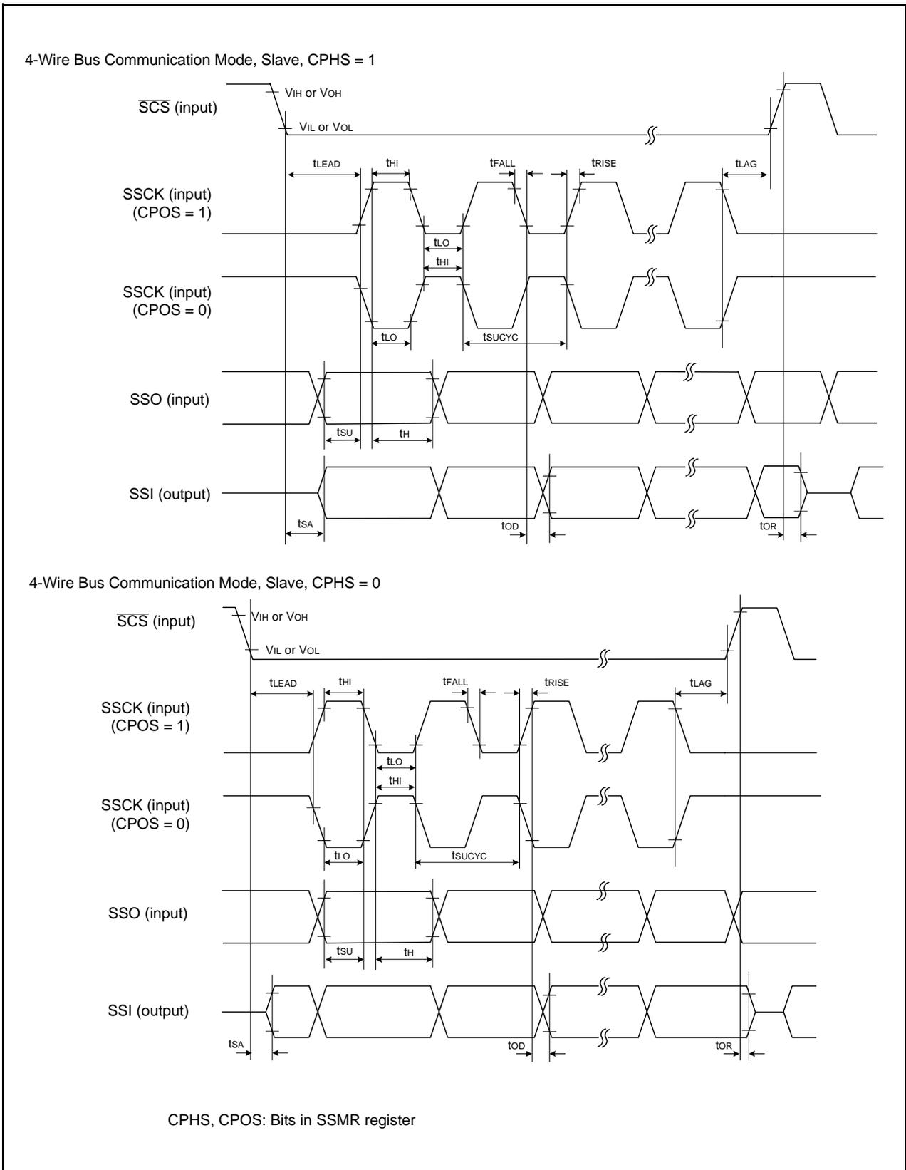
Figure 31.5 I/O Timing of Synchronous Serial Communication Unit (SSU) (Slave)
