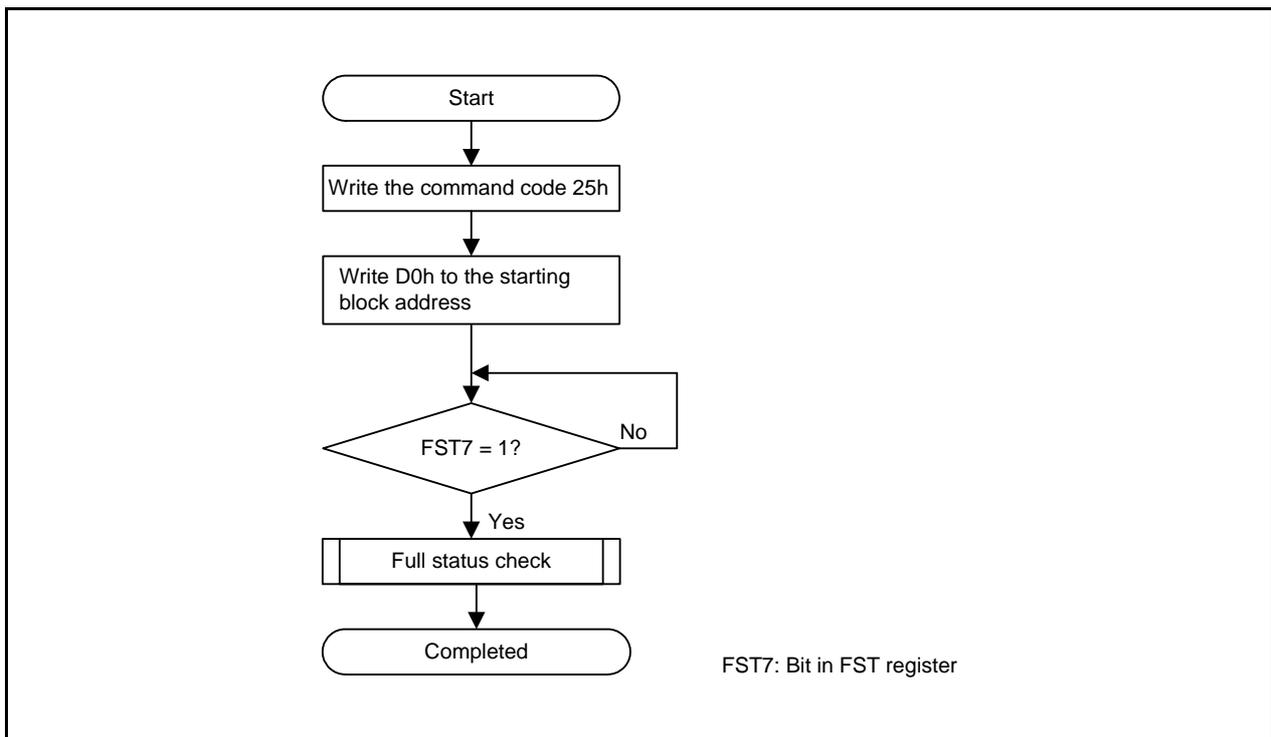
**Figure 29.15** Block Blank Check Flowchart
