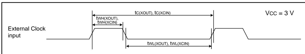
**Figure 31.12 External Clock Input Timing Diagram when  $V_{CC} = 3\text{ V}$** **Table 31.25 TRAI0 Input**
