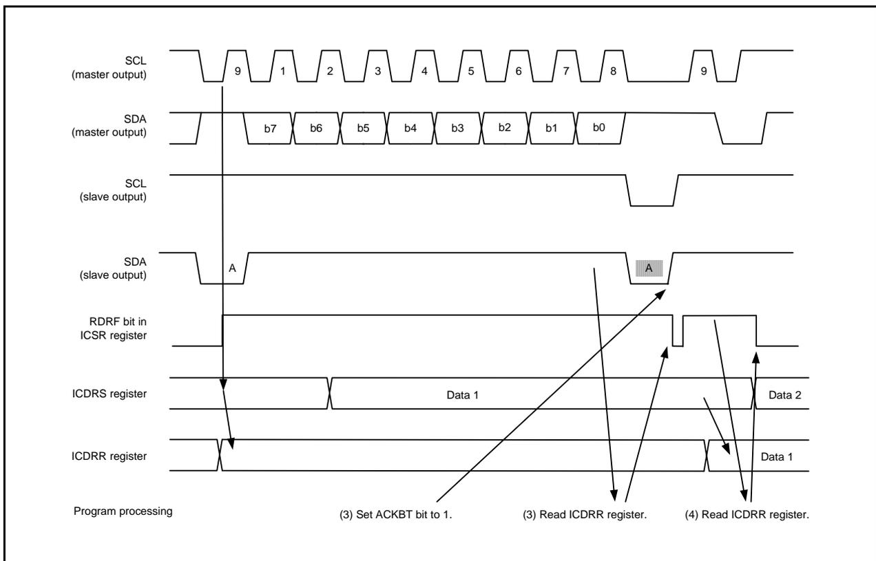
Figure 25.12 Operating Timing in Slave Receive Mode (I<sup>2</sup>C bus Interface Mode) (2)
