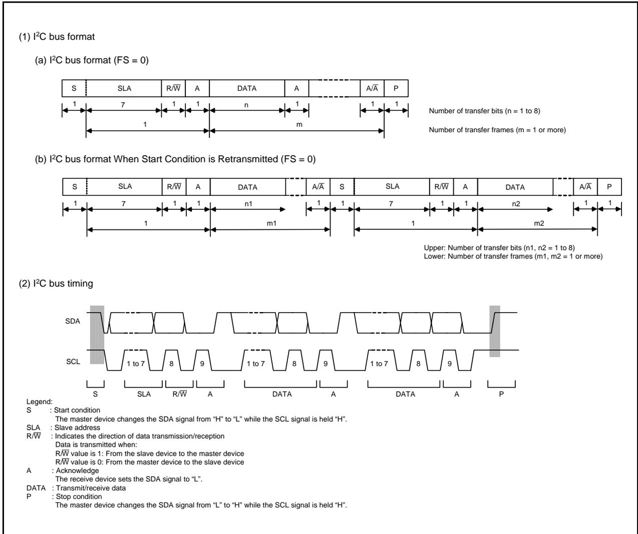
Figure 25.4 I<sup>2</sup>C bus Format and Bus Timing
