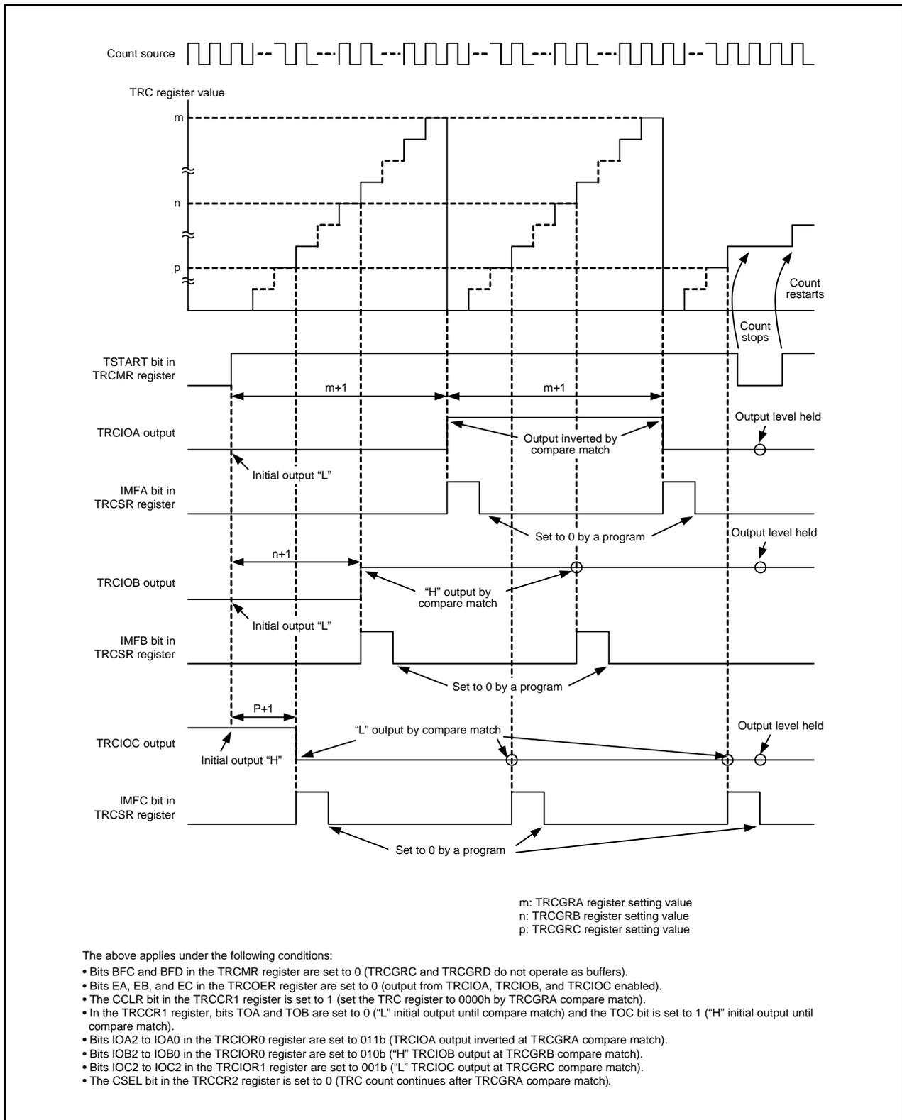
Figure 19.10 Operating Example of Output Compare Function
