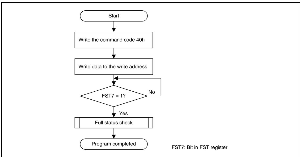
**Figure 29.8** Program Flowchart (Flash Ready Status Interrupt Disabled)
