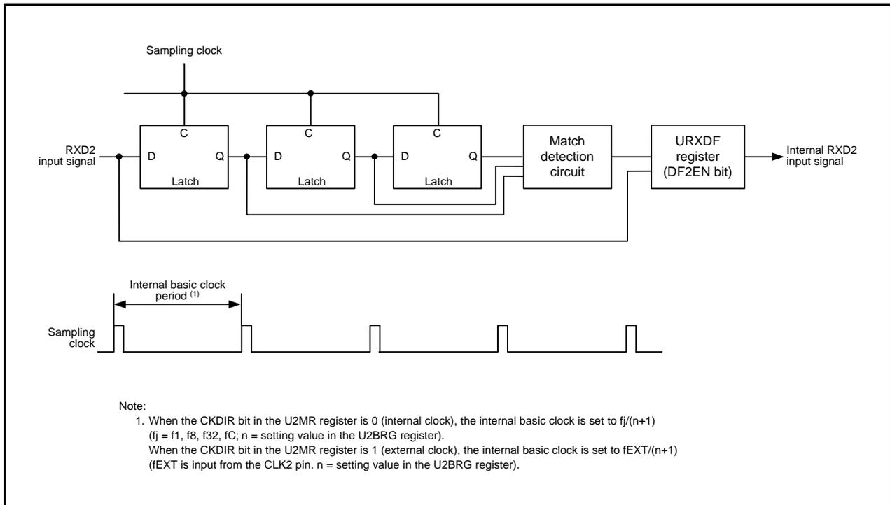
Figure 22.22 Block Diagram of RXD2 Digital Filter Circuit
