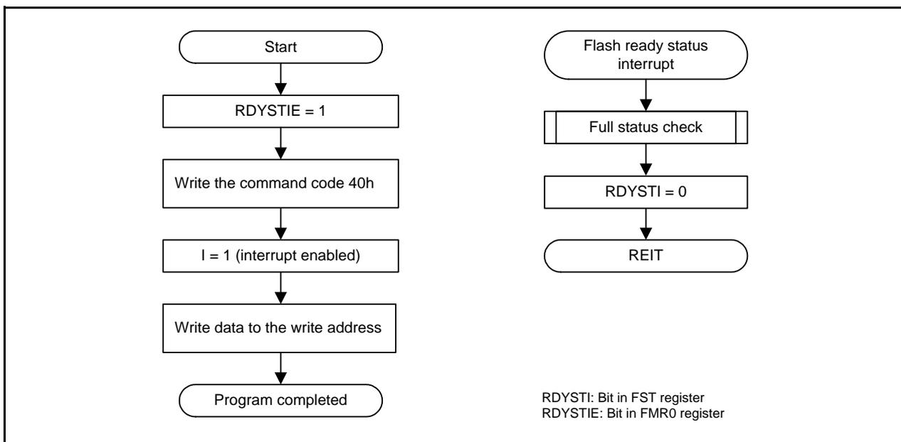
Figure 29.9 Program Flowchart (Flash Ready Status Interrupt Enabled)
