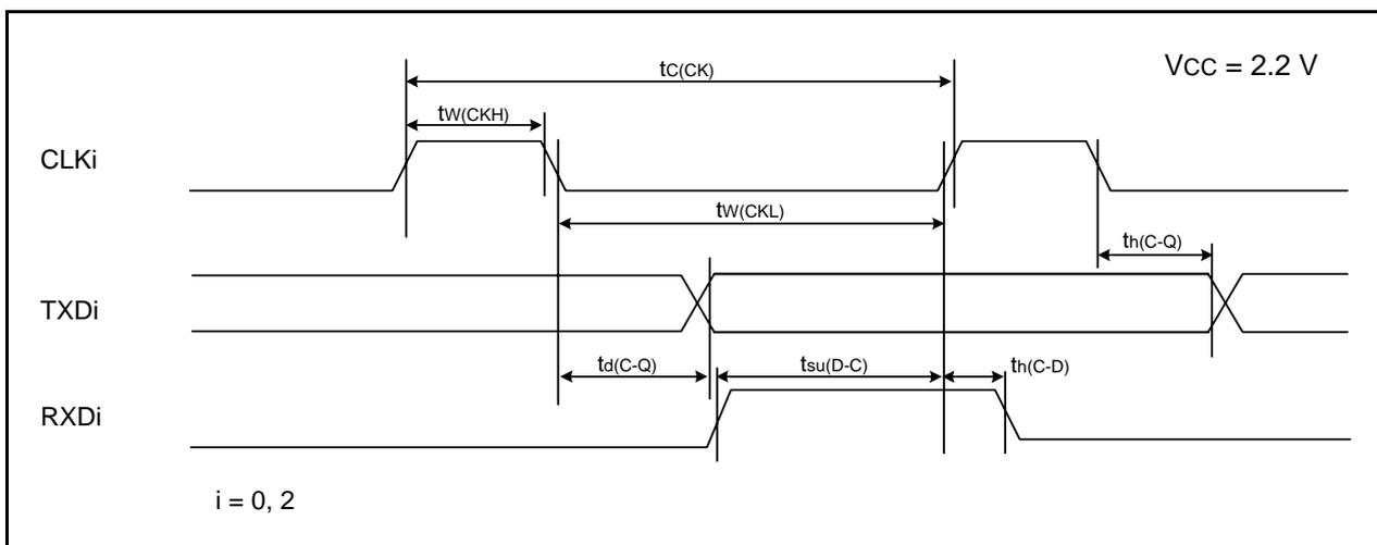
**Figure 31.18 Serial Interface Timing Diagram when  $V_{CC} = 2.2\text{ V}$**
