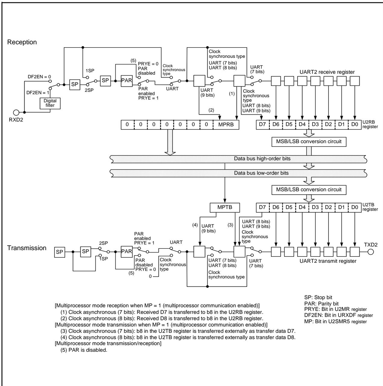
Figure 22.18 Block Diagram of Multiprocessor Communication Function
