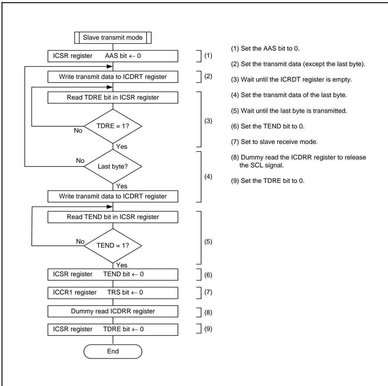
Figure 25.18 Register Setting Example in Slave Transmit Mode (I<sup>2</sup>C bus Interface Mode)
