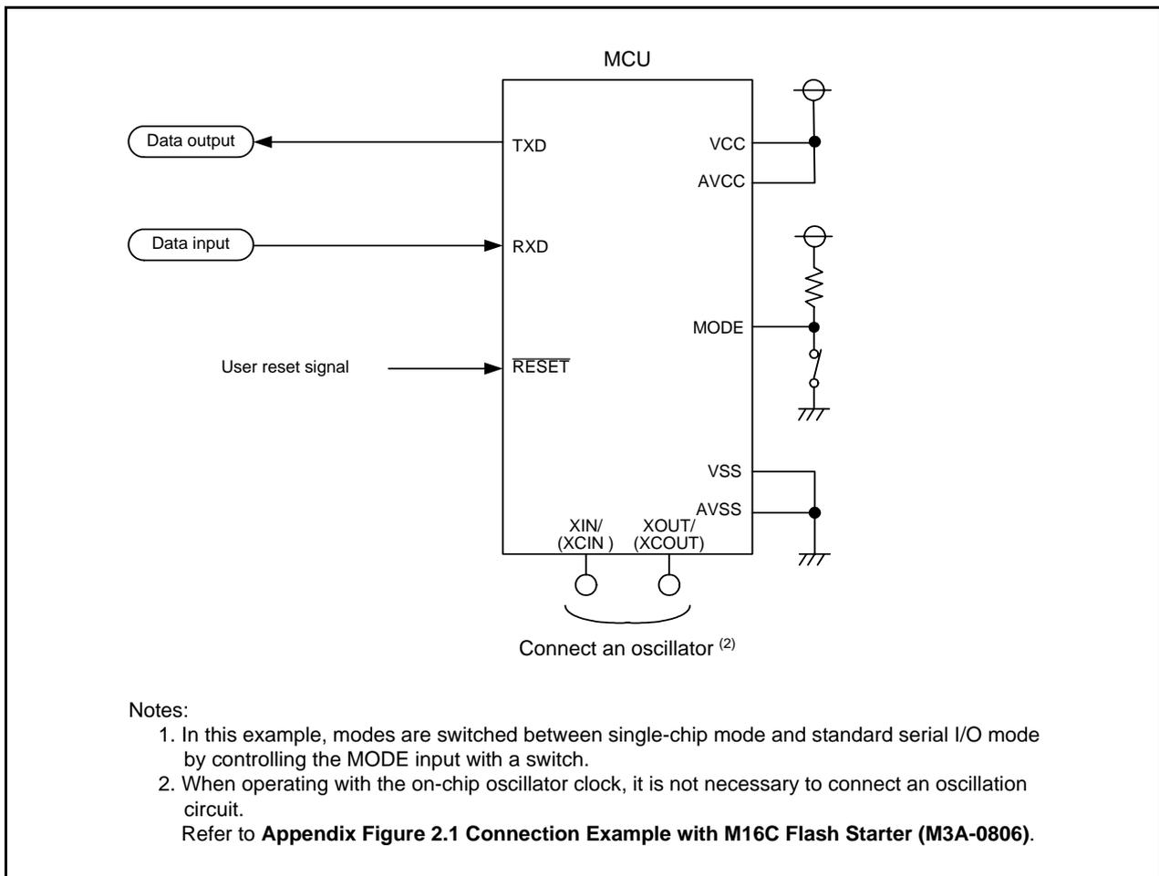
**Figure 29.17 Pin Handling in Standard Serial I/O Mode 2**
