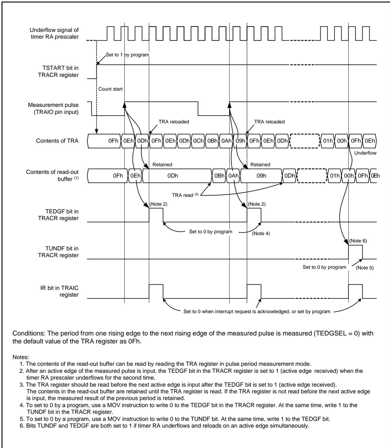
**Figure 17.4 Operating Example of Pulse Period Measurement Mode**
