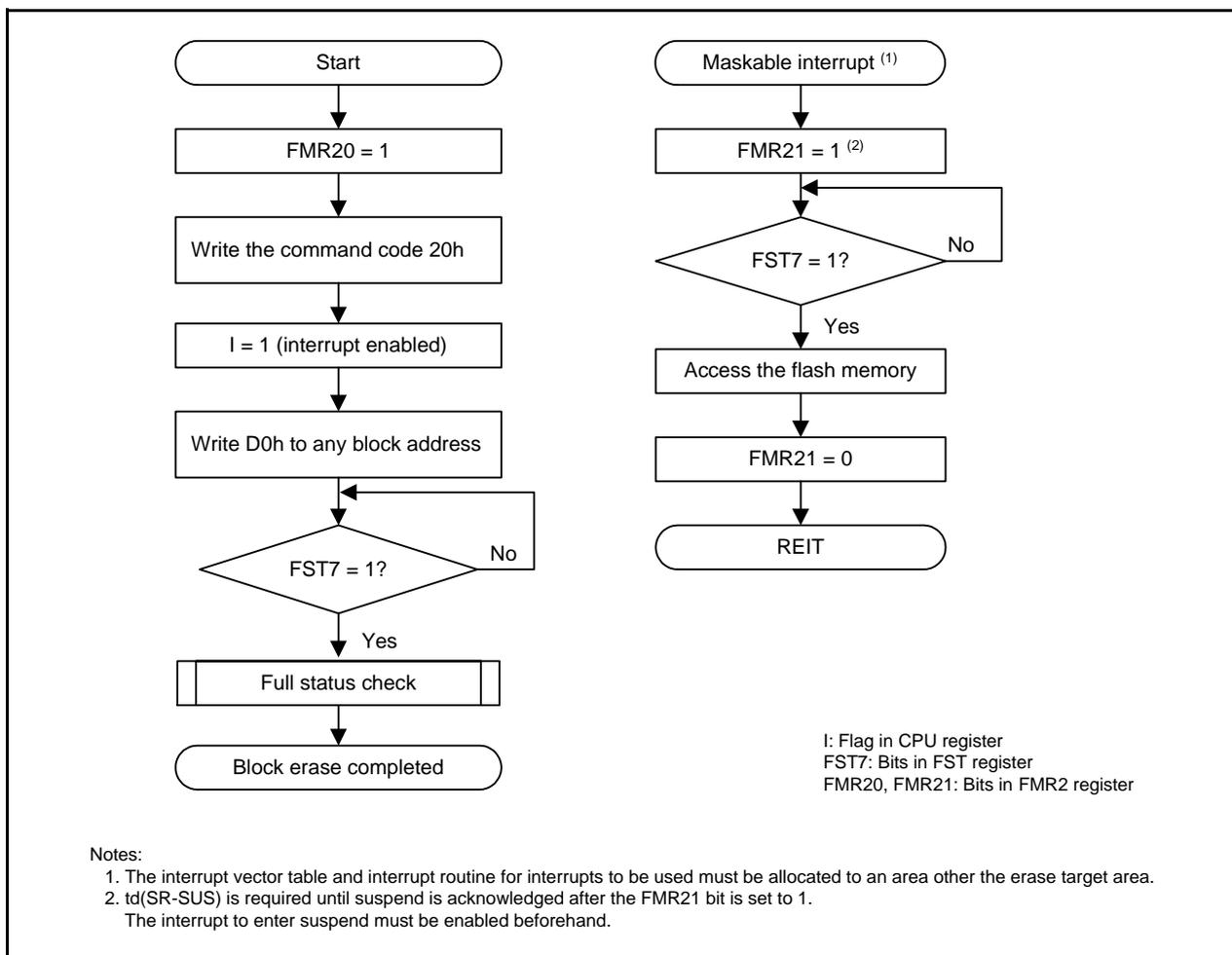
Figure 29.11 Block Erase Flowchart (Flash Ready Status Interrupt Disabled and Suspend Enabled)
