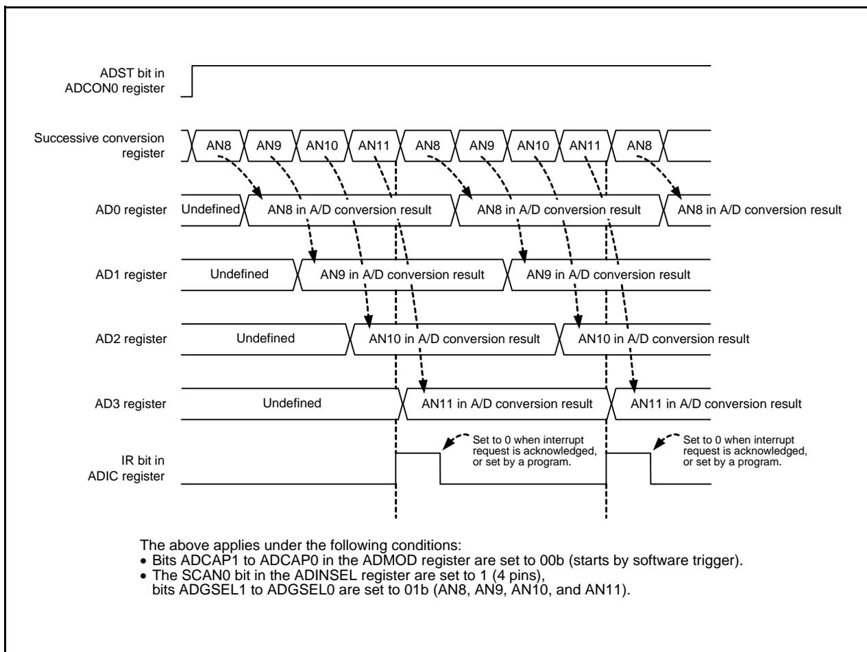
**Figure 27.9** Operating Example of Repeat Sweep Mode
