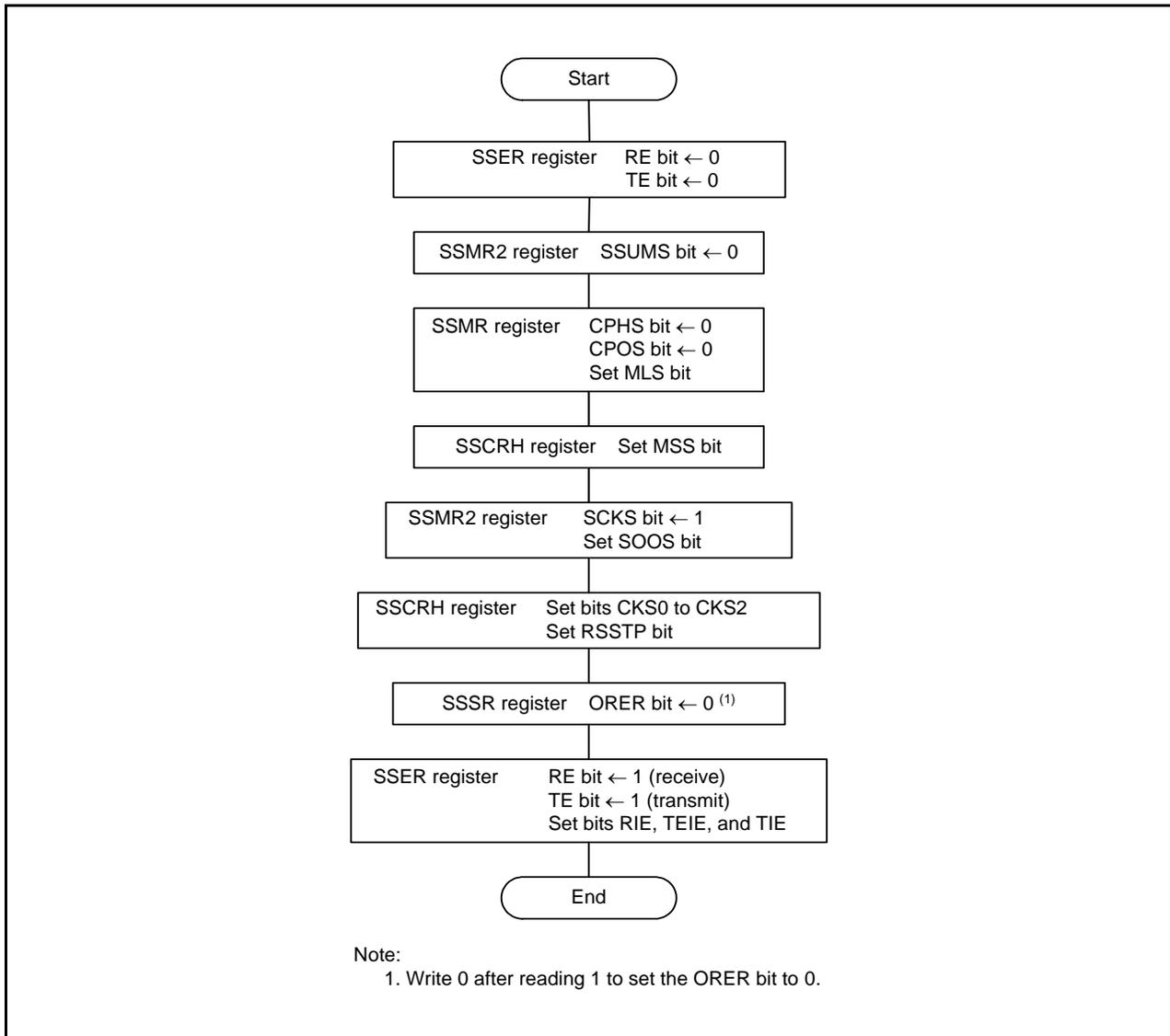
Figure 24.4 Initialization in Clock Synchronous Communication Mode
