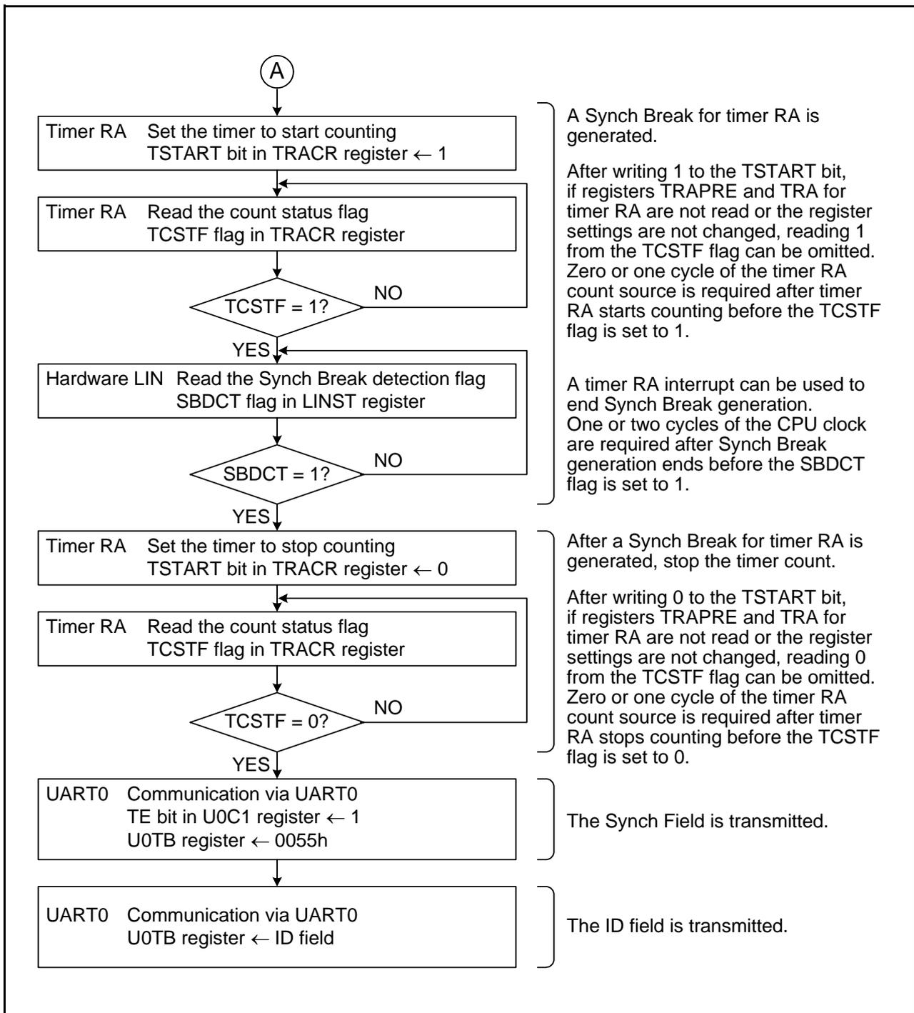
Figure 26.4 Header Field Transmission Flowchart Example (2)
