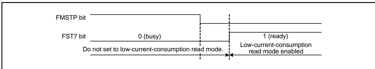
Figure 29.2 Transition to Low-Current-Consumption Read Mode
