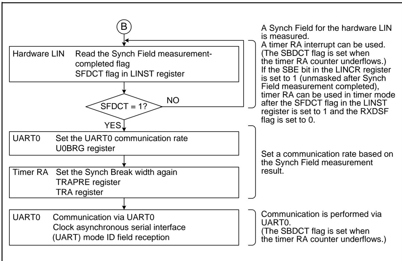
Figure 26.8 Header Field Reception Flowchart Example (3)
