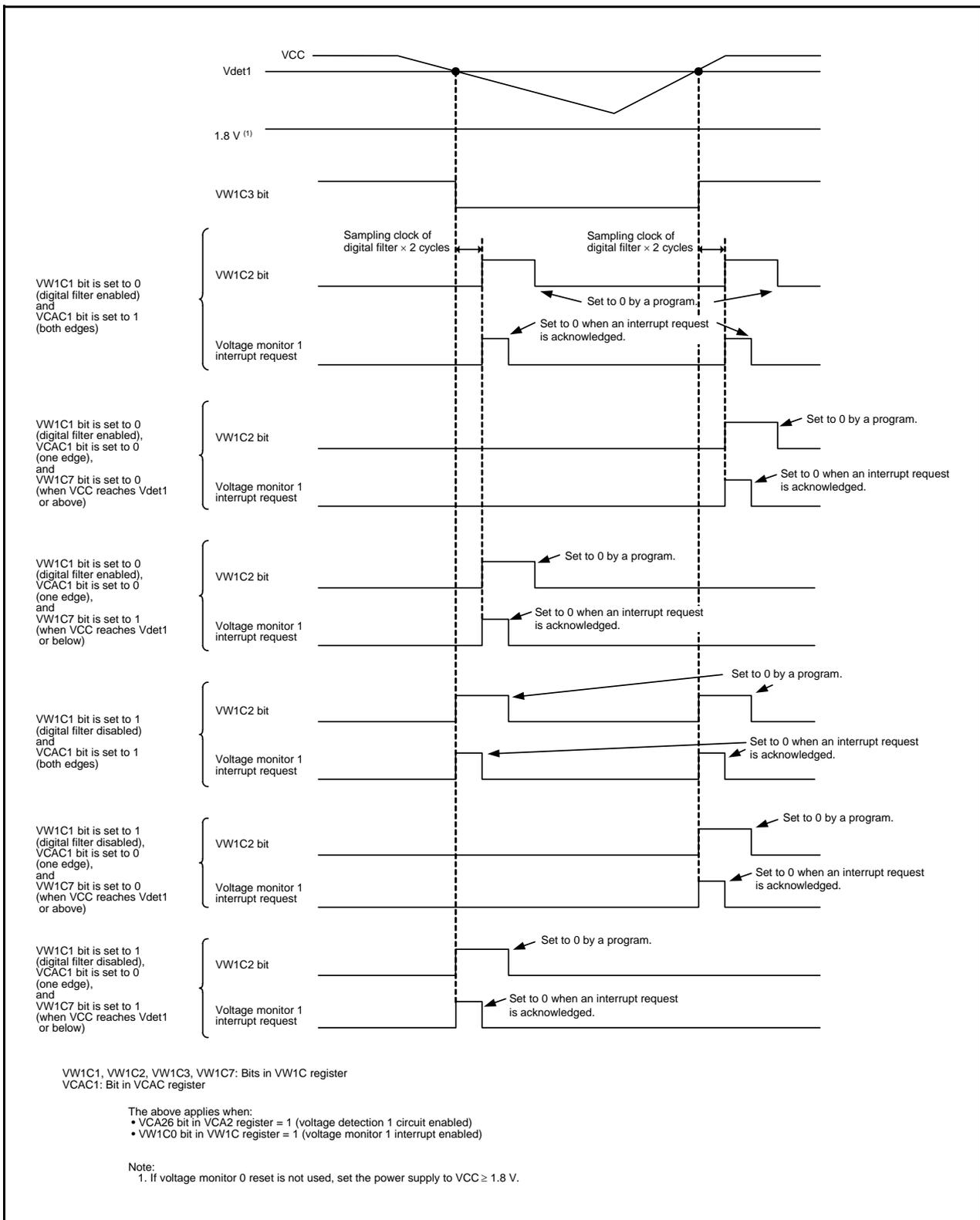
Figure 6.6 Operating Example of Voltage Monitor 1 Interrupt
