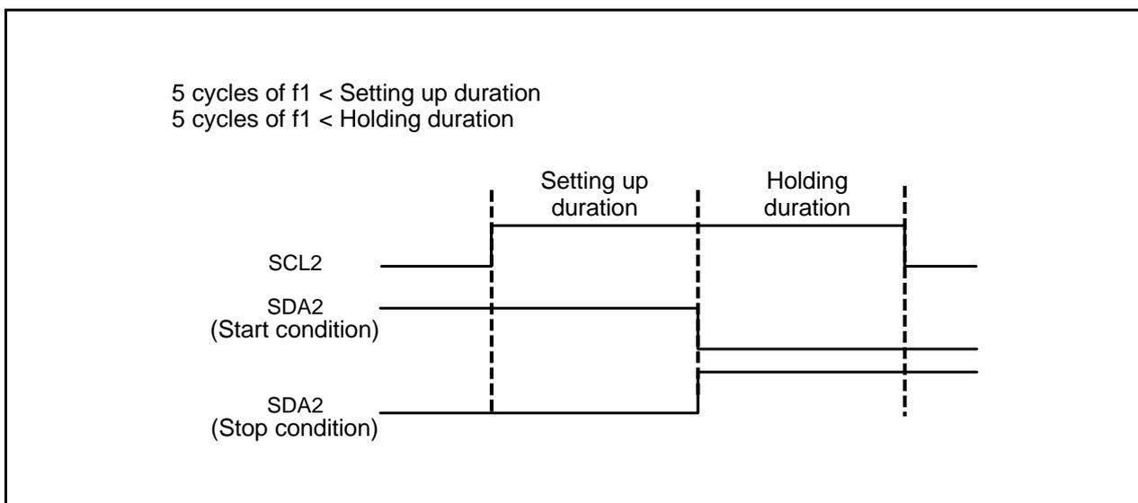
Figure 22.15 Detection of Start and Stop Conditions
