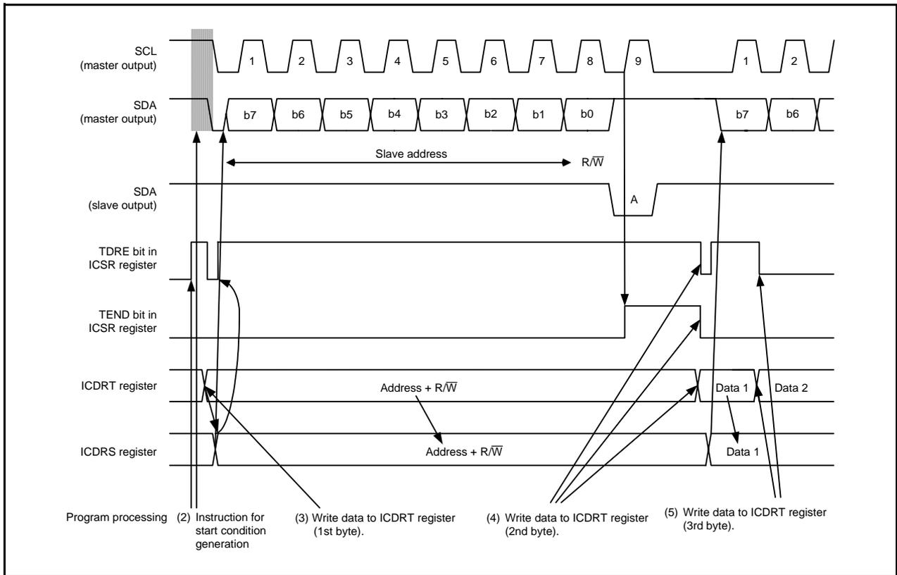
Figure 25.5 Operating Timing in Master Transmit Mode (I<sup>2</sup>C bus Interface Mode) (1)
