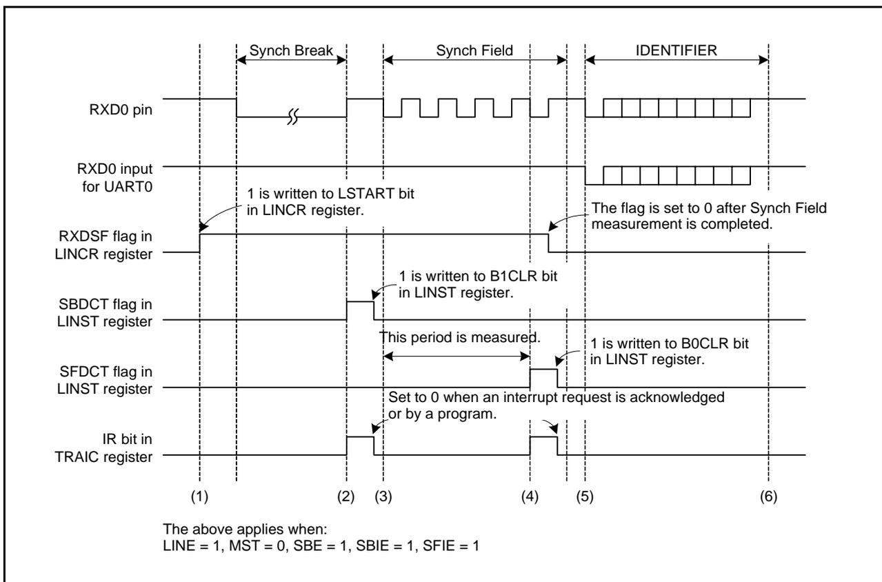
Figure 26.5 Operating Example during Header Field Reception
