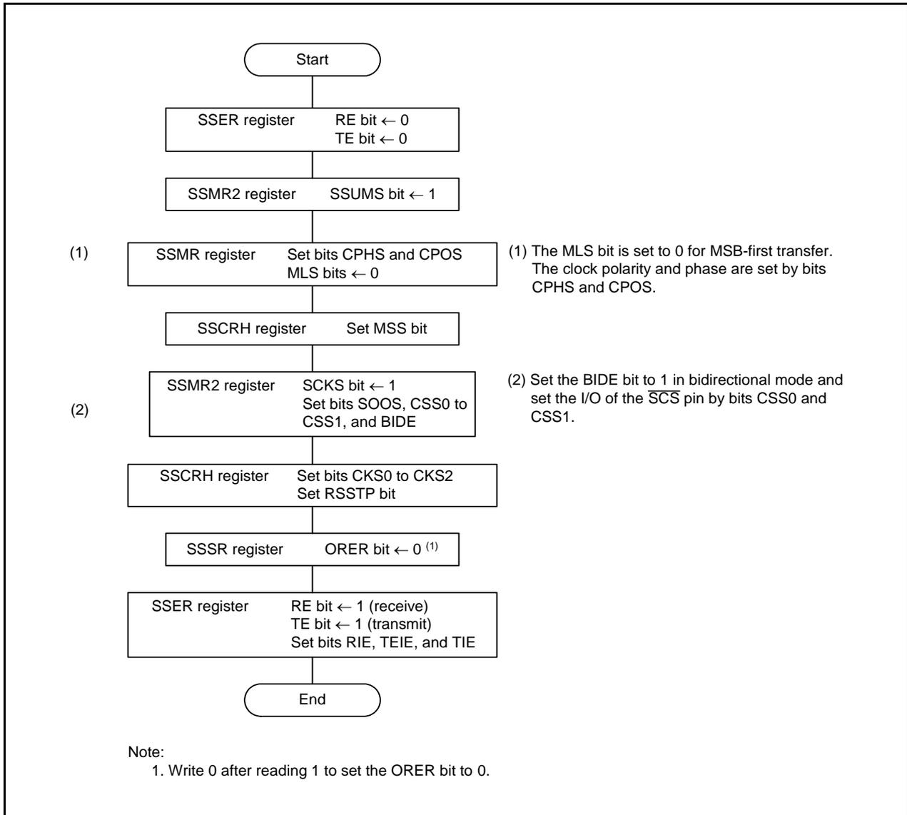
Figure 24.10 Initialization in 4-Wire Bus Communication Mode
