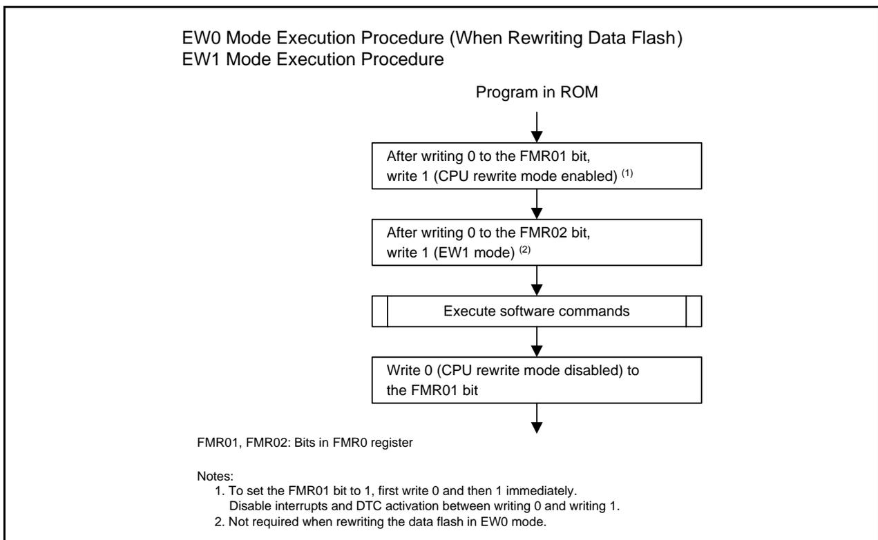
**Figure 29.5 How to Set and Exit EW0 Mode (When Rewriting Data Flash) and EW1 Mode**
