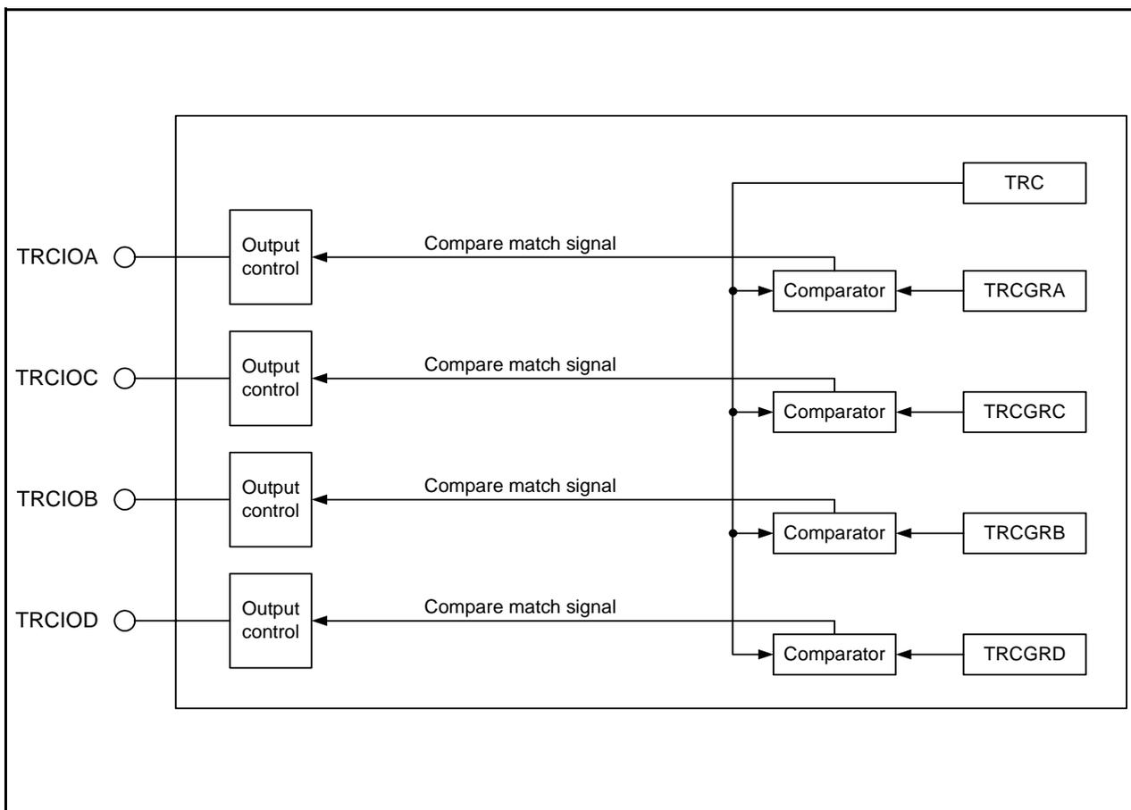
Figure 19.9 Block Diagram of Output Compare Function
