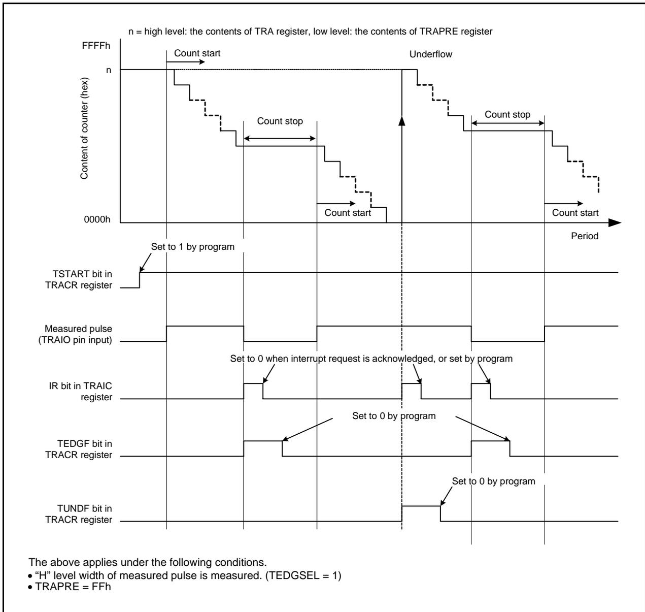
Figure 17.3 Operating Example of Pulse Width Measurement Mode
