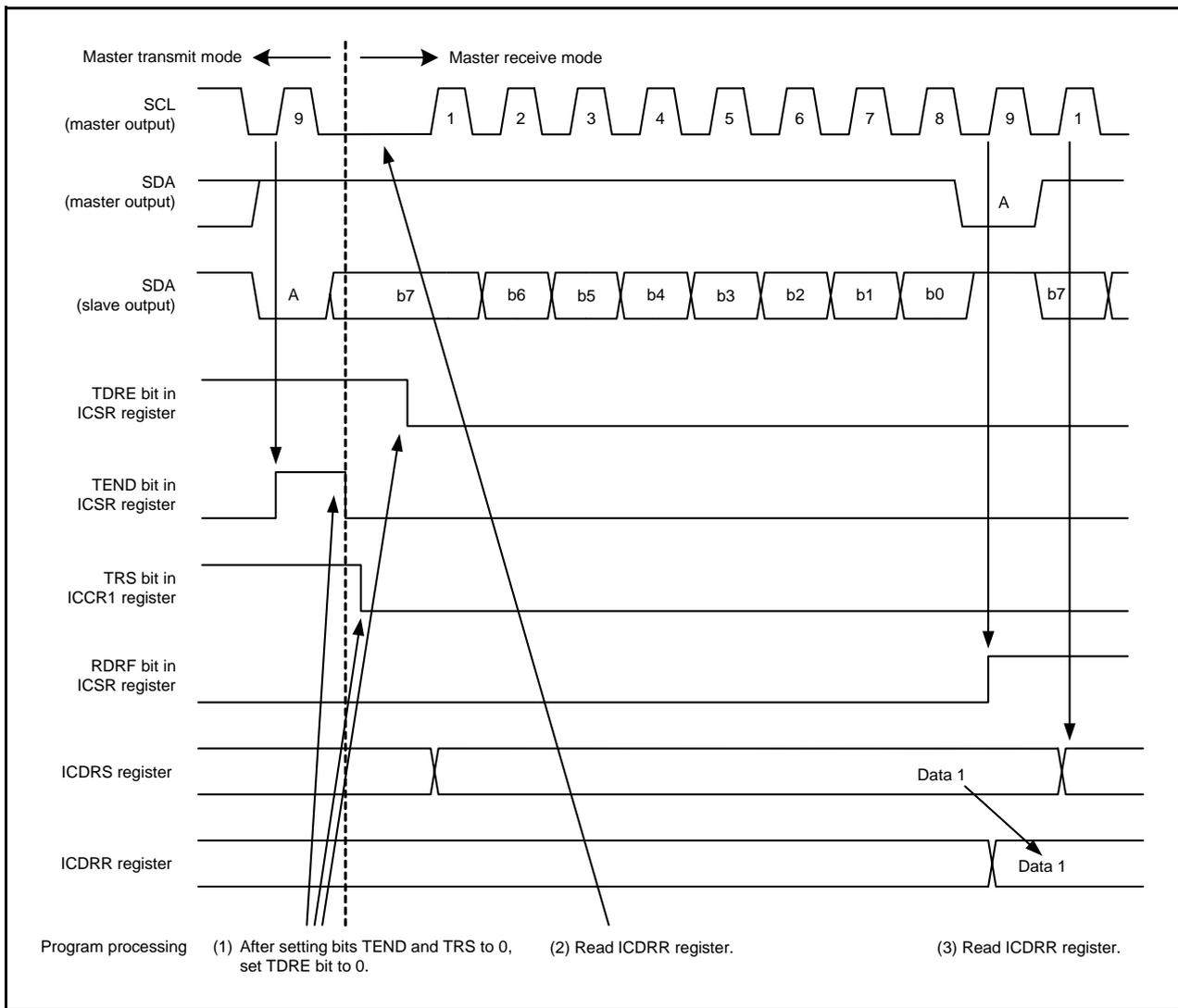
**Figure 25.7 Operating Timing in Master Receive Mode (I<sup>2</sup>C bus Interface Mode) (1)**
