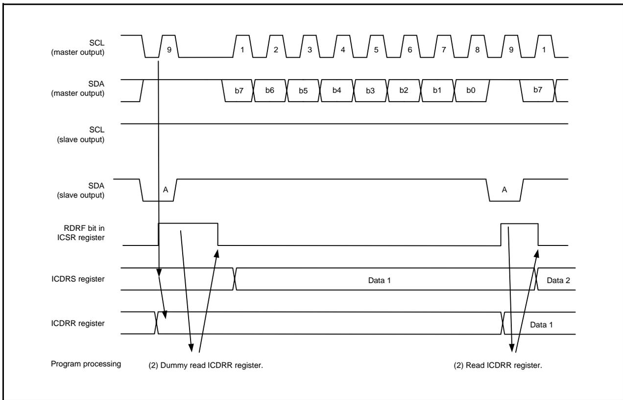
Figure 25.11 Operating Timing in Slave Receive Mode (I<sup>2</sup>C bus Interface Mode) (1)
