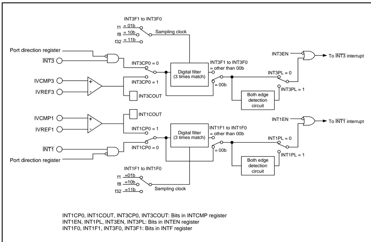
**Figure 28.1 Comparator B Block Diagram**
