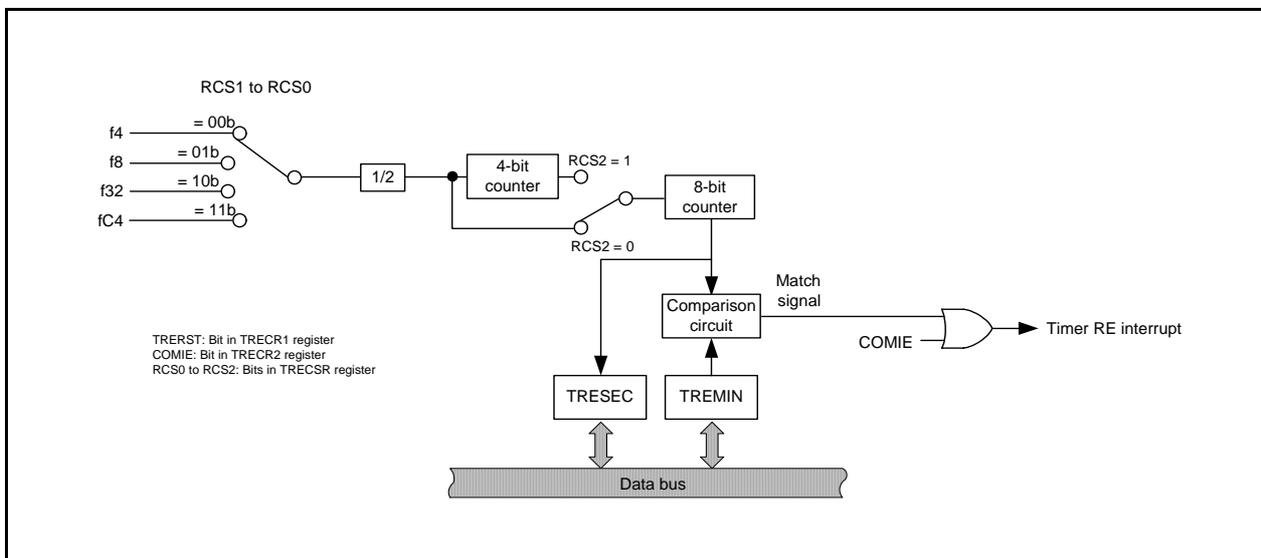
Figure 20.4 Block Diagram of Output Compare Mode
