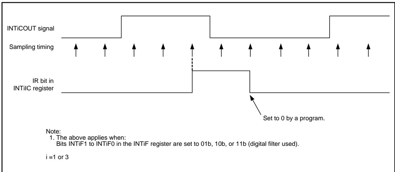
**Figure 28.4 Operating Example of Comparator Bi Digital Filter**
