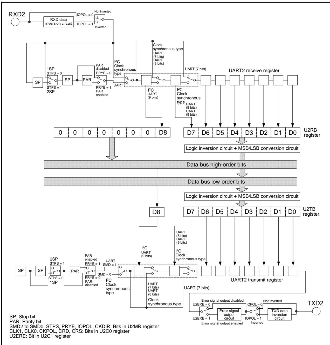
Figure 22.2 Block Diagram of UART2 Transmit/Receive Unit
