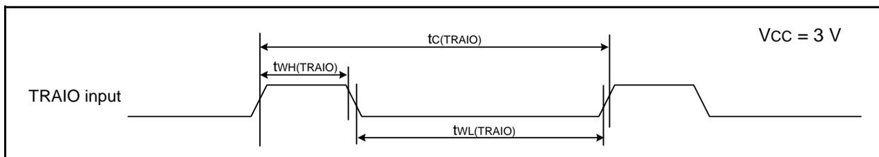
**Figure 31.13 TRAI0 Input Timing Diagram when  $V_{CC} = 3\text{ V}$**
