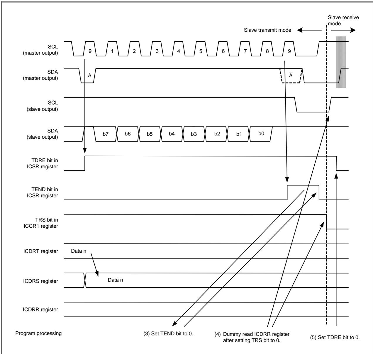
Figure 25.10 Operating Timing in Slave Transmit Mode (I<sup>2</sup>C bus Interface Mode) (2)
