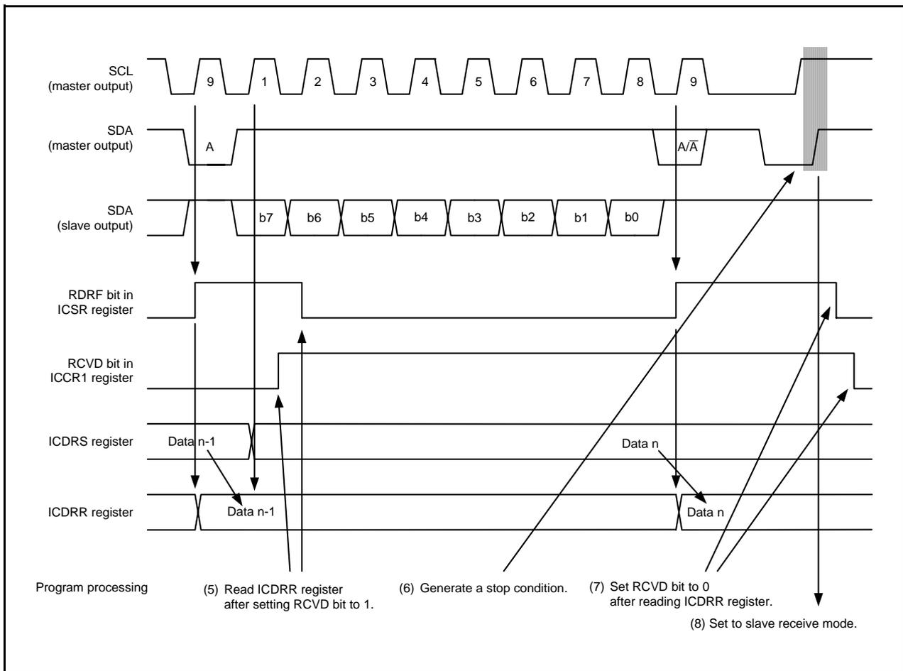
**Figure 25.8 Operating Timing in Master Receive Mode (I<sup>2</sup>C bus Interface Mode) (2)**
