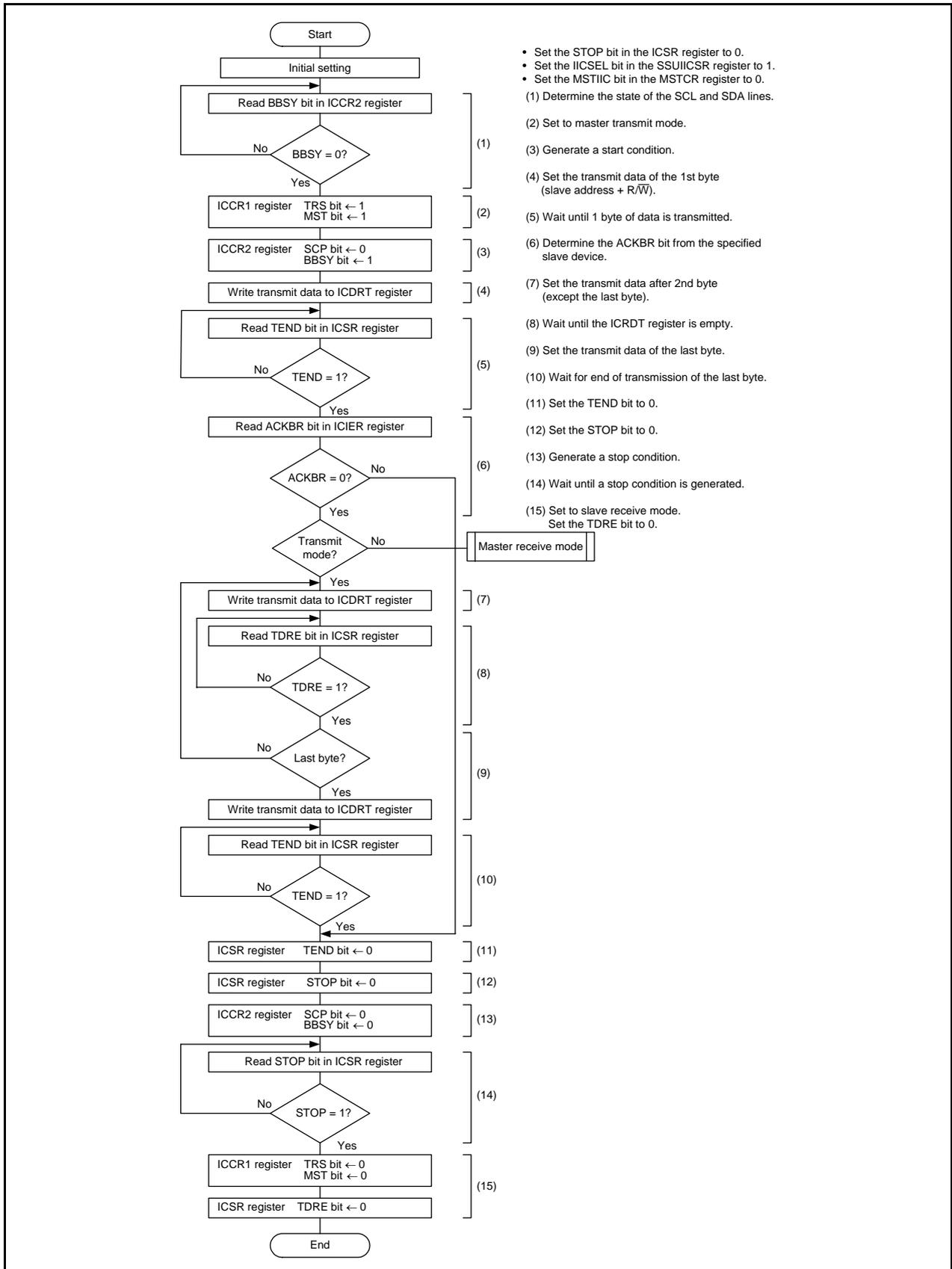
Figure 25.16 Register Setting Example in Master Transmit Mode (I<sup>2</sup>C bus Interface Mode)
