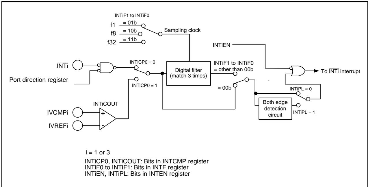
**Figure 28.3 Configuration of Comparator Bi Digital Filter**
