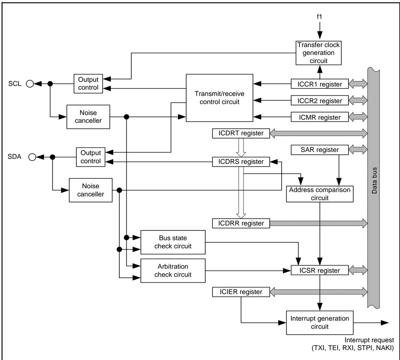
Figure 25.1 I<sup>2</sup>C bus interface Block Diagram
