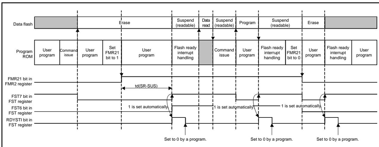
**Figure 29.3 Suspend Operation Timing**
