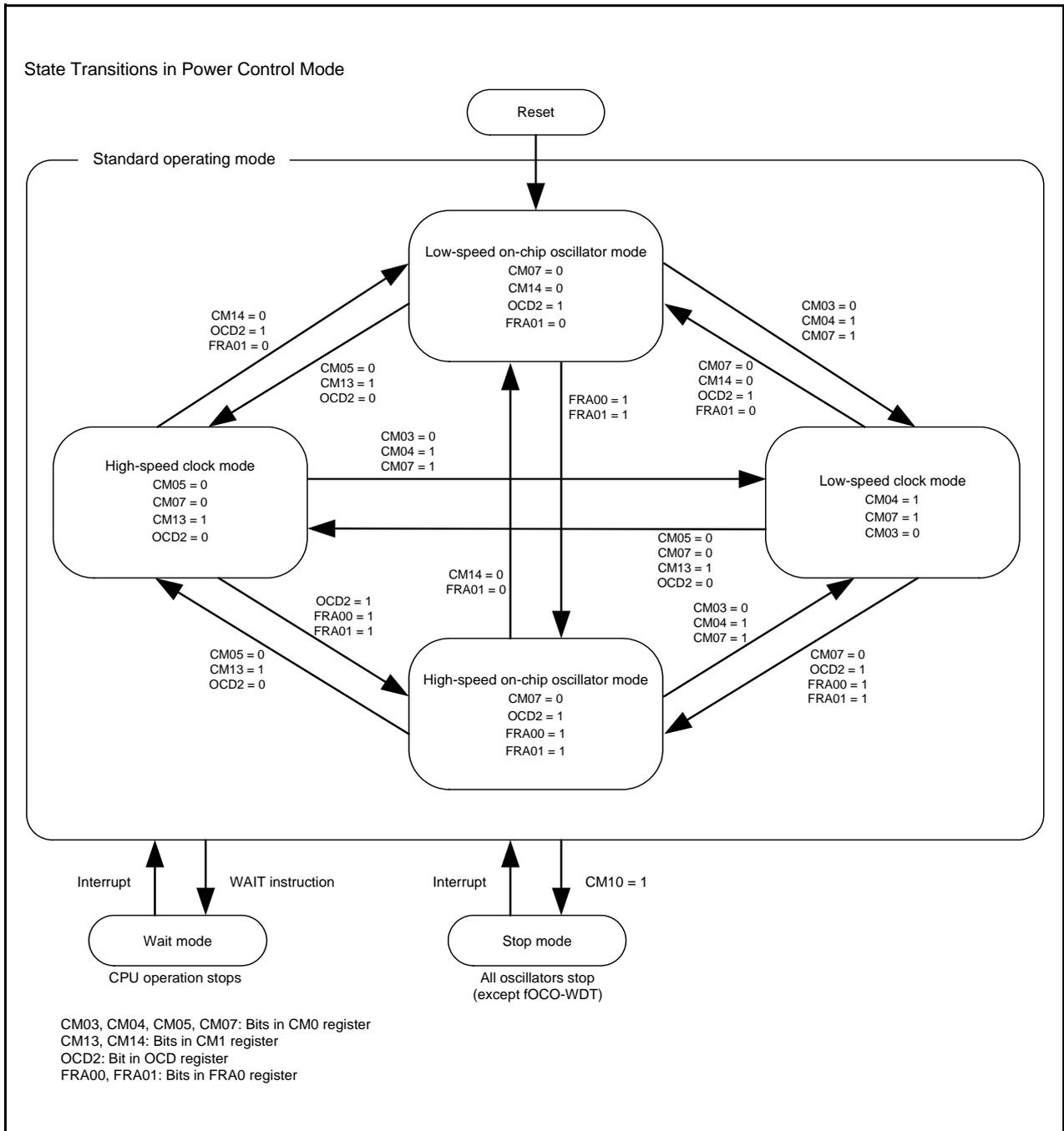
Figure 9.9 State Transitions in Power Control Mode
