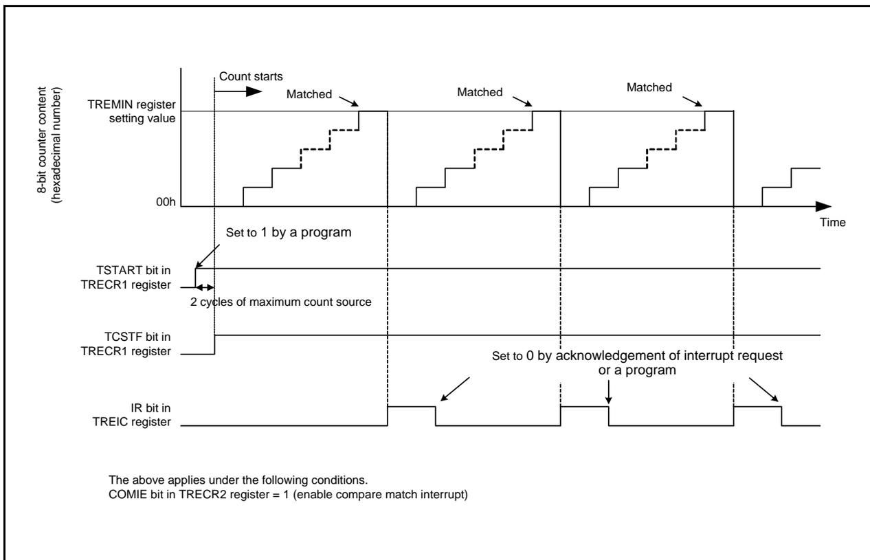
Figure 20.5 Operating Example in Output Compare Mode
