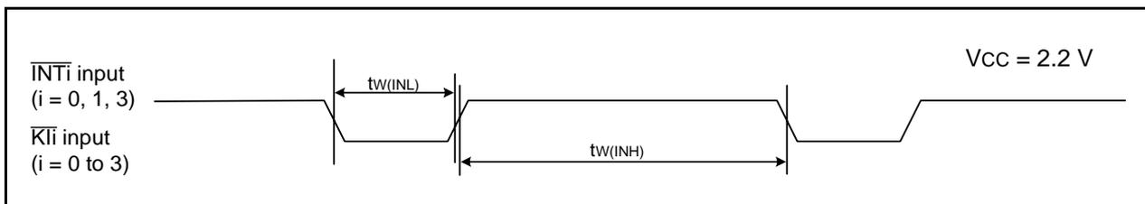
**Figure 31.19 Input Timing for External Interrupt  $\overline{INT}_i$  and Key Input Interrupt  $\overline{K}_i$  when  $V_{CC} = 2.2\text{ V}$**
