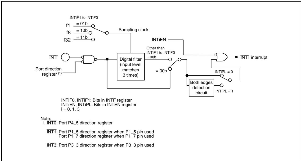
Figure 11.9 INTi Input Filter Configuration
