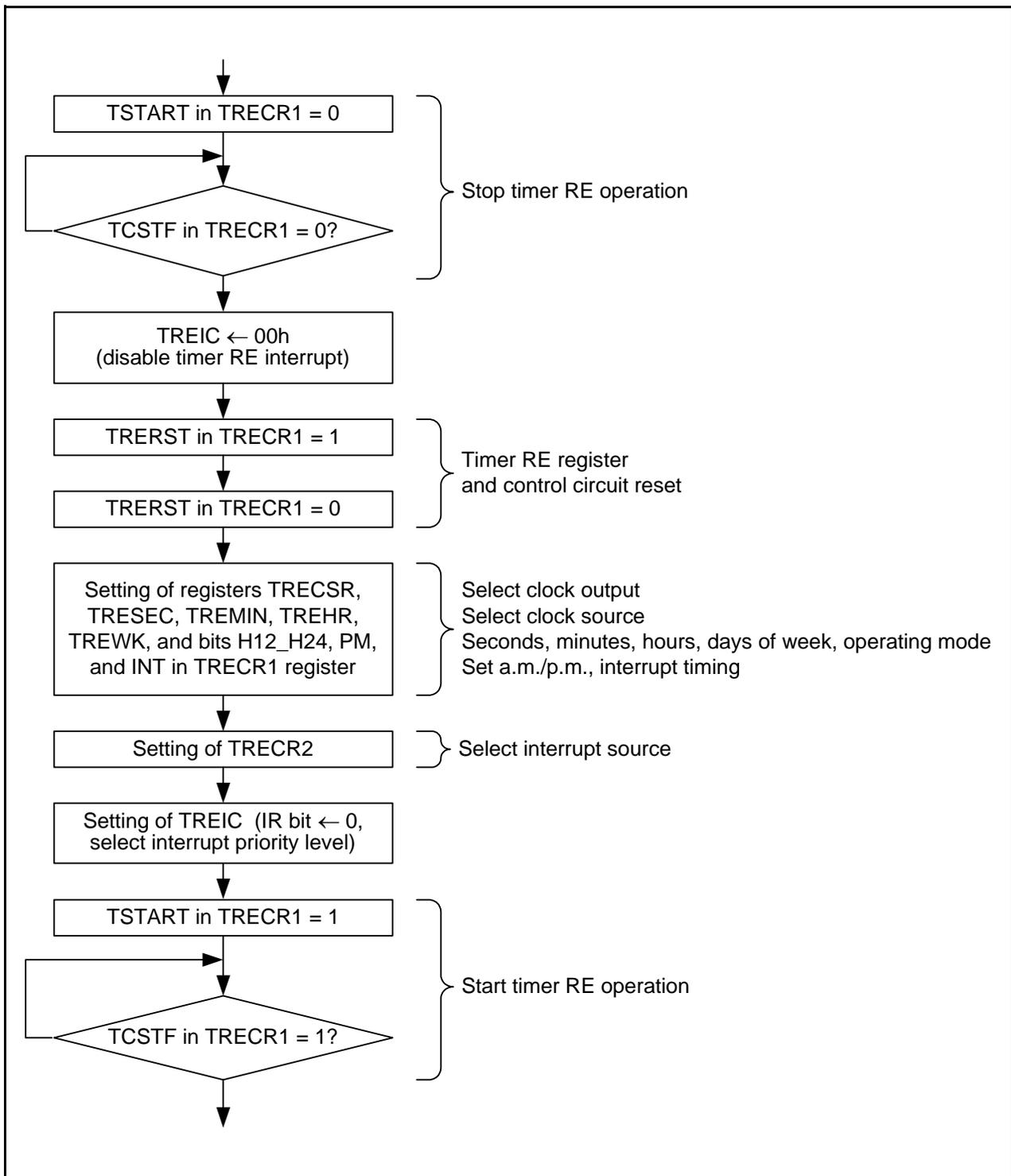
Figure 32.2 Setting Example in Real-Time Clock Mode
