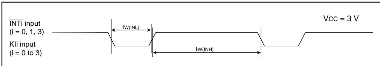
**Figure 31.15 Input Timing Diagram for External Interrupt  $\overline{INTi}$  and Key Input Interrupt  $\overline{Kli}$  when Vcc = 3 V**
