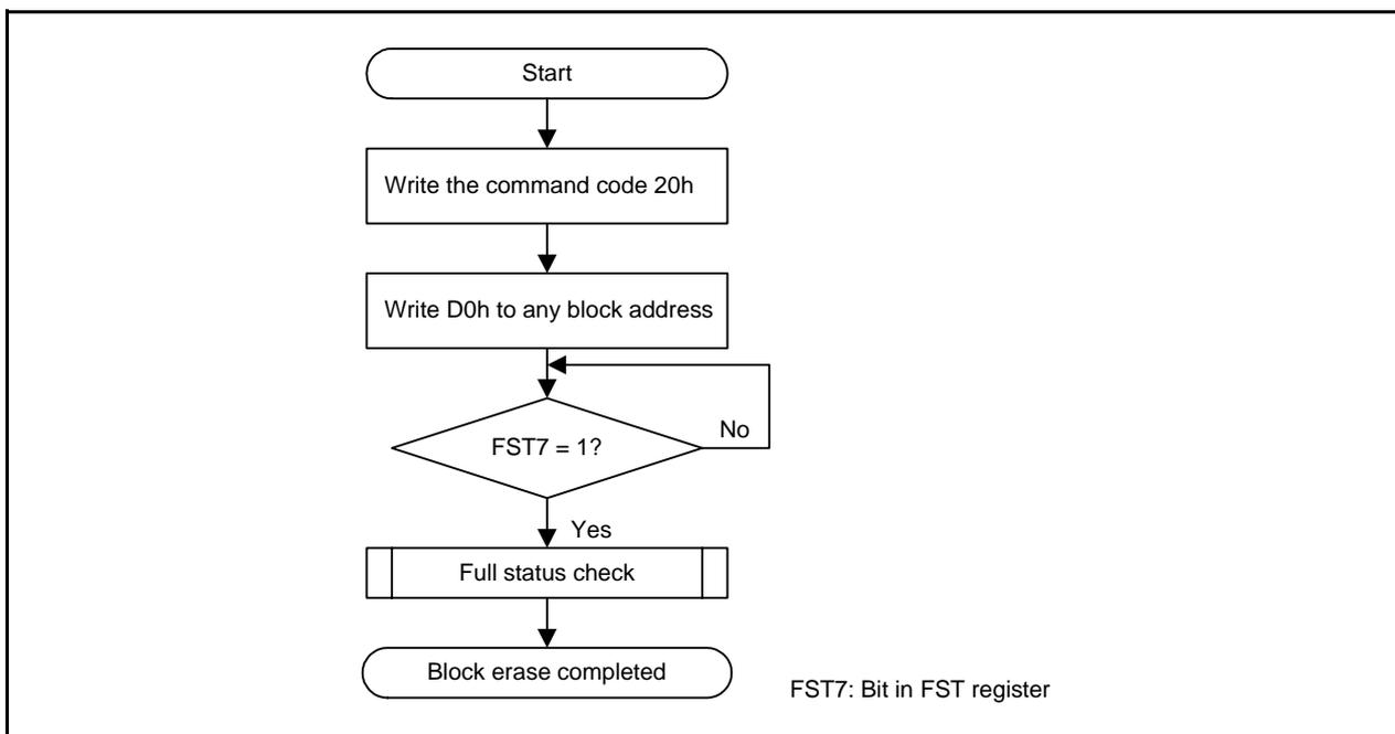
Figure 29.10 Block Erase Flowchart (Flash Ready Status Interrupt Disabled)
