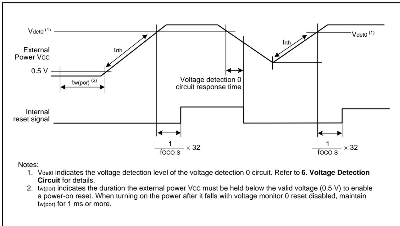
**Figure 31.3 Power-on Reset Circuit Electrical Characteristics**
