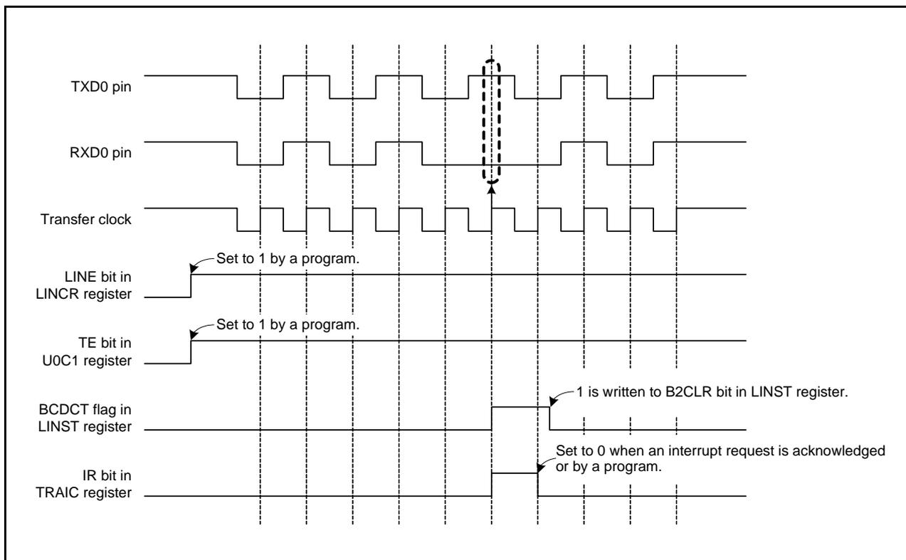
Figure 26.9 Operating Example When Bus Collision is Detected
