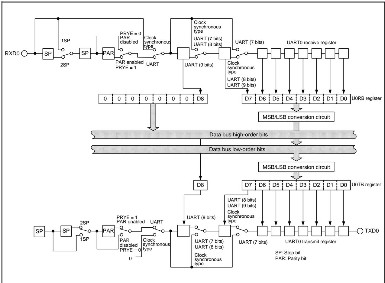
Figure 21.2 Block Diagram of UART0 Transmit/Receive Unit
