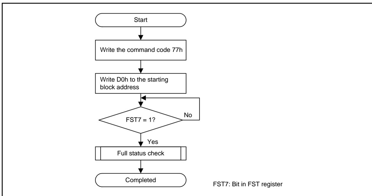
Figure 29.13 Lock Bit Program Flowchart
