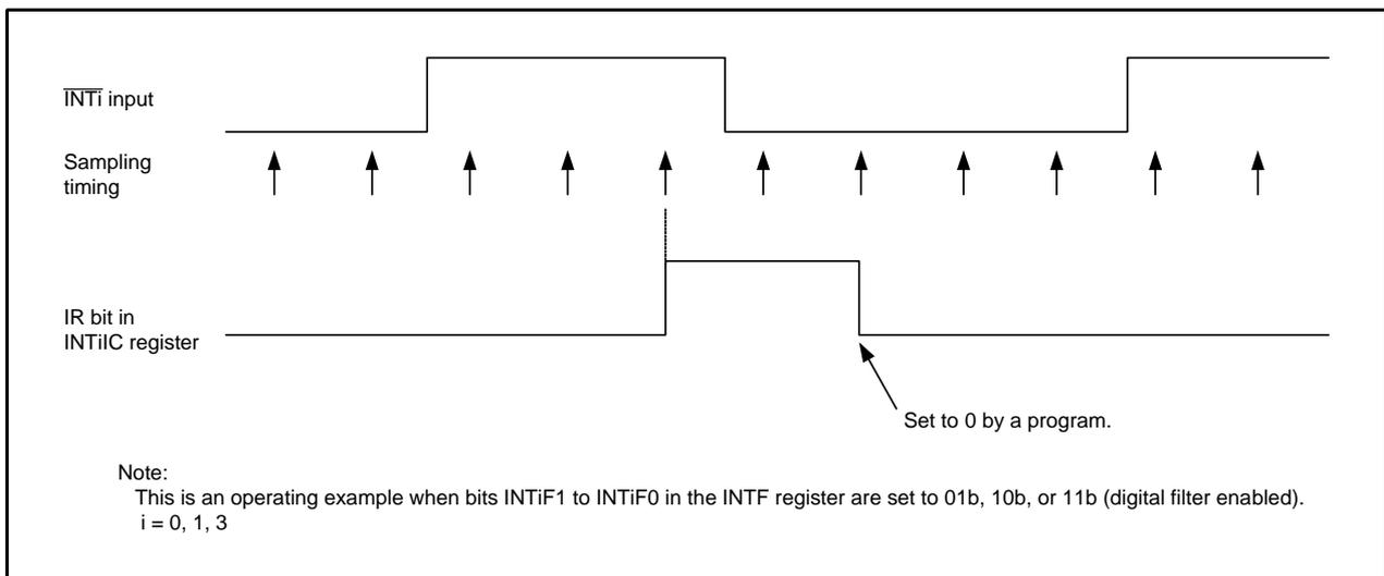
Figure 11.10 Operating Example of INTi Input Filter
