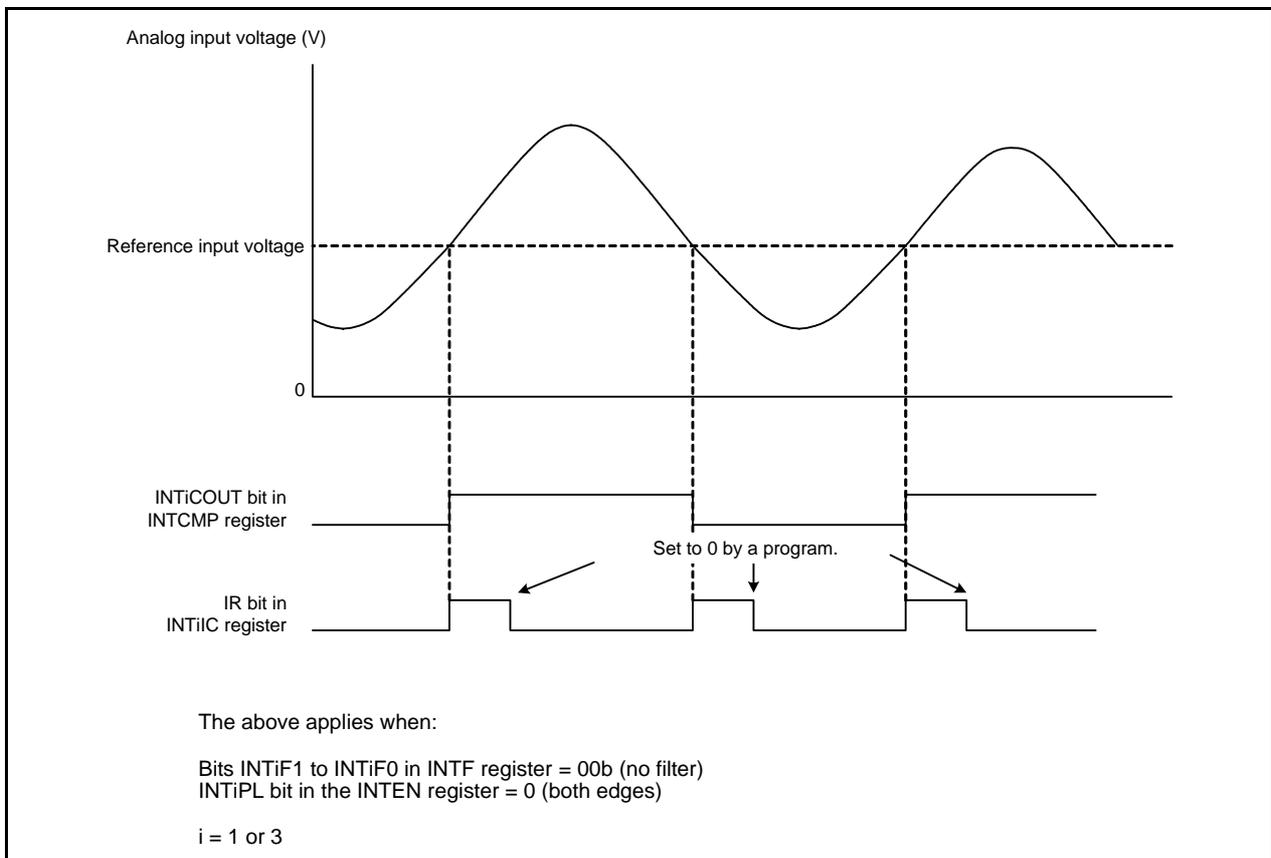
**Figure 28.2 Operating Example of Comparator Bi ( $i = 1$  or  $3$ )**
