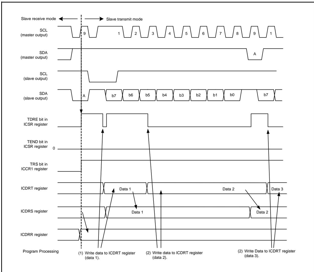
Figure 25.9 Operating Timing in Slave Transmit Mode (I<sup>2</sup>C bus Interface Mode) (1)
