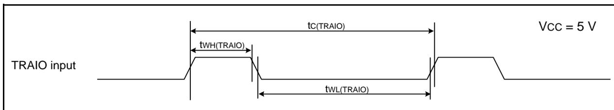
**Figure 31.9 TRAI0 Input Timing Diagram when  $V_{CC} = 5\text{ V}$**
