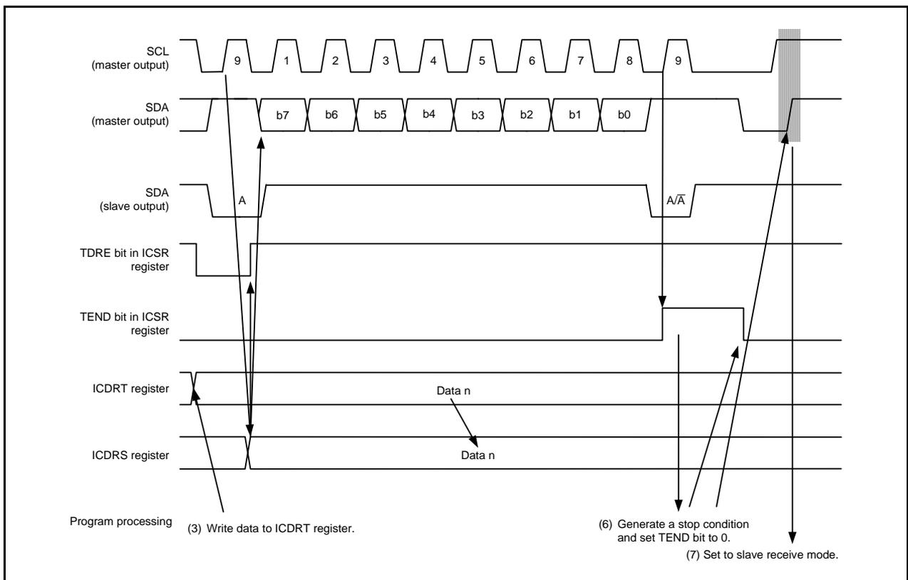
Figure 25.6 Operating Timing in Master Transmit Mode (I<sup>2</sup>C bus Interface Mode) (2)
