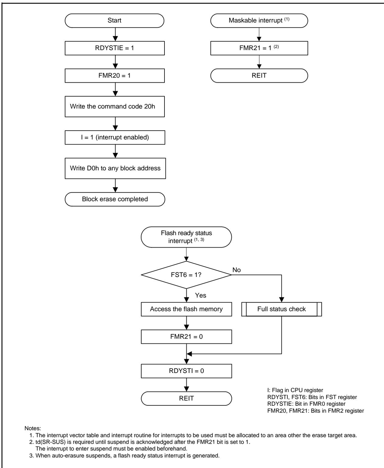
Figure 29.12 Block Erase Flowchart (Flash Ready Status Interrupt Enabled and Suspend Enabled)
