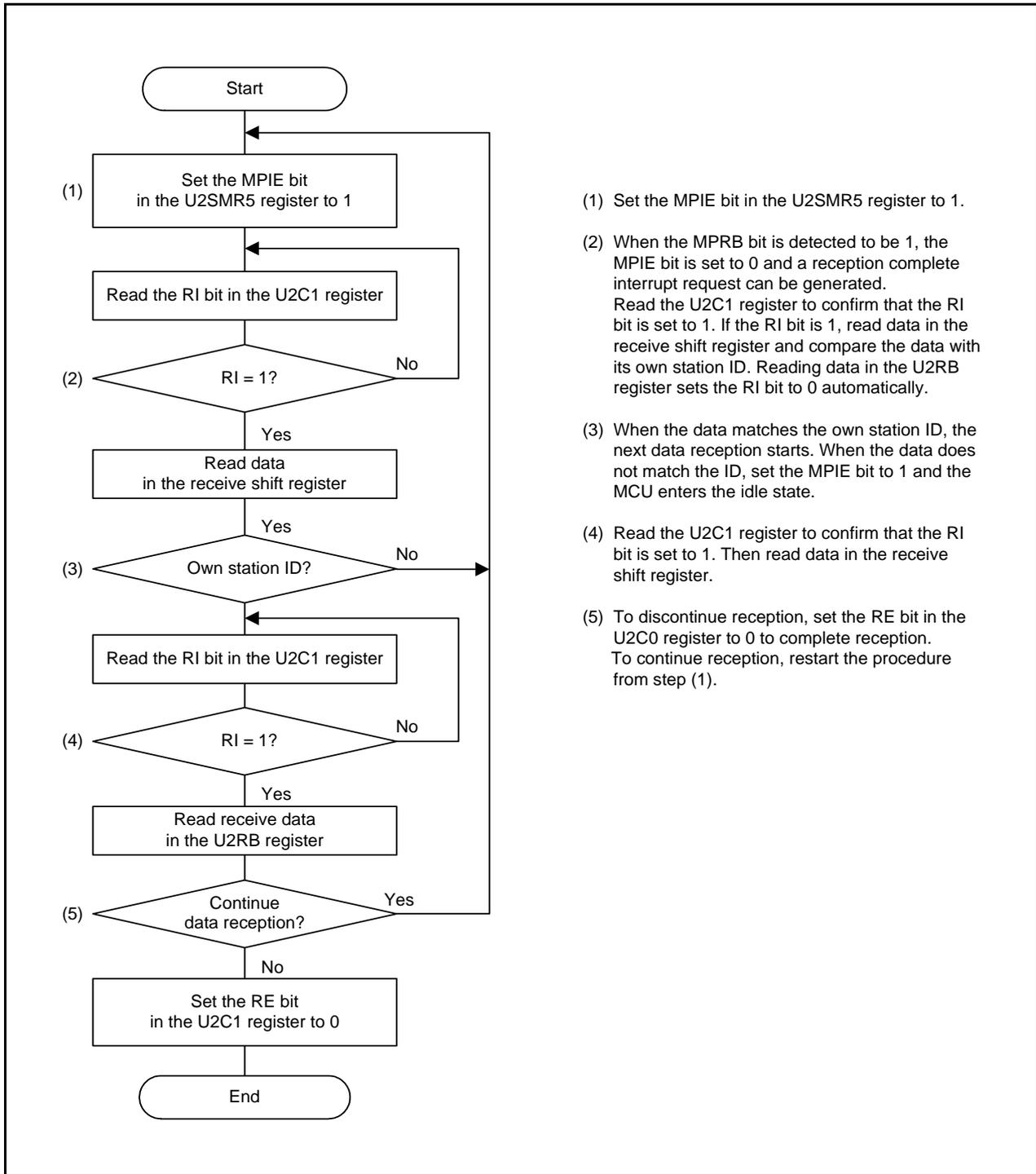
Figure 22.20 Sample Flowchart of Multiprocessor Data Reception
