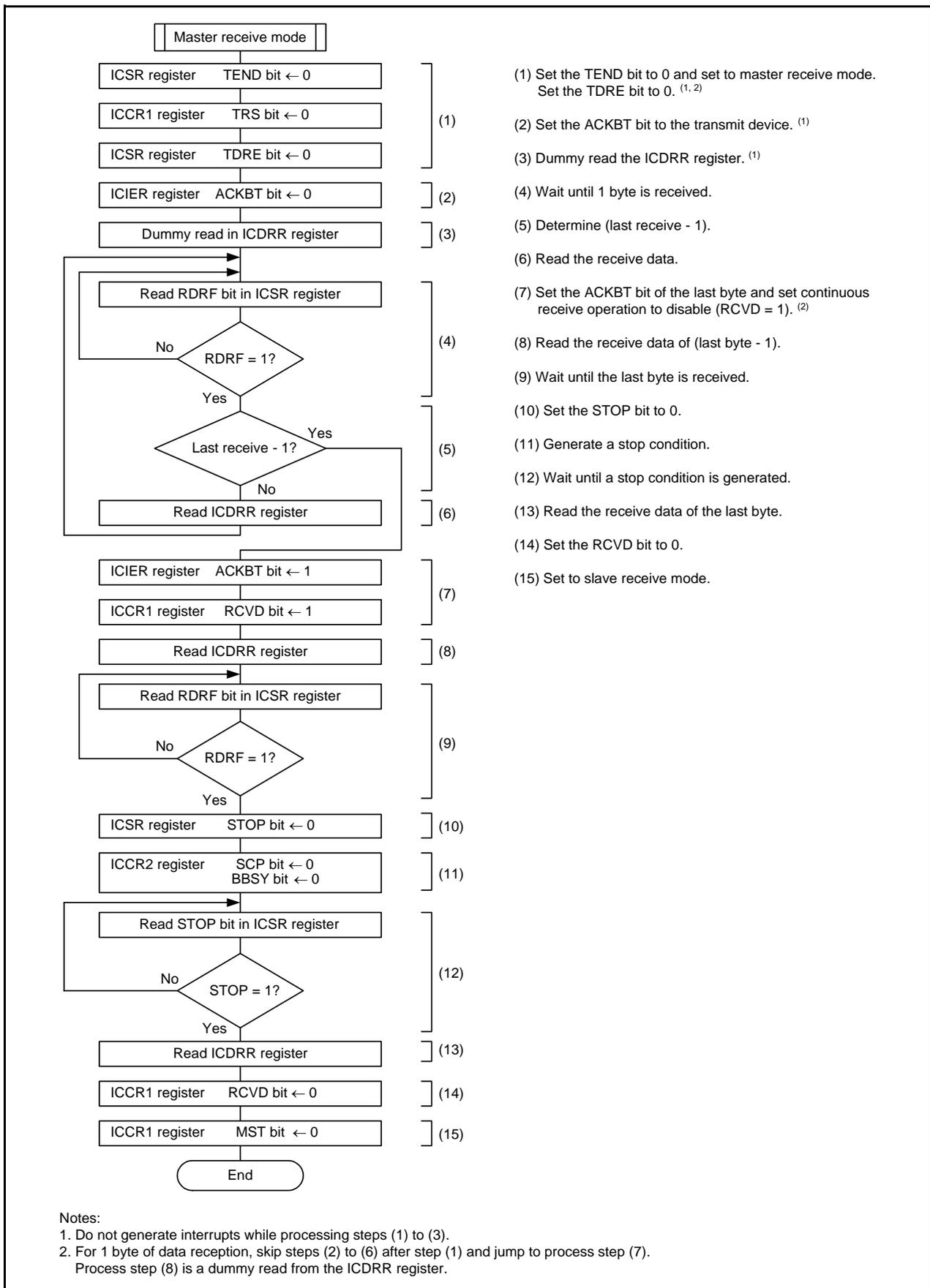
Figure 25.17 Register Setting Example in Master Receive Mode (I<sup>2</sup>C bus Interface Mode)
