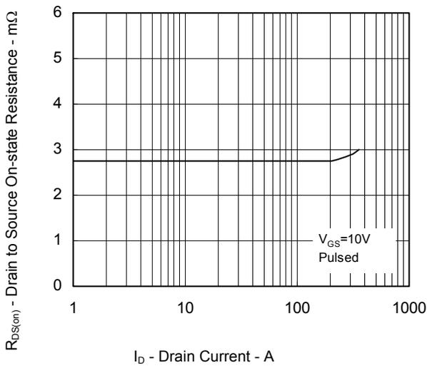
DRAIN TO SOURCE ON-STATE RESISTANCE vs.
