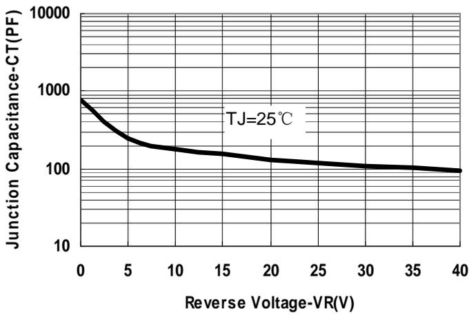
Fig.1-Typical Junction Capacitance
