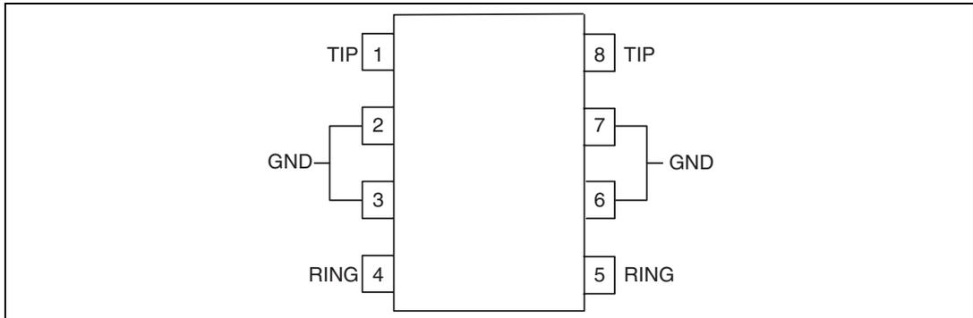
Connect pins 2, 3, 6 and 7 to ground to guarantee a good surge current capability for long duration disturbances.
