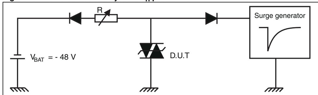
This is a go no-go test, which can confirm the holding current ( $I_H$ ) level.
