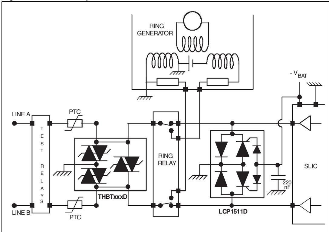
Figure 10. Protection for telephone set with ground key
