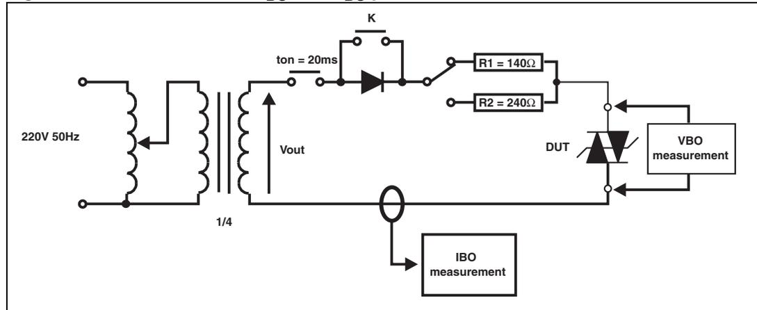
Pulse test duration ( $t_p = 20 \text{ ms}$ ):
