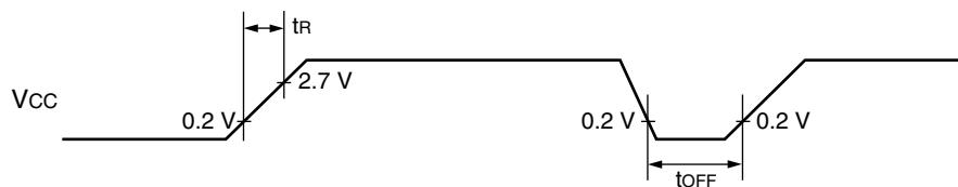
Sudden changes in the power supply voltage may cause a power-on reset.
