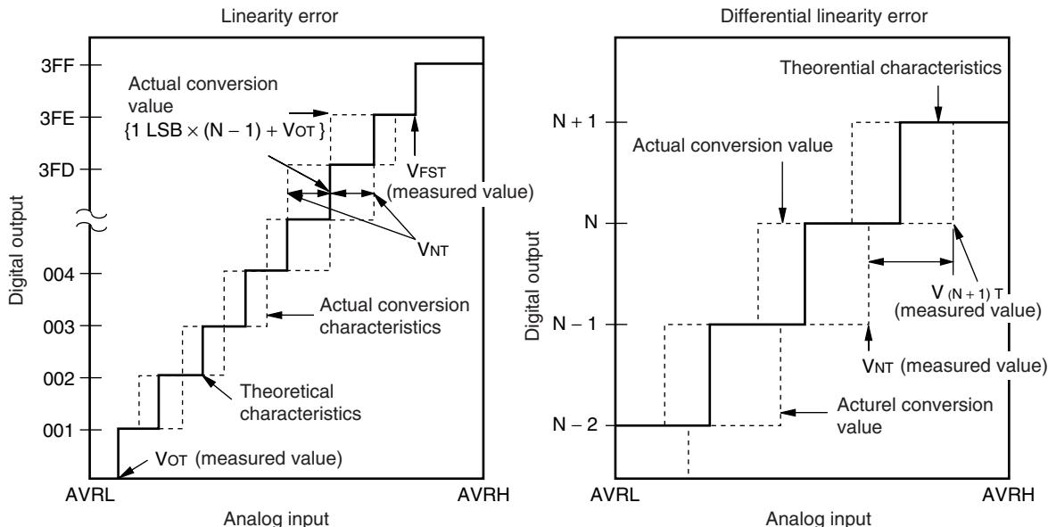
$$\text{Linearity error of digital output } N = \frac{V_{NT} - \{1 \text{ LSB} \times (N - 1) + V_{OT}\}}{1 \text{ LSB}} \text{ [LSB]}$$
