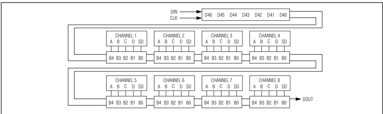
Figure 1. Data Flow of Serial Shift Register
