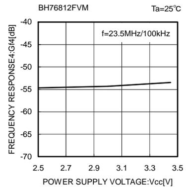
Fig. 29 Frequency response 4 vs. Supply voltage
