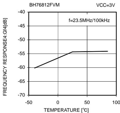
Fig. 30 Frequency response 4 vs. Temperature
