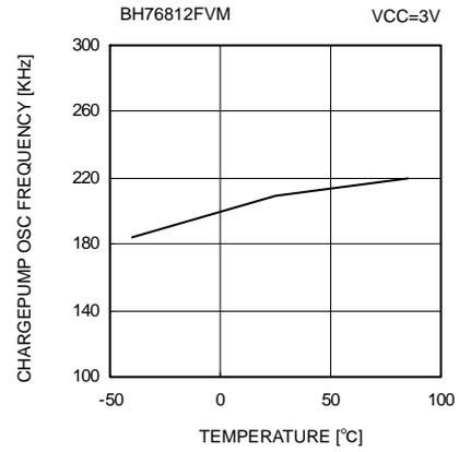
Fig. 35 Charge pump oscillation frequency vs. Temperature
