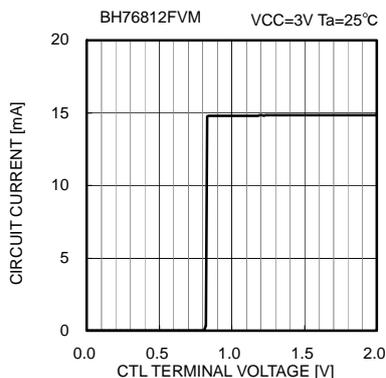
Fig. 48 Circuit current vs. CTL terminal voltage
