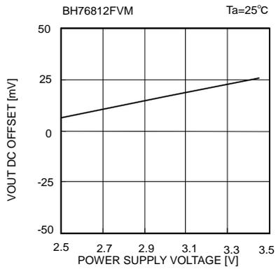
Fig. 20 Vout DC offset voltage vs. Supply voltage
