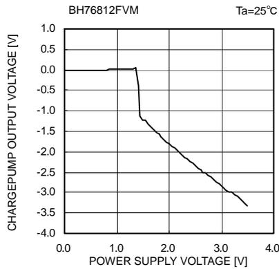
Fig. 36 Charge pump output voltage vs. Supply voltage
