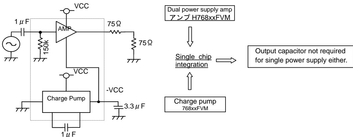
Fig. 6 BH768xxFVM Configuration Diagram
