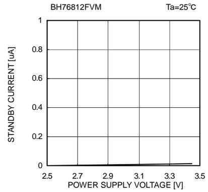
Fig. 17 Circuit Current (Standby) vs. Supply Voltage
