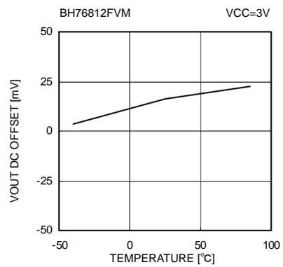
Fig. 21 Vout DC offset voltage vs. Temperature
