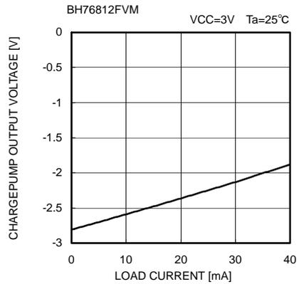
Fig. 37 Charge pump load regulation
