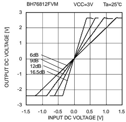
Fig. 33 Output DC voltage – Input DC voltage
