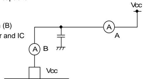
2) Decoupling capacitor + Resistance 10Ω
