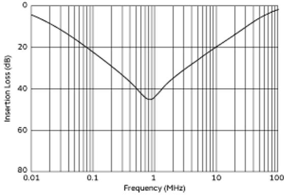
Common Mode Insertion Loss (Typ.)
