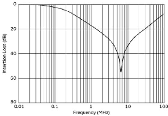
Differential Mode Insertion Loss (Typ.)
