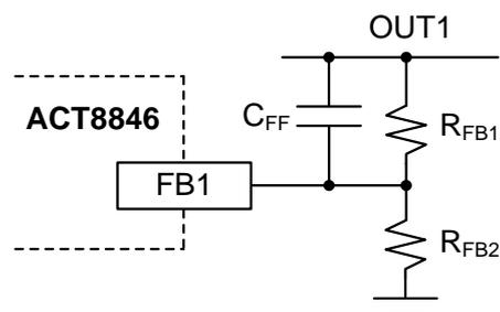
Figure 4 shows the feedback network necessary to set the output voltage for REG1 when using the adjustable output voltage option. Connect the FB1 pin to the output directly to regulate the output voltage at 1.2V. Select components as follows: Set  $R_{FB2} = 51k\Omega$ , then calculate  $R_{FB1}$  using the following equation:
