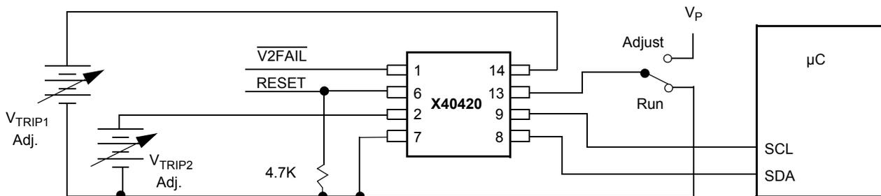
Figure 6.  $V_{TRIPX}$  Set/Reset Sequence (X = 1, 2)
