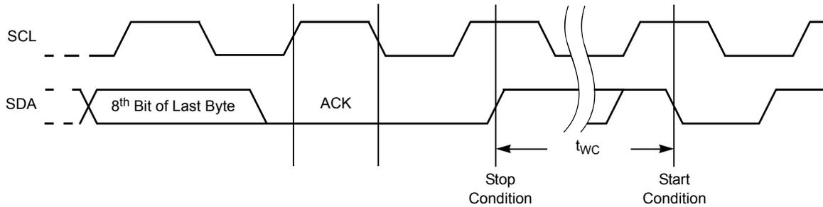
**Nonvolatile Write Cycle Timing**
