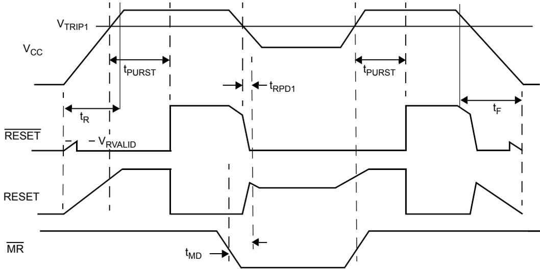
LOW VOLTAGE AND WATCHDOG TIMINGS PARAMETERS (@25°C, VCC = 5V)
