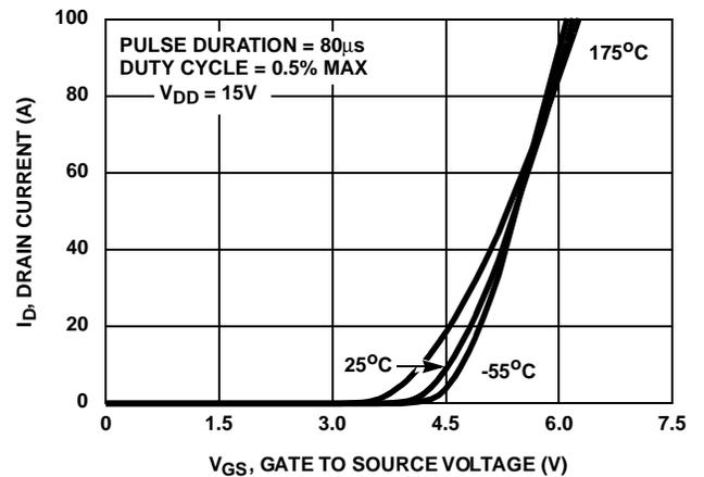
FIGURE 8. TRANSFER CHARACTERISTICS
