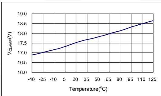
Figure 15. PWM Gate Output Clamping Voltage
