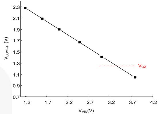
**Figure 37.  $V_{COMP-H}$  Voltage vs.  $V_{IN}$  Voltage Characteristic Curve**
