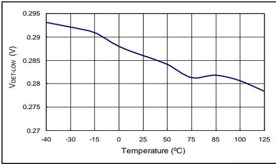
Figure 21. Lower Clamp Voltage of DET Pin
