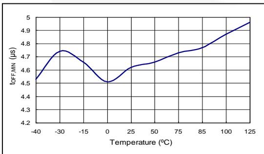
Figure 19. PWM Minimum Off-Time for V<sub>FB</sub> > V<sub>NI</sub>
