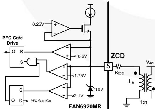
**Figure 30. Internal Block of the Zero-Current Detection**
