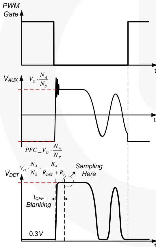
**Figure 46. Operation Waveform of Output Over-Voltage Detection**
