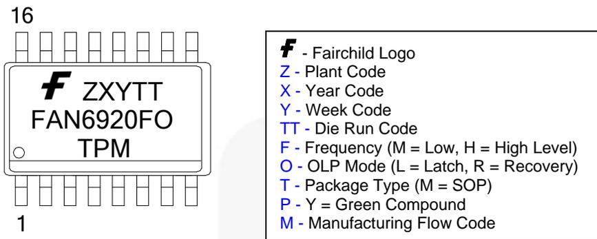
Figure 3. Marking Diagram
