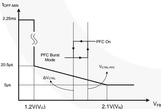
**Figure 40.  $V_{FB}$  Voltage vs.  $t_{OFF-MIN}$  Time Characteristic Curve**
