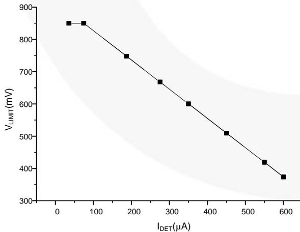
Figure 44.  $I_{DET}$  Current vs.  $V_{LIMIT}$  Voltage Characteristic Curve
