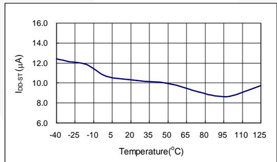
Figure 9. Startup Current
