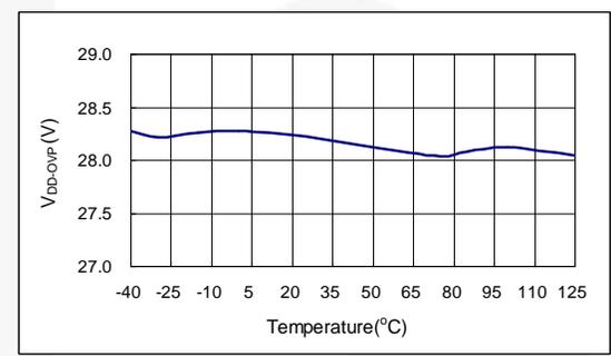
Figure 8. V<sub>DD</sub> Over-Voltage Protection Threshold
