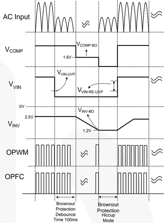
Figure 34. Operation Waveforms of Brownout / In Protection
