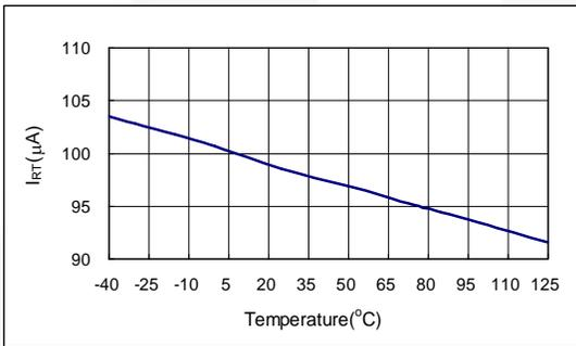
Figure 23. Internal Source Current of RT Pin
