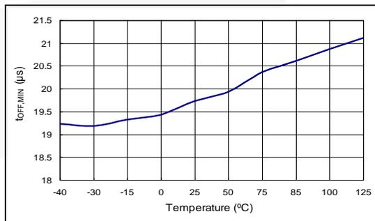
Figure 20. PWM Minimum Off-Time for V<sub>FB</sub> = V<sub>G</sub>
