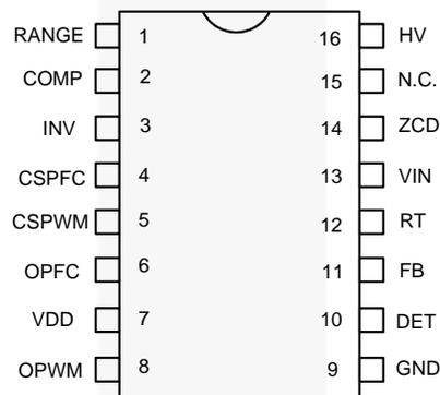
Figure 4. Pin Configuration
