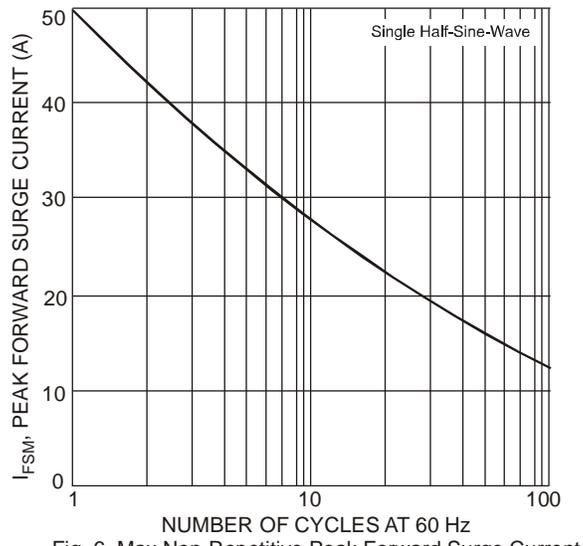
Fig. 6 Max Non-Repetitive Peak Forward Surge Current
