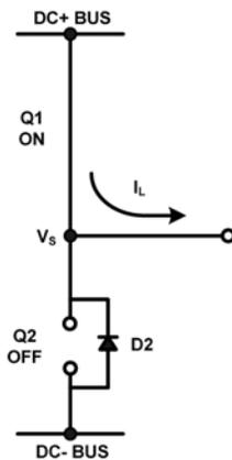
**Figure 6: Q1 conducting**
