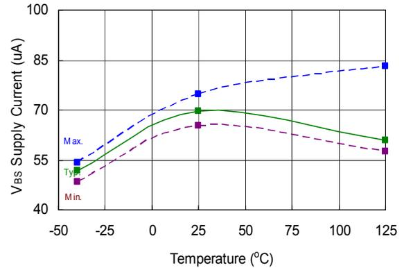
**Figure 21. V<sub>BS</sub> Supply Current vs. Temperature**
