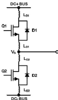
Figure 10: Parasitic Elements
