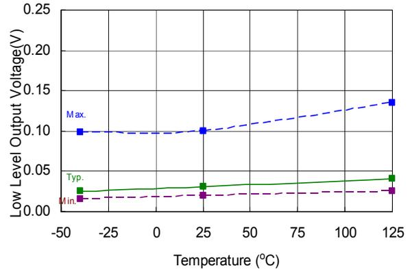
**Figure 19. Low Level Output Voltage vs. Temperature**
