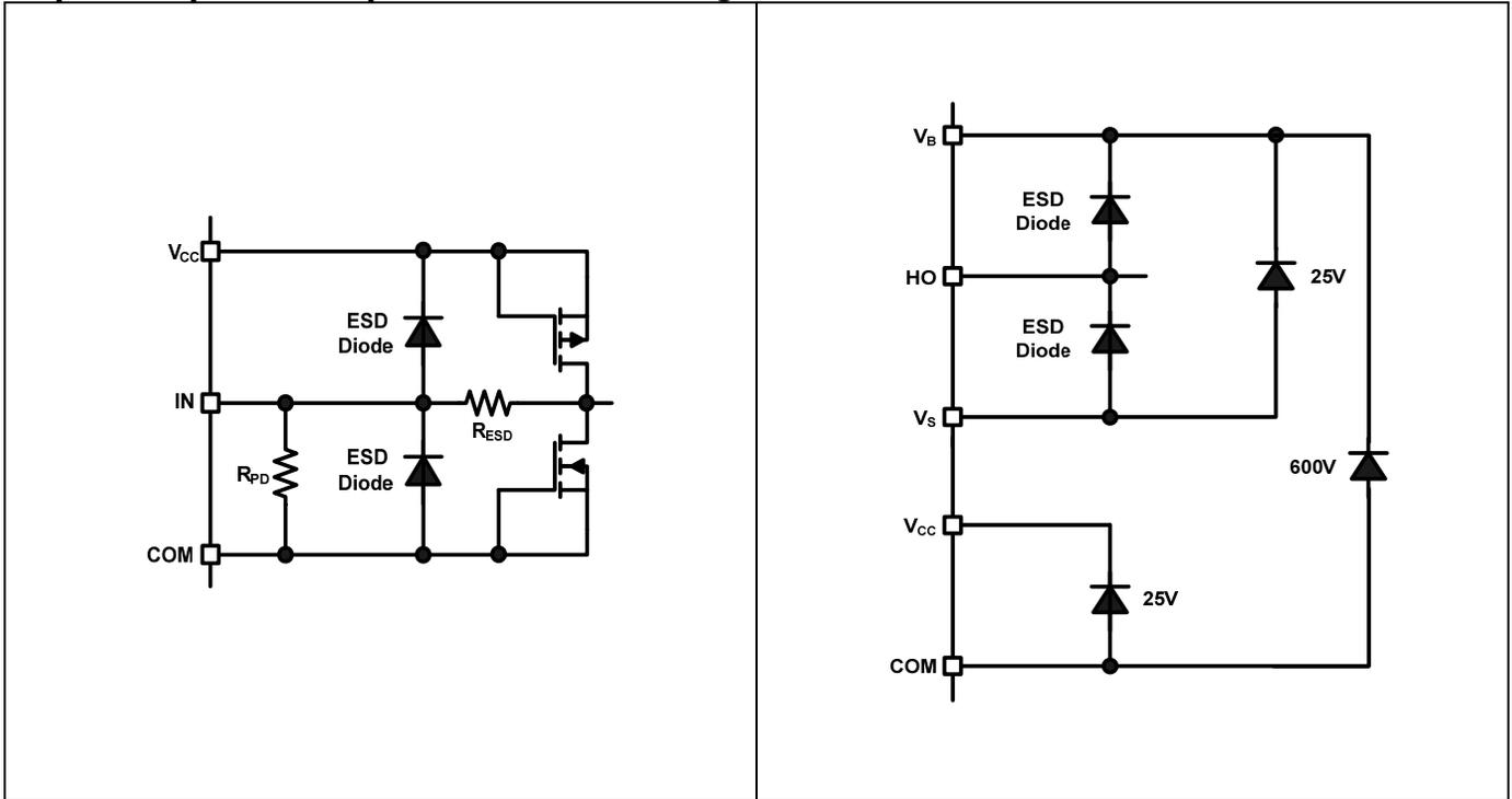
**Input/Output Pin Equivalent Circuit Diagrams: AUIRS2118S**
