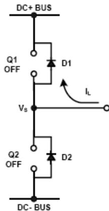
Figure 8: D1 conducting
