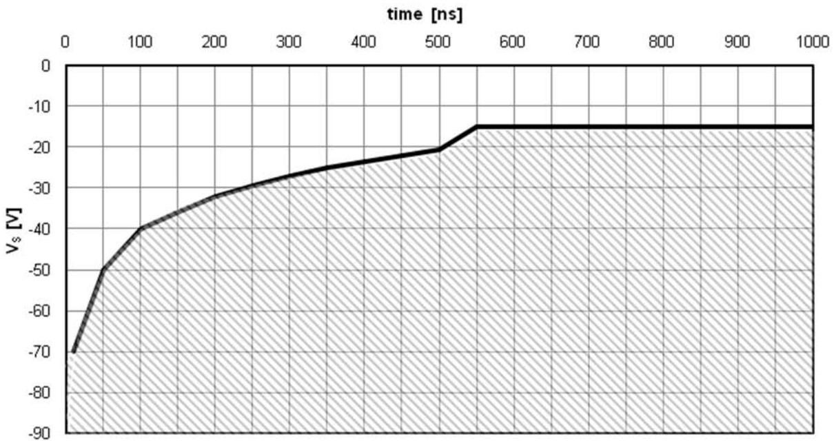
**Figure 13: Negative  $V_s$  transient SOA for AUIRS2117(8)S @  $V_{BS}=15V$**
