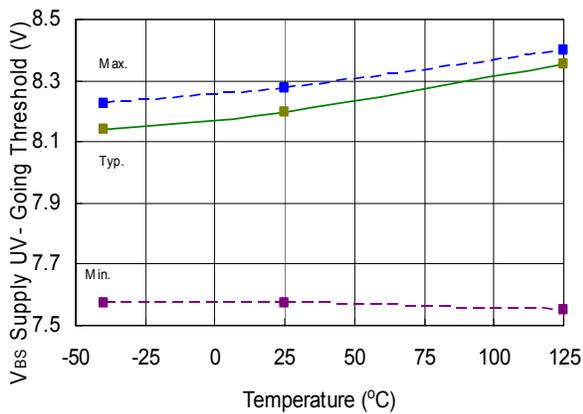
**Figure 28. V<sub>BS</sub> Undervoltage Threshold (-) vs. Temperature**
