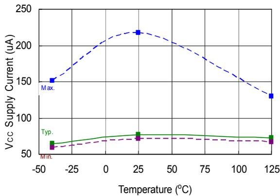
**Figure 22. V<sub>CC</sub> Supply Current vs. Temperature**
