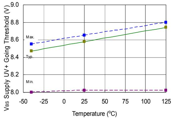
**Figure 27. V<sub>BS</sub> Undervoltage Threshold (+) vs. Temperature**
