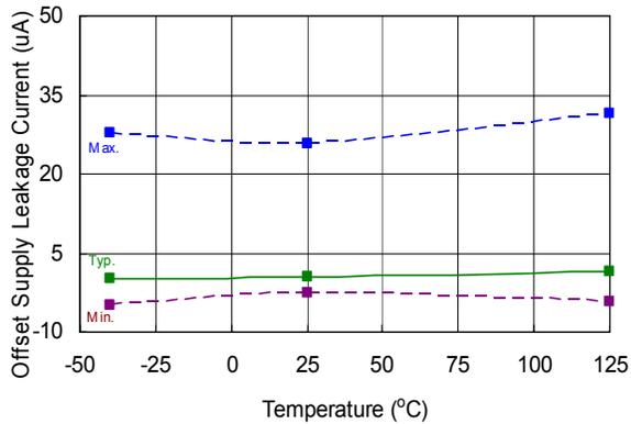
**Figure 20. Offset Supply Leakage Current vs. Temperature**
