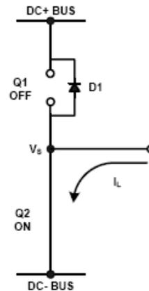
Figure 9: Q2 conducting
