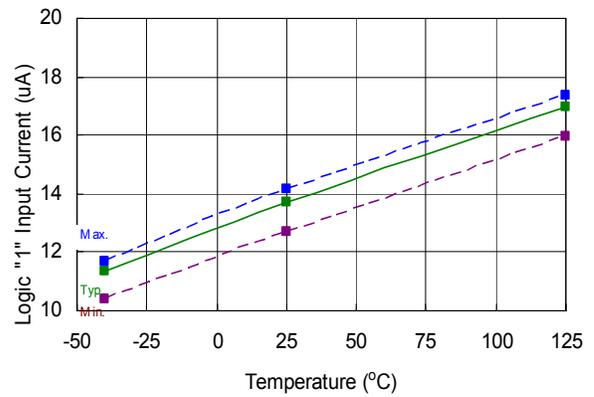
**Figure 23. Logic "1" Input Current vs. Temperature**
