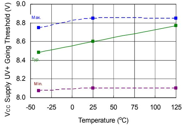
**Figure 25. V<sub>CC</sub> Undervoltage Threshold (+) vs. Temperature**
