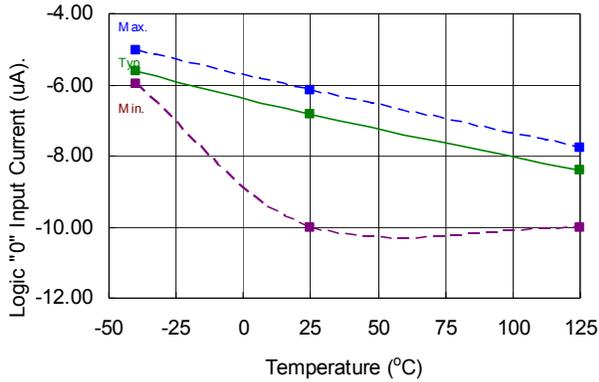
**Figure 24. Logic "0" (2118 "1") Input Current vs. Temperature**
