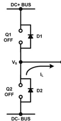
**Figure 7: D2 conducting**
