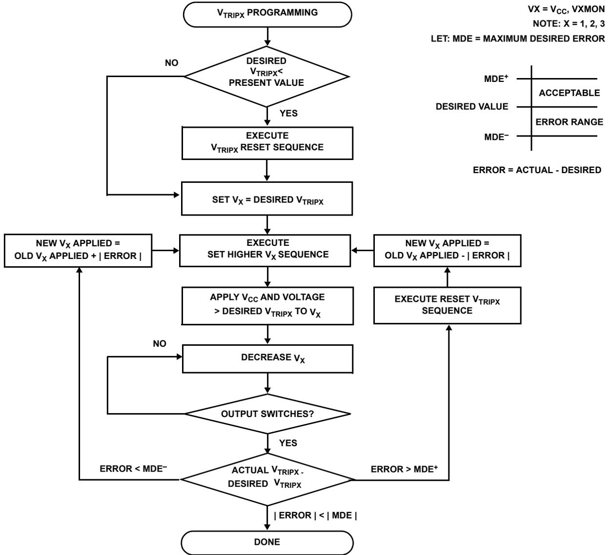
FIGURE 6.  $V_{TRIPX}$  SET/RESET SEQUENCE (X = 1, 2, 3)
