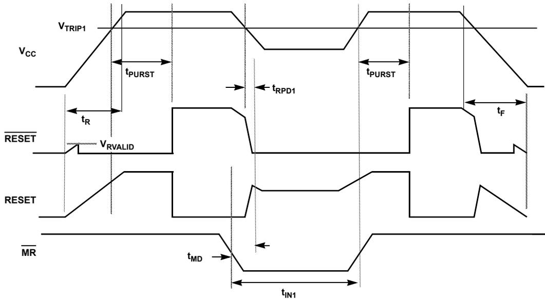
**Low Voltage and Watchdog Timings Parameters (@ +25°C,  $V_{CC} = 5V$ )**
