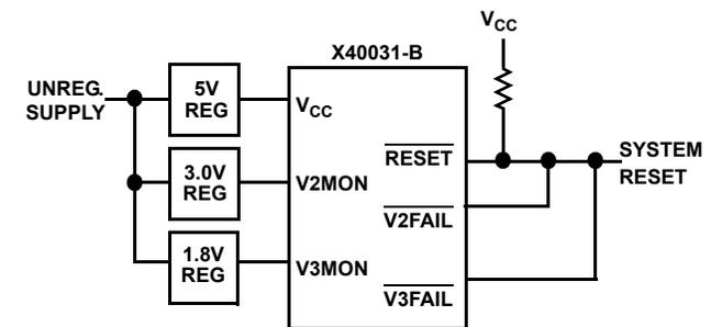
NOTICE: NO EXTERNAL COMPONENTS REQUIRED TO MONITOR THREE VOLTAGES.
