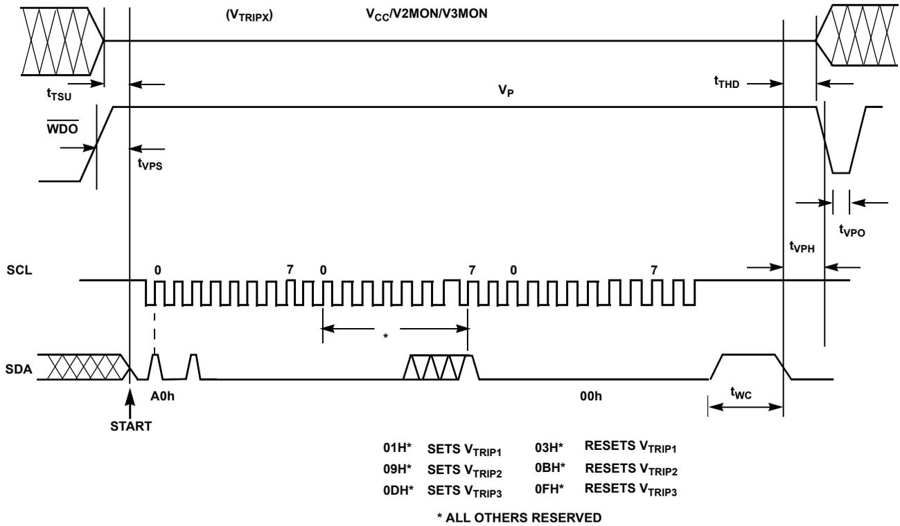
**V<sub>TRIP1</sub>, V<sub>TRIP2</sub>, V<sub>TRIP3</sub> Programming Specifications**      V<sub>CC</sub> = 2.0V to 5.5V; Temperature = +25°C
