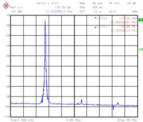
**FIGURE 2. EDGE AT 11MHz, 78MSPS CLOCK**
