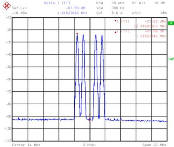
**FIGURE 5. FOUR EDGE CARRIERS AT 12.4–15.6MHz,**
