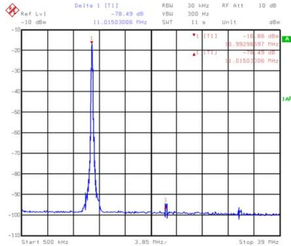
**FIGURE 4. GSM AT 11MHz, 78MSPS CLOCK**
