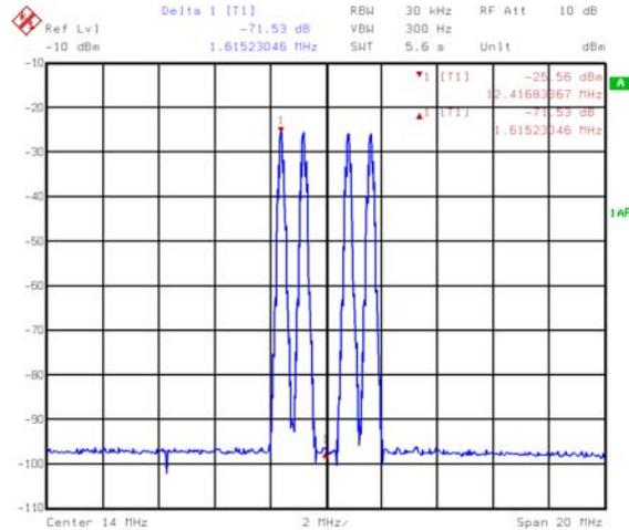
**FIGURE 6. FOUR GSM CARRIERS AT 12.4–15.6MHz,**
