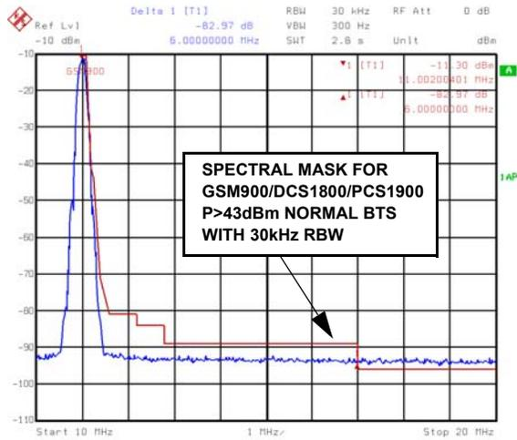
**FIGURE 1. EDGE AT 11MHz, 78MSPS CLOCK**
