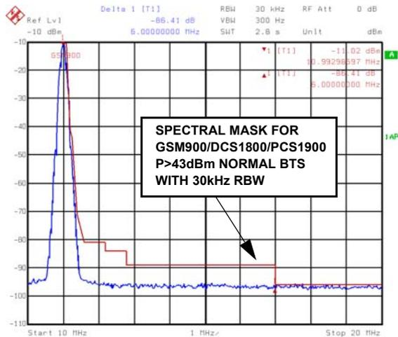
**FIGURE 3. GSM AT 11MHz, 78MSPS CLOCK**
