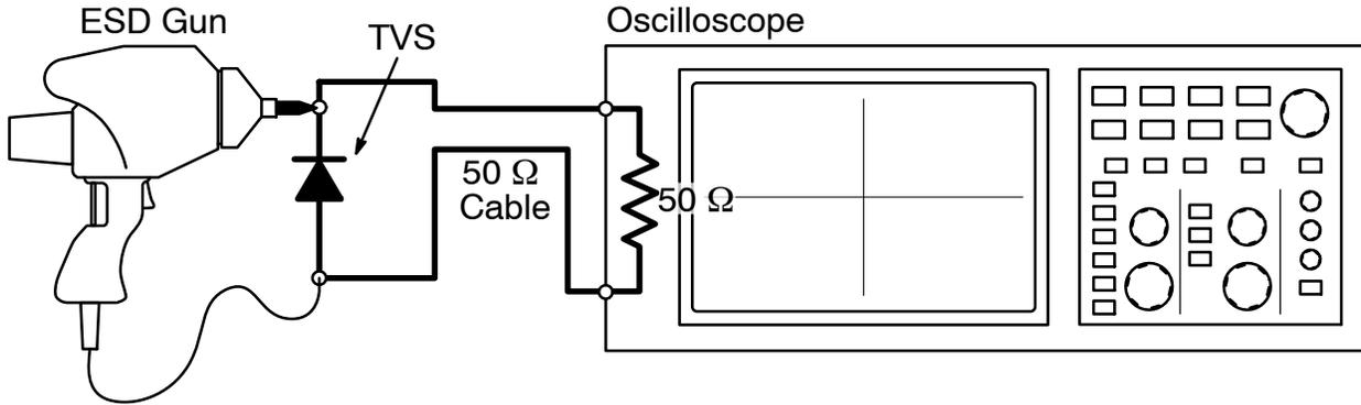
Figure 14. Diagram of ESD Clamping Voltage Test Setup
