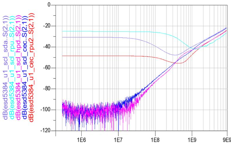
Figure 2. Crosstalk Measurements
