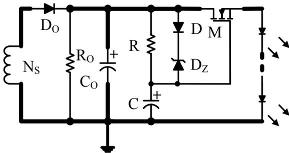
Figure14: Ripple Suppressor
