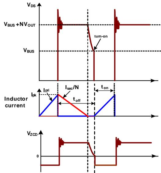
Figure 2: Boundary-Conduction Mode
