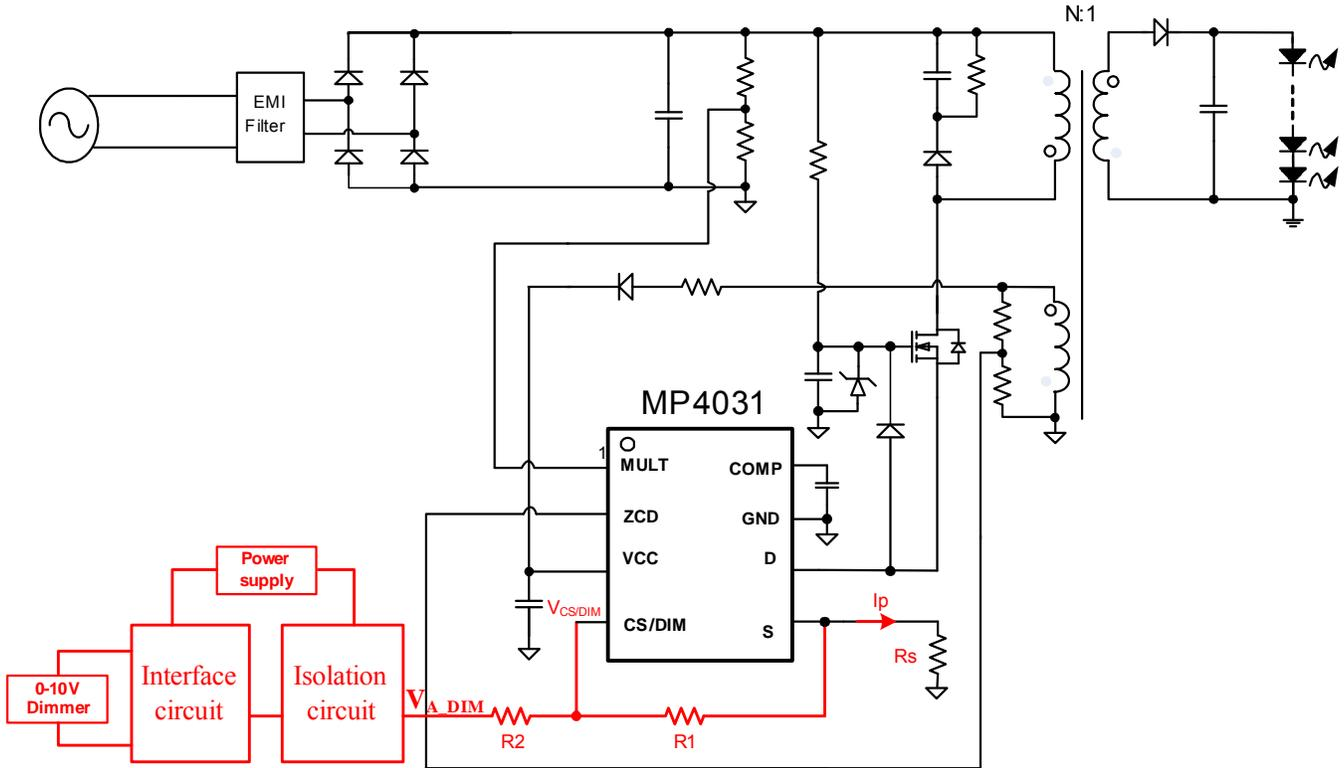
**Figure 13: Typical Application Circuit for Analog Dimming**
