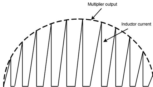
**Figure 4: Power-Factor Correction**
