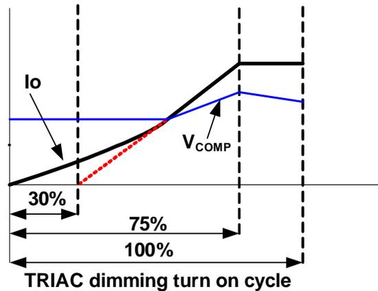
**Figure 12: Dimming Curve**
