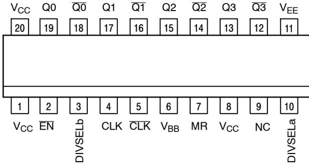
NOTE: All V<sub>CC</sub> pins are tied together on the die.
