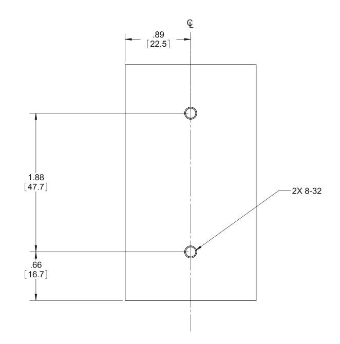
Tolerances: ± 0.02 in / 0.5 mm. All dimensions are in: inches [millimeters]
