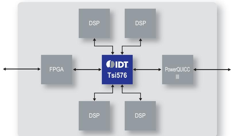
In video infrastructure cards, equipment vendors must maximize the number of DSPs per card to manage compression and decompression algorithms. These DSPs are controlled by a local processor and all these components are linked together by a low power, small form factor, low latency, multicast enabled Tsi576.
