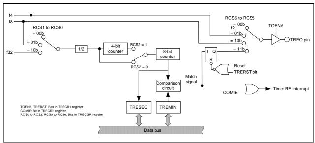
Figure 14.114 Block Diagram of Output Compare Mode
