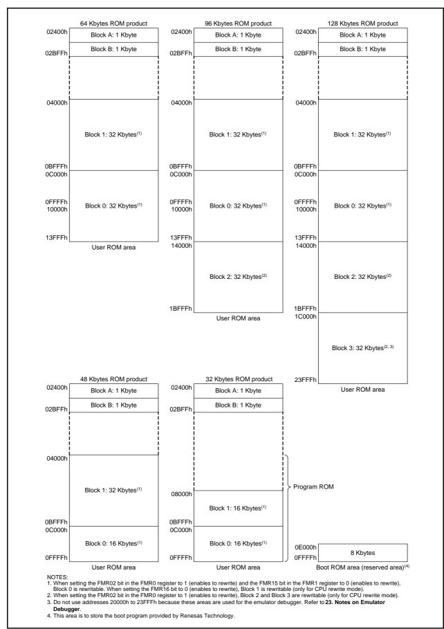
Figure 19.2 Flash Memory Block Diagram for R8C/21 Group
