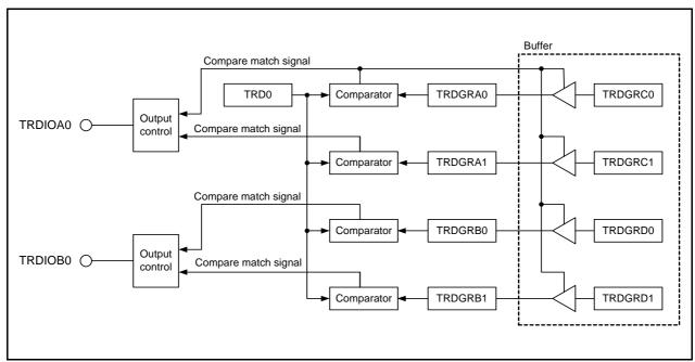
Figure 14.98 Block Diagram of PWM3 Mode
