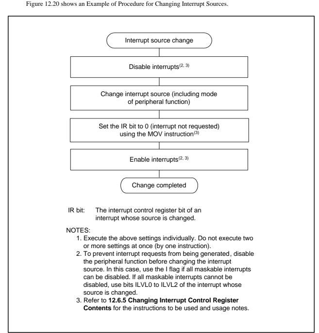
**Figure 12.20 Example of Procedure for Changing Interrupt Sources**
