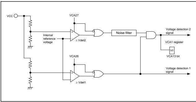
**Block Diagram of Voltage Detection Circuit** Figure 6.1
