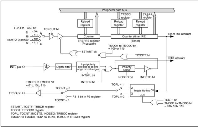
Figure 14.13 Block Diagram of Timer RB
