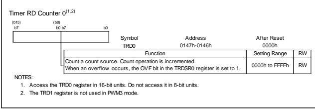
Figure 14.106 TRD0 Register in PWM3 Mode
