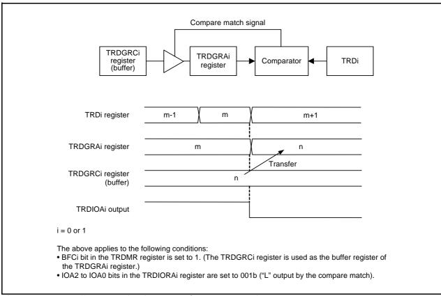
Figure 14.30 Buffer Operation in Output Compare Function
