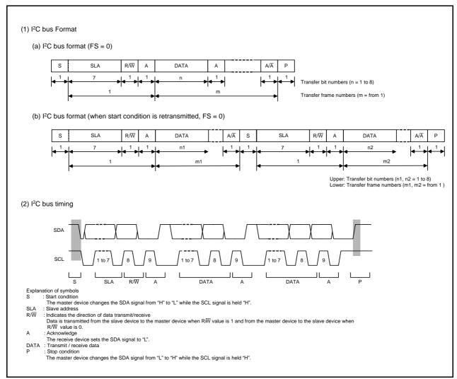
Figure 16.32 I<sup>2</sup>C Bus Format and Bus Timing
