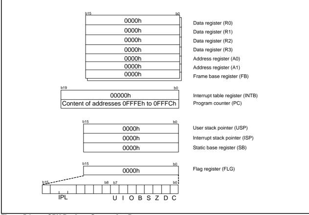
Figure 5.2 CPU Register Status after Reset
