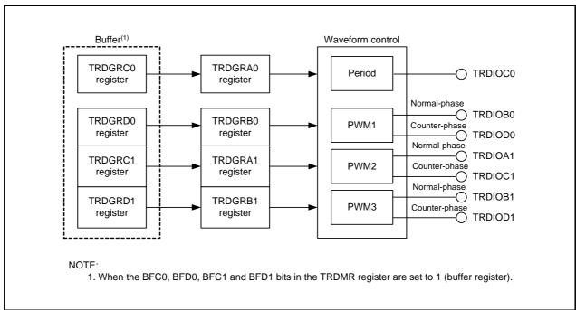
Figure 14.76 Block Diagram of Reset Synchronous PWM Mode
