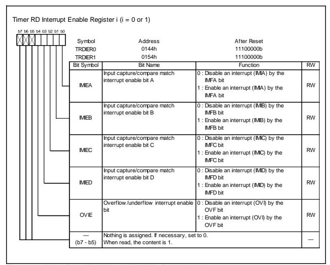
Figure 14.105 Registers TRDIER0 and TRDIER1 in PWM3 Mode
