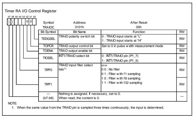
Figure 14.9 TRAIOC Register in Pulse Width Measurement Mode
