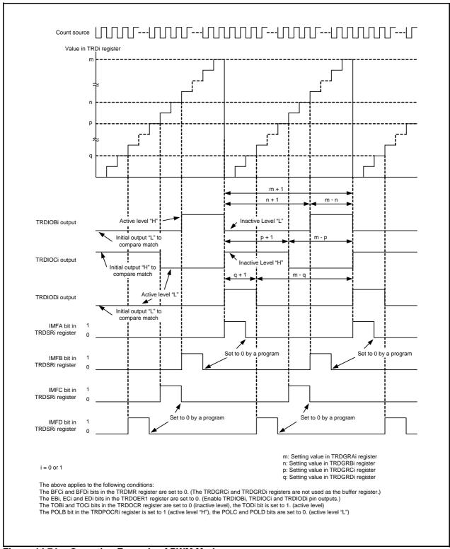
**Figure 14.74 Operating Example of PWM Mode**
