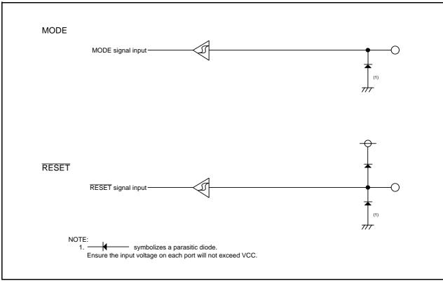
Figure 7.8 Configuration of I/O Pins
