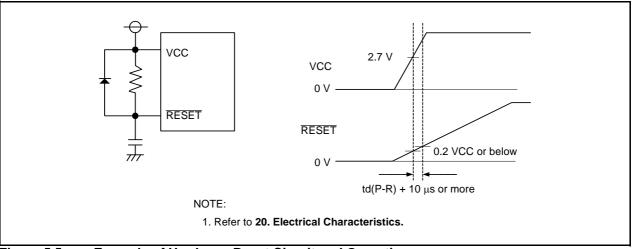
Figure 5.5 **Example of Hardware Reset Circuit and Operation**
