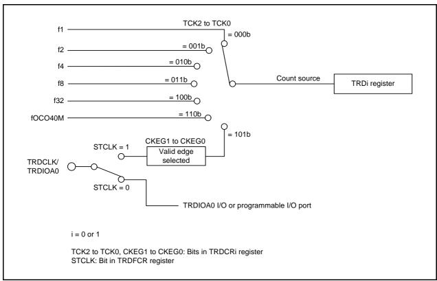
Figure 14.28 Block Diagram of Count Source
