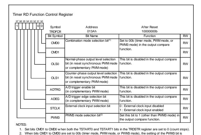
Figure 14.50 TRDFCR Register in Output Compare Function
