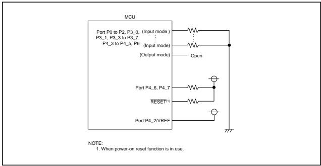
Figure 7.13 Unassigned Pin Handling
