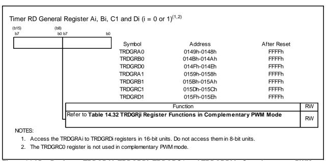
**Figure 14.95** Registers TRDGRAi, TRDGRBi, TRDGRC1 and TRDGRDi in Complementary PWM Mode
