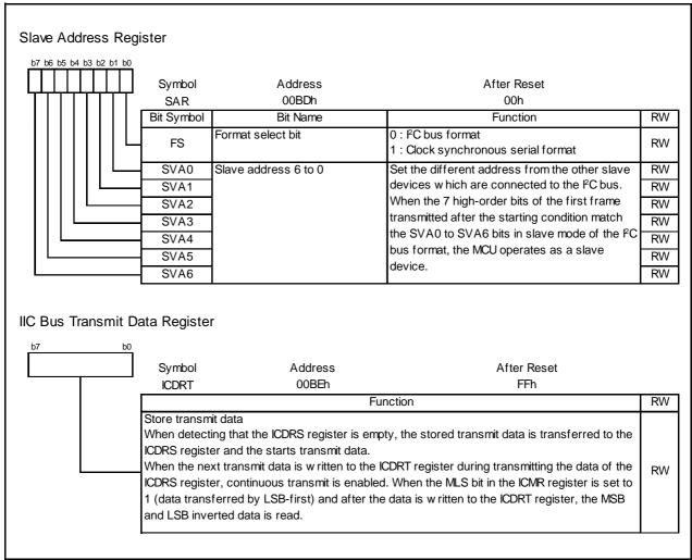
**Figure 16.29** Registers SAR and ICDRT
