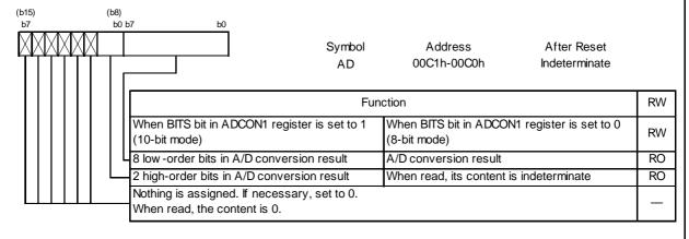
Figure 18.3 Registers ADCON1, ADCON2, and AD
