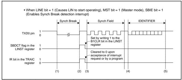
Figure 17.4 Typical Operation when Sending a Header Field
