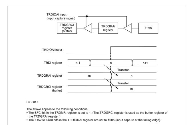
Figure 14.29 Buffer Operation in Input Capture Function
