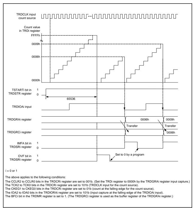
**Figure 14.45 Operating Example of Input Capture Function**
