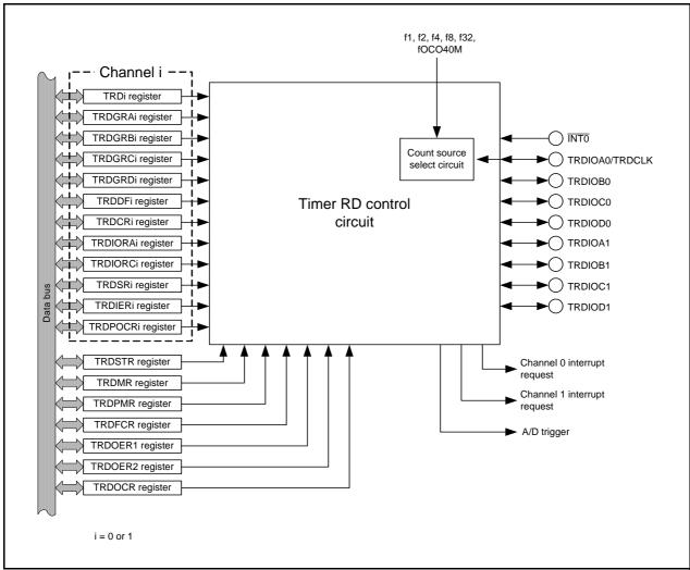
Figure 14.27 Block Diagram of Timer RD
