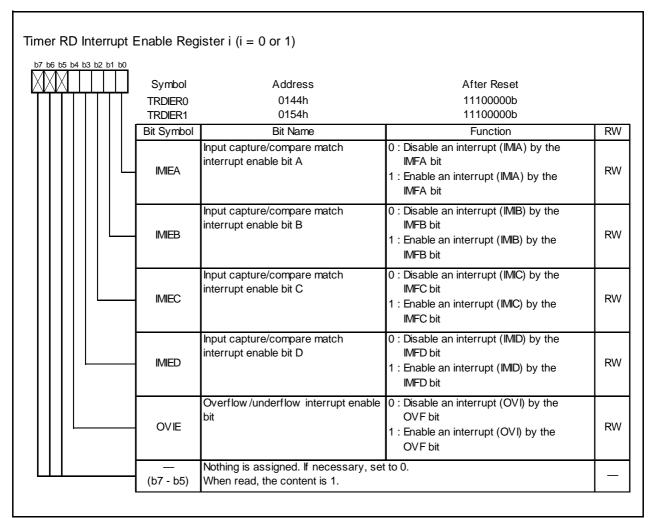
**Figure 14.70** Registers TRDIER0 to TRDIER1 in PWM Mode
