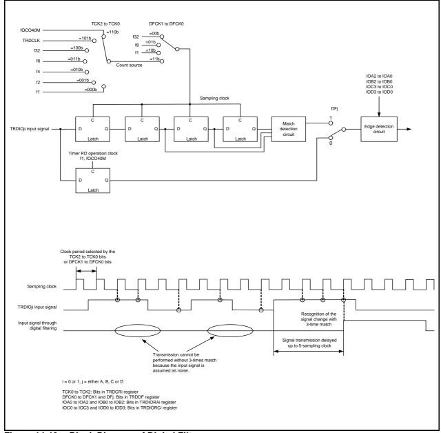
Figure 14.46 Block Diagram of Digital Filter
