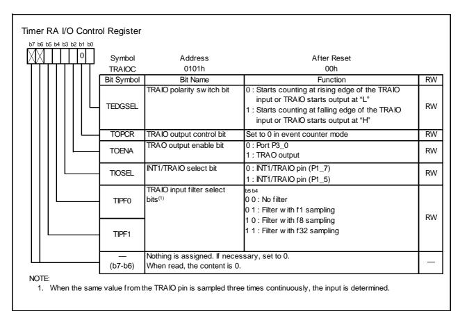
Figure 14.8 TRAIOC Register in Event Counter Mode
