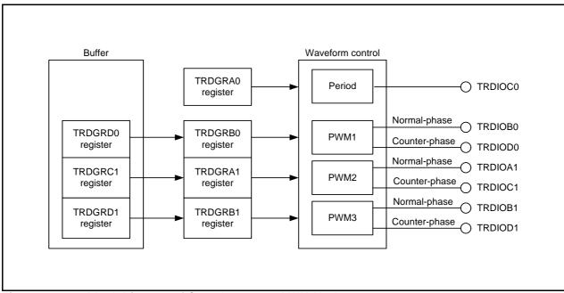
Figure 14.86 Block Diagram of Complementary PWM Mode
