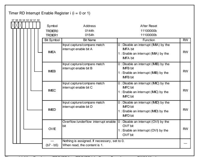
Registers TRDIER0 to TRDIER1 in Reset Synchronous PWM Mode **Figure 14.82**
