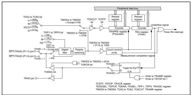
Figure 14.1 Block Diagram of Timer RA
