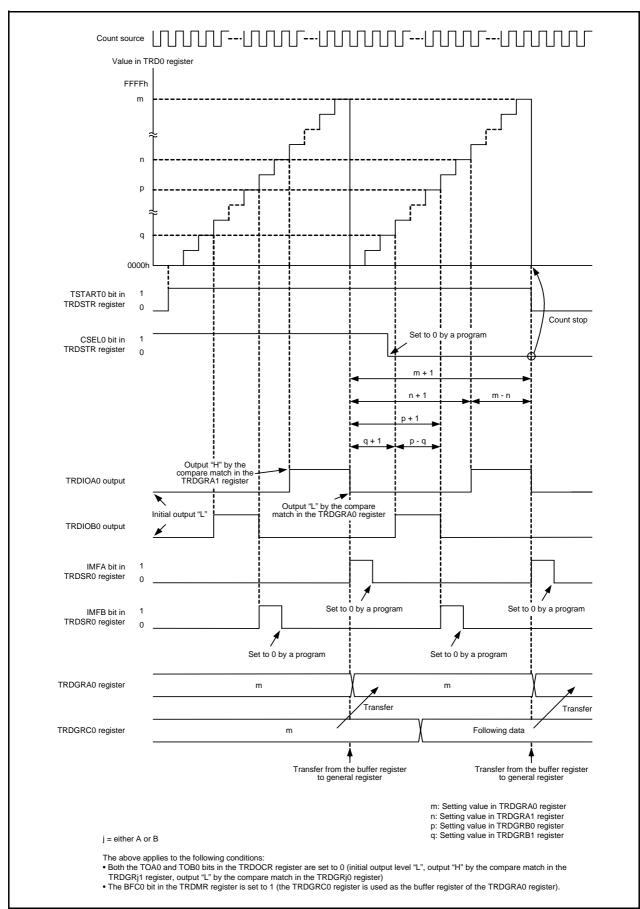
Figure 14.108 Operating Example of PWM3 Mode
