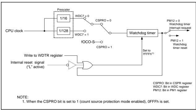
Figure 13.1 Block Diagram of Watchdog Timer
