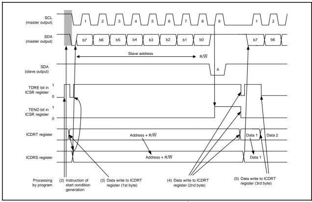
**Figure 16.33** Operating Timing in Master Transmit Mode (I<sup>2</sup>C Bus Interface Mode) (1)
