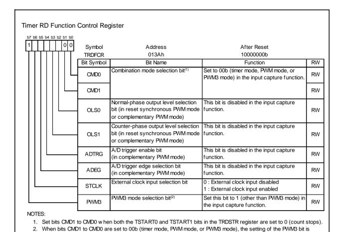
**Figure 14.36** TRDFCR Register in Input Capture Function
