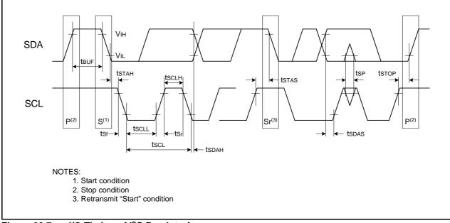
Figure 20.7 I/O Timing of I<sup>2</sup>C Bus Interface
