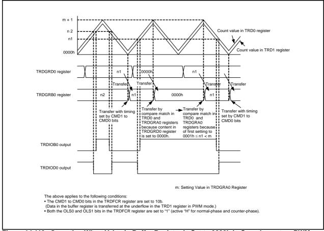
Figure 14.113 Operation When Value in Buffer Register Is Set to 0000h in Complementary PWM
