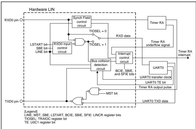
Figure 17.1 Block Diagram of Hardware LIN
