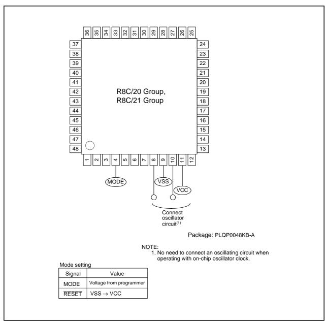
**Figure 19.17** Pin Connections for Standard Serial I/O Mode 3
