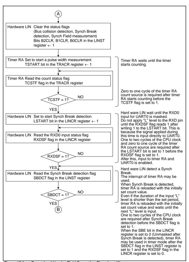
Figure 17.9 Example of Header Field Reception Flowchart (2)
