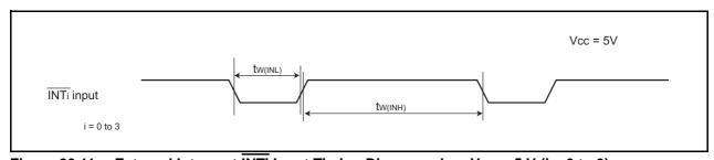
External Interrupt INTi Input Timing Diagram when Vcc = 5 V (i = 0 to 3) **Figure 20.11**
