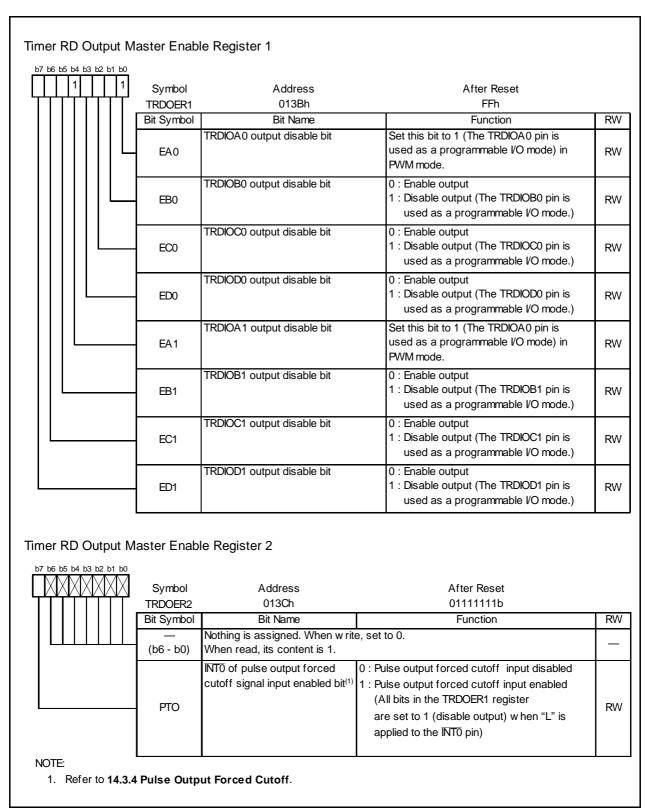
**Figure 14.67** Registers TRDOER1 to TRDOER2 in PWM Mode
