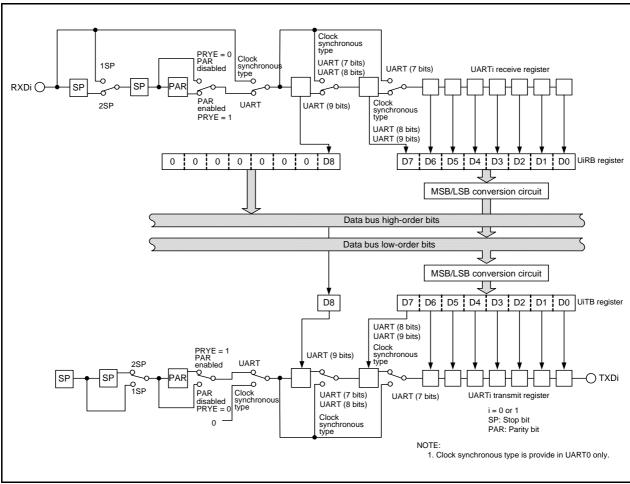
Figure 15.2 UARTi (i = 0 or 1) Transmit/Receive Unit
