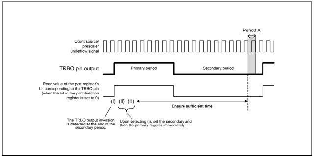
Workaround Example (b) When TRBO Pin Output Value is Read **Figure 14.26**
