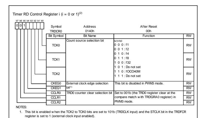
Figure 14.103 TRDCR0 Register in PWM3 Mode
