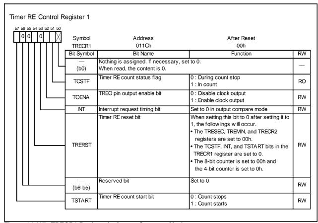
Figure 14.117 TRECR1 Register in Output Compare Mode
