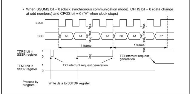
Example of Clock Synchronous Serial I/O with Chip Select Operation for Data **Figure 16.13 Transmission (Clock Synchronous Communication Mode)**
