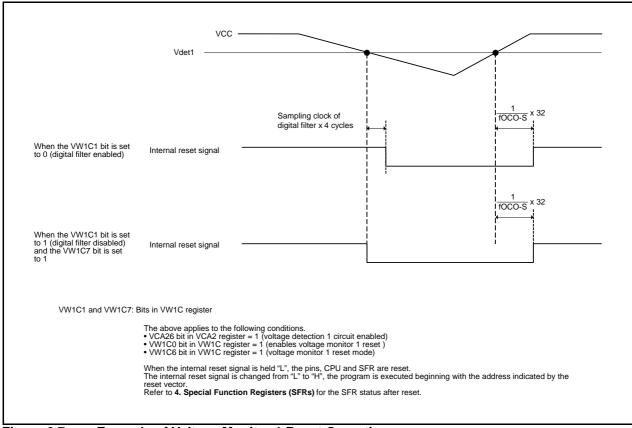
Figure 6.7 Example of Voltage Monitor 1 Reset Operation
