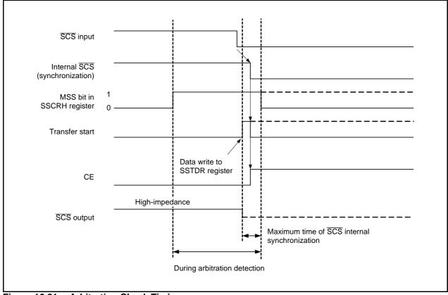
**Figure 16.21 Arbitration Check Timing**
