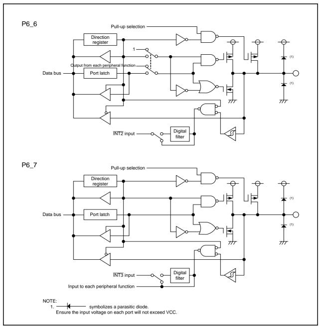
Figure 7.7 Configuration of Programmable I/O Ports (7)
