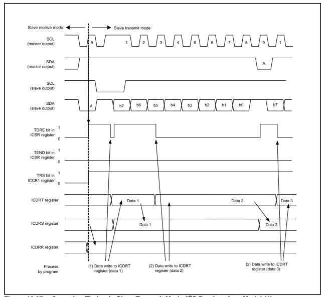
**Figure 16.37** Operating Timing in Slave Transmit Mode (I<sup>2</sup>C Bus Interface Mode) (1)
