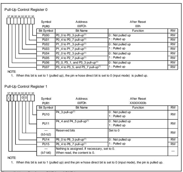
Figure 7.11 Registers PUR0 and PUR1
