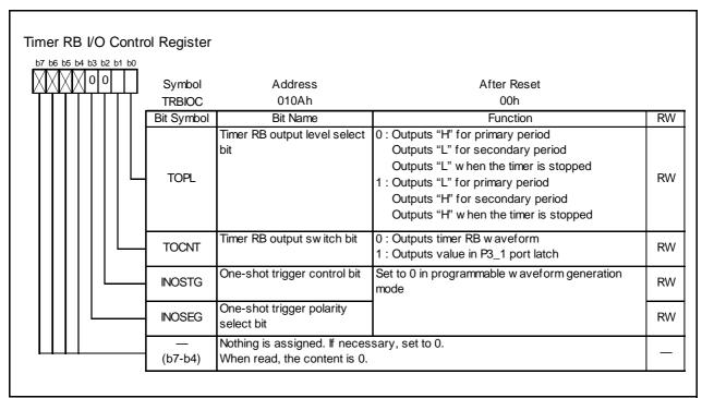
**Figure 14.19** TRBIOC Register in Programmable Waveform Generation Mode
