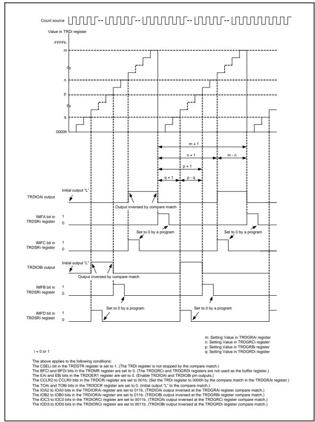
Operating Example When TRDGRCi Register is Used for Output Control of TRDIOAi **Figure 14.62** Pin and TRDGRDi Register is Used for Output Control of TRDIOBi Pin
