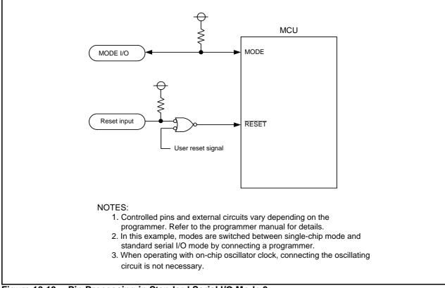
Figure 19.19 Pin Processing in Standard Serial I/O Mode 3
