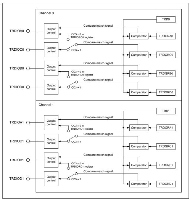
Figure 14.47 Block Diagram of Output Compare Function
