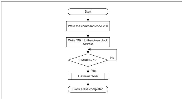
Figure 19.14 Block Erase Command (When Erase-Suspend Function Disabled)
