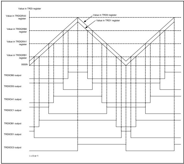
**Figure 14.96 Output Model of Complementary PWM Mode**
