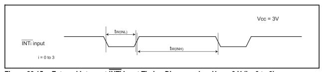
Figure 20.15 External Interrupt INTi Input Timing Diagram when Vcc = 3 V (i = 0 to 3)
