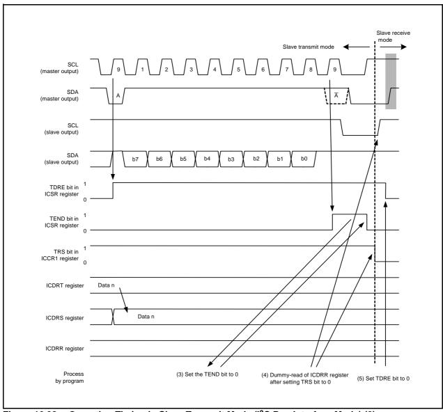
**Figure 16.38** Operating Timing in Slave Transmit Mode (I<sup>2</sup>C Bus Interface Mode) (2)
