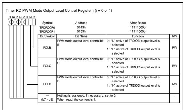
**Figure 14.71** Registers TRDPOCR0 to TRDPOCR1 in PWM Mode
