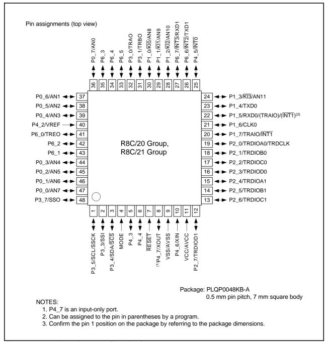
Figure 1.4 Pin Assignments (Top View)
