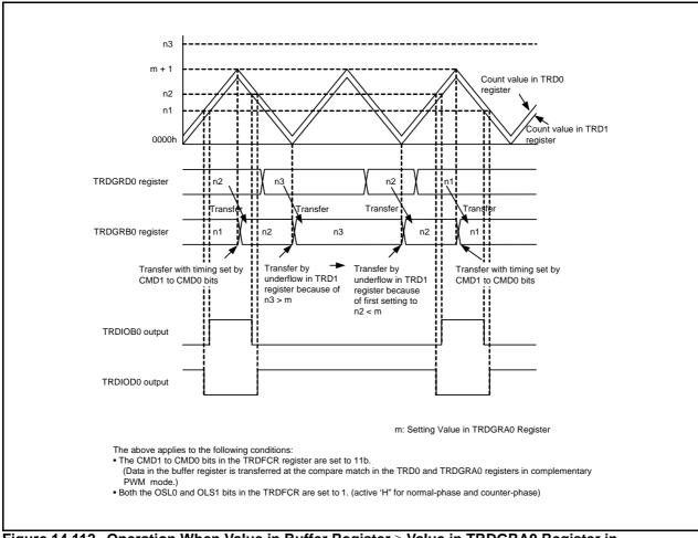
Figure 14.112 Operation When Value in Buffer Register ≥ Value in TRDGRA0 Register in **Complementary PWM Mode**
