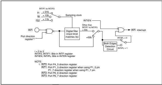
**Figure 12.14 Configuration of INTi Input Filter**
