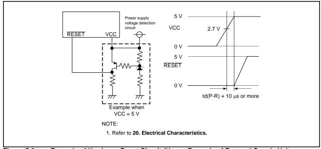
Example of Hardware Reset Circuit (Usage Example of External Supply Voltage Figure 5.6 **Detection Circuit) and Operation**
