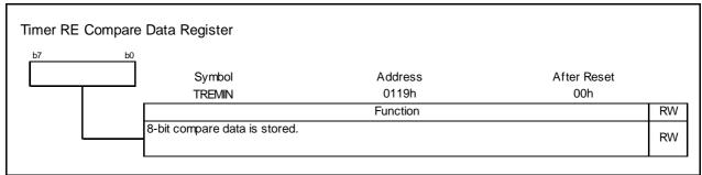
Figure 14.116 TREMIN Register in Output Compare Mode
