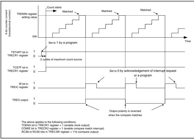
Figure 14.120 Operation in Output Compare Mode
