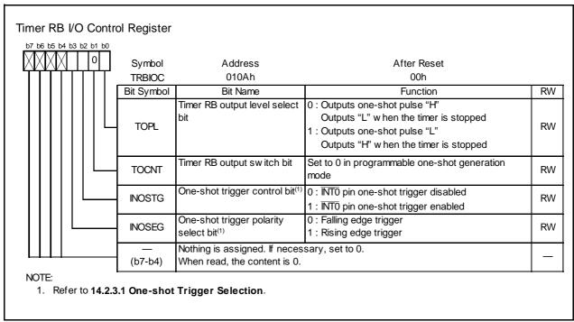
Figure 14.21 TRBIOC Register in Programmable One-Shot Generation Mode
