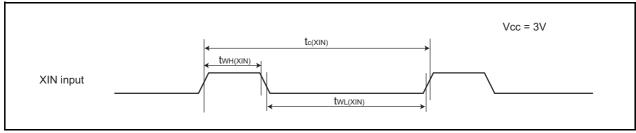
XIN Input Timing Diagram when Vcc = 3 V Figure 20.12
