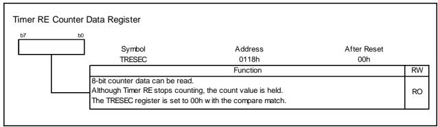
Figure 14.115 TRESEC Register in Output Compare Mode
