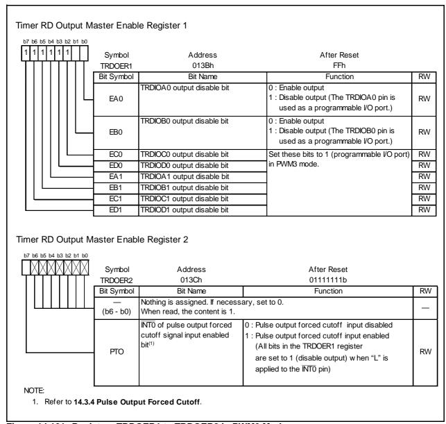
Figure 14.101 Registers TRDOER1 to TRDOER2 in PWM3 Mode
