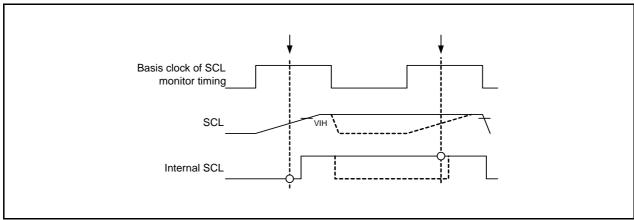
**Figure 16.45 Timing of Bit Synchronous Circuit**
