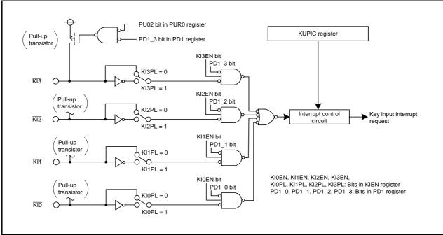
Figure 12.16 Block Diagram of Key Input Interrupt
