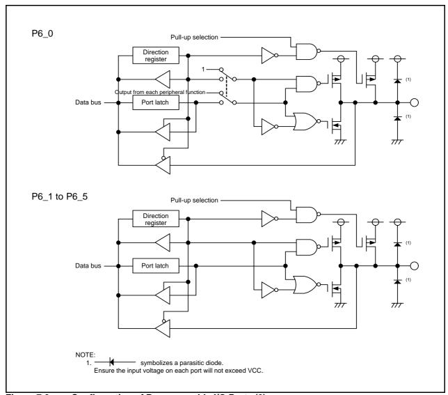
Figure 7.6 Configuration of Programmable I/O Ports (6)
