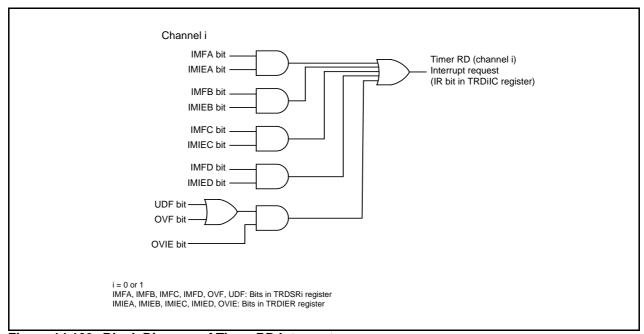
Figure 14.109 Block Diagram of Timer RD Interrupt
