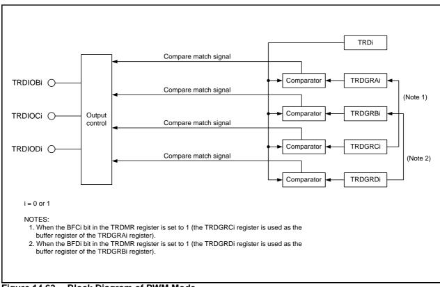
Figure 14.63 Block Diagram of PWM Mode
