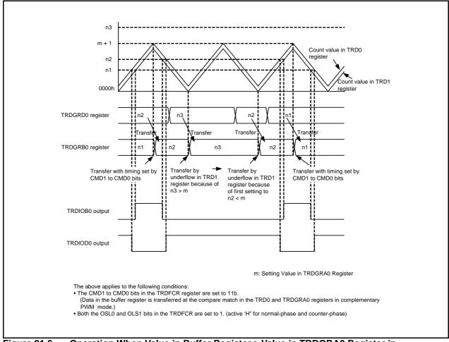
Operation When Value in Buffer Register ≥ Value in TRDGRA0 Register in Figure 21.6 **Complementary PWM Mode**
