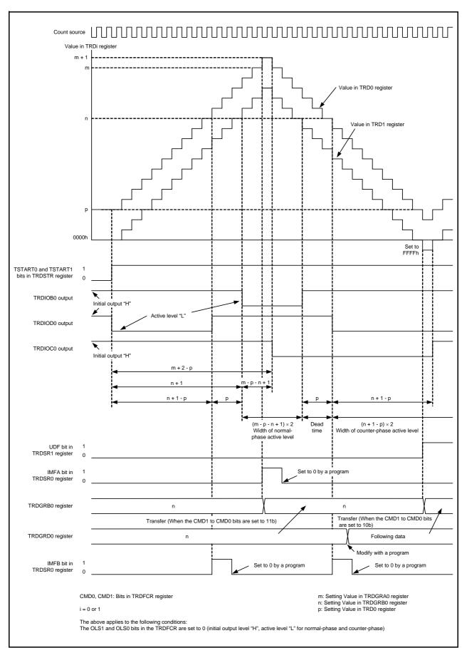
**Figure 14.97 Operating Example of Complementary PWM Mode**
