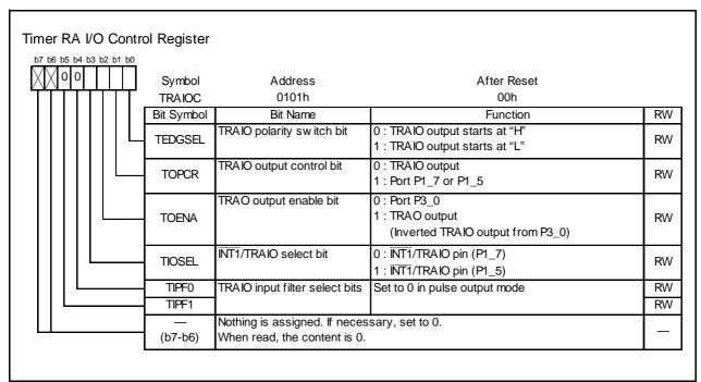
Figure 14.7 **TRAIOC Register in Pulse Output Mode**
