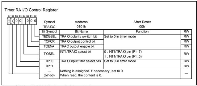
Figure 14.5 **TRAIOC Register in Timer Mode**
