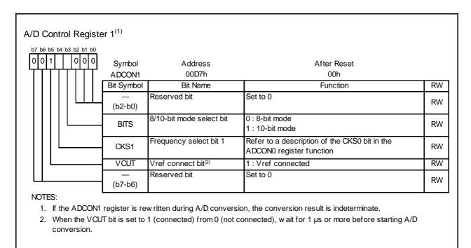
Figure 18.5 **ADCON1 Register in One-Shot Mode**
