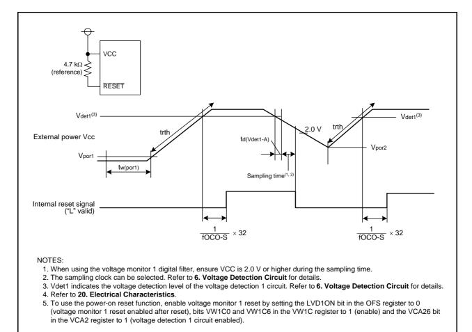
Figure 5.7 Example of Power-On Reset Circuit and Operation
