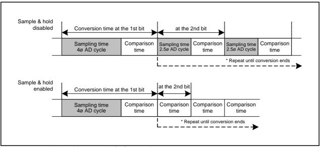
Figure 18.8 Timing Diagram of A/D Conversion
