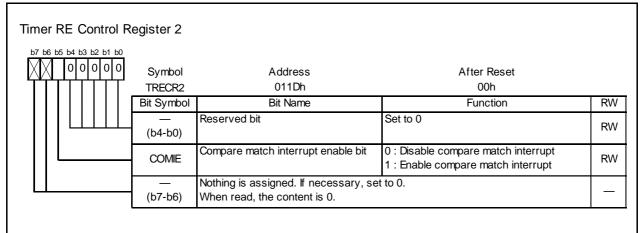
Figure 14.118 TRECR2 Register in Output Compare Mode
