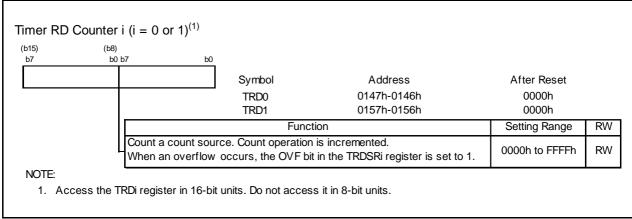
Figure 14.72 Registers TRD0 to TRD1 in PWM Mode
