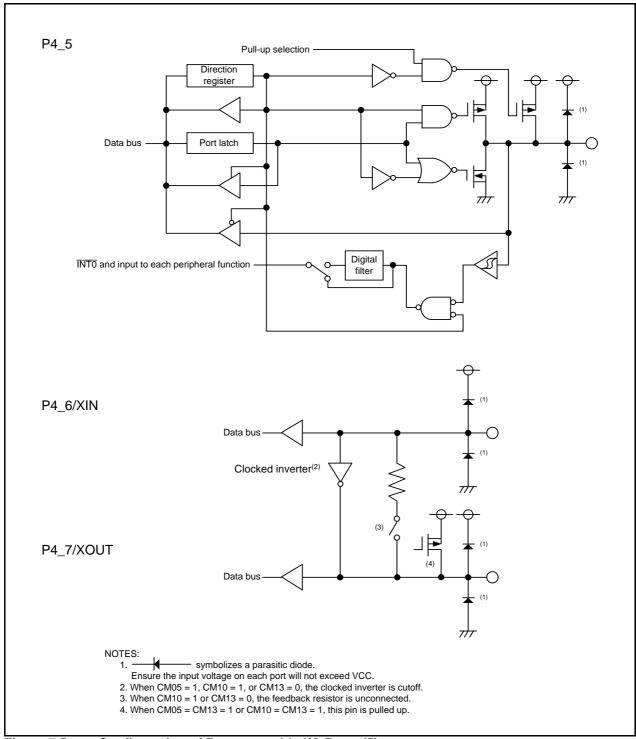
Figure 7.5 Configuration of Programmable I/O Ports (5)
