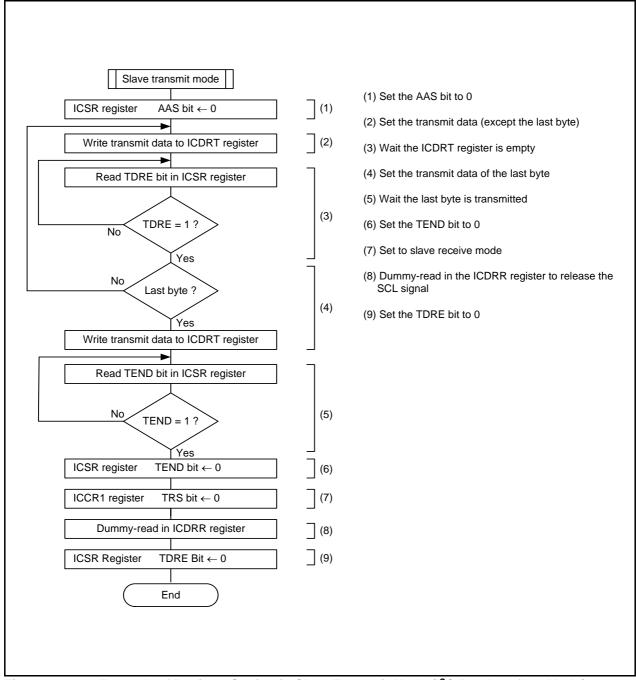
Example of Register Setting in Slave Transmit Mode (I<sup>2</sup>C Bus Interface Mode) **Figure 16.48**
