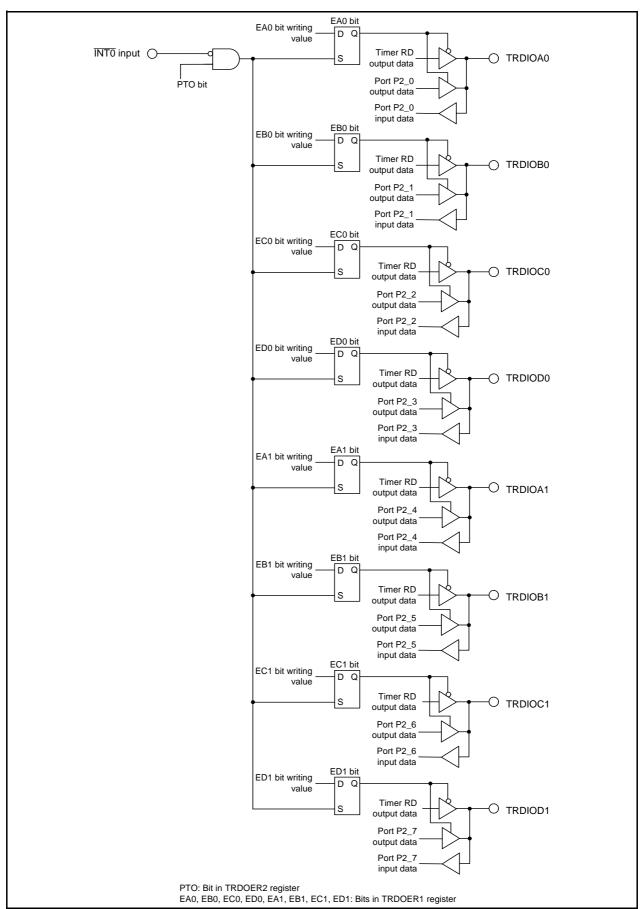
**Figure 14.32 Pulse Output Forced Cutoff**
