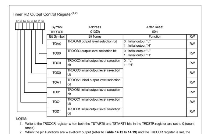
Figure 14.52 TRDOCR Register in Output Compare Function
