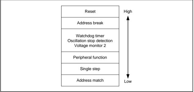
Figure 12.10 Priority Levels of Hardware Interrupts
