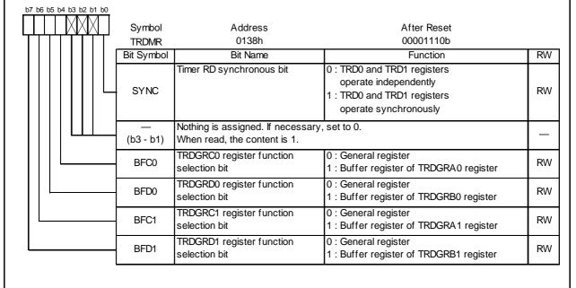
**Figure 14.34** Registers TRDSTR and TRDMR in Input Capture Function
