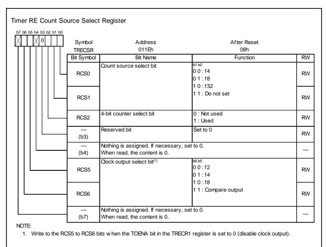
Figure 14.119 TRECSR Register in Output Compare Mode
