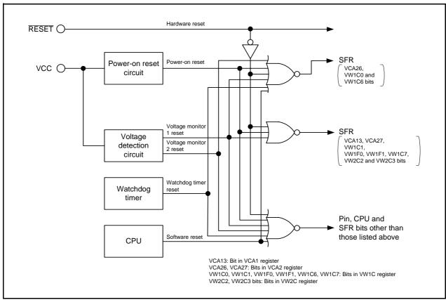
Figure 5.1 Block Diagram of Reset Circuit
