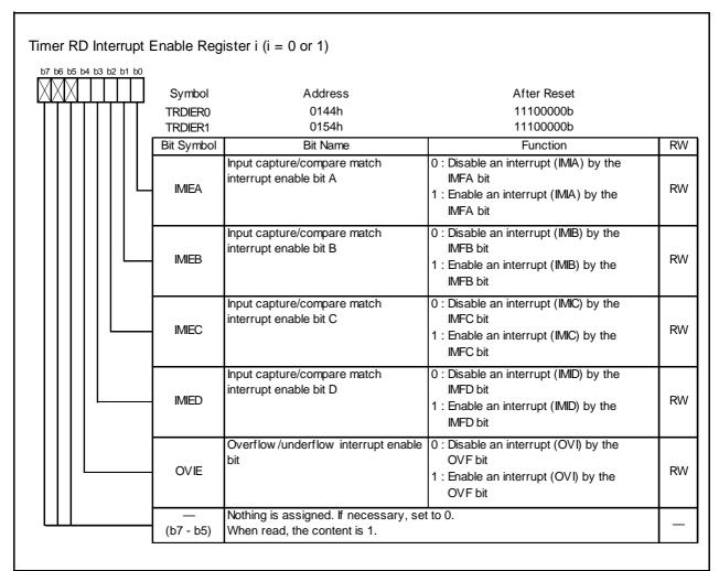
**Figure 14.57** Registers TRDIER0 to TRDIER1 in Output Compare Function
