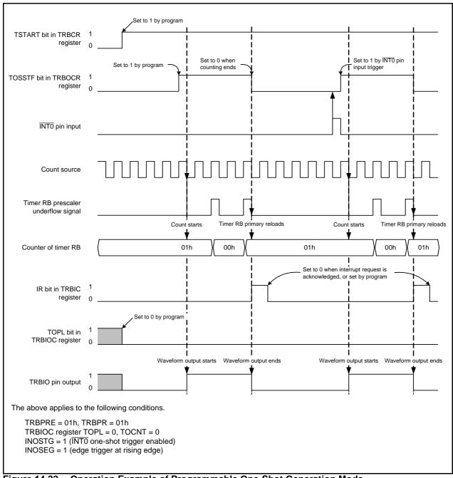
Figure 14.22 Operation Example of Programmable One-Shot Generation Mode
