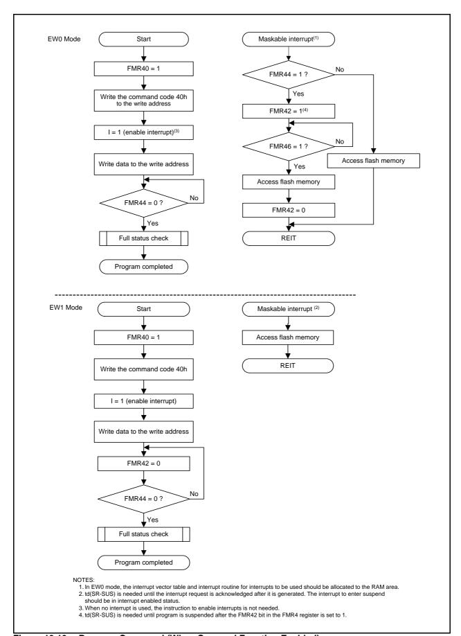
Figure 19.13 Program Command (When Suspend Function Enabled)
