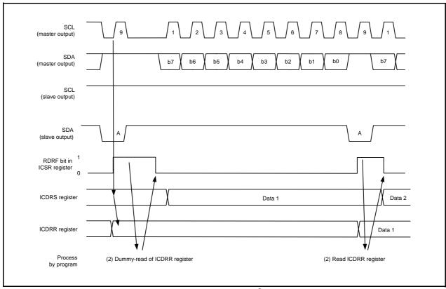
**Figure 16.39** Operating Timing in Slave Receive Mode (I<sup>2</sup>C Bus Interface Mode) (1)
