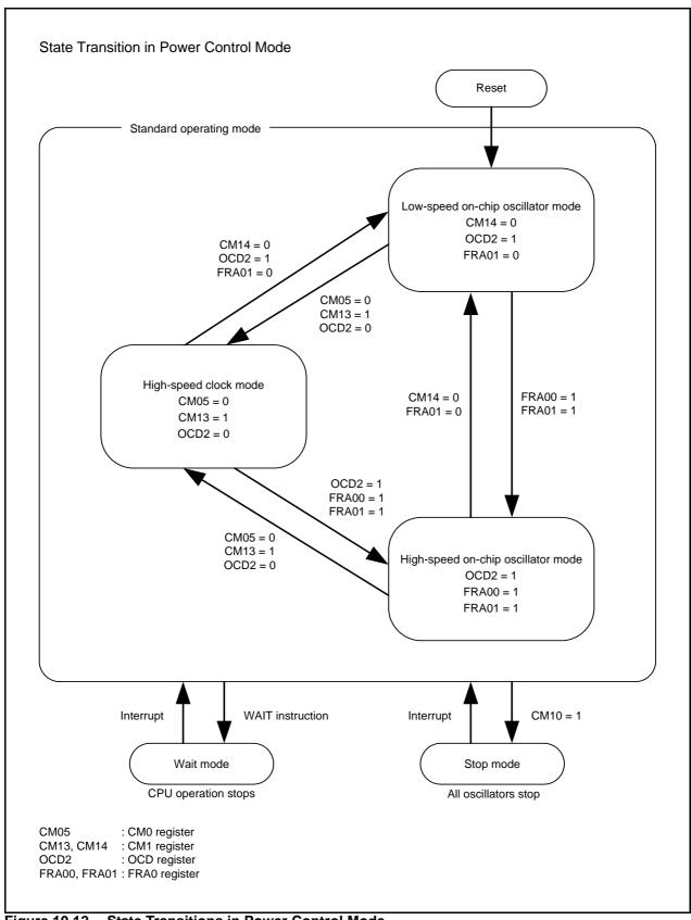
Figure 10.12 **State Transitions in Power Control Mode**
