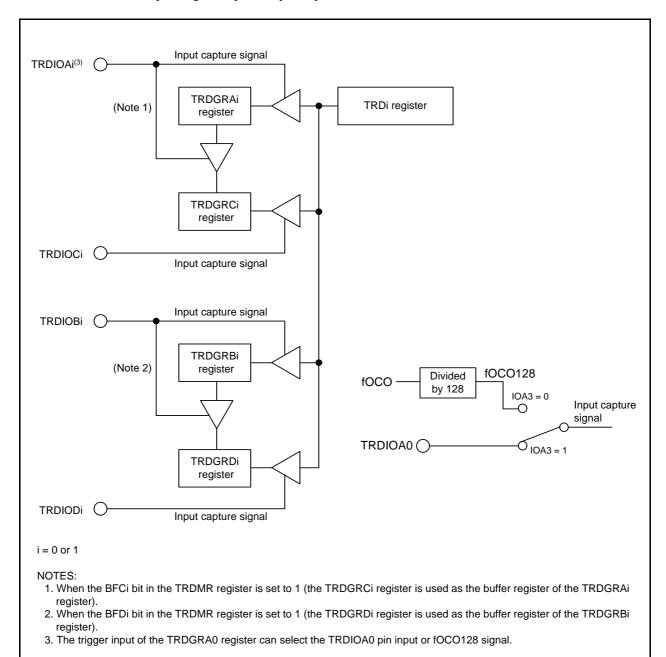
Figure 14.33 Block Diagram of Input Capture Function
