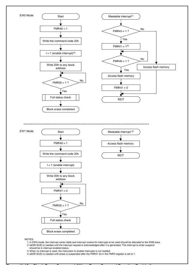
**Block Erase Command (When Erase-Suspend Function Enabled) Figure 19.15**
