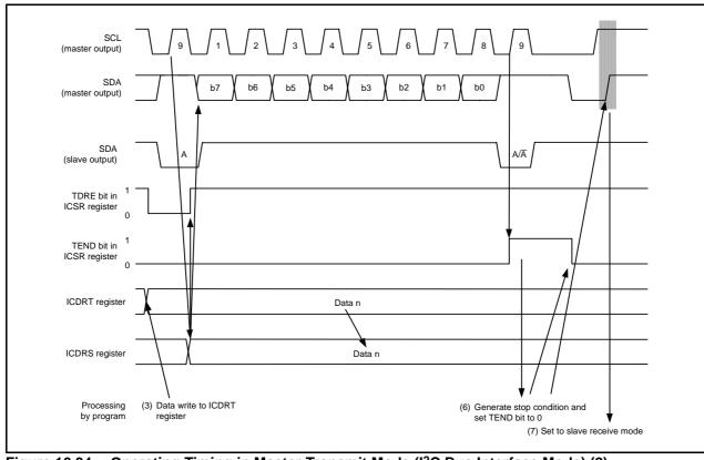
**Figure 16.34** Operating Timing in Master Transmit Mode (I<sup>2</sup>C Bus Interface Mode) (2)
