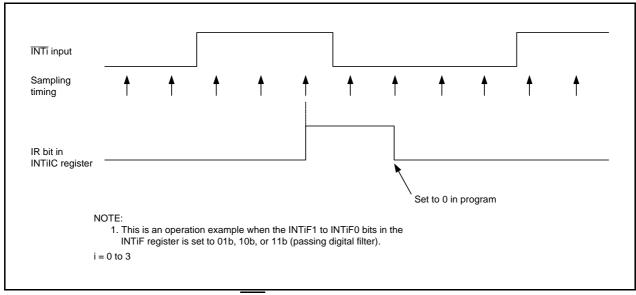
**Figure 12.15 Operating Example of INTi Input Filter**
