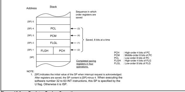
Figure 12.9 Register Saving Operation
