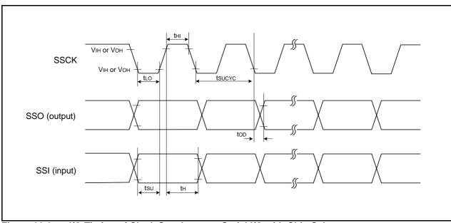
I/O Timing of Clock Synchronous Serial I/O with Chip Select (Clock Synchronous Communication Mode) Figure 20.6
