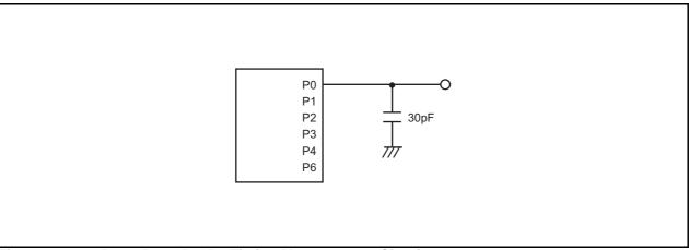
Ports P0 to P4, P6 Timing Measurement Circuit Figure 20.1
