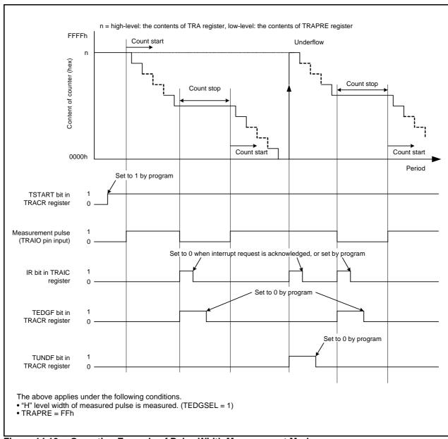
Figure 14.10 Operating Example of Pulse Width Measurement Mode
