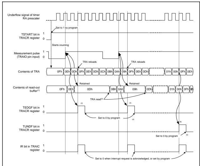
Conditions: A period from one rising edge to the next rising edge of measurement pulse is measured (TEDGSEL = 0) with the default value of the TRA register as 0Fh.
