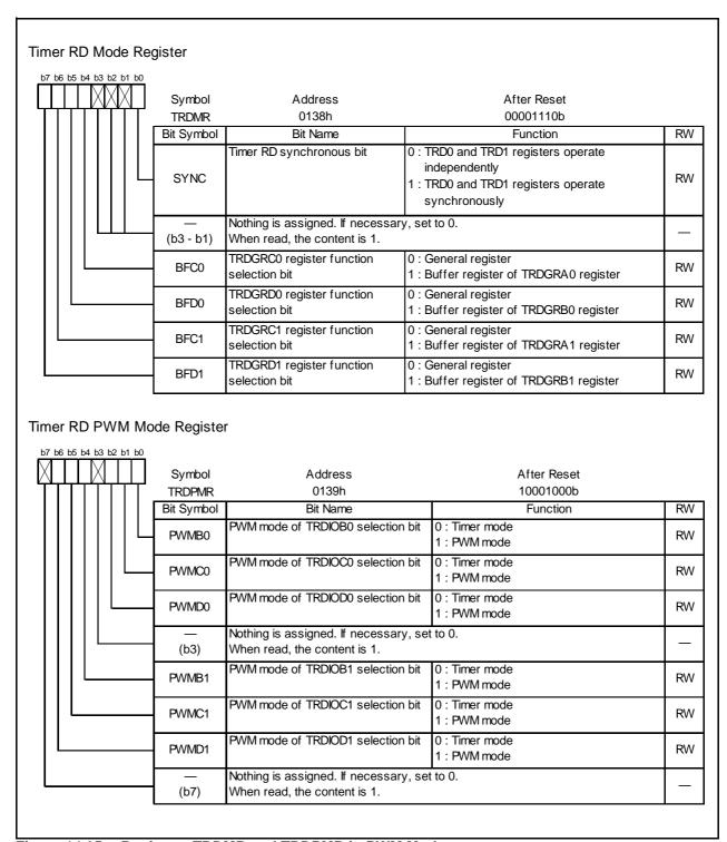
**Figure 14.65** Registers TRDMR and TRDPMR in PWM Mode
