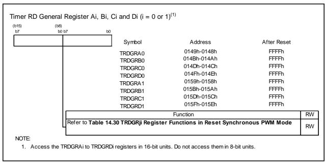
**Figure 14.84** Registers TRDGRAi, TRDGRBi, TRDGRCi and TRDGRDi in Reset Synchronous PWM Mode
