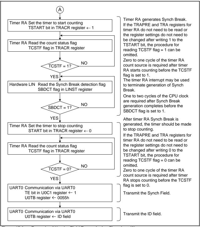
Figure 17.6 **Example of Header Field Transmission Flowchart (2)**
