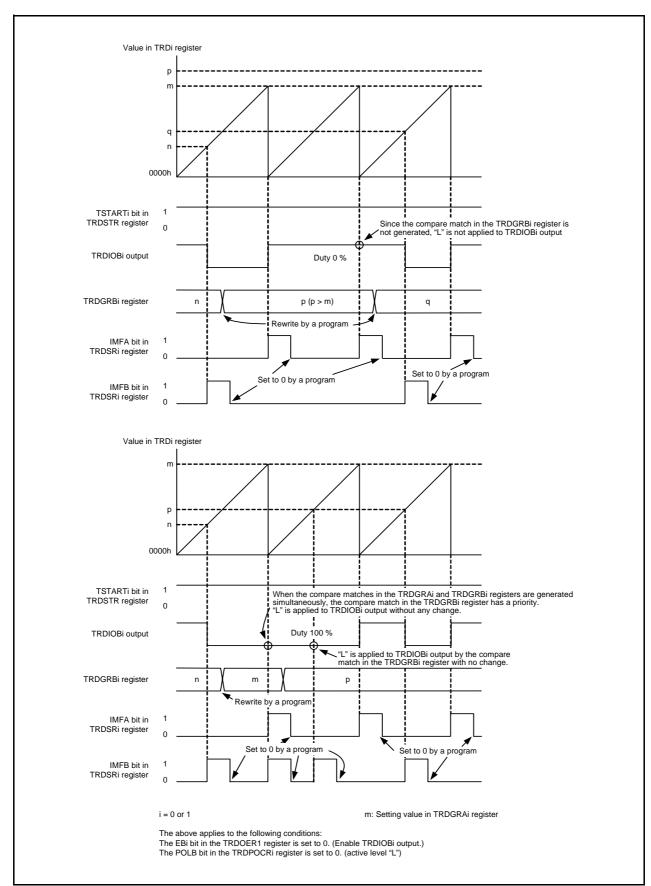
Figure 14.75 Operating Example of PWM Mode (Duty 0%, Duty 100%)
