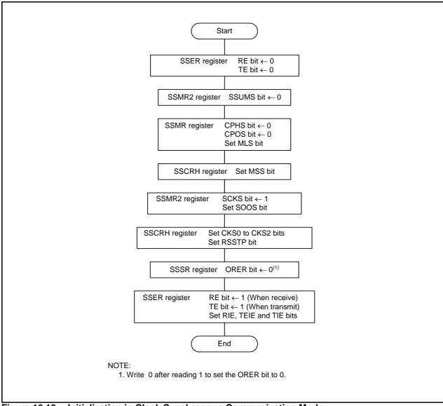
**Figure 16.12 Initialization in Clock Synchronous Communication Mode**
