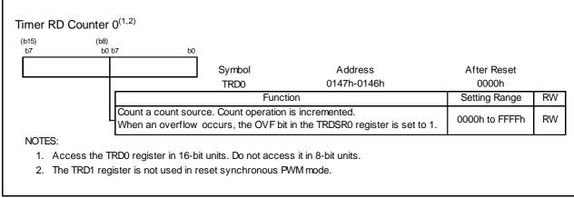
**Figure 14.83** TRD0 Registrar in Reset Synchronous PWM Mode
