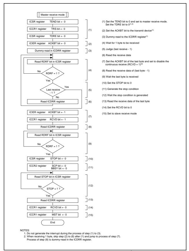
**Figure 16.47** Example of Register Setting in Master Receive Mode (I<sup>2</sup>C Bus Interface Mode)
