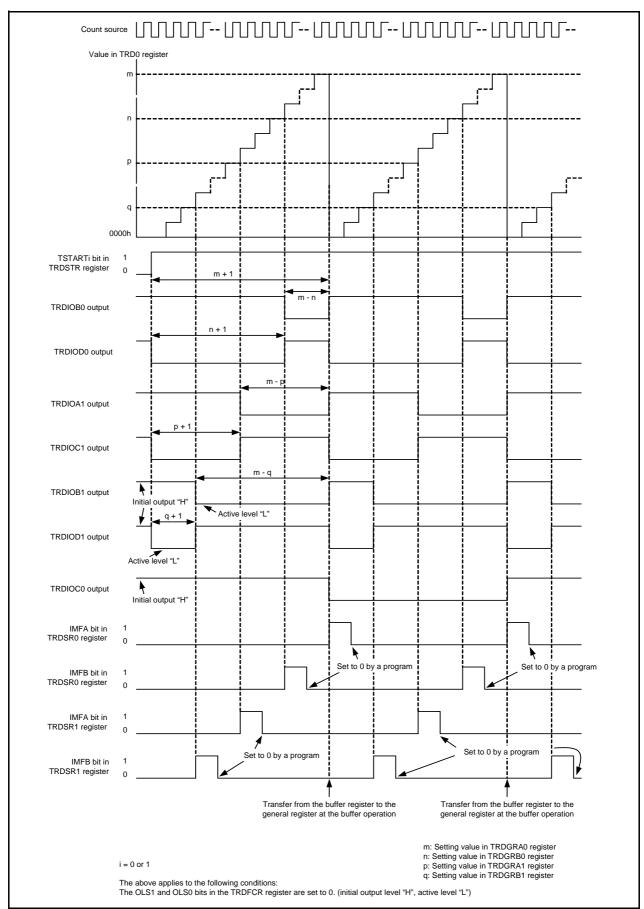
**Figure 14.85 Operating Example of Reset Synchronous PWM Mode**
