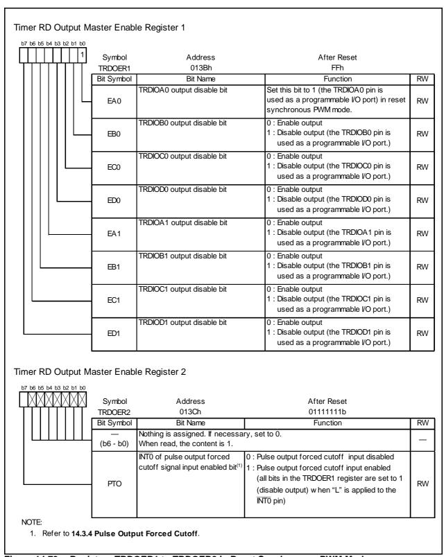
Figure 14.79 Registers TRDOER1 to TRDOER2 in Reset Synchronous PWM Mode
