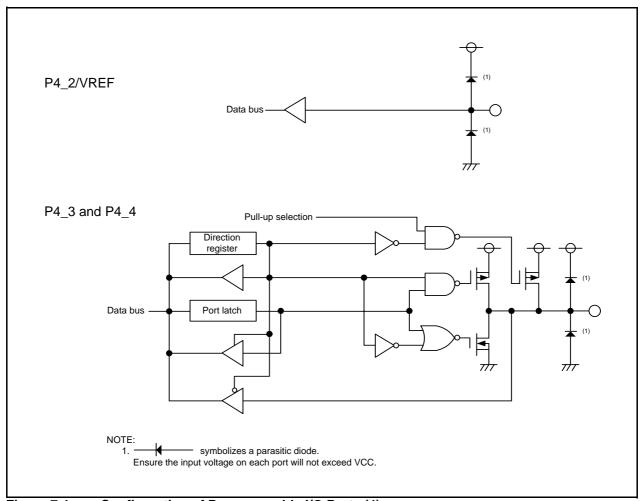
Configuration of Programmable I/O Ports (4) Figure 7.4
