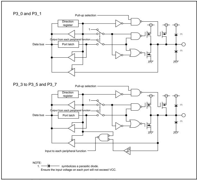
Figure 7.3 Configuration of Programmable I/O Ports (3)
