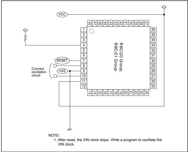
Appendix Figure 3.1 Example of Oscillation Evaluation Circuit
