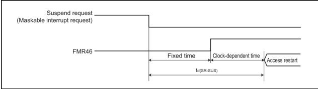
Figure 20.2 Time delay until Suspend
