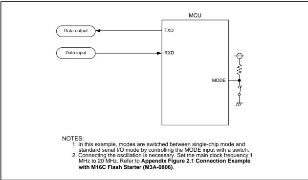
Figure 19.18 Pin Processing in Standard Serial I/O Mode 2
