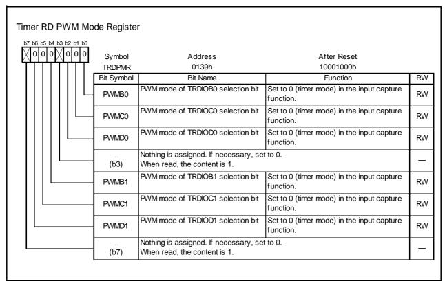
**Figure 14.35 TRDPMR Register in Input Capture Function**
