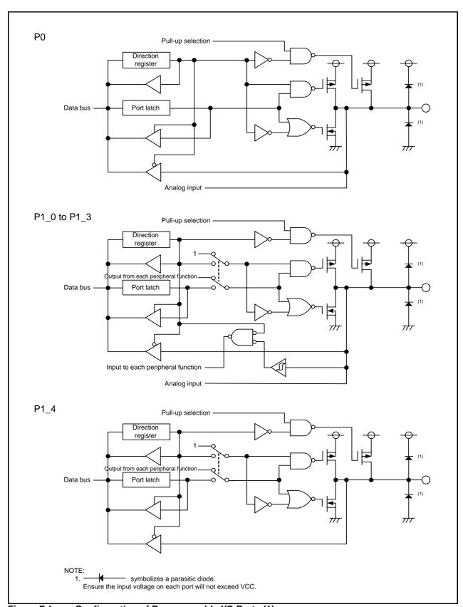
Figure 7.1 Configuration of Programmable I/O Ports (1)
