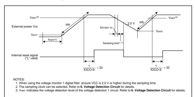
Figure 20.3 **Power-on Reset Circuit Electrical Characteristics**
