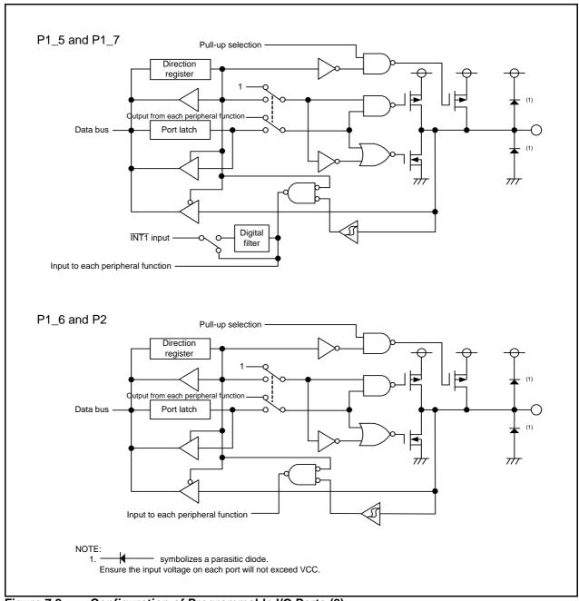
Figure 7.2 Configuration of Programmable I/O Ports (2)
