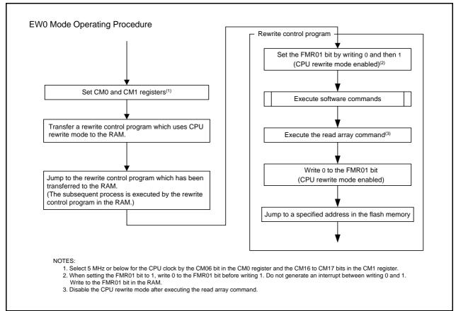
Figure 19.9 How to Set and Exit EW0 Mode
