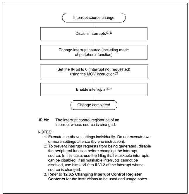
Figure 21.1 Example of Procedure for Changing Interrupt Sources
