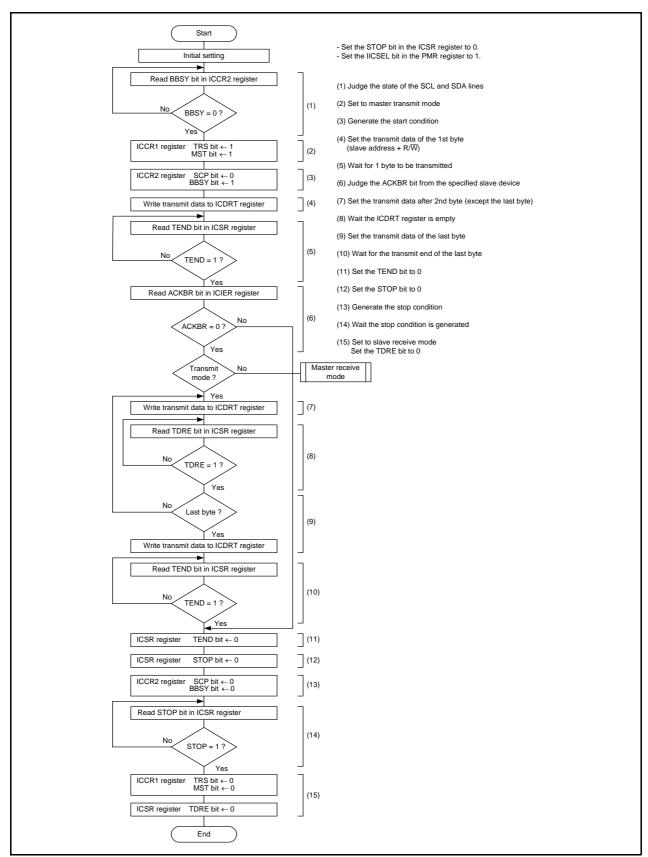
Example of Register Setting in Master Transmit Mode (I<sup>2</sup>C Bus Interface Mode) **Figure 16.46**
