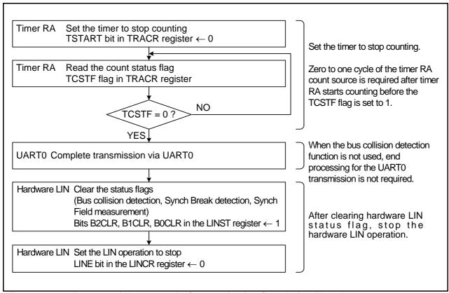
Figure 17.12 Example of Hardware LIN Communication Completion Flowchart
