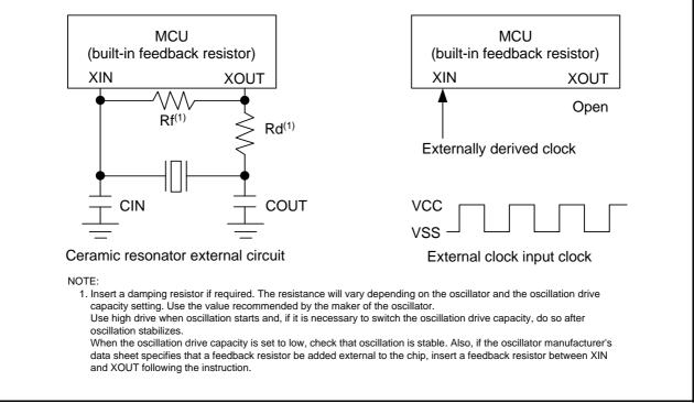
Figure 10.8 Examples of XIN Clock Connection Circuit
