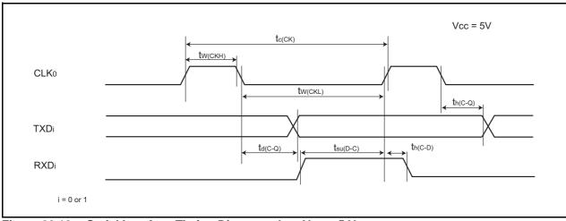
Serial Interface Timing Diagram when Vcc = 5 V Figure 20.10
