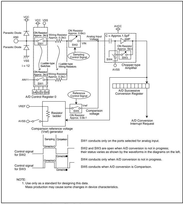
**Figure 18.10 Internal Equivalent Circuit of Analog Input**
