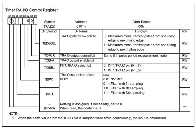
**Figure 14.11** TRAIOC Register in Pulse Period Measurement Mode
