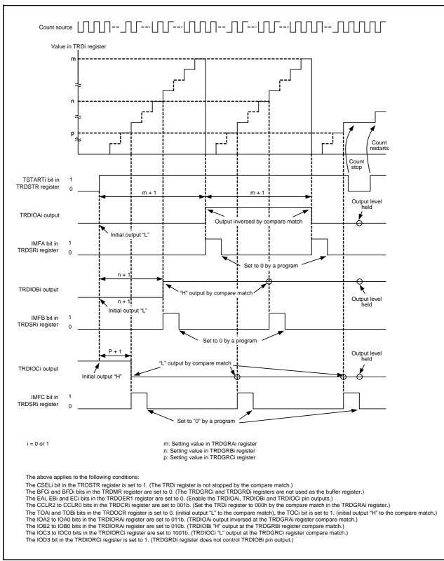
**Figure 14.60 Operating Example of Output Compare Function**
