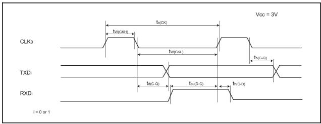
Serial Interface Timing Diagram when Vcc = 3 V **Figure 20.14**
