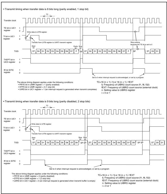
**Figure 15.10 Transmit Timing in UART Mode**
