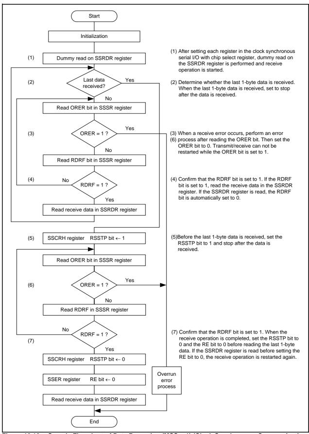
Sample Flowchart of Data Reception (MSS = 1) (Clock Synchronous Communication **Figure 16.16** Mode)
