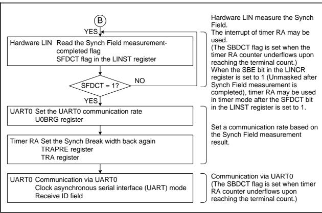
Figure 17.10 Example of Header Field Reception Flowchart (3)
