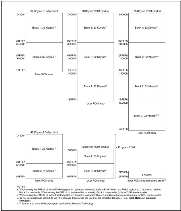
Figure 19.1 Flash Memory Block Diagram for R8C/20 Group
