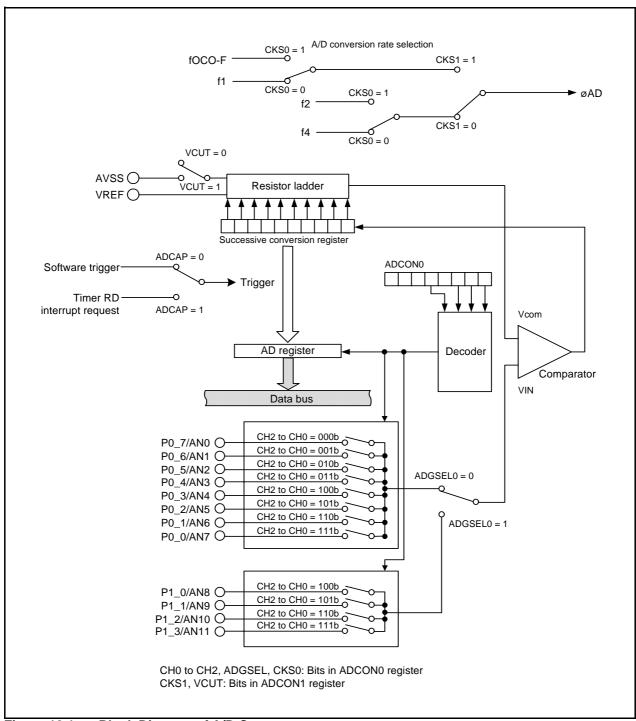
Figure 18.1 Block Diagram of A/D Converter
