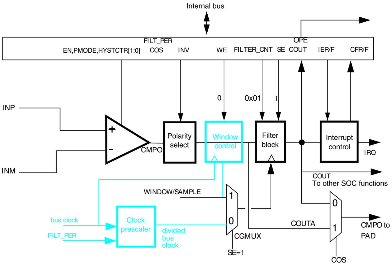
**Figure 32-28. Sampled, Non-Filtered (# 3A): sampling point externally driven**
