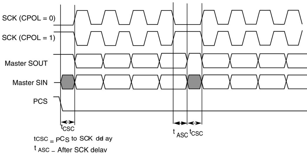
**Figure 46-74. Example of continuous transfer (CPHA=1, CONT=1)**
