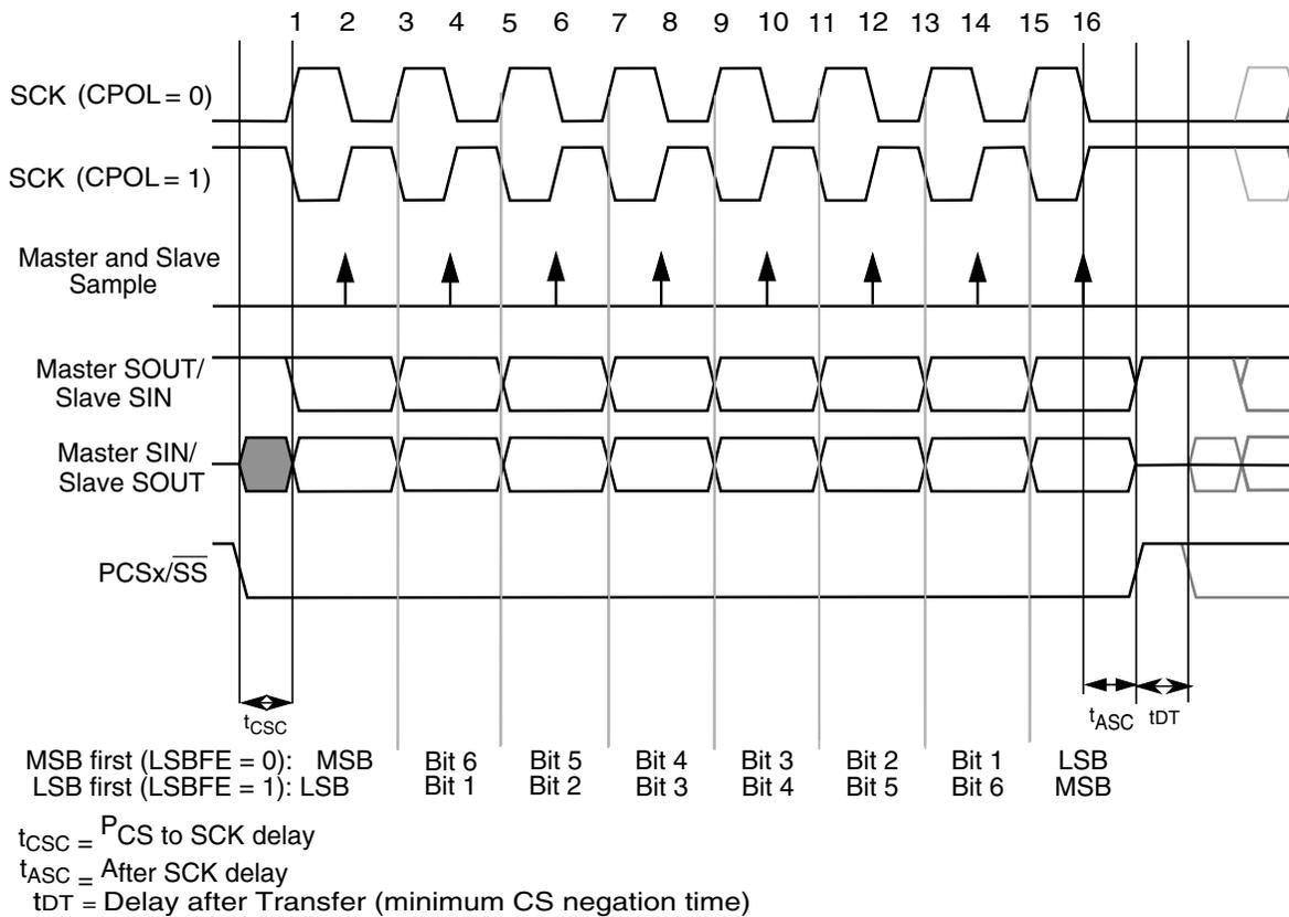
**Figure 46-72. Module transfer timing diagram (MTFE=0, CPHA=1, FMSZ=8)**
