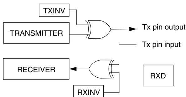
Figure 48-70. Single-wire operation (C1[LOOPS] = 1, C1[RSRC] = 1)
