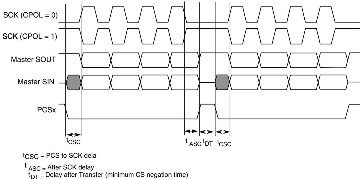
**Figure 46-73. Example of non-continuous format (CPHA=1, CONT=0)**
