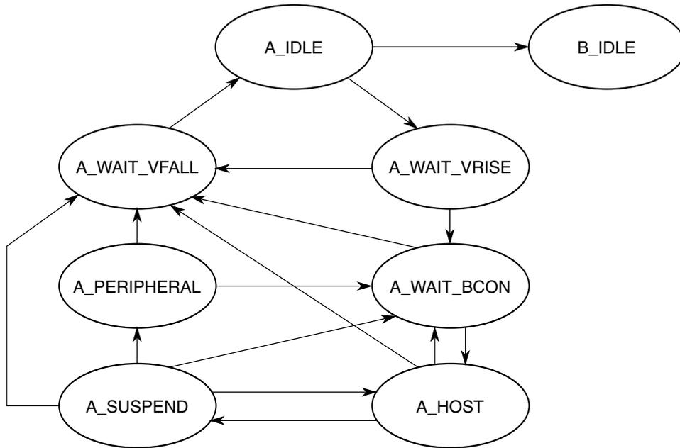
**Figure 43-93. Dual role A device flow diagram**
