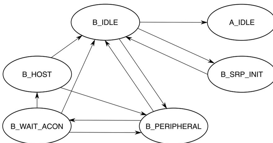
**Figure 43-94. Dual role B device flow diagram**
