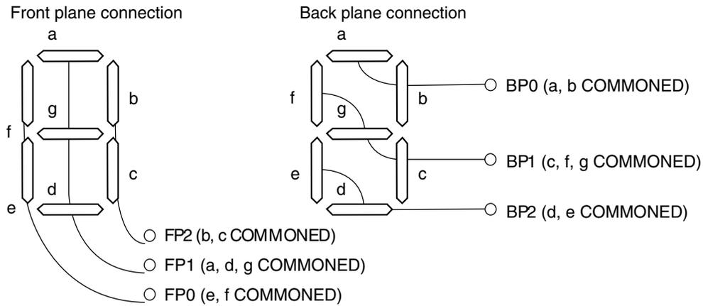
The above segment assignments are provided by the specification for the LCD glass for this example. For this LCD controller any of the LCD pins can be configured to be front plane 0-2 or back plane 0-2. For this example, set LCD\_P0 as FP0, LCD\_P1 as FP1, and LCD\_P2 as FP2. For this example, set LCD\_P3 as BP0, LCD\_P4 as BP1 and LCD\_P5 as BP2.
