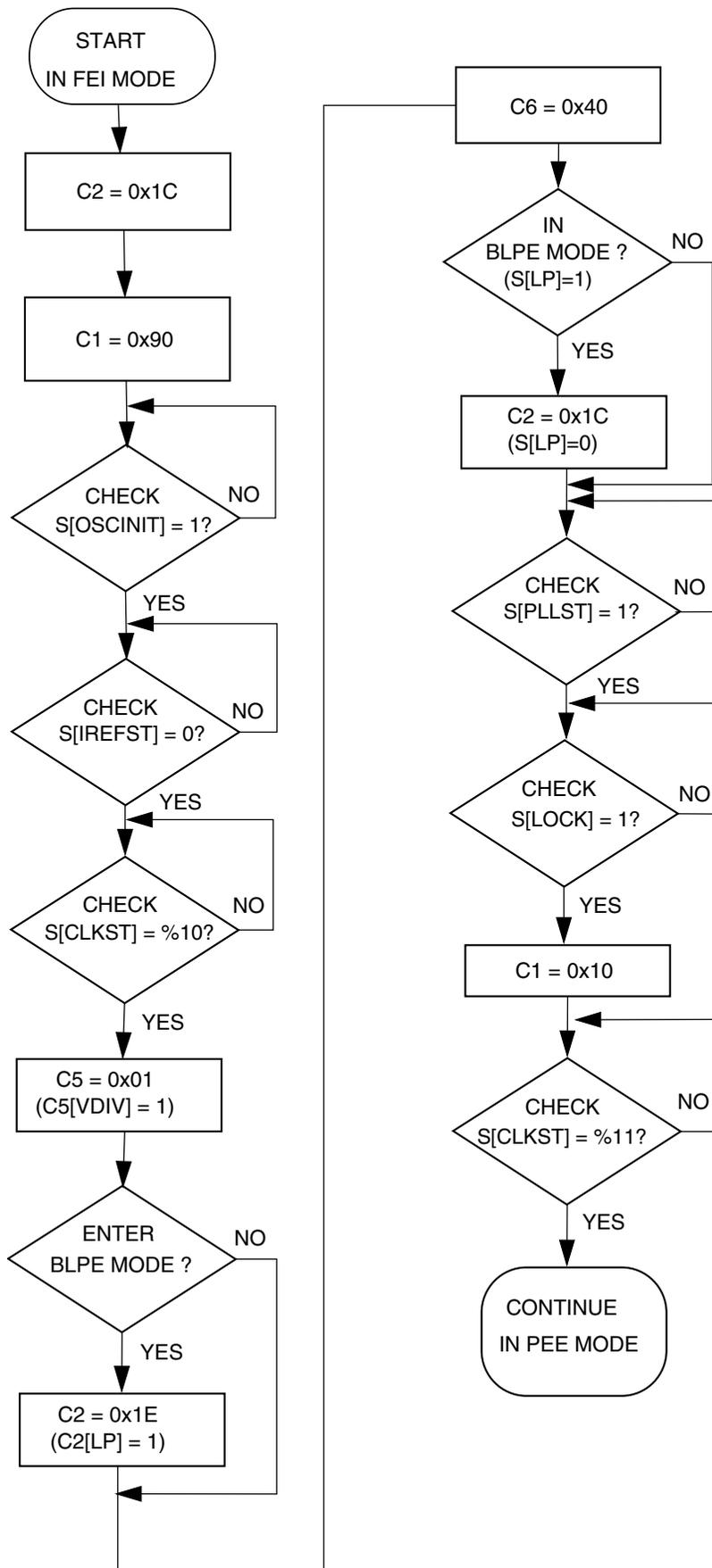
**Figure 24-15. Flowchart of FEI to PEE mode transition using an 4 MHz crystal**
