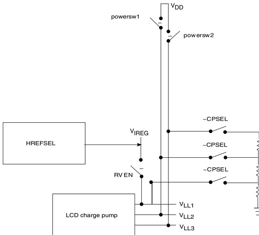
Figure 52-32. LCD charge pump block diagram
