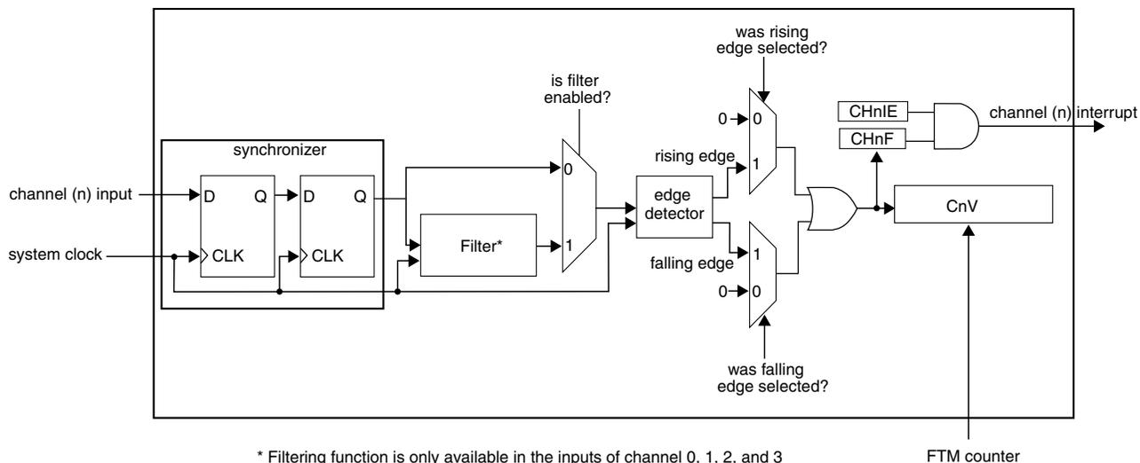
**Figure 38-175. Input Capture mode**
