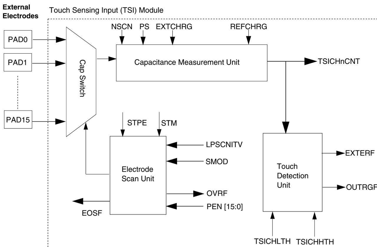
Figure 51-1. TSI block diagram
