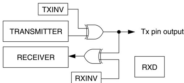
**Figure 48-71. Loop operation ( $C1[LOOPS] = 1$ ,  $C1[RSRC] = 0$ )**
