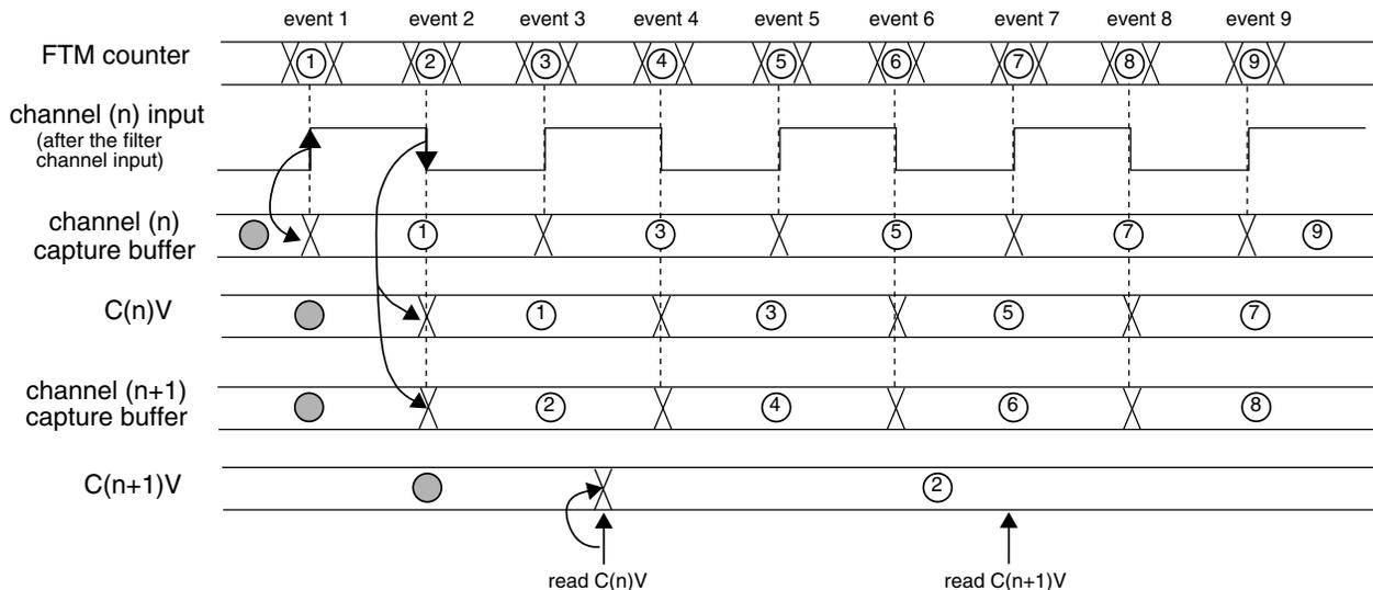
**Figure 38-249. Dual Edge Capture mode read coherency mechanism**
