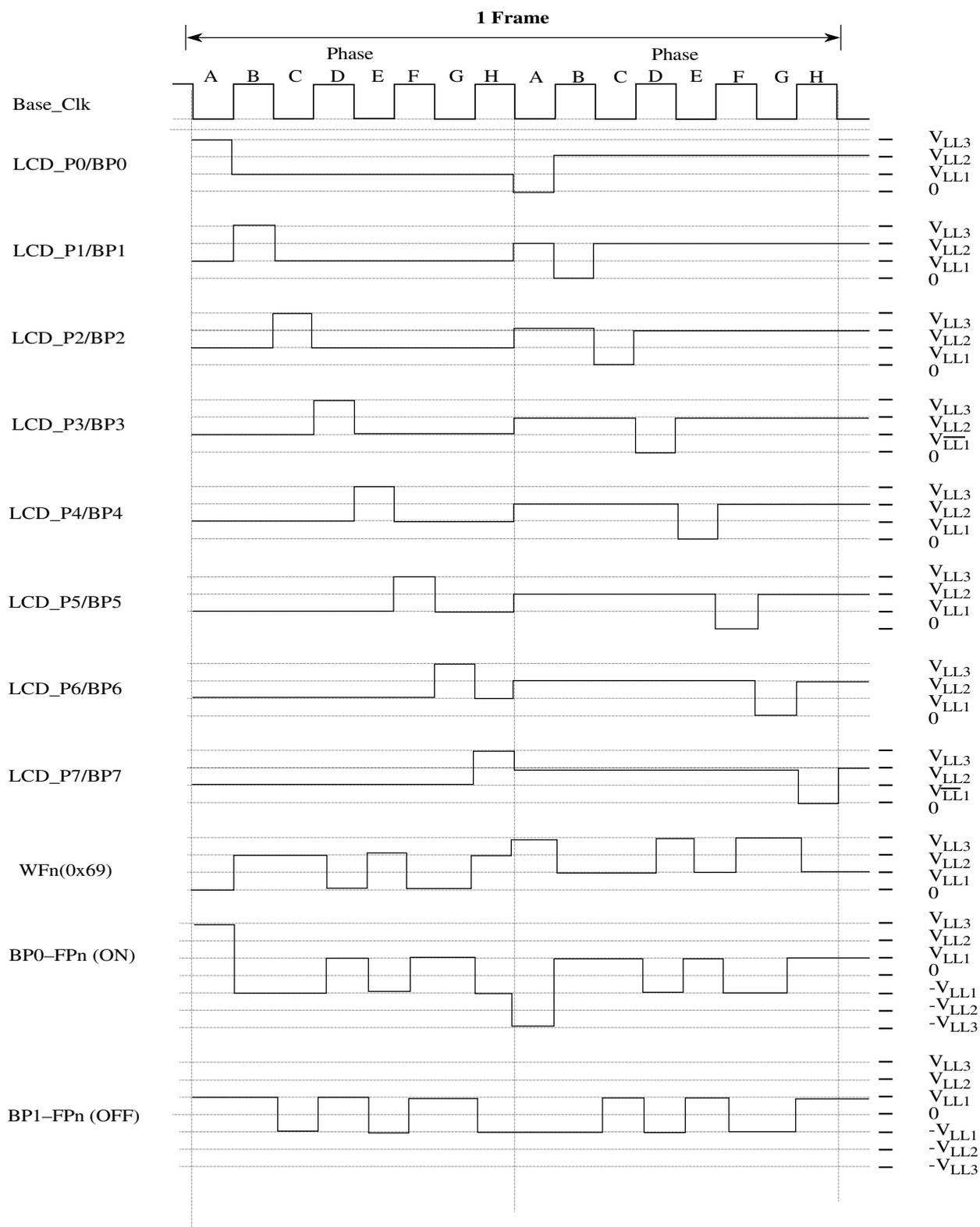
Figure 52-31. 1/8 Duty and 1/3 bias (low-power waveform)
