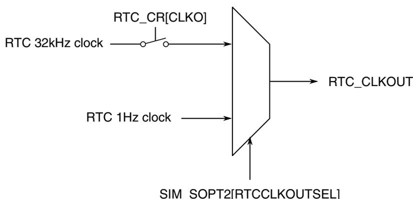
**Figure 3-46. RTC\_CLKOUT generation**
