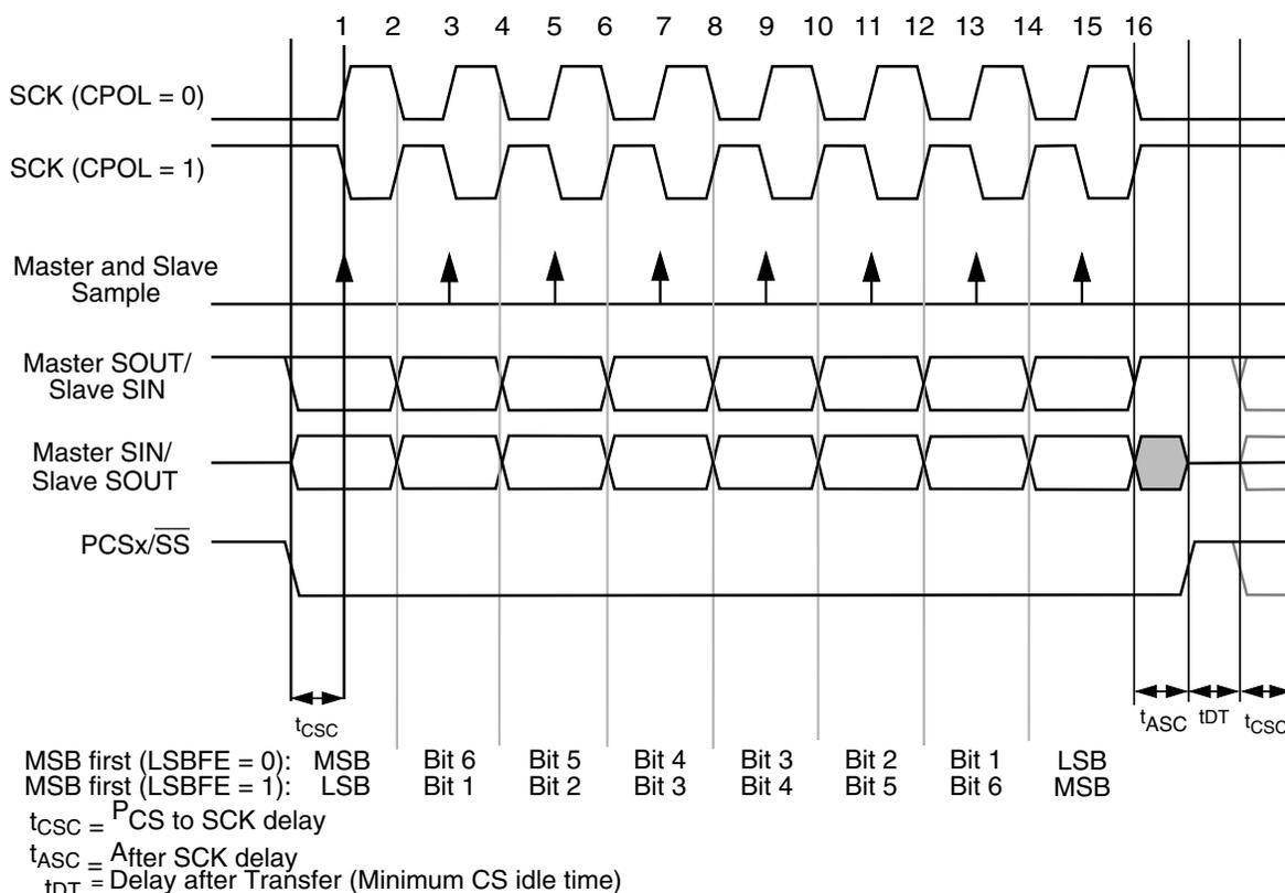
**Figure 46-71. Module transfer timing diagram (MTFE=0, CPHA=0, FMSZ=8)**
