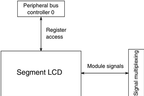
Figure 3-60. SLCD configuration
