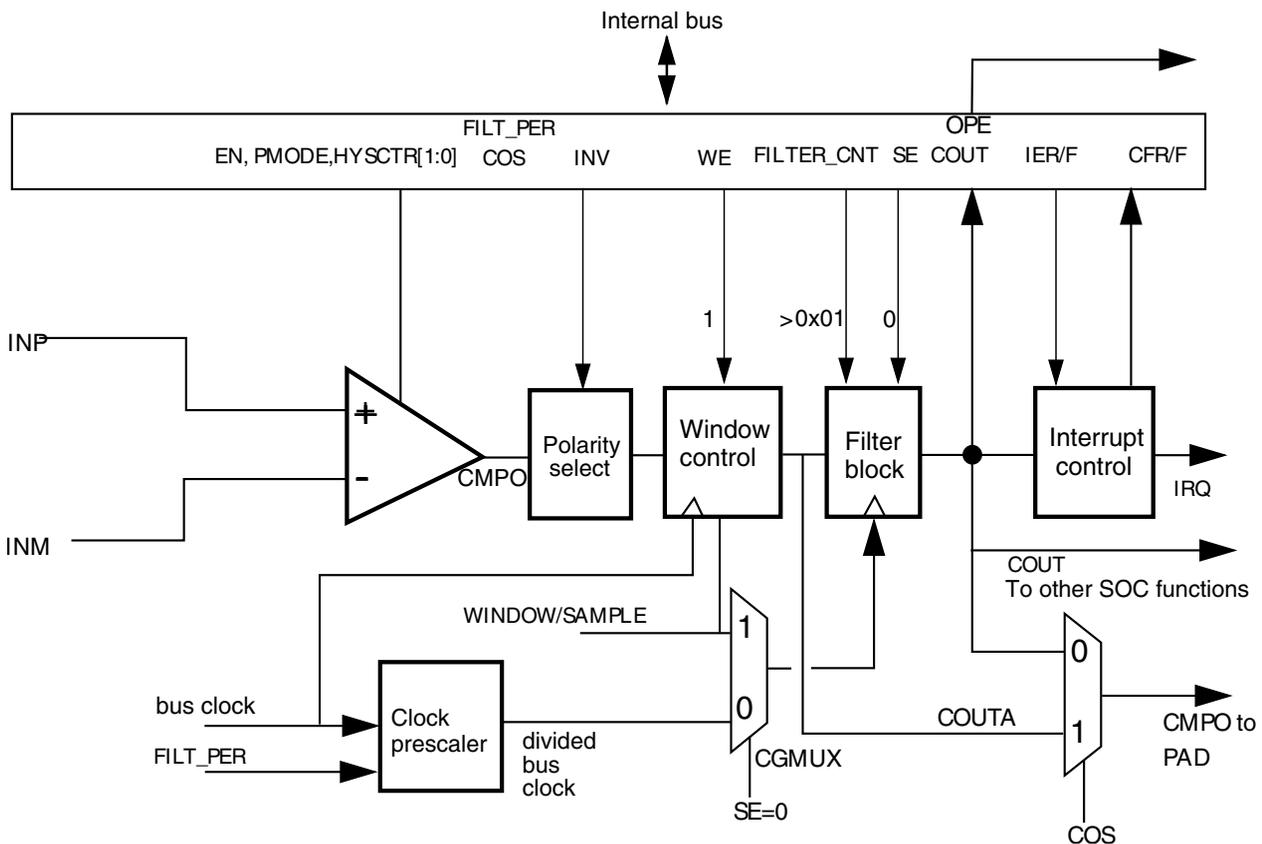
Figure 32-35. Windowed/Filtered mode
