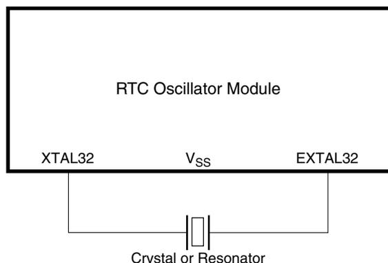
**Figure 26-2. Crystal Connections**
