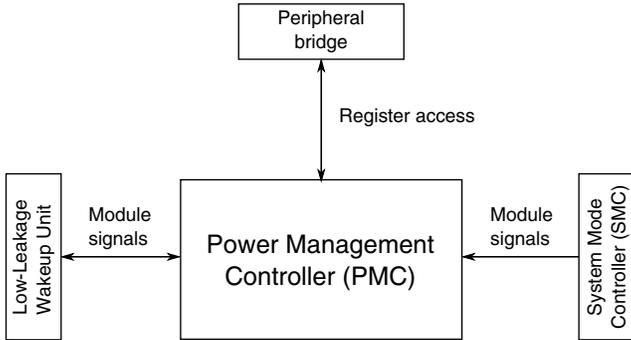
**Figure 3-7. PMC configuration**
