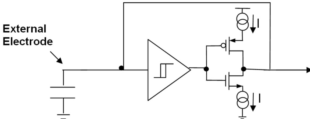
**Figure 51-33. TSI electrode oscillator circuit**
