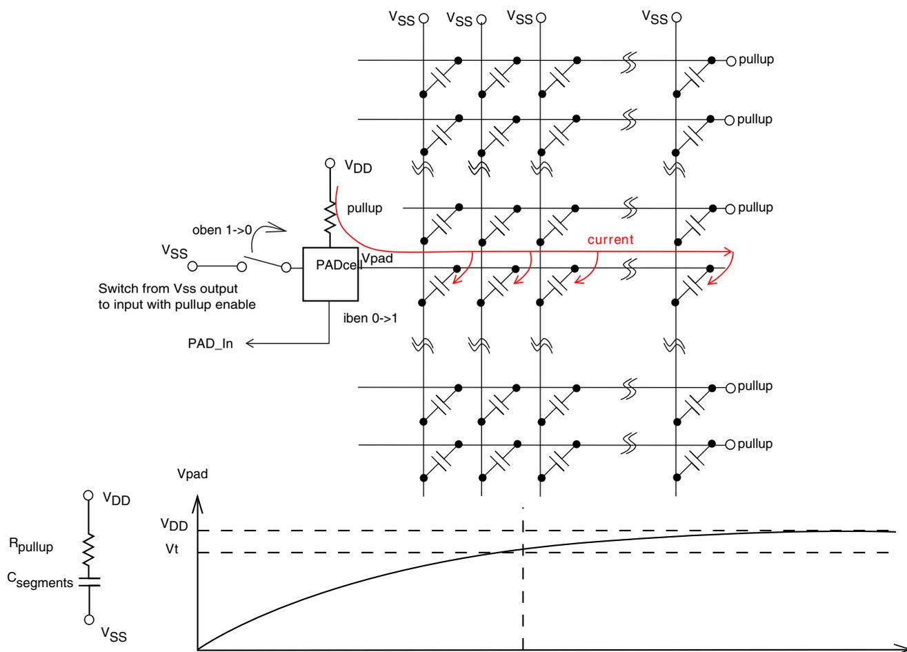
**Figure 52-33. Pullup fault detect in connection/segment normal case**
