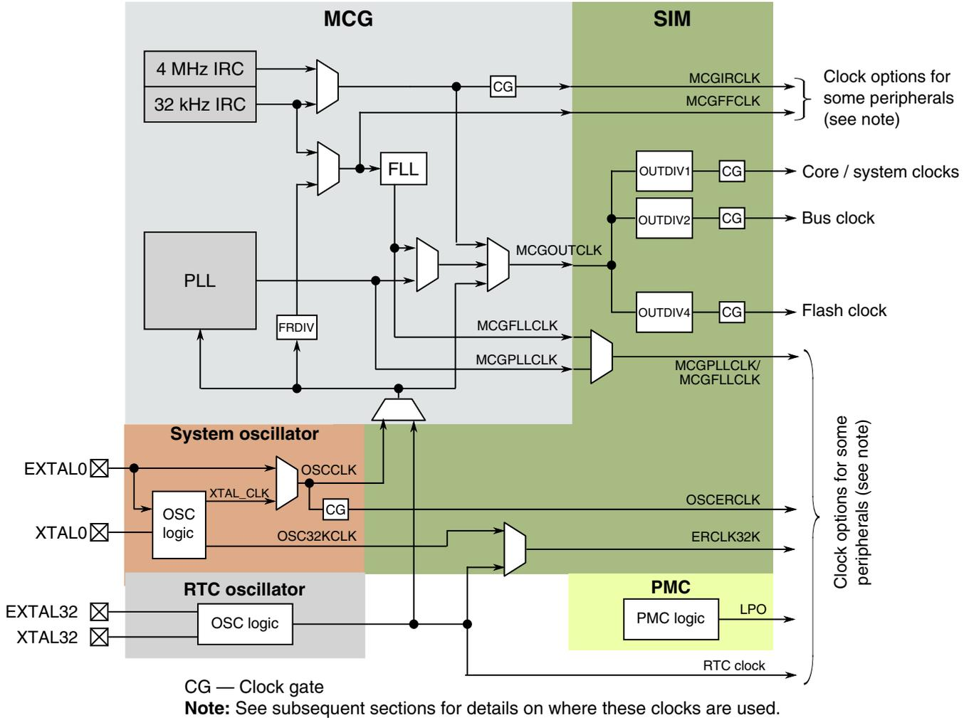
**Figure 5-1. Clocking diagram**
