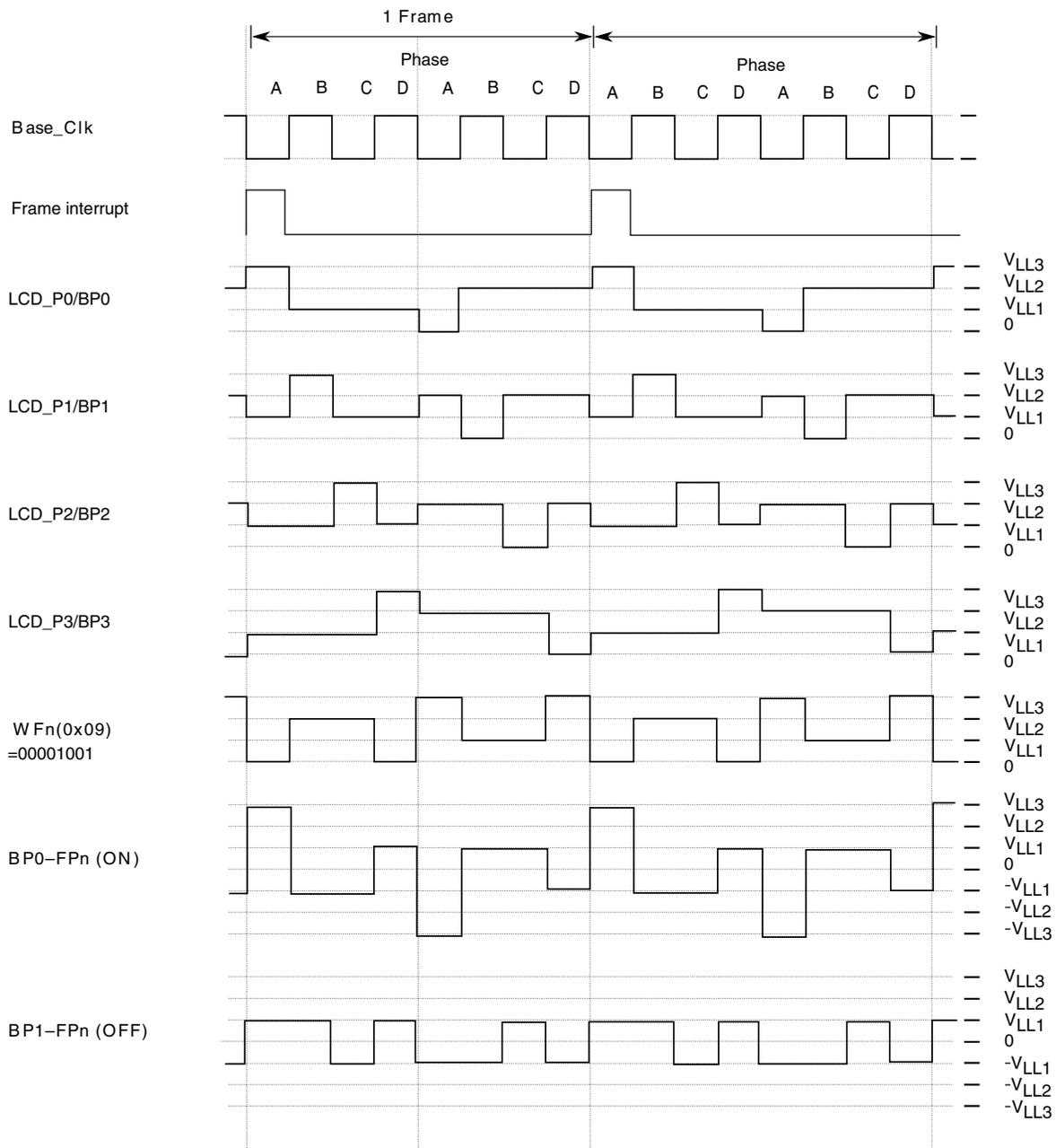
Figure 52-30. 1/4 duty and 1/3 bias (low-power waveform)
