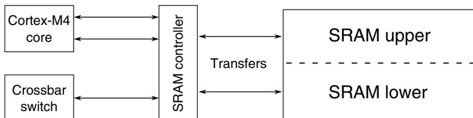
**Figure 3-21. SRAM configuration**
