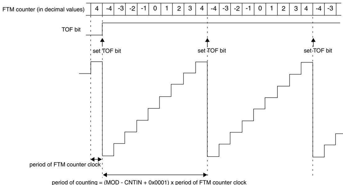
**Figure 38-168. Example of FTM up and signed counting**
