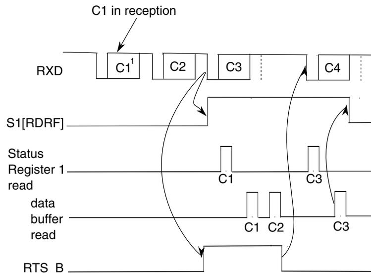
**Figure 48-57. Receiver hardware flow control timing diagram**
