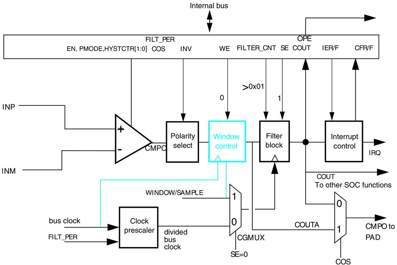
**Figure 32-31. Sampled, Filtered (# 4B): sampling point internally derived**
