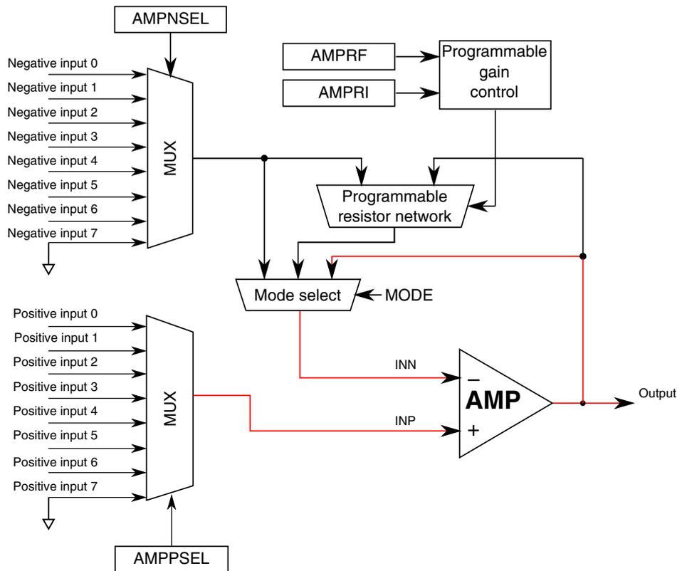
Figure 34-12. OPAMP block diagram in buffered configuration mode
