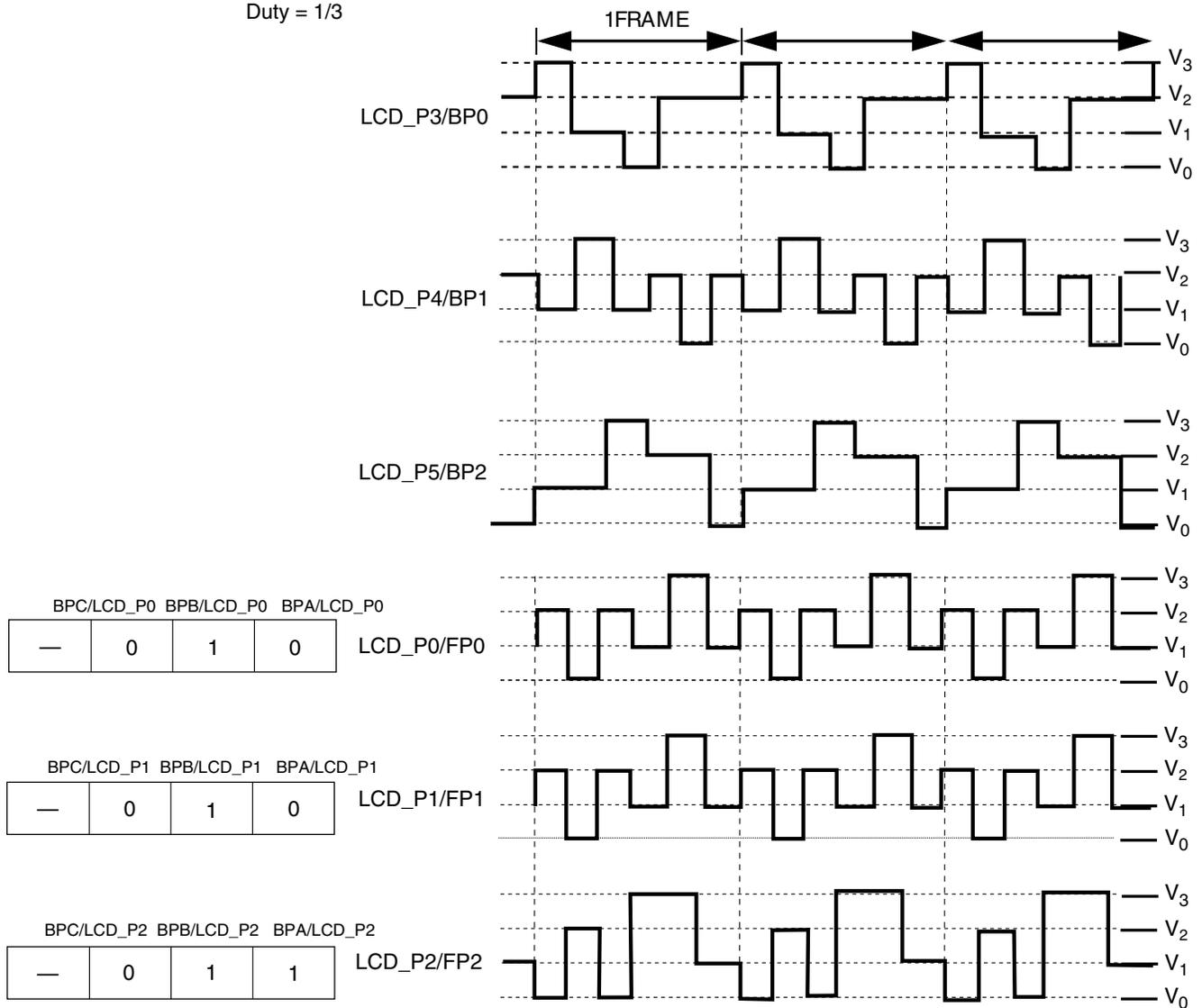
Figure 52-40. LCD waveforms
