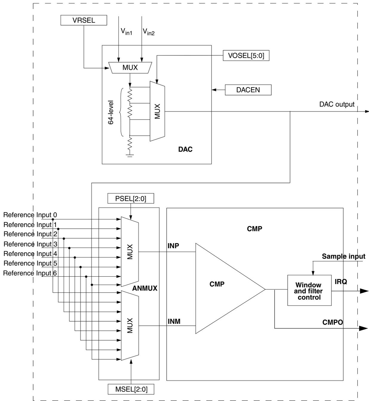
Figure 32-1. CMP, DAC and ANMUX block diagram
