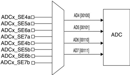
Figure 3-30. ADCx\_SEn channels a and b selection
