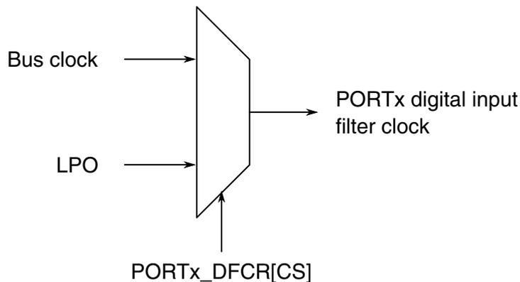
**Figure 5-4. PORT<sub>x</sub> digital input filter clock generation**
