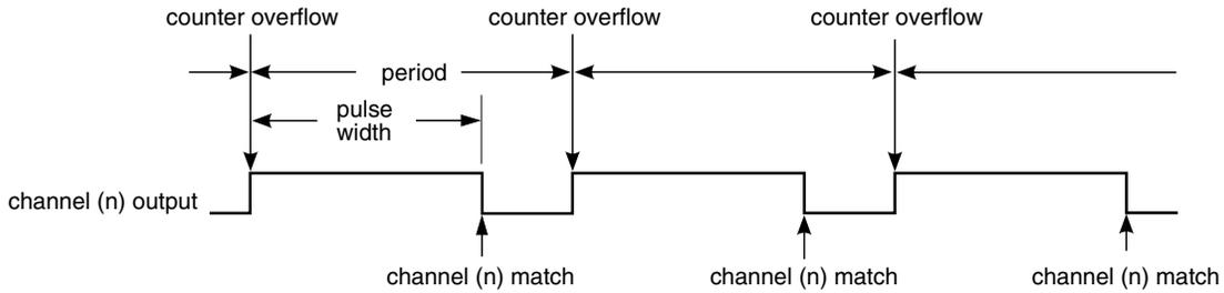
**Figure 38-181. EPWM period and pulse width with ELSnB:ELSnA = 1:0**
