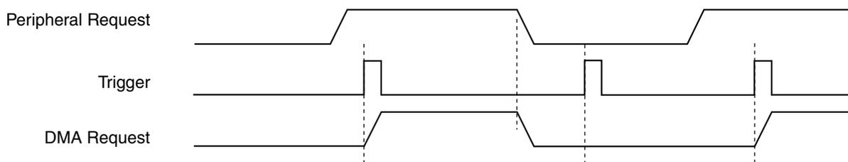
**Figure 20-21. DMA MUX channel triggering: ignored trigger**
