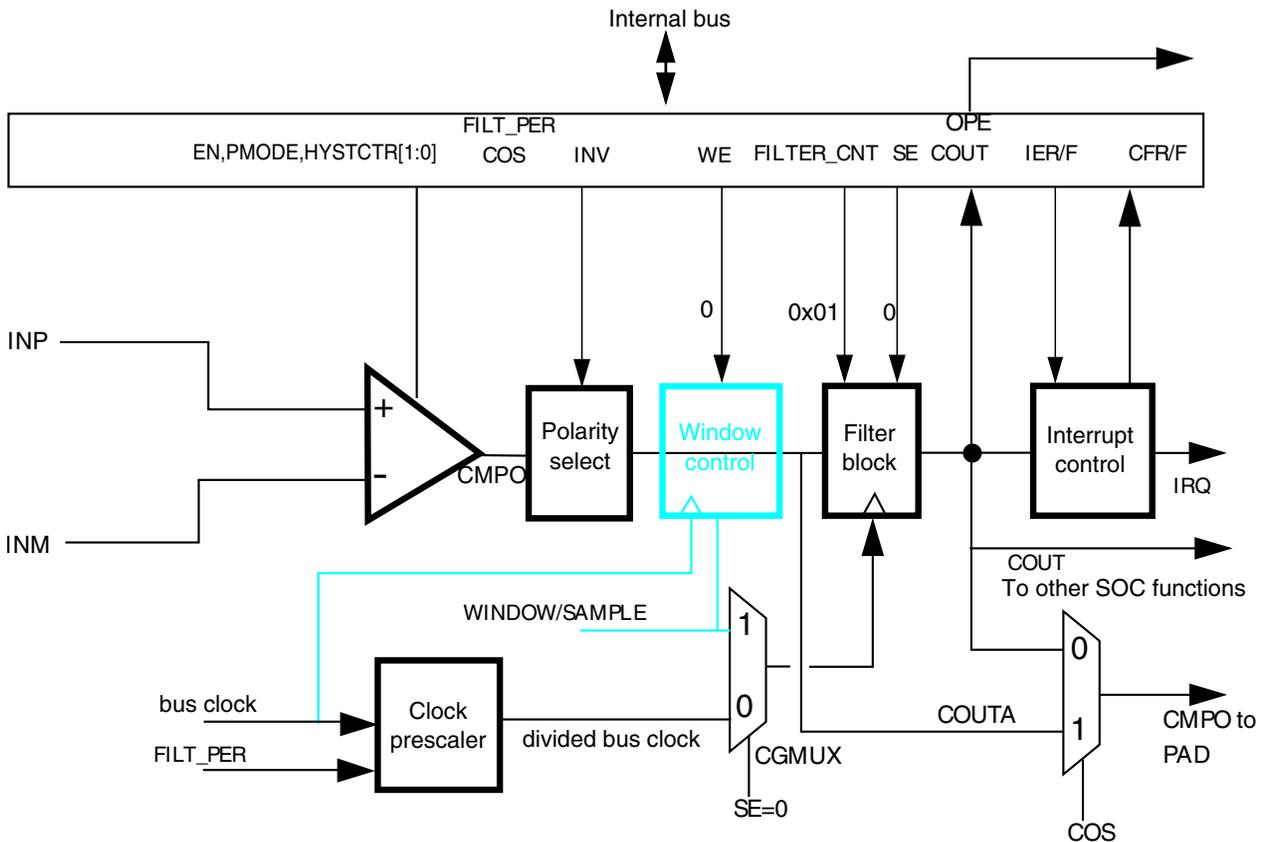
Figure 32-29. Sampled, Non-Filtered (# 3B): sampling interval internally derived
