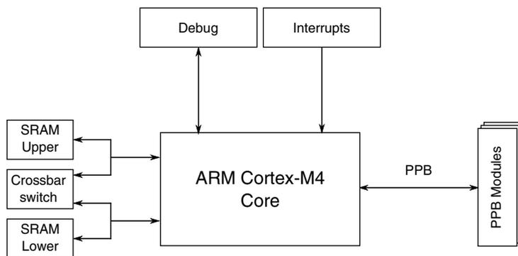
**Figure 3-1. Core configuration**
