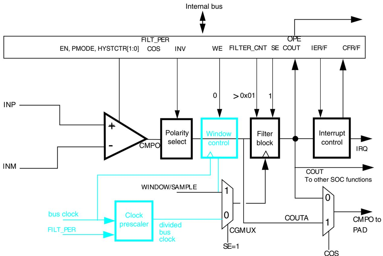
Figure 32-30. Sampled, Filtered (# 4A): sampling point externally driven
