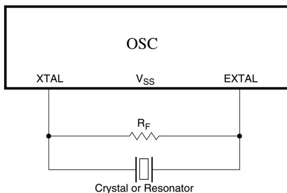
**Figure 25-3. Crystal/Ceramic Resonator Connections - Connection 2**
