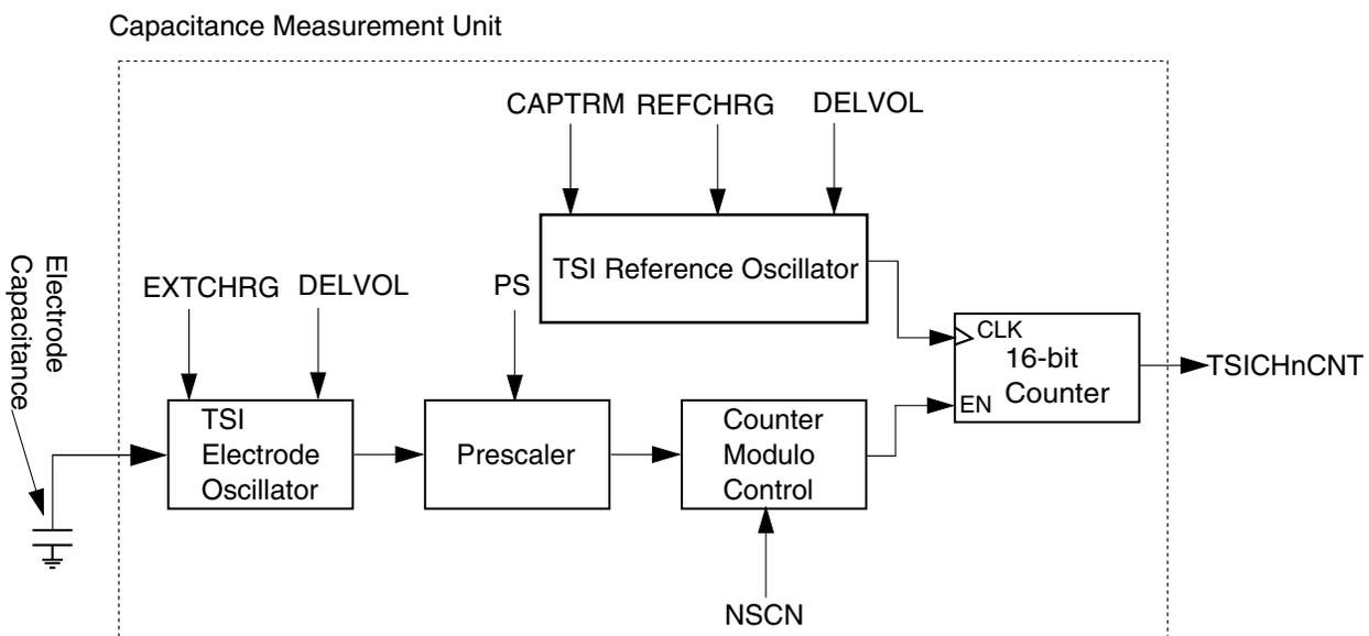
**Figure 51-2. TSI capacitance measurement unit block diagram**
