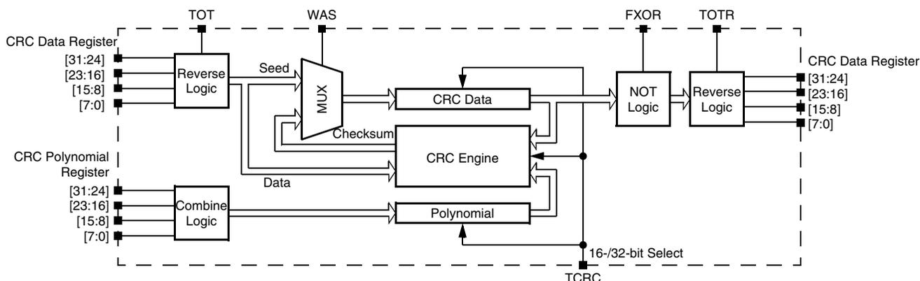
Figure 30-1. Programmable cyclic redundancy check (CRC) block diagram
