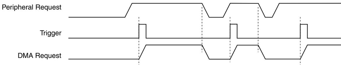
**Figure 20-20. DMA MUX channel triggering: normal operation**
