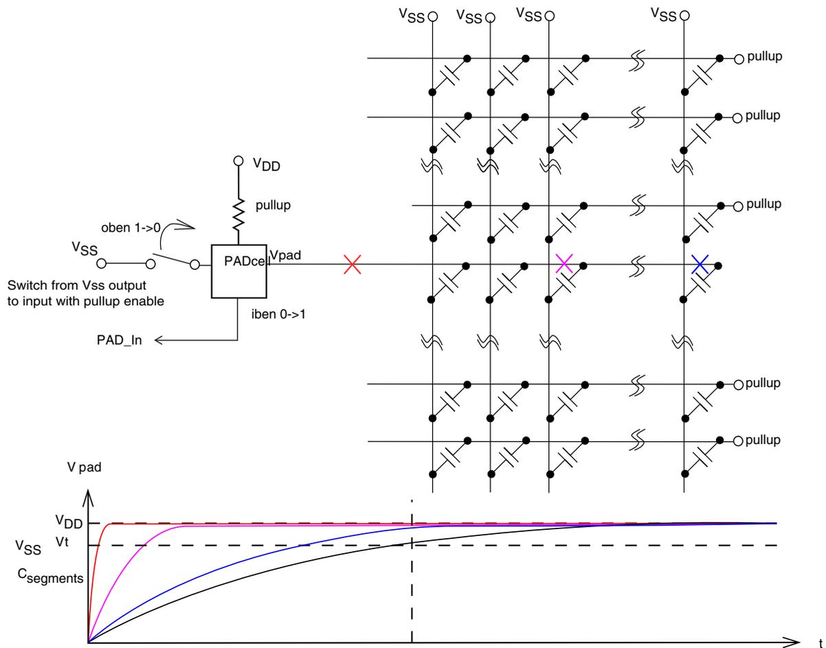
If there's any open case in connection or panel, the  $C_{segments}$  will become smaller, which makes the pullup time shorter.
