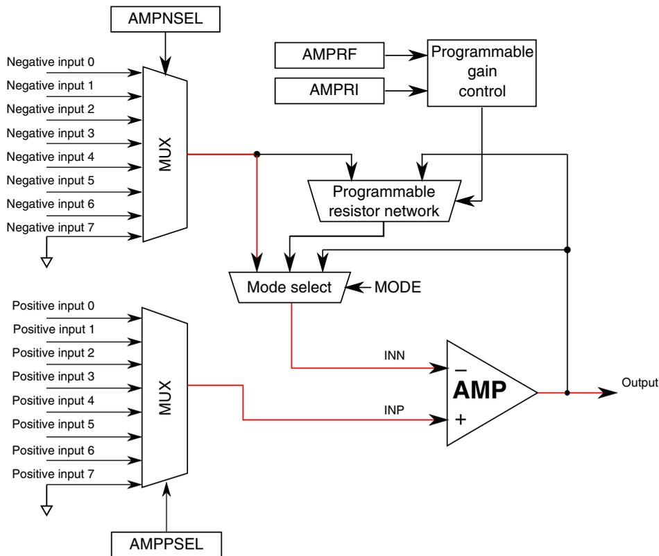
**Figure 34-11. OPAMP block diagram in general-purpose mode**
