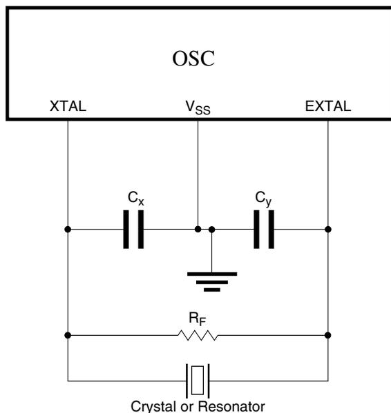
**Figure 25-4. Crystal/Ceramic Resonator Connections - Connection 3**
