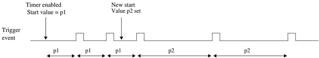
**Figure 39-25. Dynamically setting a new load value**
