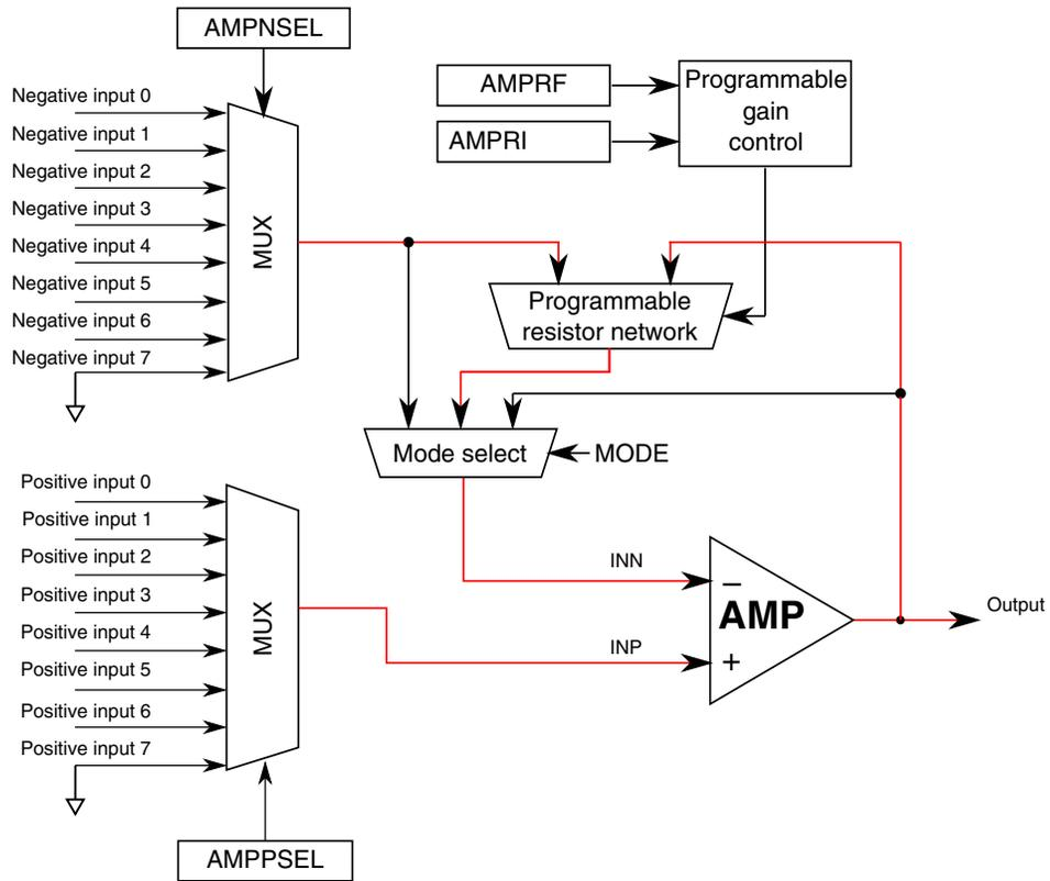
Figure 34-13. OPAMP block diagram in programmable gain mode
