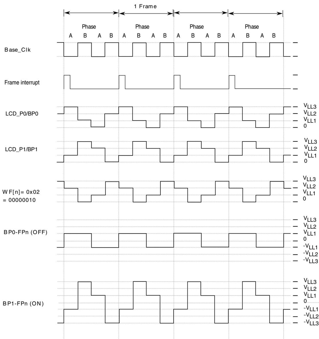
Figure 52-29. 1/2 duty and 1/3 bias (low-power waveform)
