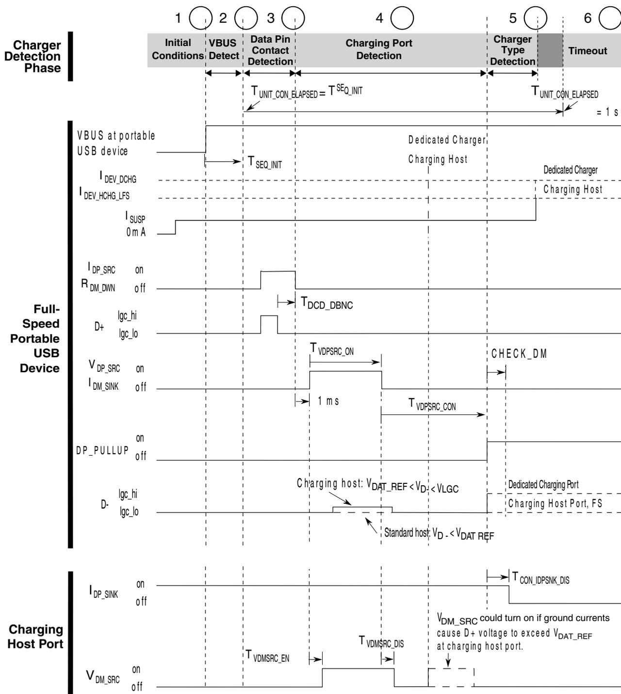
**Figure 44-9. Full speed charger detection timing**
