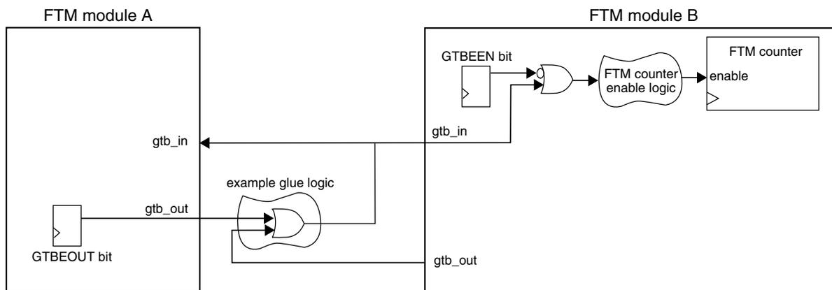
**Figure 38-258. Global time base (GTB) block diagram**
