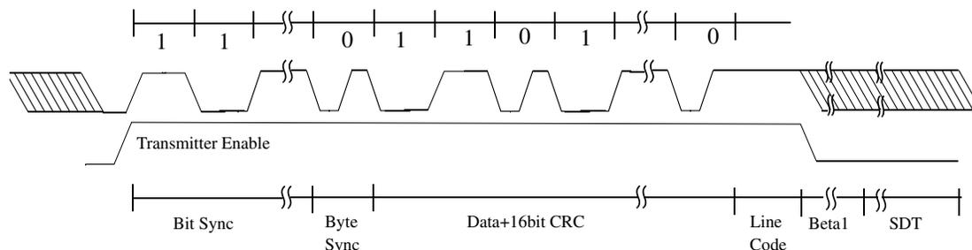
**Figure 48-49. Frame format with differential manchester encoding**
