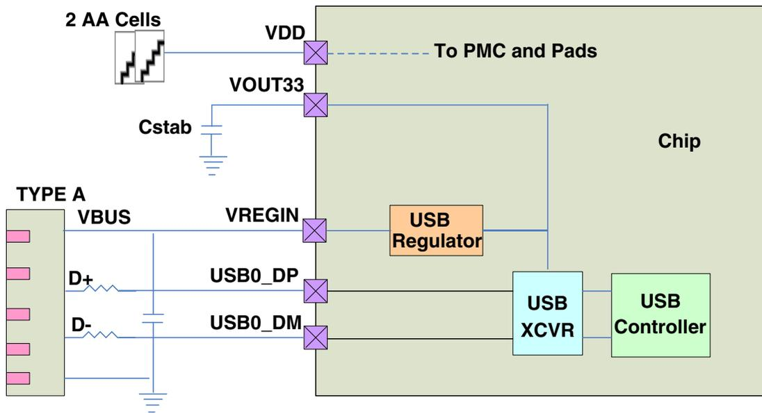
Figure 3-48. USB regulator AA cell usecase
