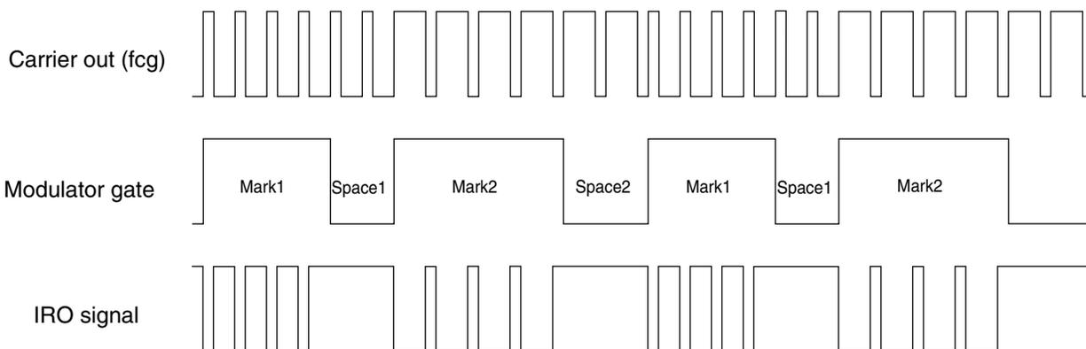
**Figure 41-18. Example: CMT output in FSK mode**
