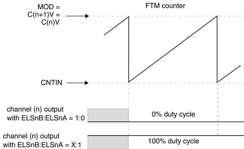
**Figure 38-196. Channel (n) output if (C(n)V = C(n+1)V = MOD)**
