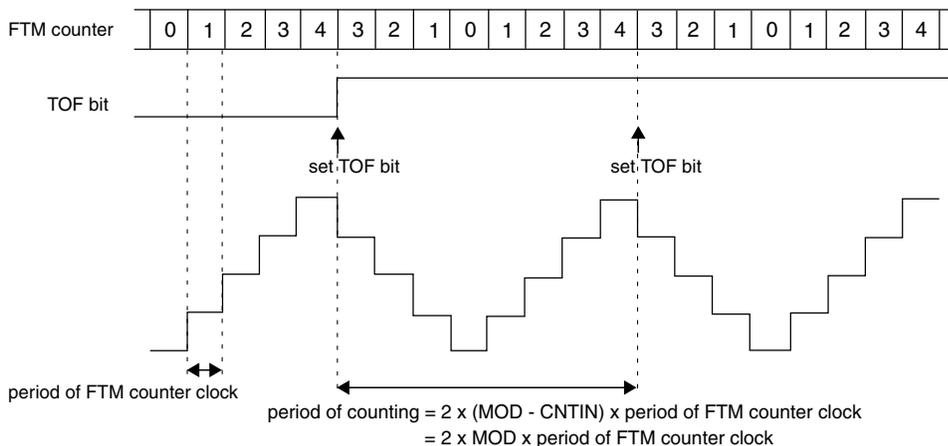
**Figure 38-171. Example of up-down counting when CNTIN = 0x0000**
