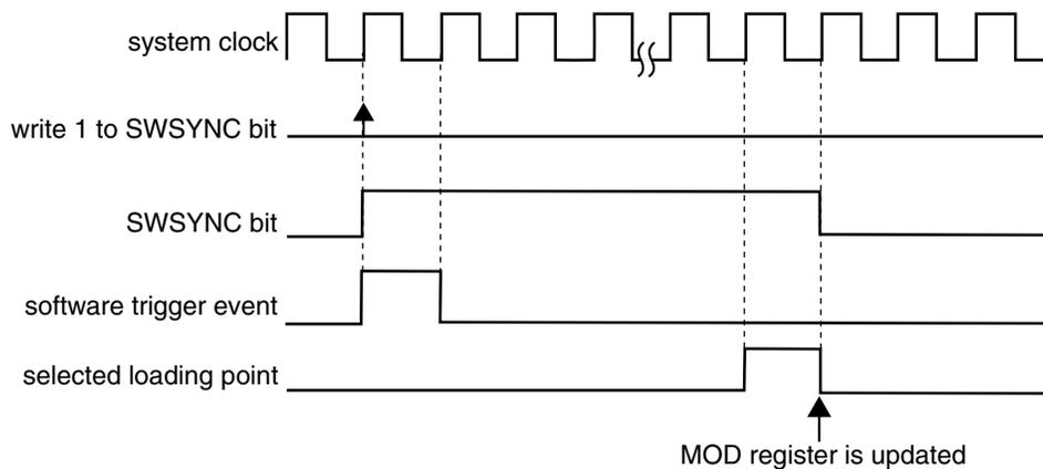
**Figure 38-213. MOD synchronization with (SYNCMODE = 0) and (PWMSYNC = 1)**
