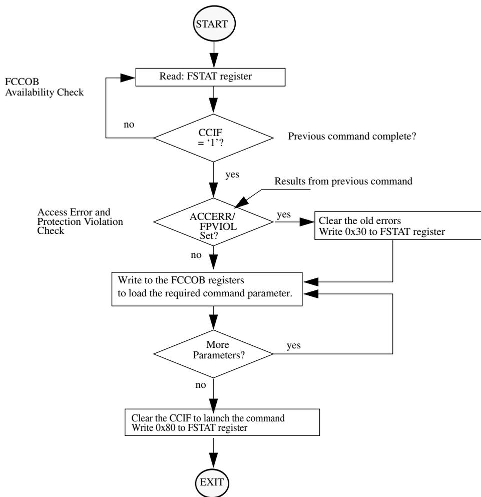
Figure 28-32. Generic Flash Command Write Sequence Flowchart
