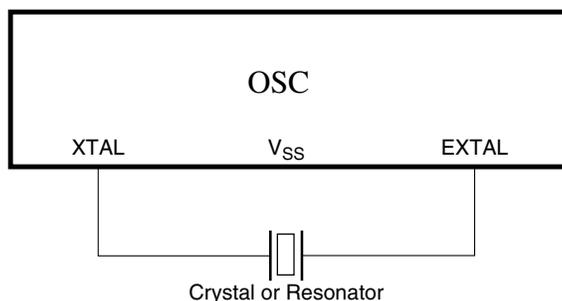
**Figure 25-2. Crystal/Ceramic Resonator Connections - Connection 1**
