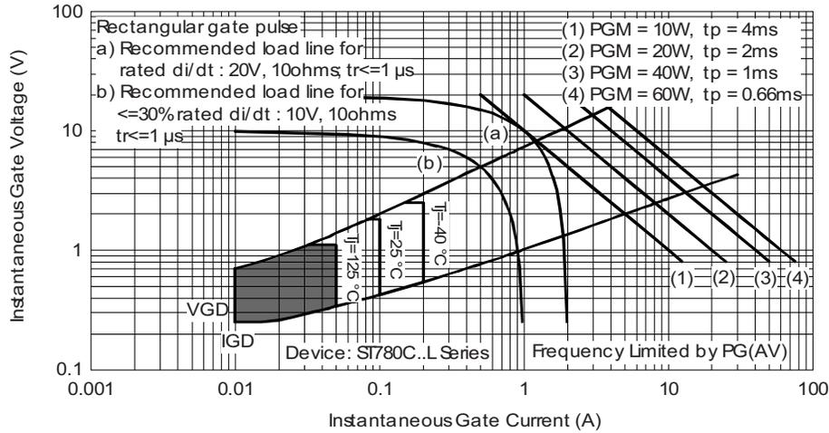
Fig. 11 - Gate Characteristics
