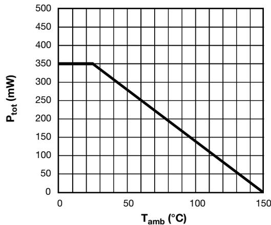
Fig. 1 - P<sub>tot</sub> - Admissible Power Dissipation vs. Ambient Temperature
