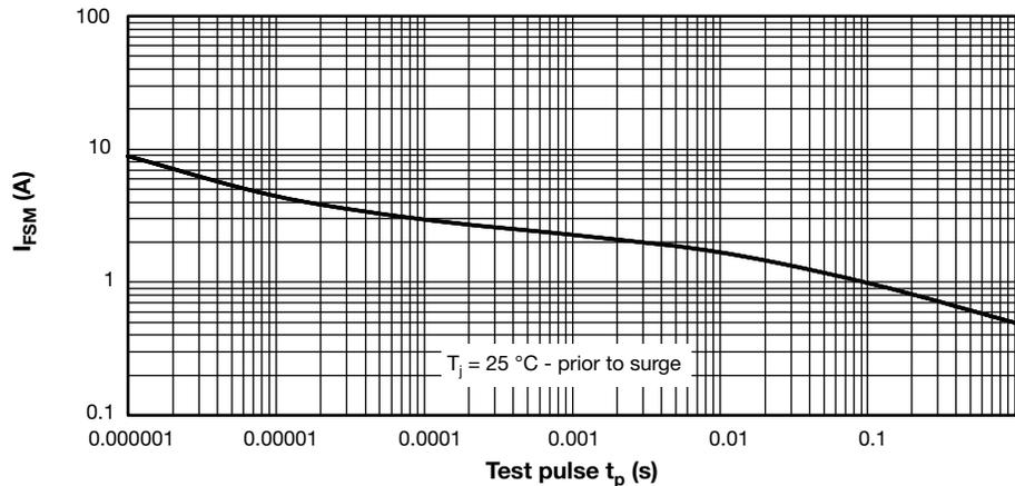
Fig. 2 - I<sub>FSM</sub> - Non-Repetitive Peak Forward Current vs. Pulse Duration - Maximum Admissible Values of Square Pulses
