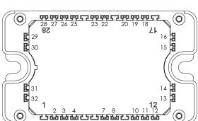
All multiple inputs and outputs must be shorted together Example: 13/14; 29/30; 22/23 ...
