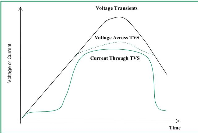
**Figure 2 - Peak Pulse Power Rating Curve**
