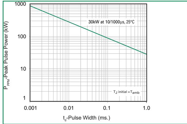
**Figure 3 - Peak Pulse Power Derating Curve**
