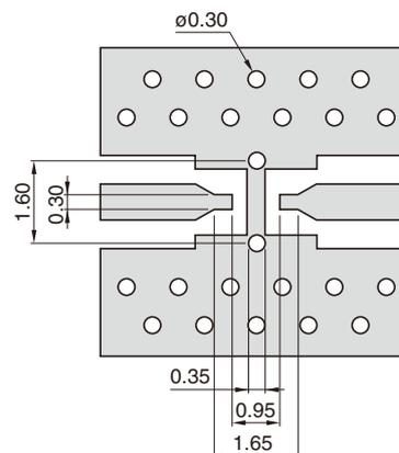
Line width should be designed to match 50Ω characteristic impedance, depending on PCB material and thickness.
