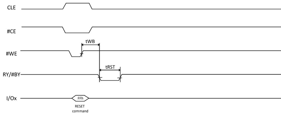
Figure 9-17 Reset Operation
