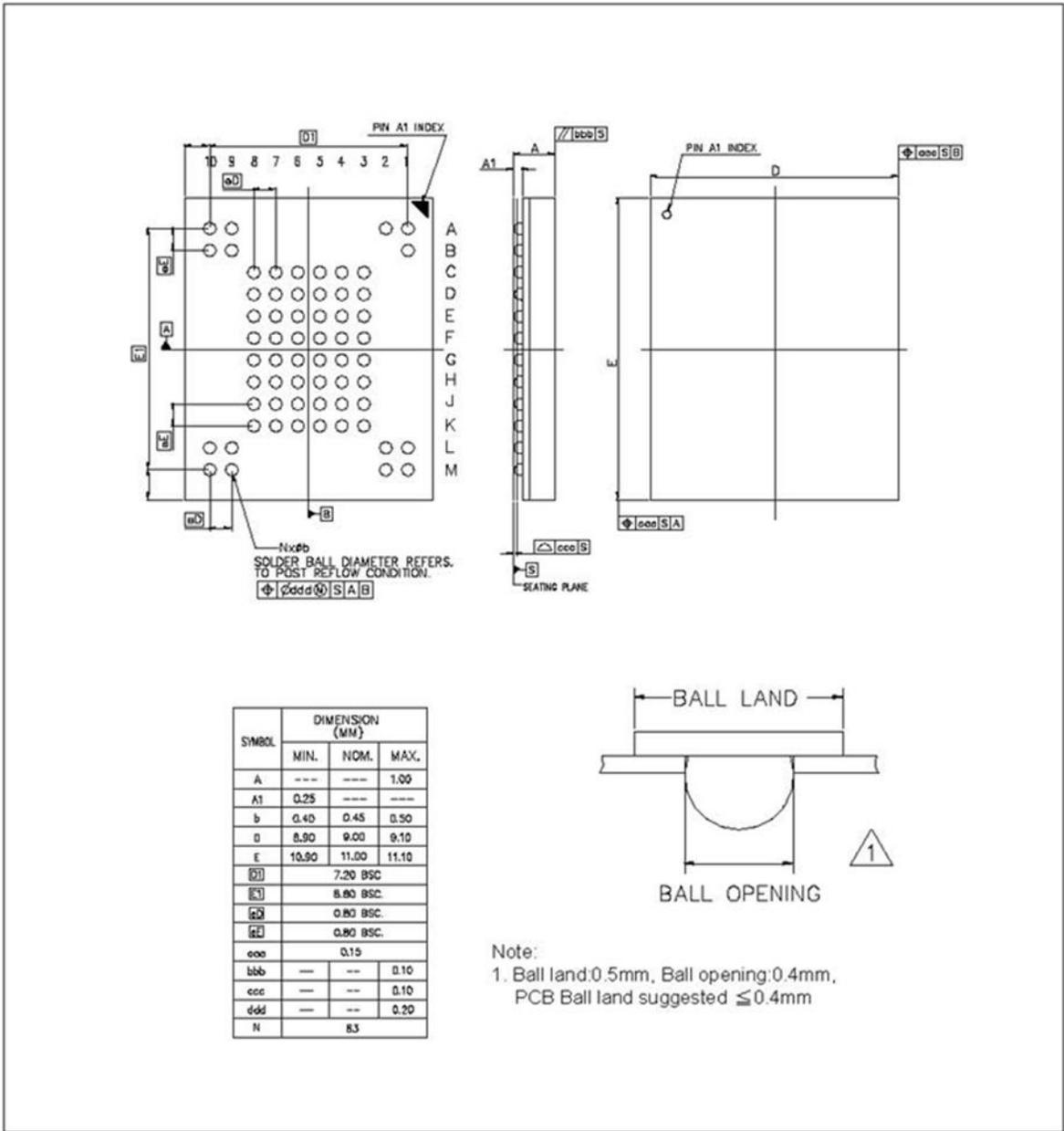
Figure 13-3 Fine-Pitch Ball Grid Array 63-Ball (9x11mm)
