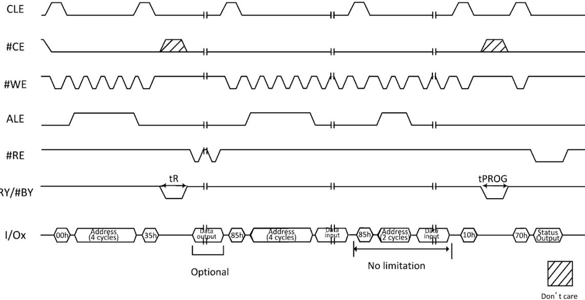
Figure 9-15 Copy Back Operation with Random Data Input
