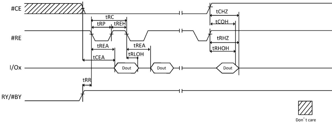
Figure 11-5 Serial Access Cycle after Read (EDO)
