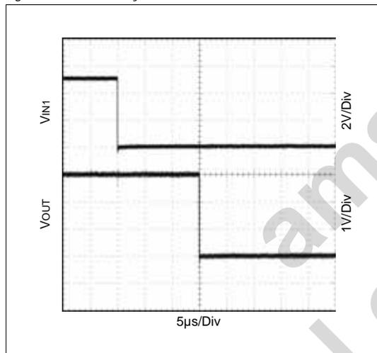
Figure 9. Reset Active Timeout Period; VIN2 = 3.0V
