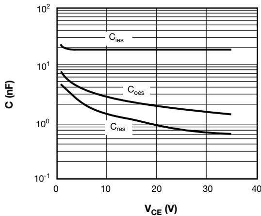
Fig. 6 - Typical Capacitance vs. Collector to Emitter Voltage
