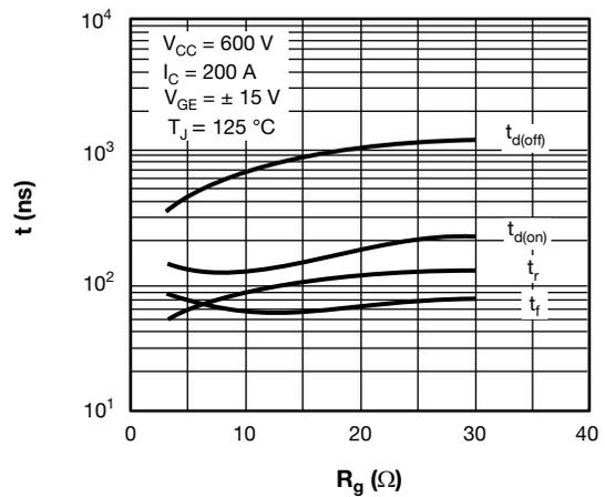
Fig. 8 - Typical Switching Times vs. Gate Resistance  $R_g$
