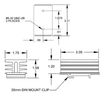
DIMENSIONS: inches TOLERANCES: ±0.02 inches MATERIAL: AISI 6063-T5 Aluminum
