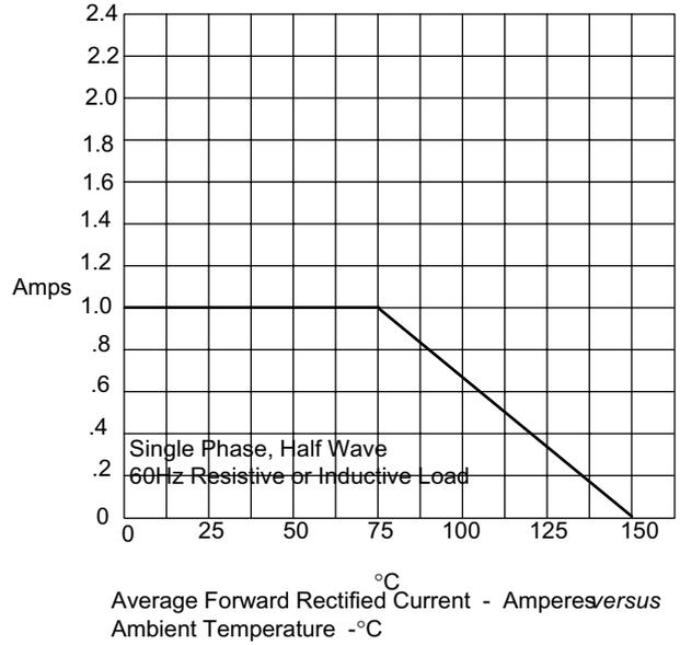
Average Forward Rectified Current - Amperes versus
