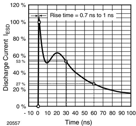
Fig. 1 - ESD Discharge Current Wave Form
