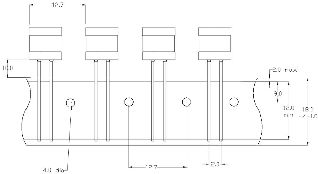
Supplied on cut tape roll packaging, 800 parts per roll.
