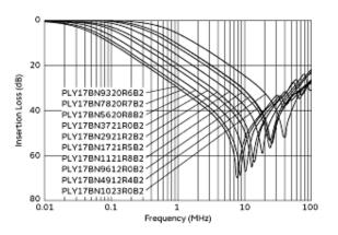
Common Mode Insertion Loss-Frequency Characteristics
