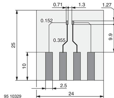
Fig. 4 - Board for  $R_{thJA}$  definition (in mm)
