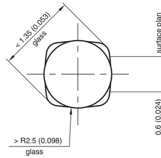
\* The gap between plug and glass can be either on cathode or anode side
