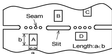
Products (A,B,C,D) shall be located carefully so that products are not subject to the mechanical stress due to warping the board. Because they may be subjected the mechanical stress in order of  $A > C > B \cong D$ .
