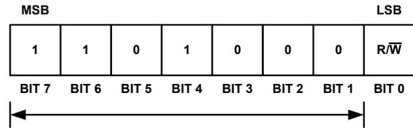
FIGURE 5. I<sup>2</sup>C SLAVE ADDRESS
