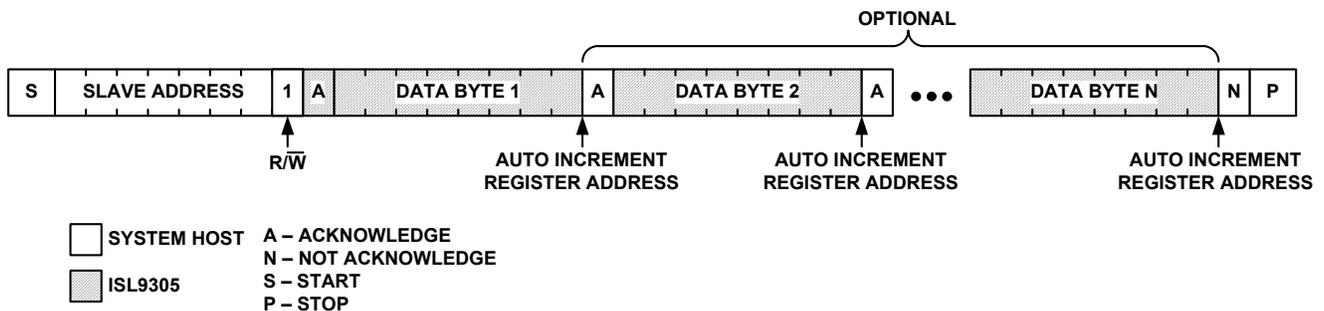
FIGURE 8. I<sup>2</sup>C READ NOT SPECIFYING REGISTER ADDRESS
