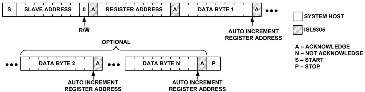
FIGURE 6. I<sup>2</sup>C WRITE
