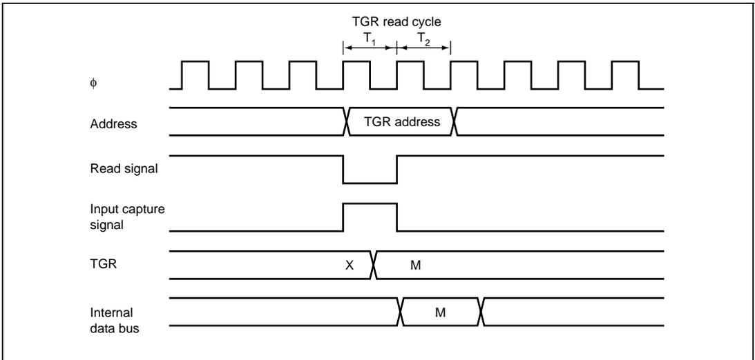
**Figure 12.51 Contention between TGR Read and Input Capture**
