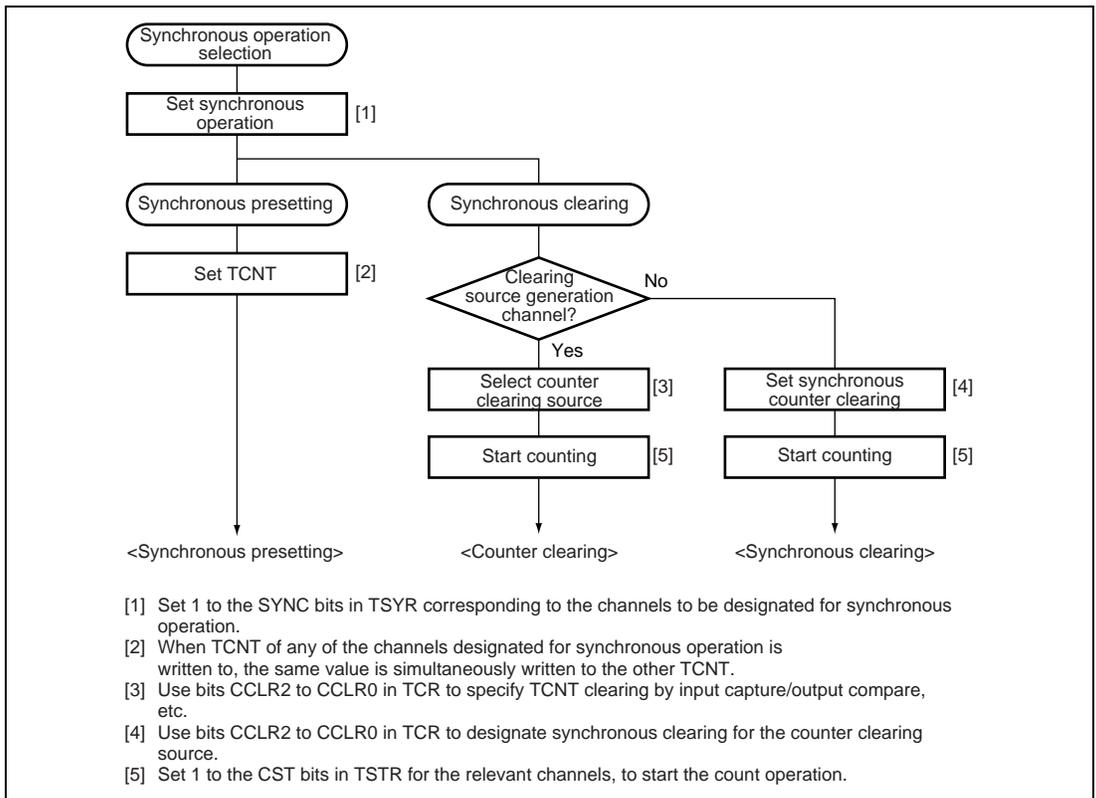
**Figure 12.14 Example of Synchronous Operation Setting Procedure**
