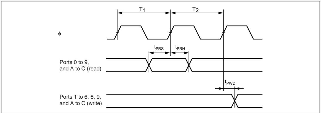
Figure 24.14 I/O Port Input/Output Timing
