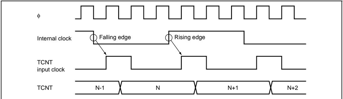
**Figure 12.33 Count Timing in Internal Clock Operation**
