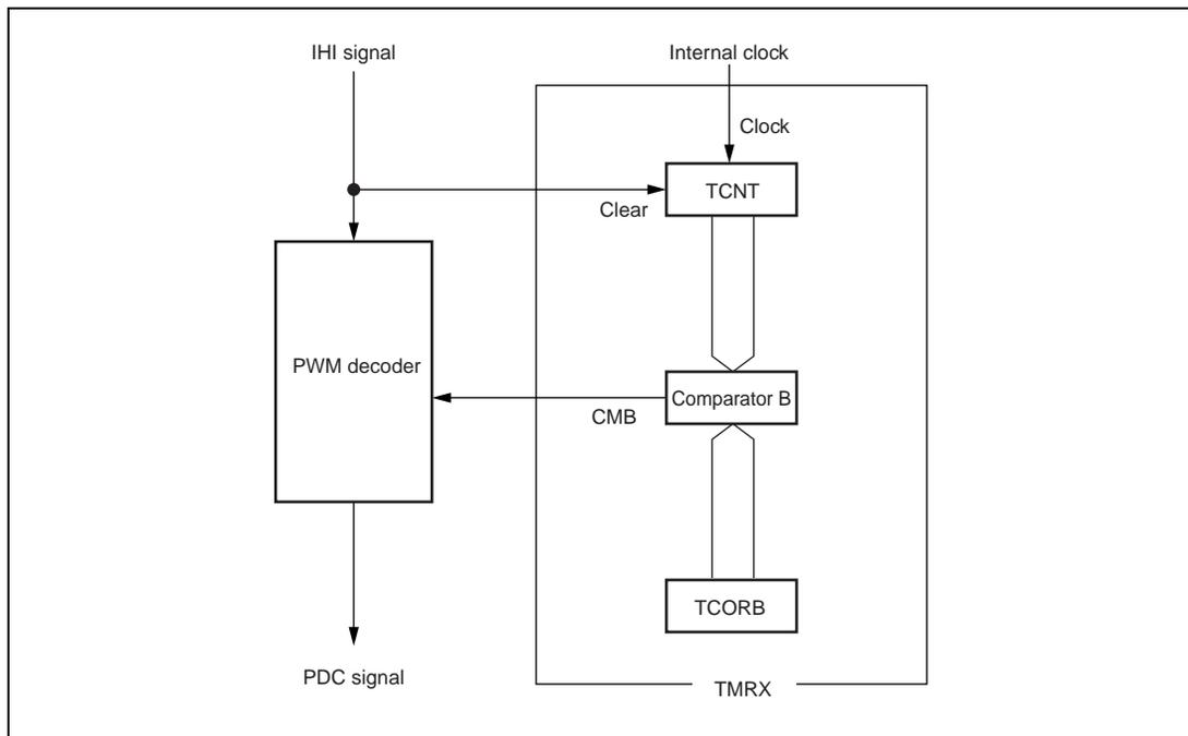
**Figure 13.3 Block Diagram for PWM Decoding**
