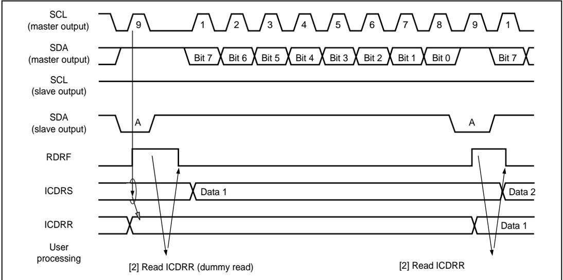
**Figure 17.11 Operation Timing in Slave Receive Mode (1)**
