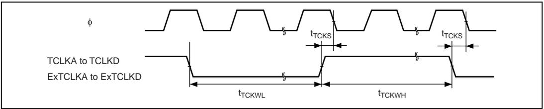
**Figure 24.18 TPU Clock Input Timing**
