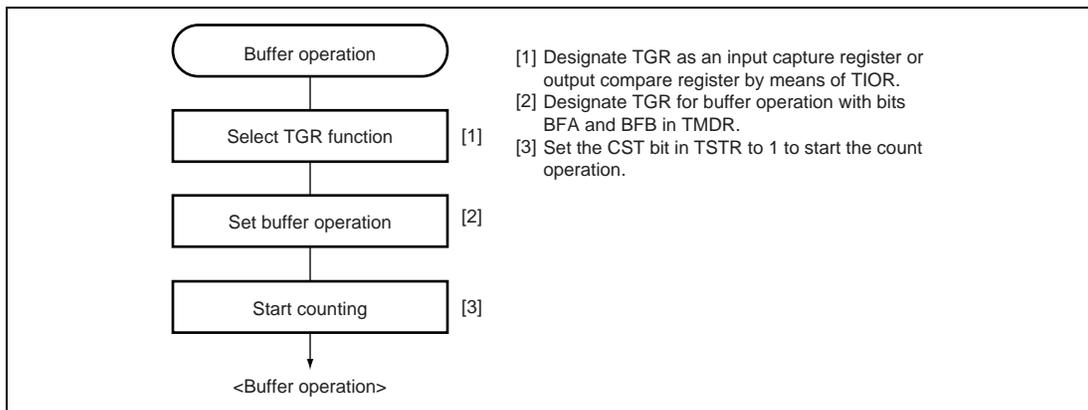
**Figure 12.18 Example of Buffer Operation Setting Procedure**
