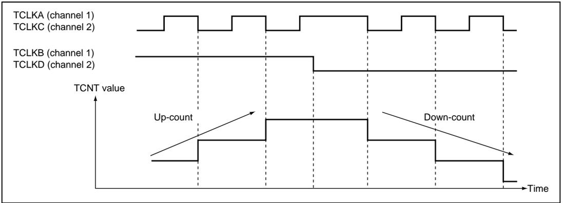
**Figure 12.30 Example of Phase Counting Mode 2 Operation**
