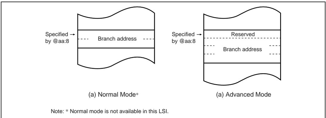
**Figure 2.12 Branch Address Specification in Memory Indirect Mode**
