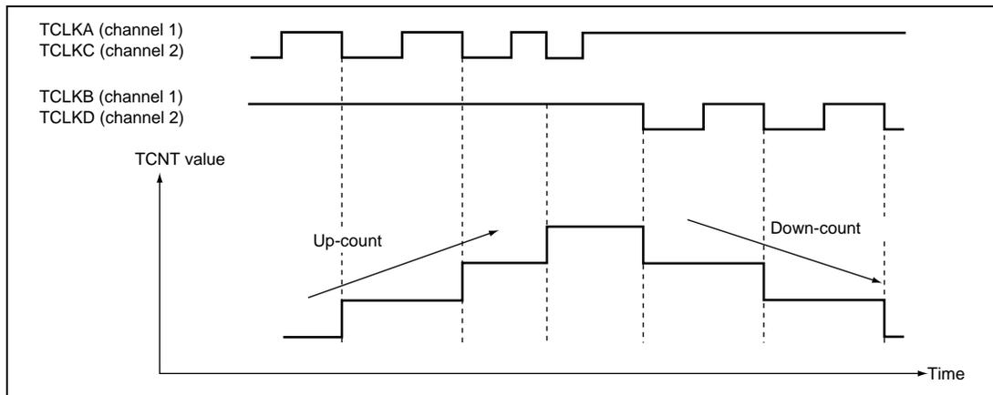
**Figure 12.31 Example of Phase Counting Mode 3 Operation**
