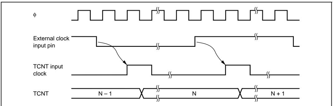
**Figure 11.5** Count Timing for External Clock Input
