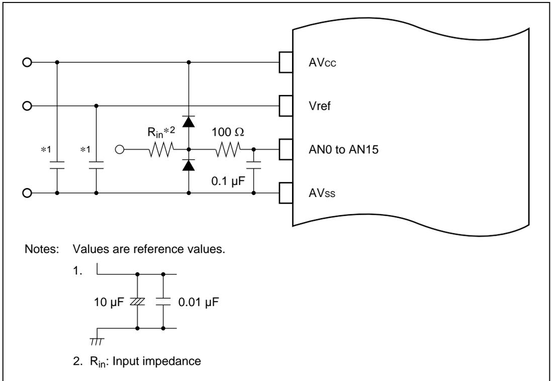
Figure 18.7 Example of Analog Input Protection Circuit
