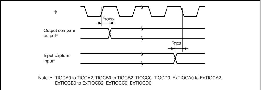
**Figure 24.17 TPU Input/Output Timing**
