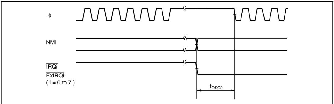
**Figure 24.5 Oscillation Stabilization Timing (Exiting Software Standby Mode)**
