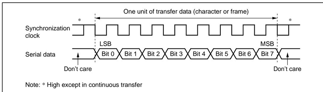
**Figure 16.14 Data Format in Clocked Synchronous Communication (LSB-First)**
