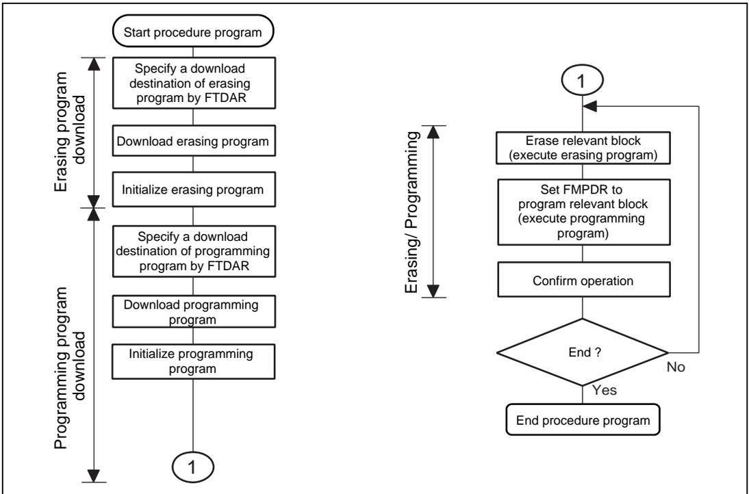
**Figure 20.13 Repeating Procedure of Erasing and Programming**
