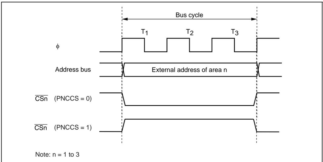
Figure 6.2  $\overline{CSn}$  Signal Output Polarity and Output Timing
