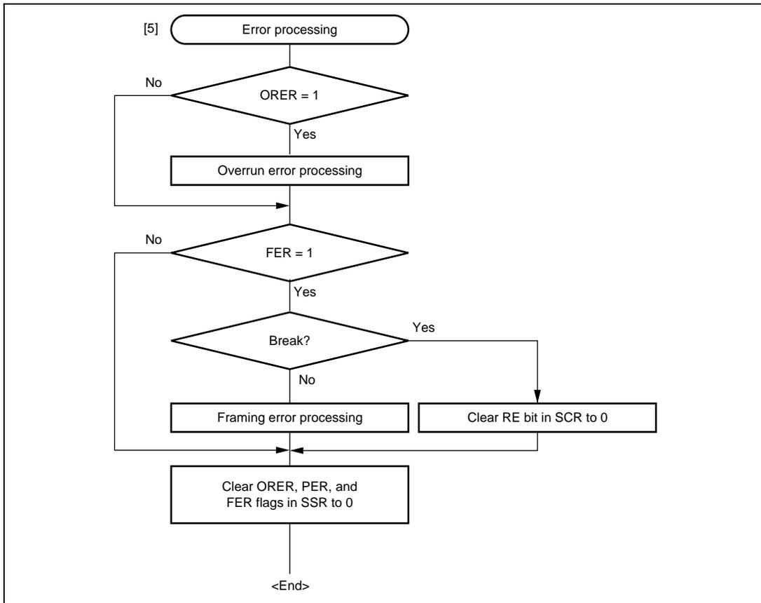
**Figure 16.13 Sample Multiprocessor Serial Reception Flowchart (2)**
