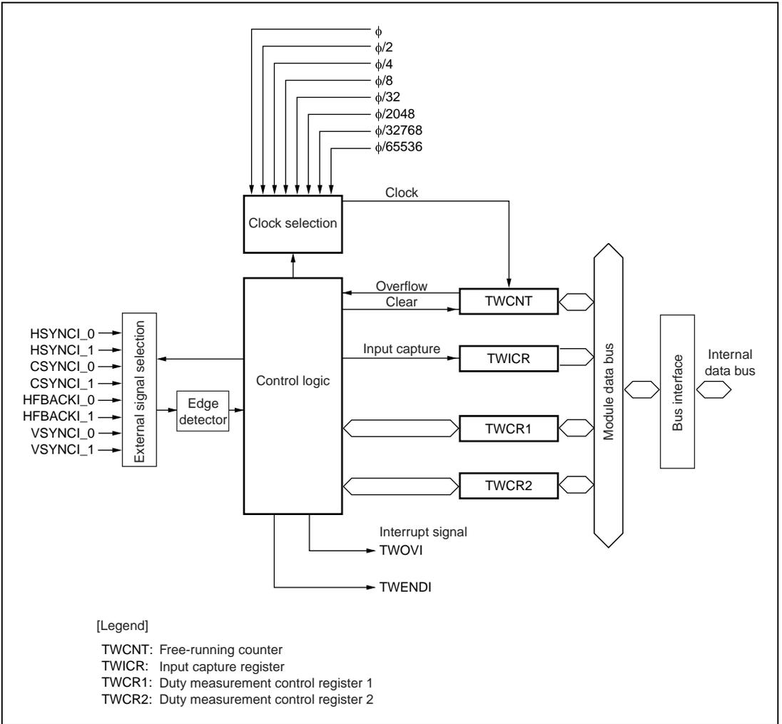
**Figure 14.1 Block Diagram of Duty Measurement Circuit**
