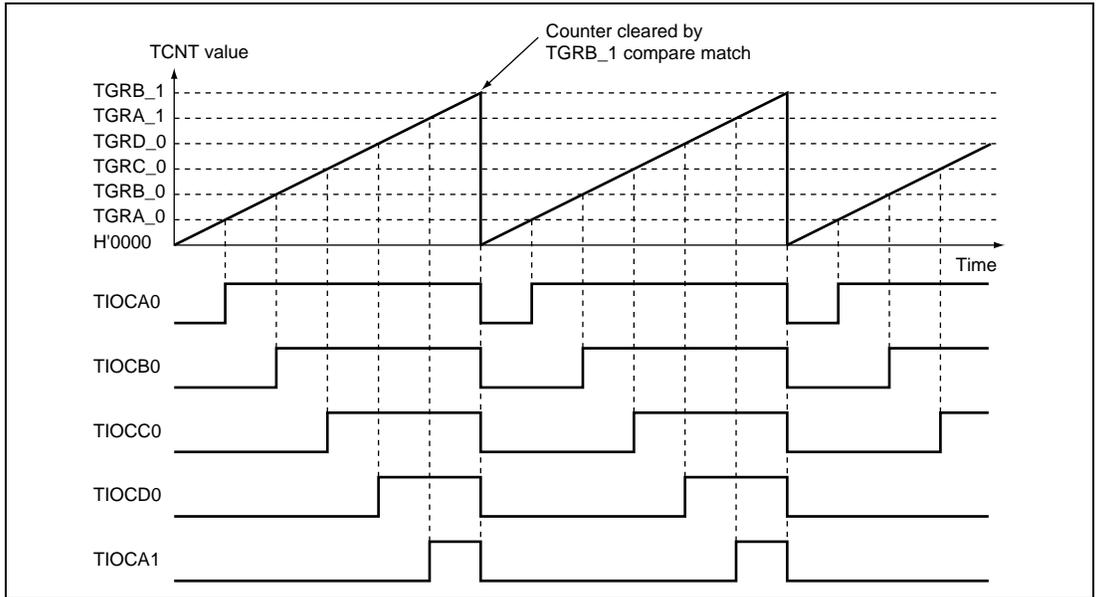
**Figure 12.26 Example of PWM Mode Operation (2)**
