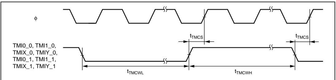
**Figure 24.20 8-Bit Timer Clock Input Timing**
