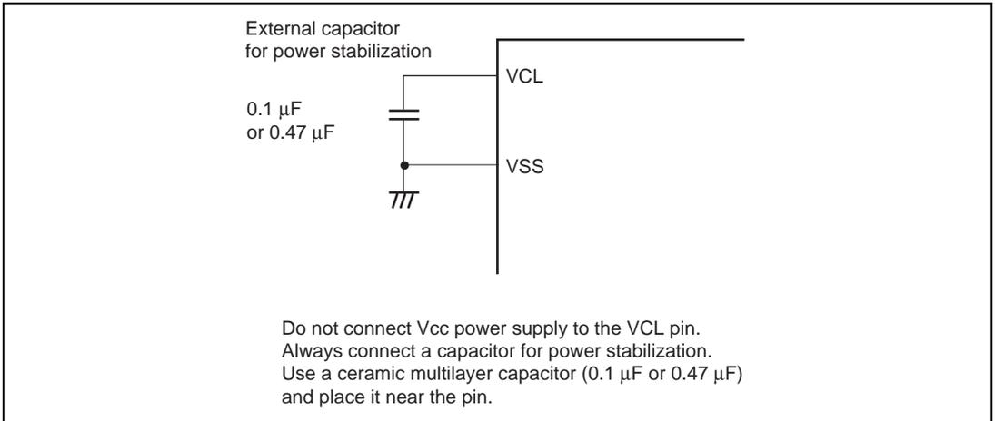
**Figure 24.27 Connection of VCL Capacitor**
