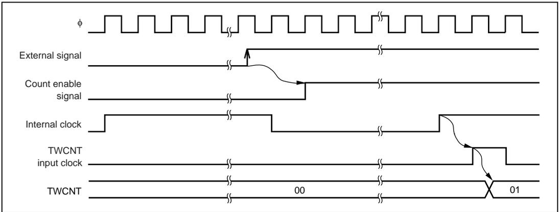
Figure 14.5 Count Start Timing for Duty Measurement
