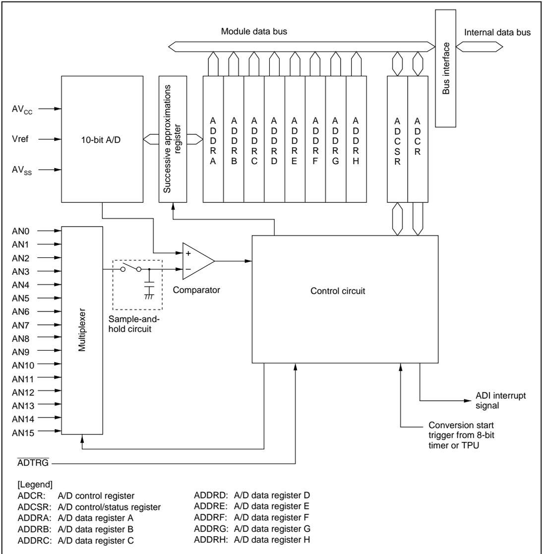
Figure 18.1 Block Diagram of A/D Converter
