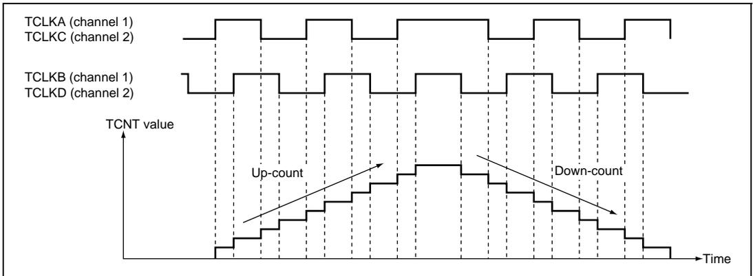
**Figure 12.29 Example of Phase Counting Mode 1 Operation**
