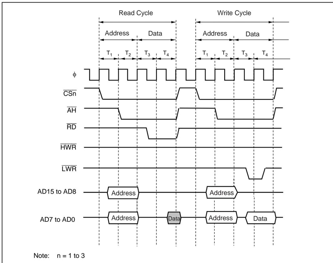
**Figure 6.19 Bus Timing for 16-Bit, 2-State Data Access Space (4)
