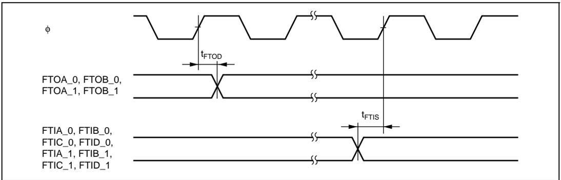
Figure 24.15 FRT Input/Output Timing
