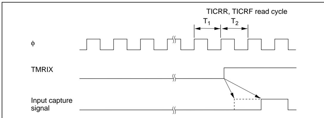
**Figure 11.12 Timing of Input Capture Signal**
