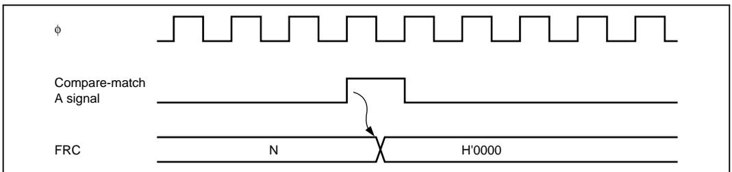
**Figure 10.6 Clearing of FRC by Compare-Match A Signal**
