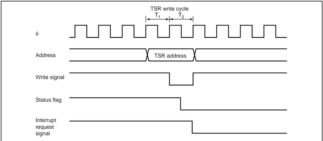
**Figure 12.45 Timing for Status Flag Clearing by CPU**
