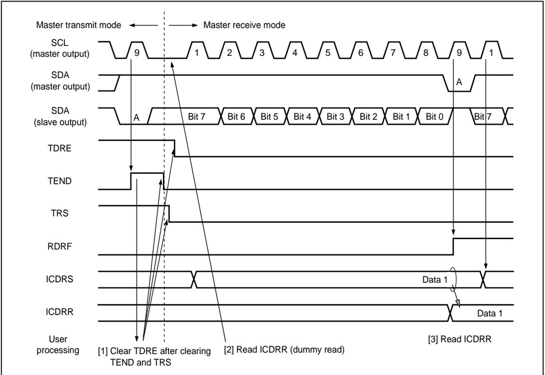
**Figure 17.7 Operation Timing in Master Receive Mode (1)**
