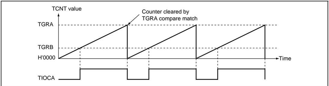
**Figure 12.25 Example of PWM Mode Operation (1)**
