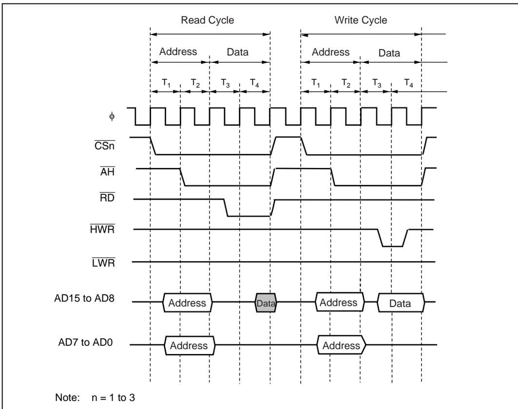
**Figure 6.17 Bus Timing for 16-Bit, 2-State Data Access Space (2)
