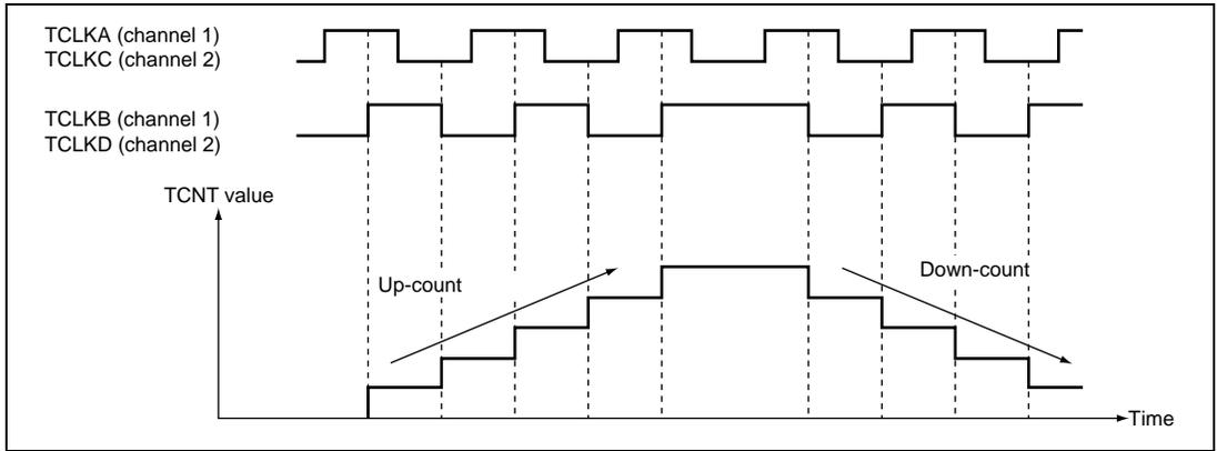
**Figure 12.32 Example of Phase Counting Mode 4 Operation**
