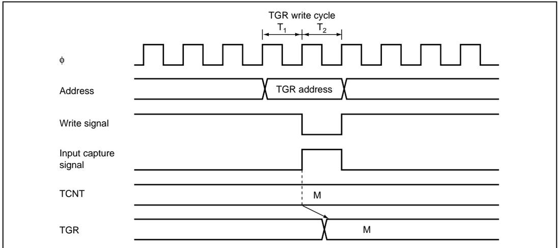
**Figure 12.52 Contention between TGR Write and Input Capture**
