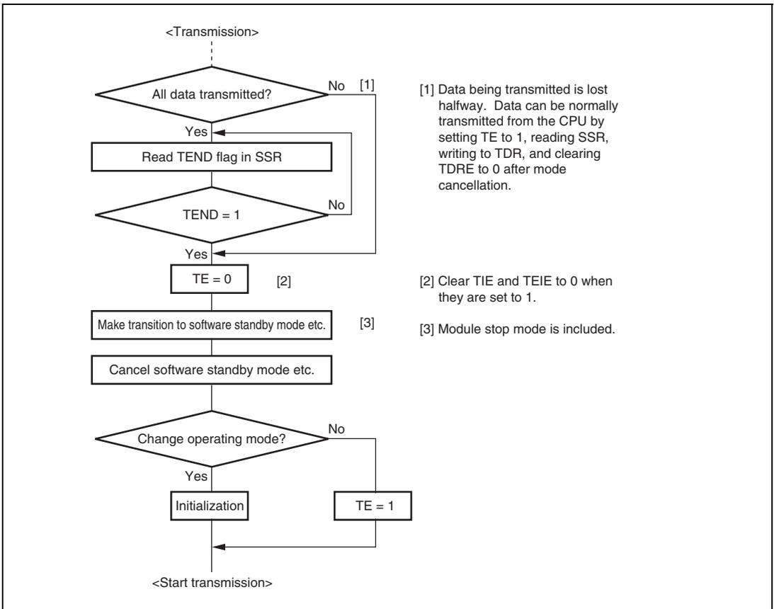
**Figure 16.21 Sample Flowchart for Mode Transition during Transmission**
