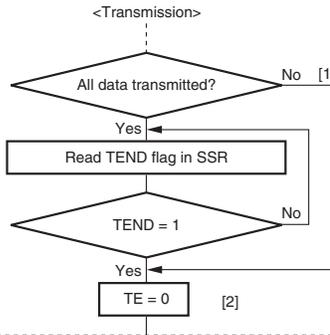
[1] Data being transmitted is lost halfway. Data can be normally transmitted from the CPU by setting TE to 1, reading SSR, writing to TDR, and clearing TDRE to 0 after mode cancellation.
