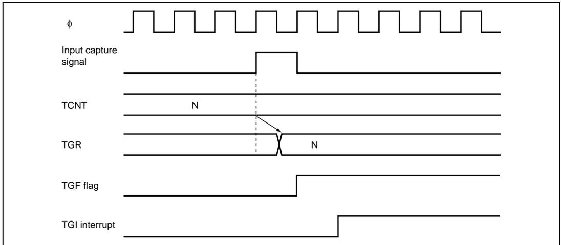
**Figure 12.42 TGI Interrupt Timing (Input Capture)**
