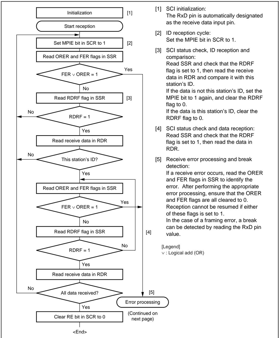
Figure 16.13 Sample Multiprocessor Serial Reception Flowchart (1)
