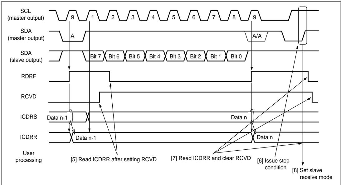
**Figure 17.8 Operation Timing in Master Receive Mode (2)**
