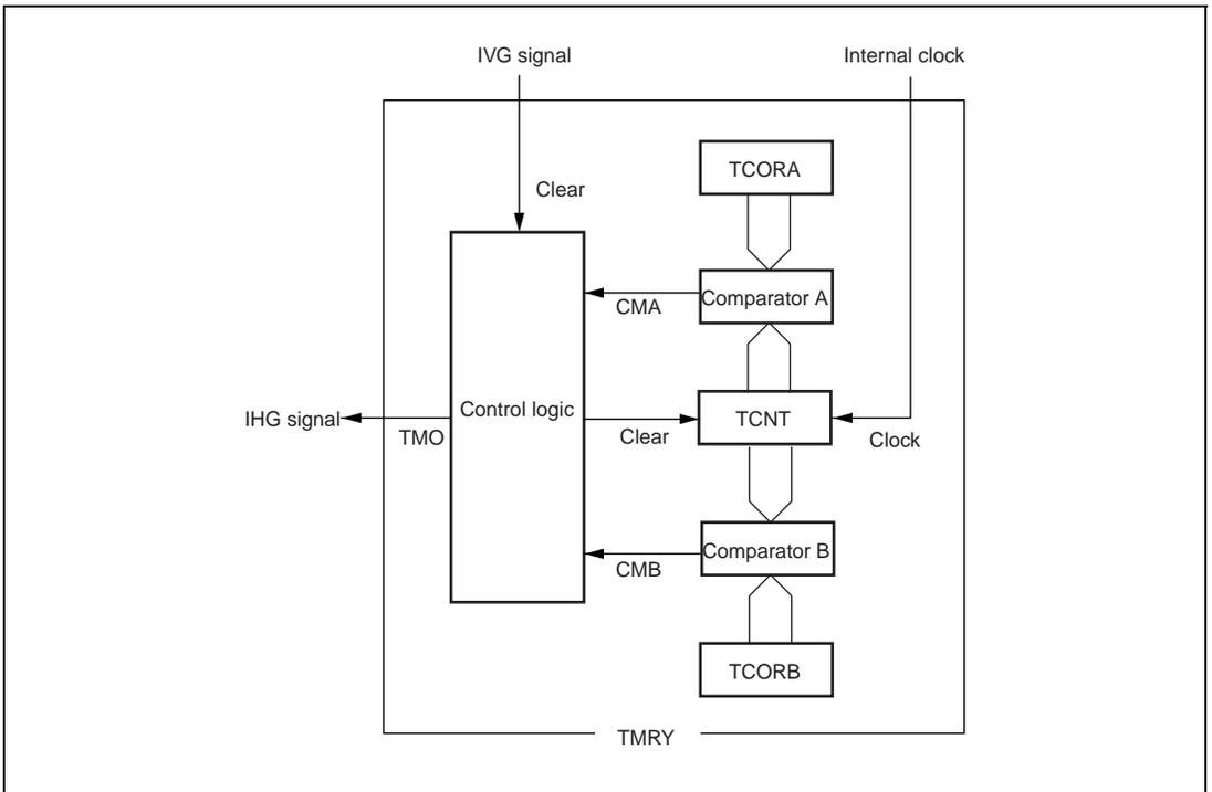
**Figure 13.15 Block Diagram for IHG Signal Generation**
