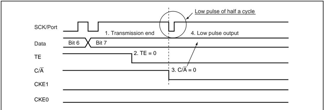
**Figure 16.25 Switching from SCK Pins to Port Pins**
