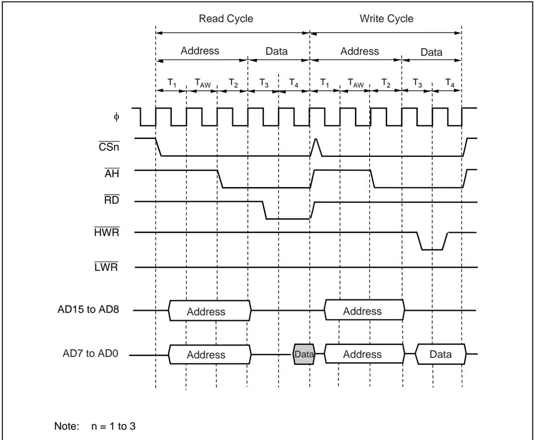
**Figure 6.18 Bus Timing for 16-Bit, 2-State Access Space (3)
