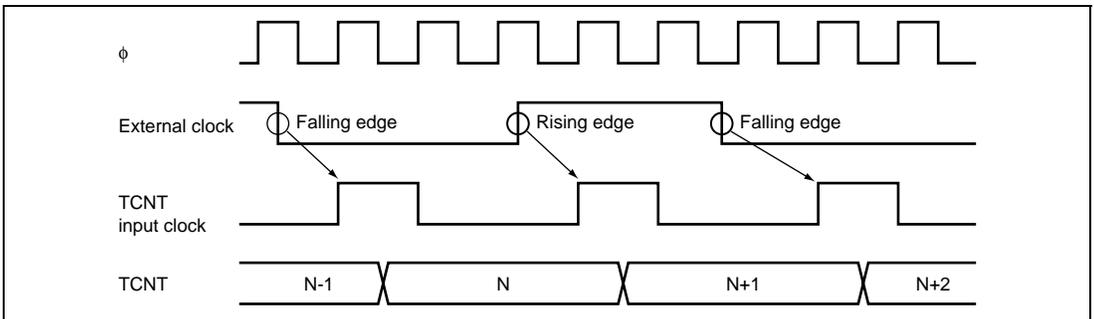
**Figure 12.34 Count Timing in External Clock Operation**
