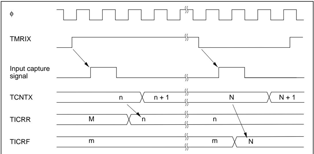
**Figure 11.11 Timing of Input Capture Operation**
