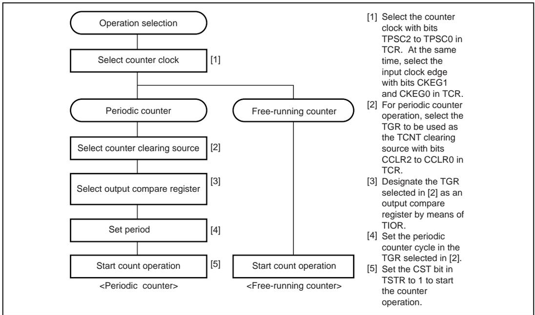
**Figure 12.6 Example of Counter Operation Setting Procedure**
