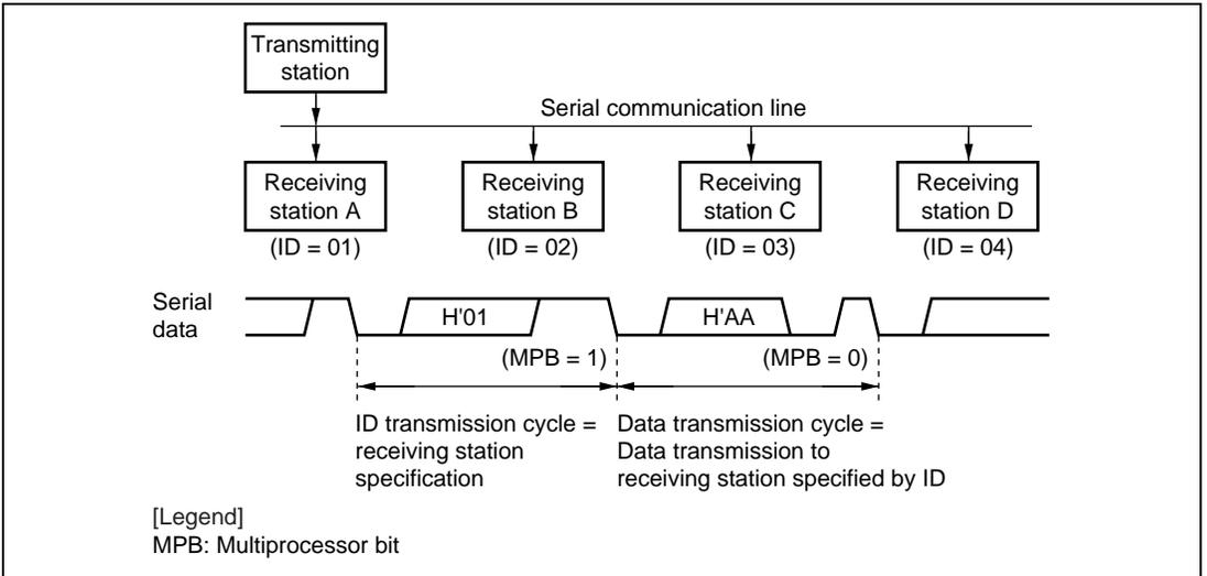
**Figure 16.10 Example of Communication Using Multiprocessor Format
