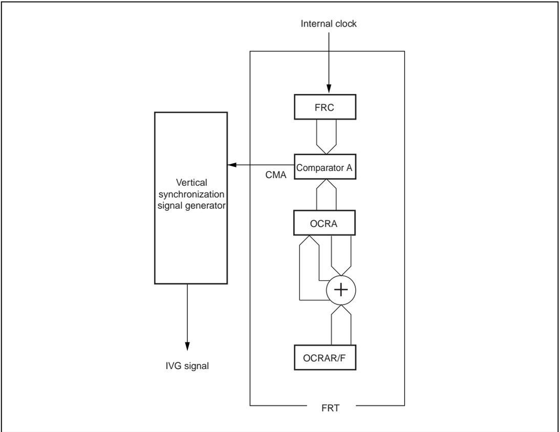
**Figure 13.14 Block Diagram for IVG Signal Generation**
