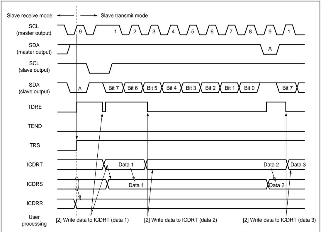
**Figure 17.9 Operation Timing in Slave Transmit Mode (1)**
