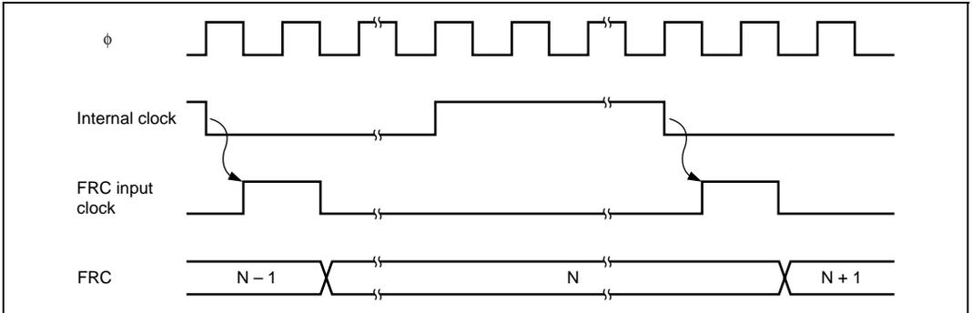
**Figure 10.3 Increment Timing with Internal Clock Source**
