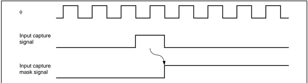
**Figure 10.15 Timing of Input Capture Mask Signal Setting**
