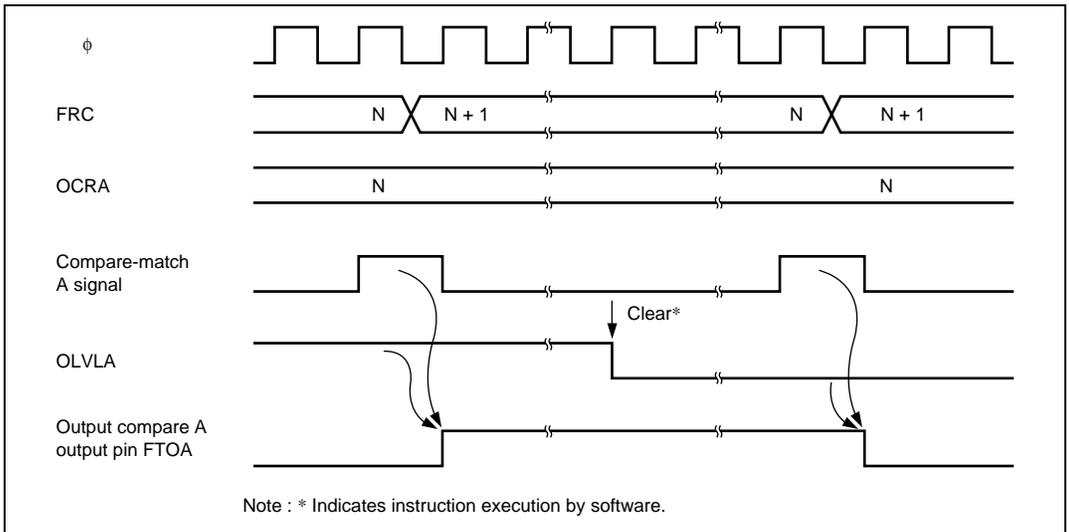
**Figure 10.5 Timing of Output Compare A Output**
