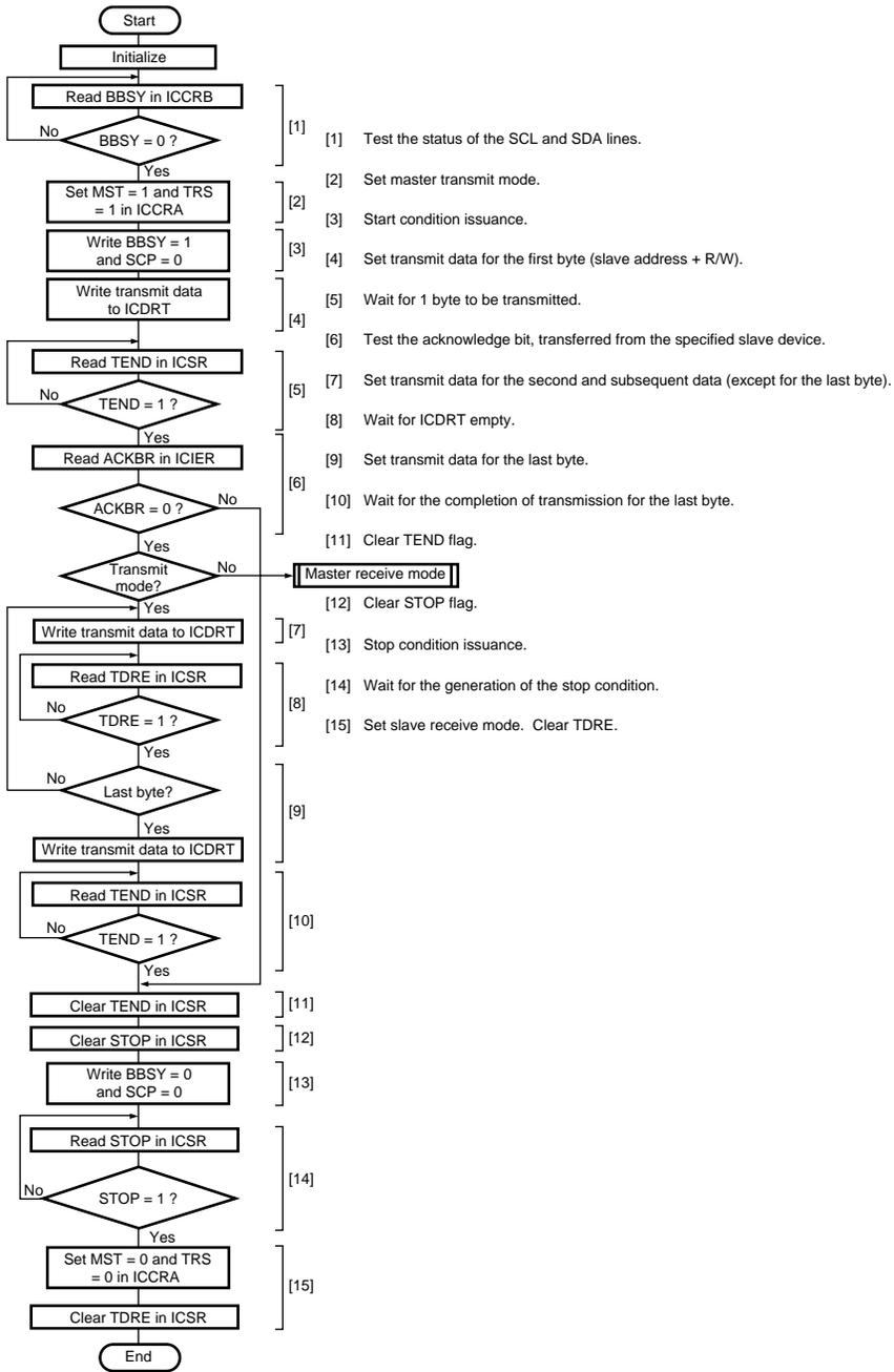
Figure 17.14 Sample Flowchart for Master Transmit Mode
