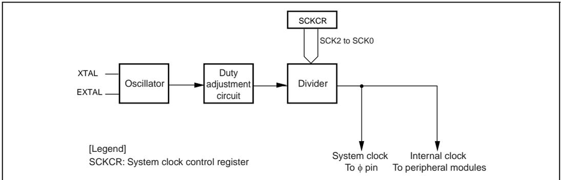
**Figure 21.1 Block Diagram of Clock Pulse Generator**
