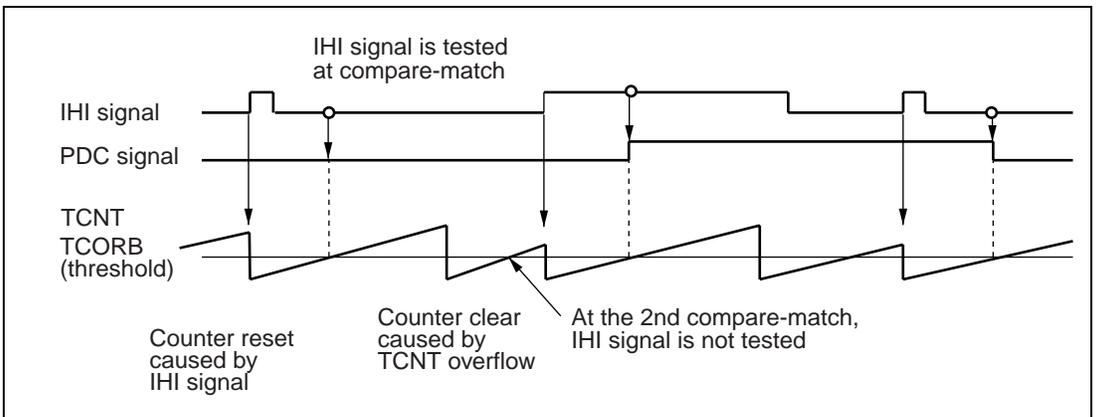
**Figure 13.4 Timing Chart for PWM Decoding**
