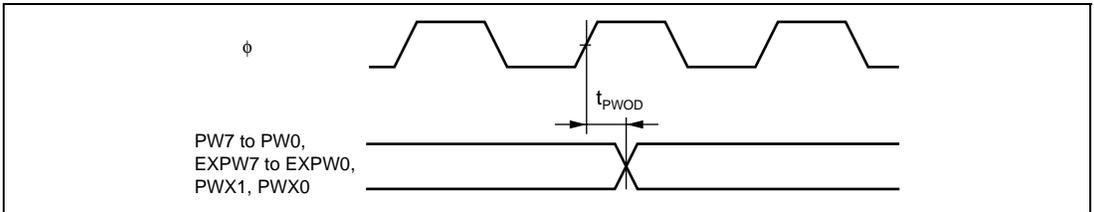
**Figure 24.22 PWM, PWMX Output Timing**
