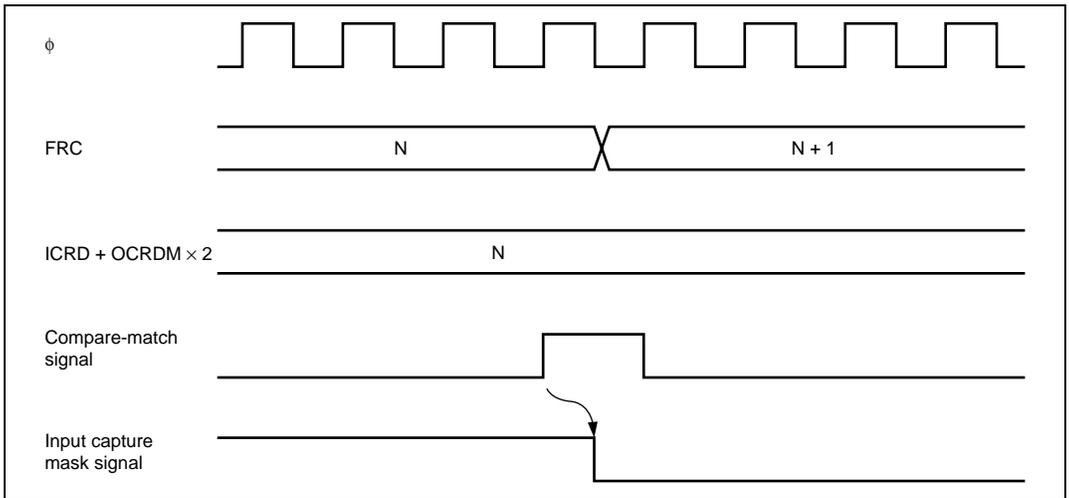
**Figure 10.16 Timing of Input Capture Mask Signal Clearing**
