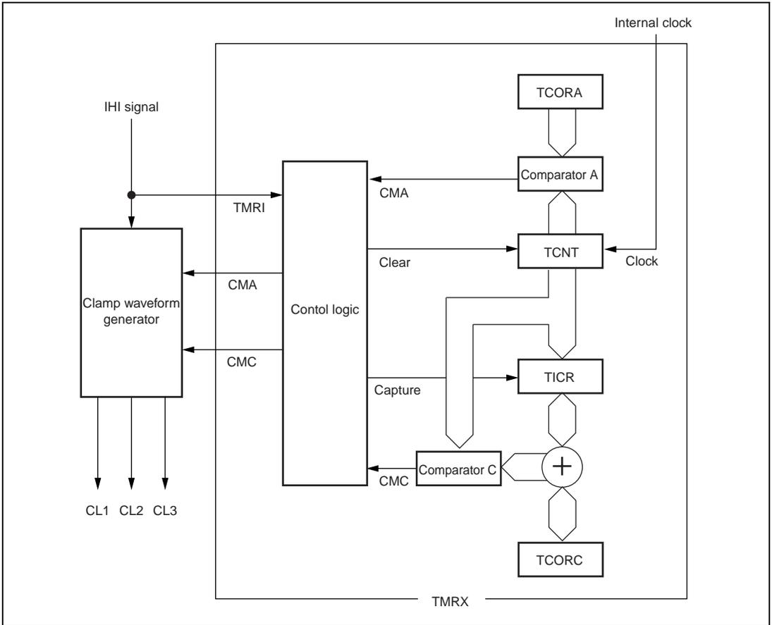
**Figure 13.5 Block Diagram for Clamp Waveform Generation**
