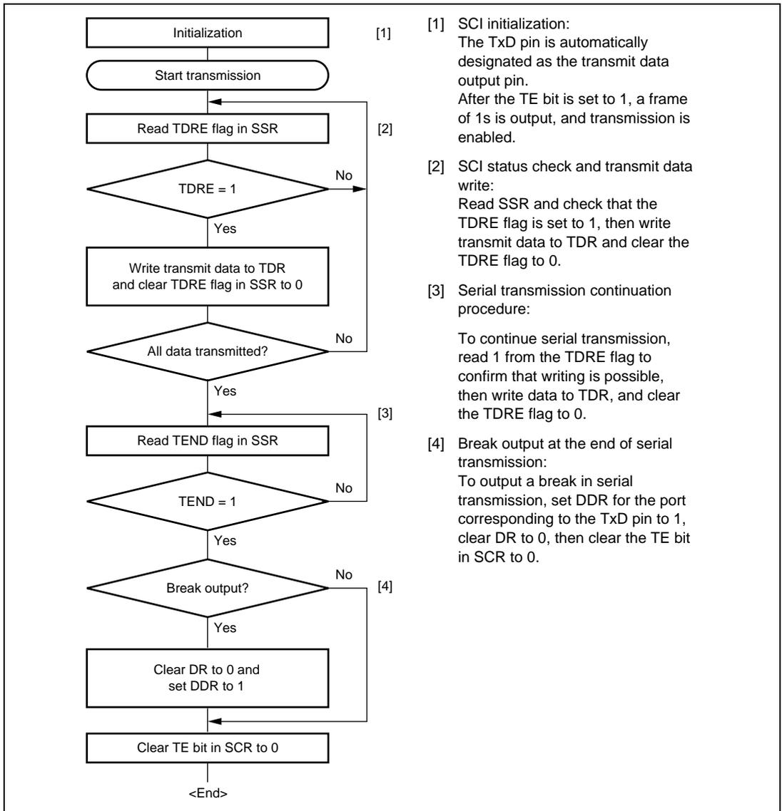
**Figure 16.7 Sample Serial Transmission Flowchart**
