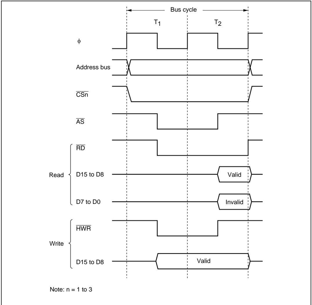
Figure 6.5 Bus Timing for 8-Bit, 2-State Access Space
