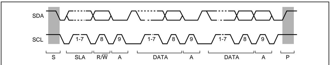
**Figure 17.4 I<sup>2</sup>C Bus Timing**
