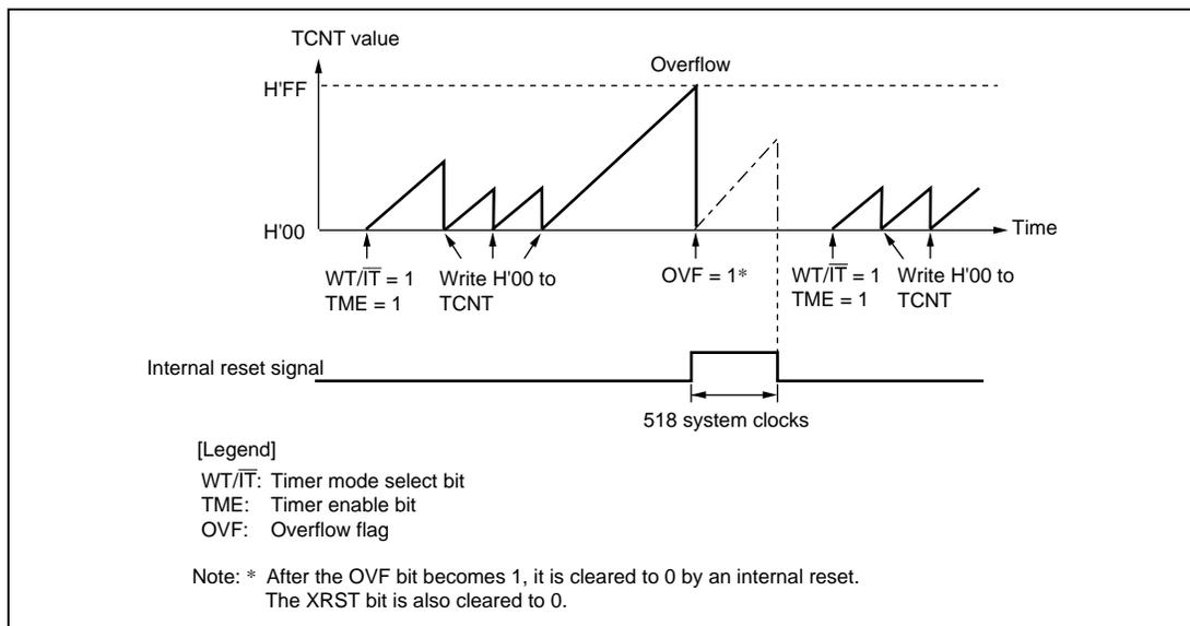
Figure 15.2 Watchdog Timer Mode ( $\overline{RST/NMI} = 1$ ) Operation
