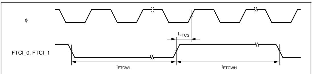
Figure 24.16 FRT Clock Input Timing
