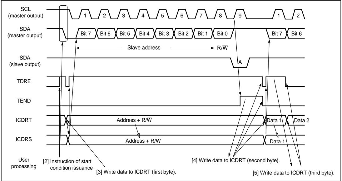
**Figure 17.5 Operation Timing in Master Transmit Mode (1)**
