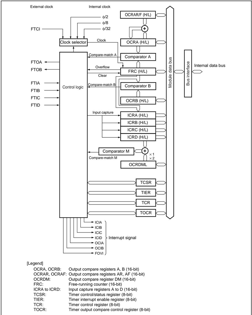
**Figure 10.1 Block Diagram of 16-Bit Free-Running Timer**
