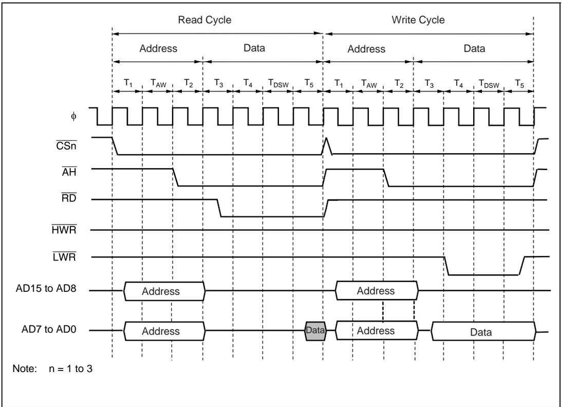
**Figure 6.23 Bus Timing for 16-Bit, 3-State Data Access Space (2)
