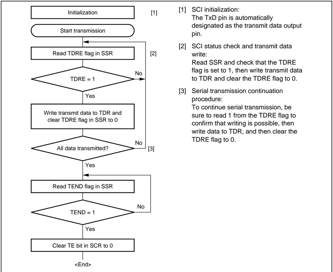
**Figure 16.17 Sample Serial Transmission Flowchart**
