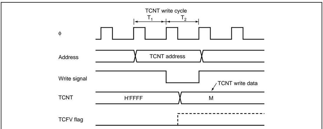
**Figure 12.55 Contention between TCNT Write and Overflow**
