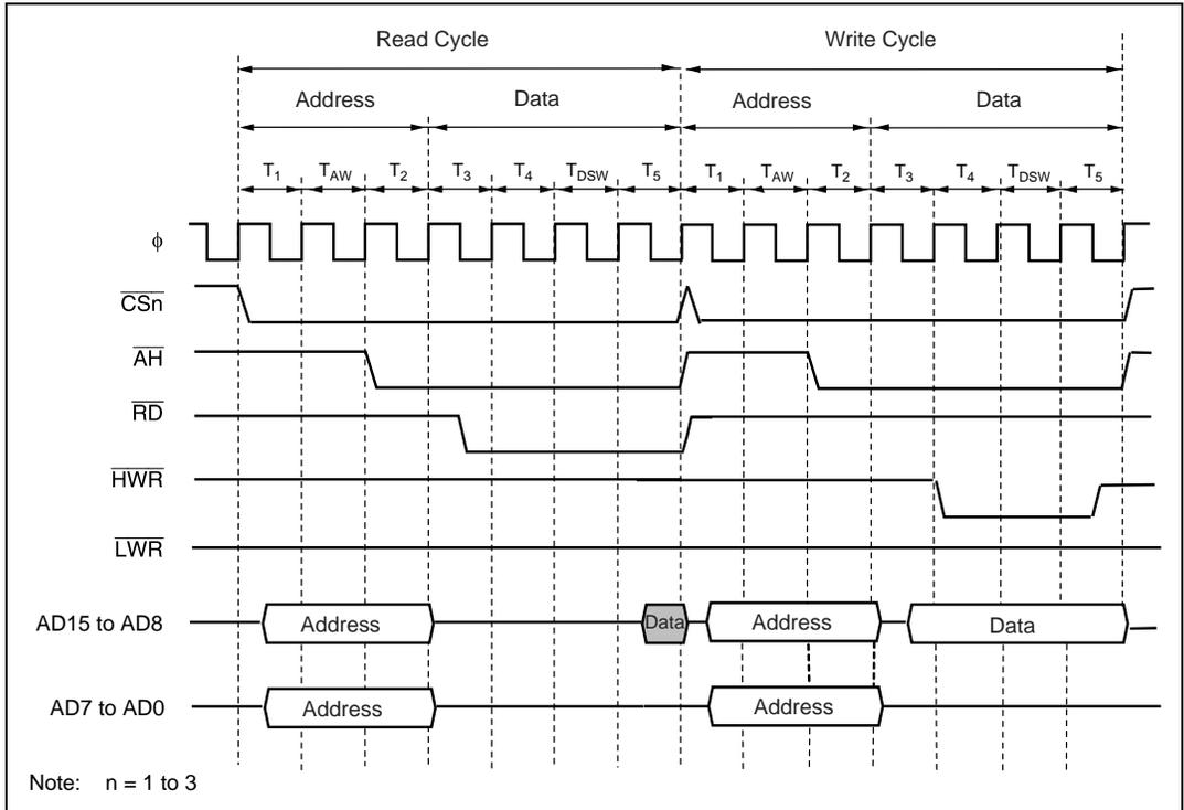
**Figure 6.22 Bus Timing for 16-Bit, 3-State Data Access Space (1)**
