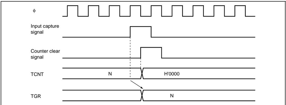
**Figure 12.38 Counter Clear Timing (Input Capture)**
