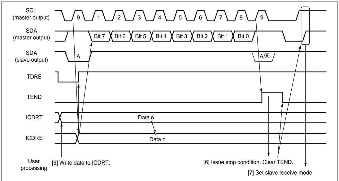
**Figure 17.6 Operation Timing in Master Transmit Mode (2)**
