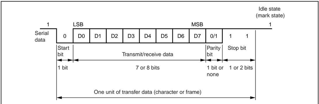
**Figure 16.2 Data Format in Asynchronous Communication**
