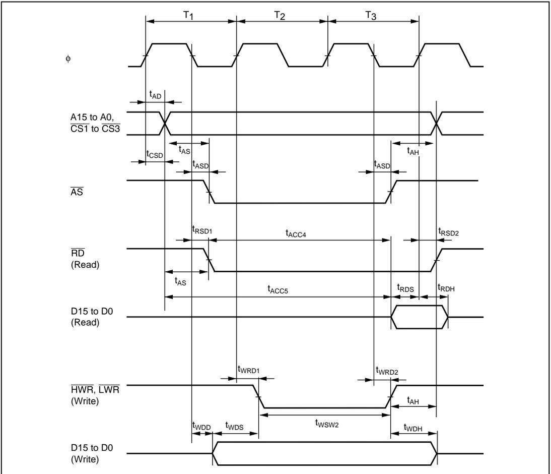
Figure 24.9 Basic Bus Timing/3-State Access
