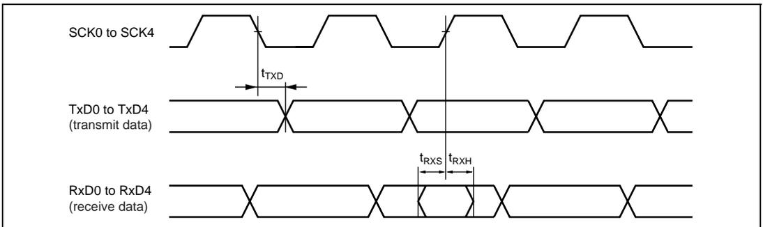
**Figure 24.24 SCI Input/Output Timing (Clock Synchronous Mode)**
