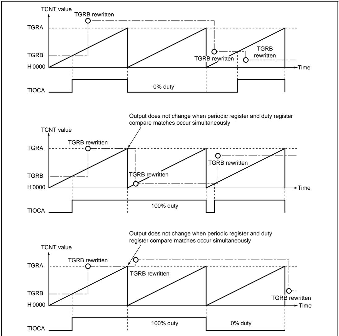
**Figure 12.27 Example of PWM Mode Operation (3)**
