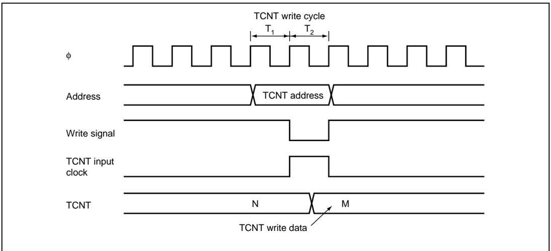
**Figure 12.48** Contention between TCNT Write and Increment Operations
