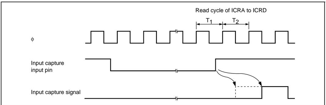
**Figure 10.8 Timing of Input Capture Input Signal (When ICRA to ICRD are Read)**
