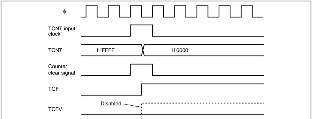
**Figure 12.54 Contention between Overflow and Counter Clearing**
