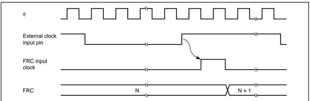
**Figure 10.4 Increment Timing with External Clock Source**
