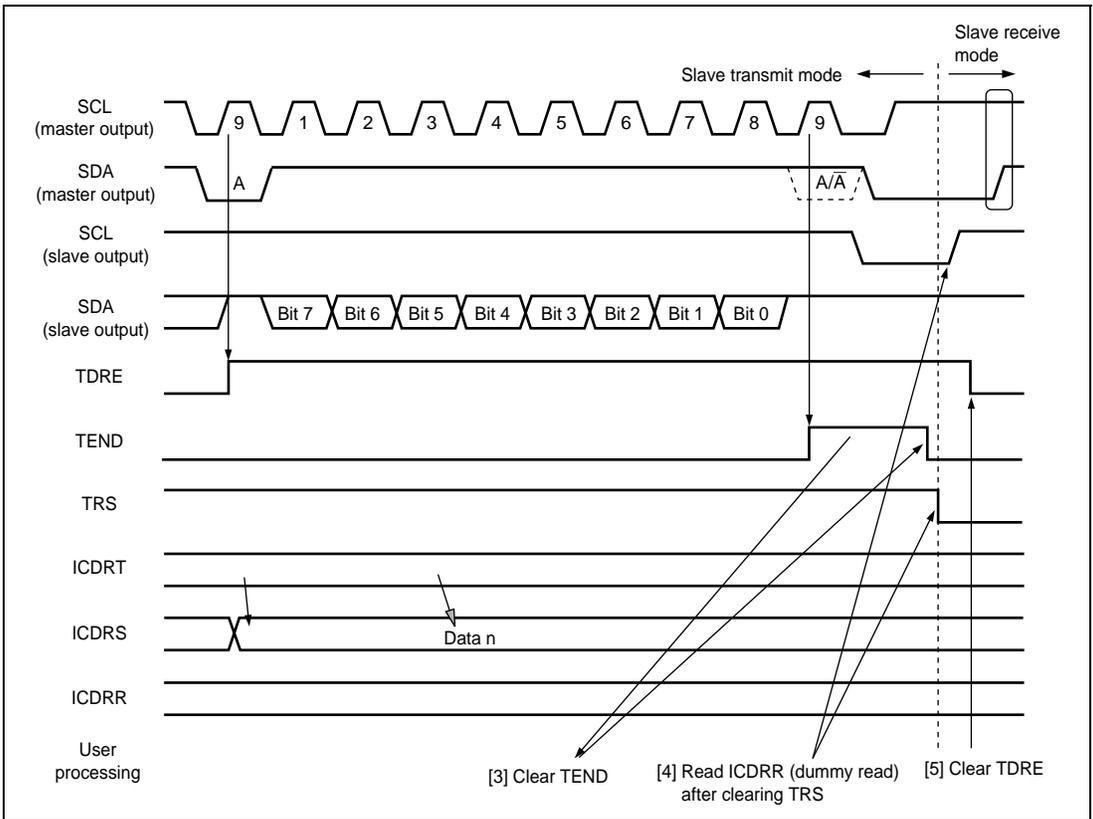
**Figure 17.10 Operation Timing in Slave Transmit Mode (2)**
