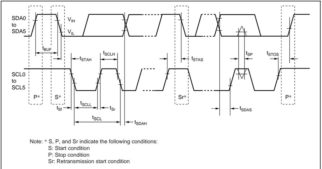
**Figure 24.26 Input/Output Timing of I<sup>2</sup>C Bus Interface 3**
