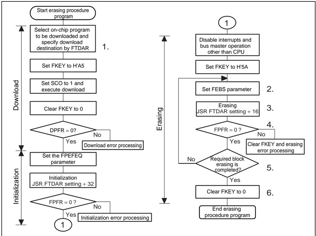
**Figure 20.12 Erasing Procedure**
