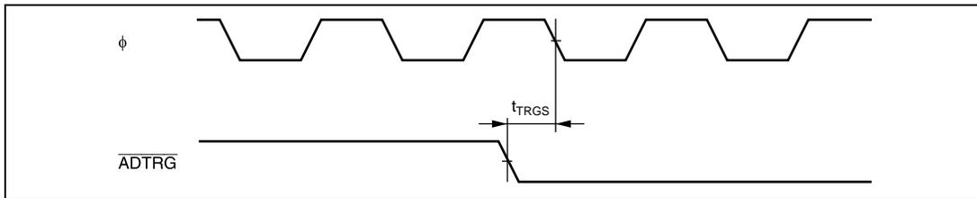
Figure 24.25 A/D Converter External Trigger Input Timing
