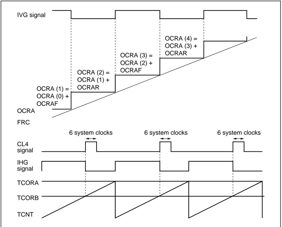
**Figure 13.16 IVG Signal/IHG Signal/CL4 Signal Timing Chart**
