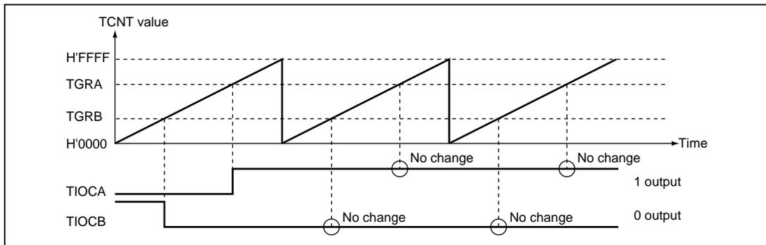
**Figure 12.10 Example of 0 Output/1 Output Operation**
