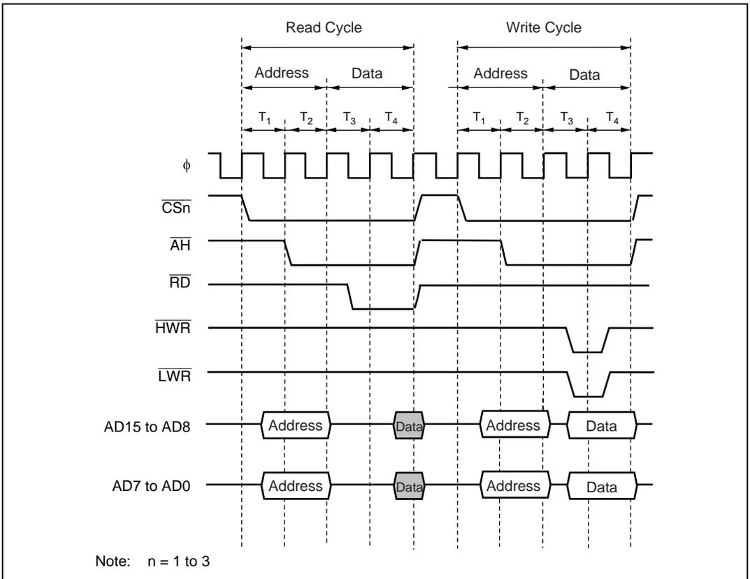
**Figure 6.21 Bus Timing for 16-Bit, 2-State Data Access Space (6)
