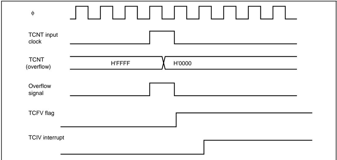
**Figure 12.43 TCIV Interrupt Setting Timing**
