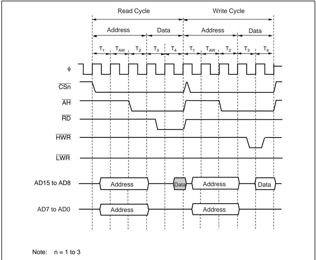
**Figure 6.16 Bus Timing for 16-Bit, 2-State Data Access Space (1)
