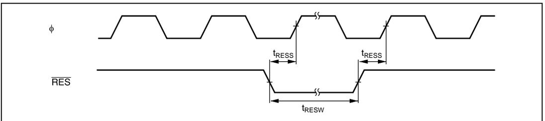
**Figure 24.6 Reset Input Timing**
