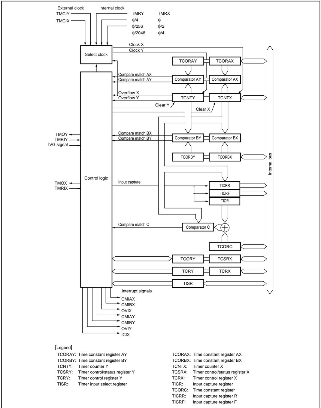
**Figure 11.2 Block Diagram of 8-Bit Timer (TMR)**
