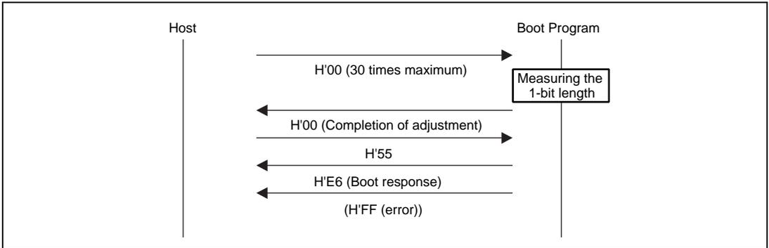
**Figure 20.20 Bit-Rate-Adjustment Sequence**
