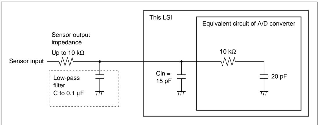
**Figure 18.6 Example of Analog Input Circuit**
