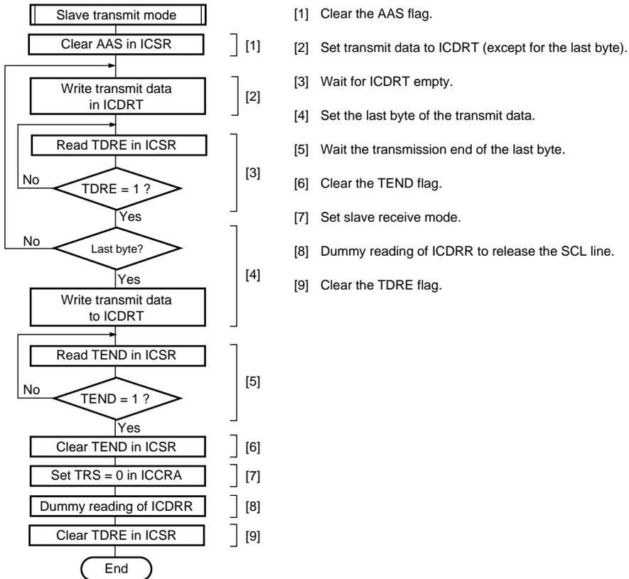
**Figure 17.16 Sample Flowchart for Slave Transmit Mode**
