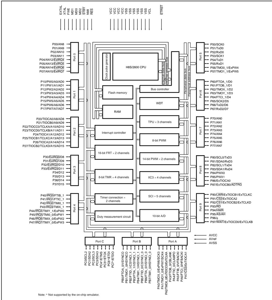
Figure 1.1 Internal Block Diagram of H8S/2437 Group
