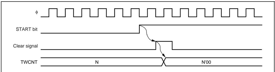
**Figure 14.4 TWCNT Clear Timing by Setting START Bit**
