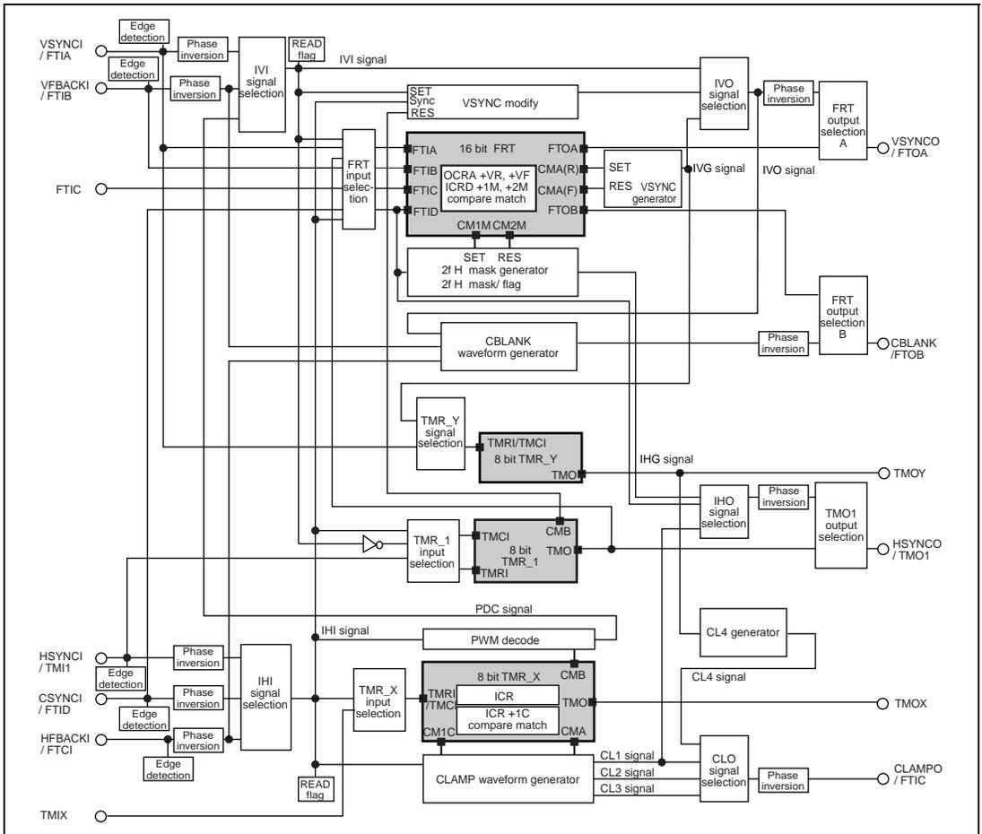
**Figure 13.2 Block Diagram of Timer Connection**
