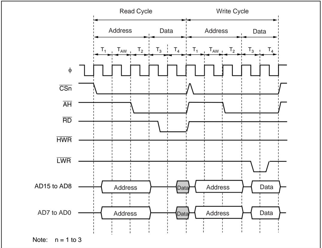
**Figure 6.20 Bus Timing for 16-Bit, 2-State Data Access Space (5)
