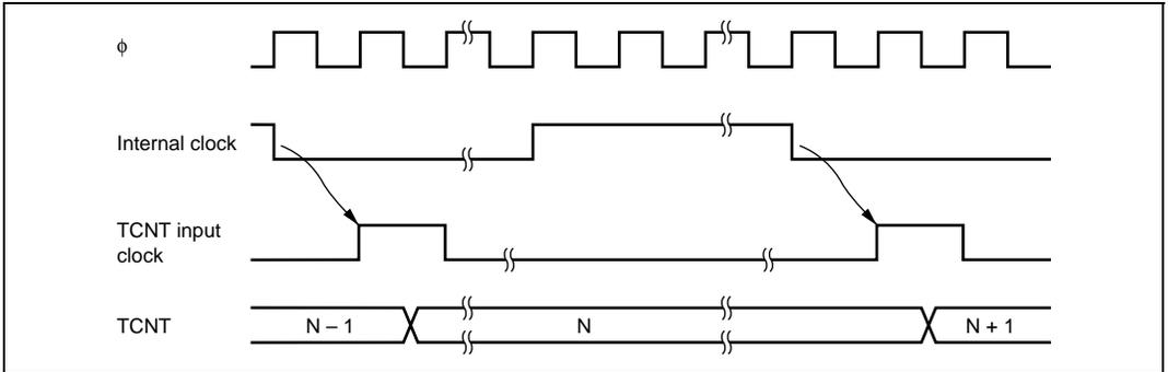
**Figure 11.4** Count Timing for Internal Clock Input
