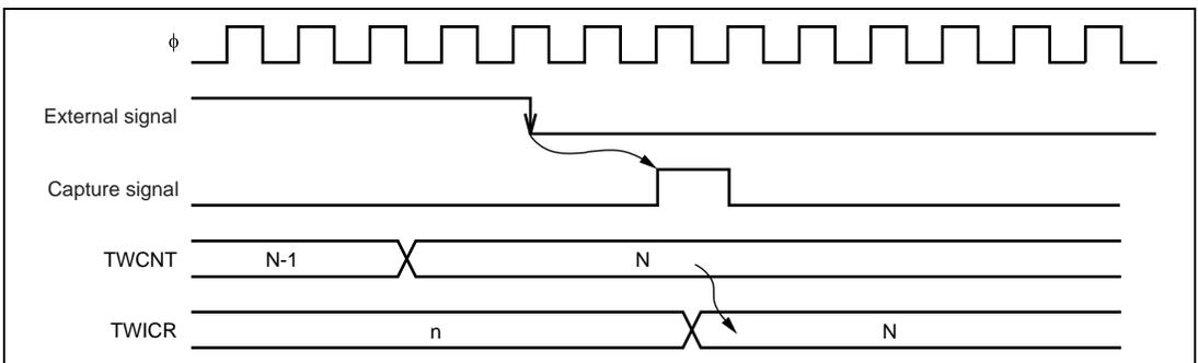
Figure 14.6 Input Capture Timing during Duty Measurement
