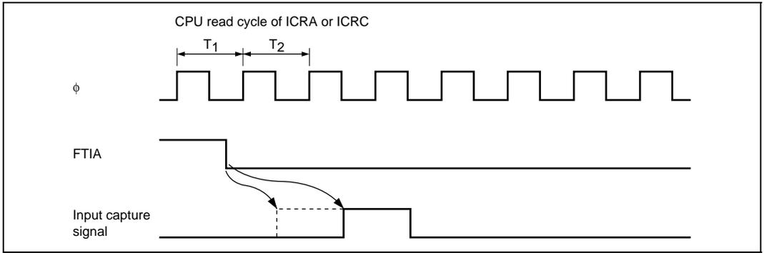
**Figure 10.10 Buffered Input Capture Timing (BUFEA = 1)**
