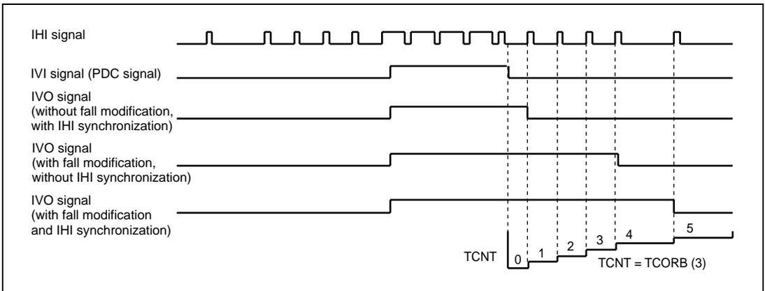
**Figure 13.13 Fall Modification and IHI Synchronization Timing Chart**
