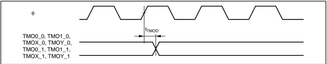
**Figure 24.19 8-Bit Timer Output Timing**
