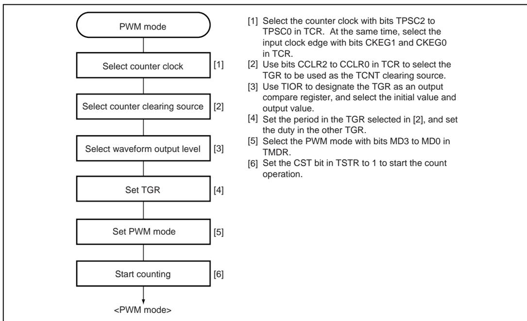
**Figure 12.24 Example of PWM Mode Setting Procedure**
