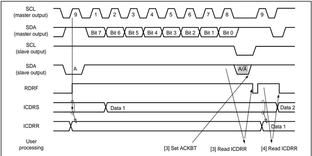
**Figure 17.12 Operation Timing in Slave Receive Mode (2)**
