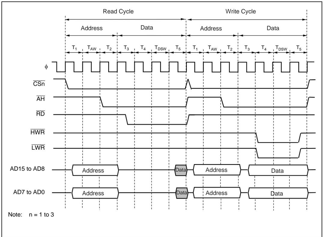
**Figure 6.24 Bus Timing for 16-Bit, 3-State Data Access Space (3)**
