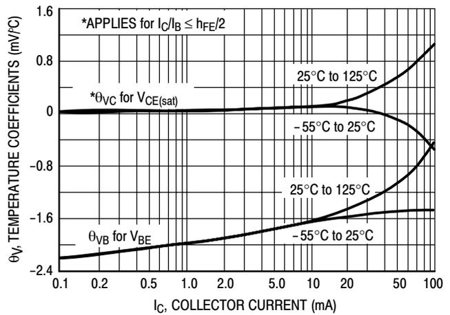
Figure 12. Temperature Coefficients
