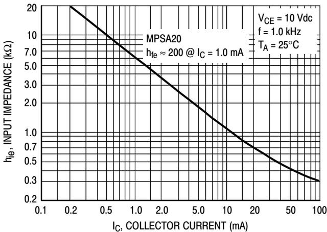
Figure 17. Input Impedance
