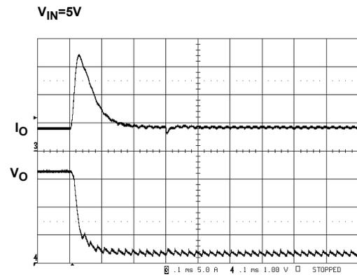
FIGURE 20. SHORT-CIRCUIT PROTECTION
