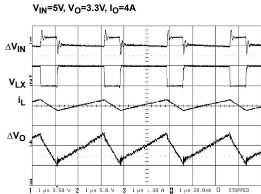
FIGURE 14. SWITCHING WAVEFORMS
