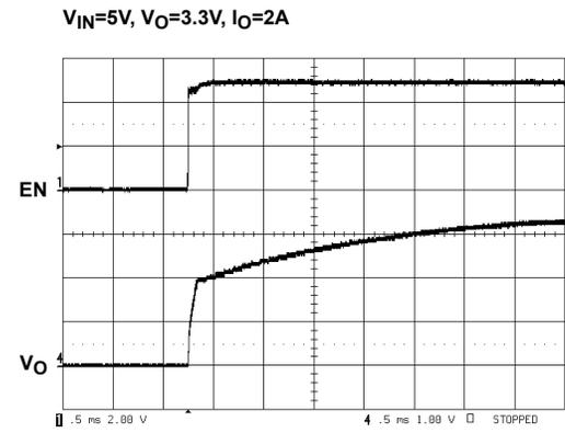
FIGURE 18. RELEASING EN
