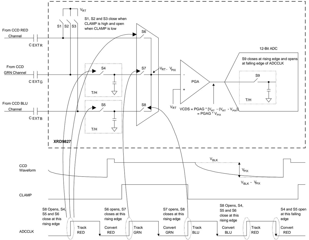
**Figure 19. CDS Timing (Triple Channel)
