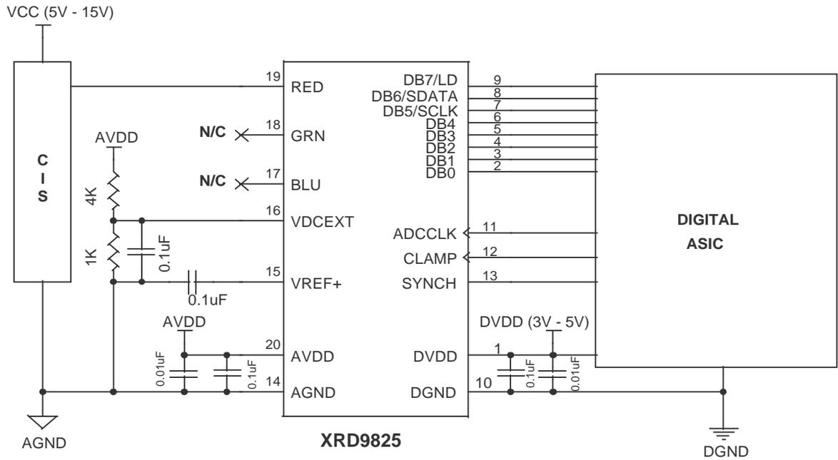
**Figure 5. Typical Application Circuitry CIS DC Coupled Non-Inverted Mode**
