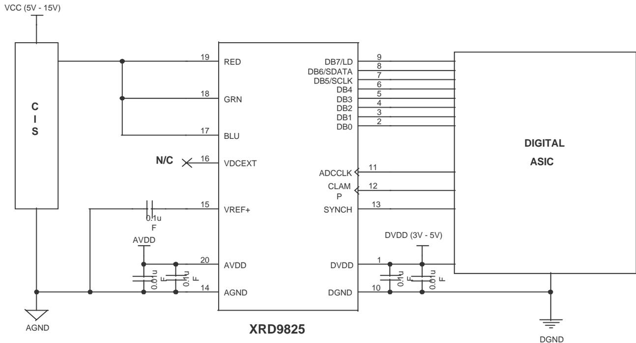
**Figure 11. Typical Application Circuitry Internal CIS Rotating Gain and Offset Line-By-Line**
