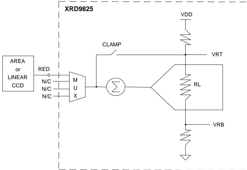
**Figure 13. CCD AC Coupled Application**
