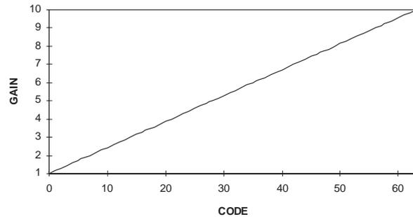
Figure 20. Transfer Curve for the 6-Bit PGA
