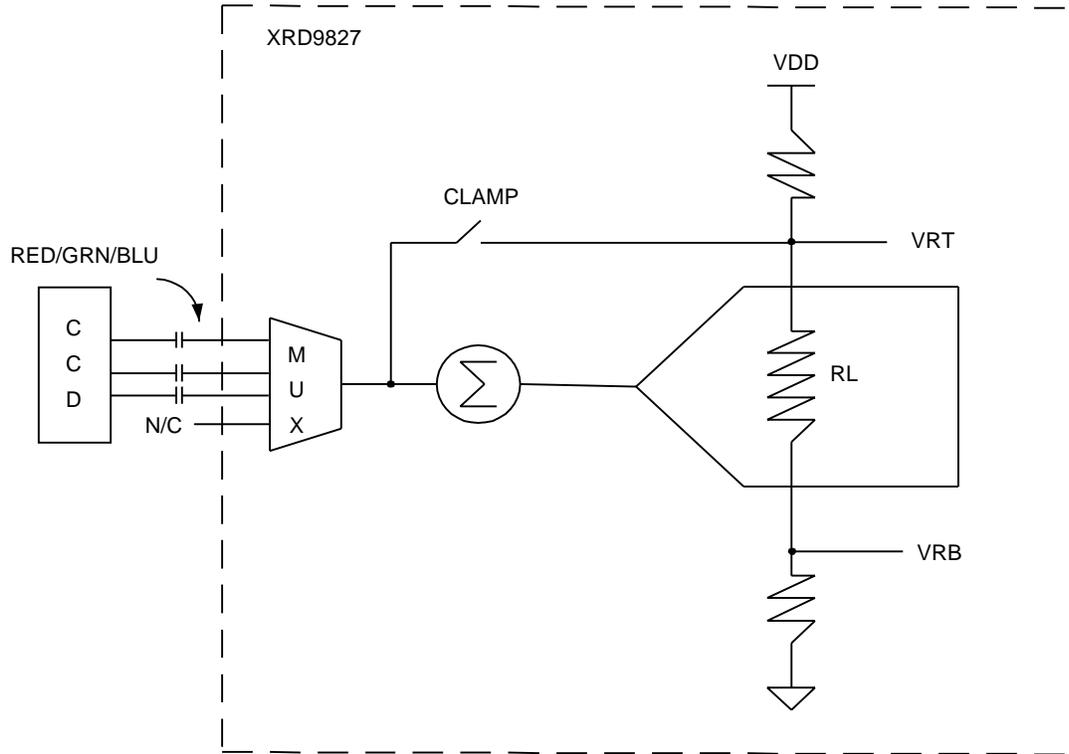
Figure 16. CCD AC Coupled Application
