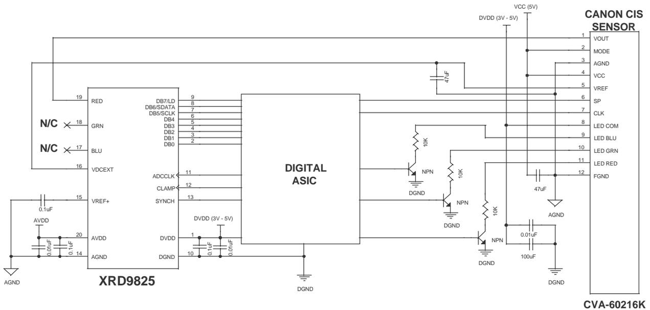
**Figure 10. Typical Application Circuitry Internal CIS Reference Circuit Mode
