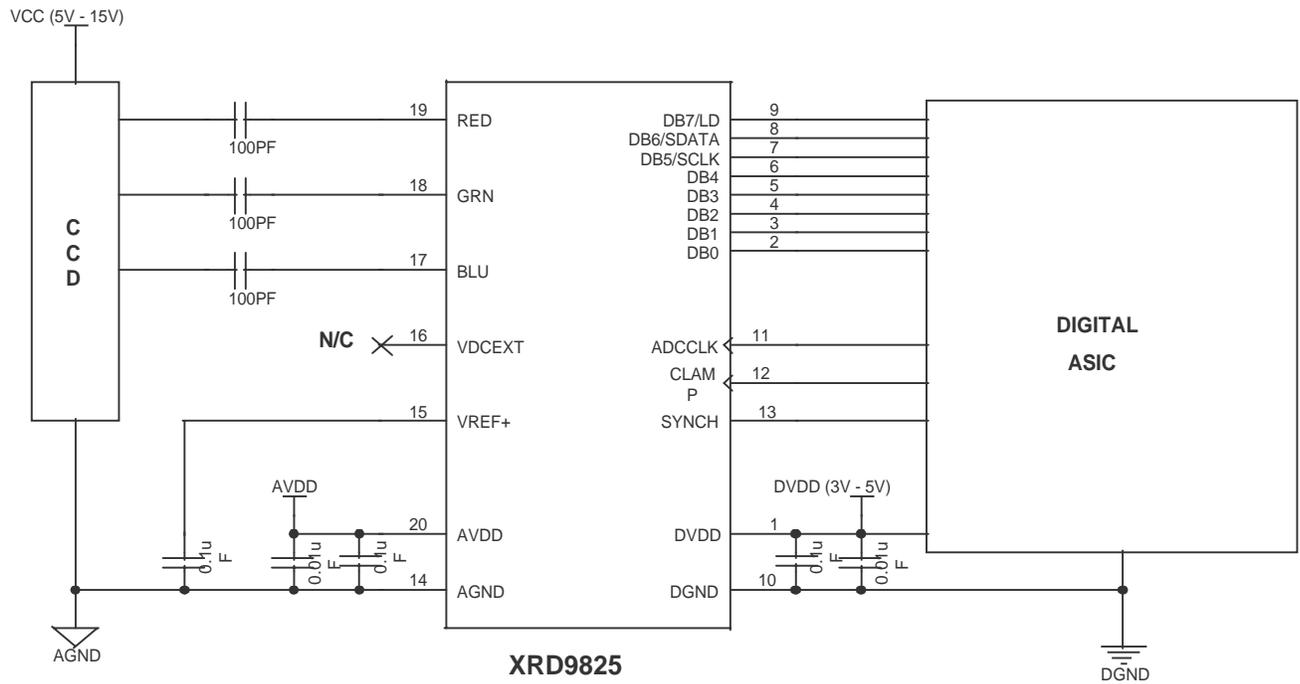
**Figure 17. Typical Application Circuitry Triple Channel CCD
