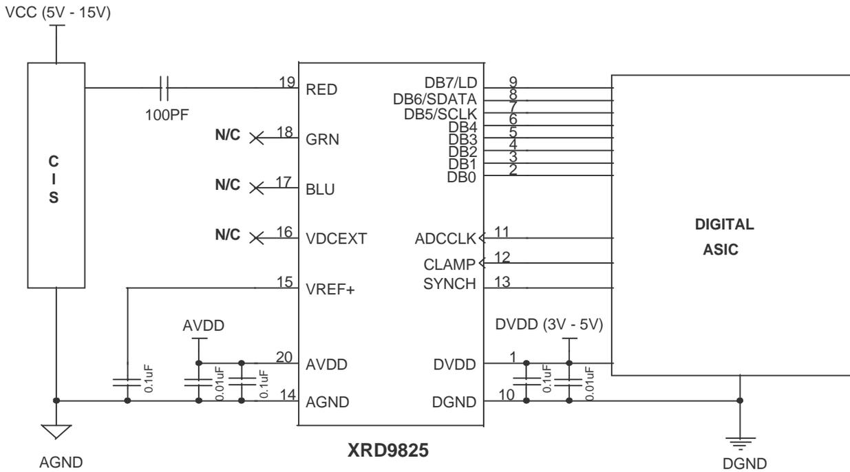
**Figure 8. Typical Application Circuitry CIS AC Coupled Non-Inverted**
