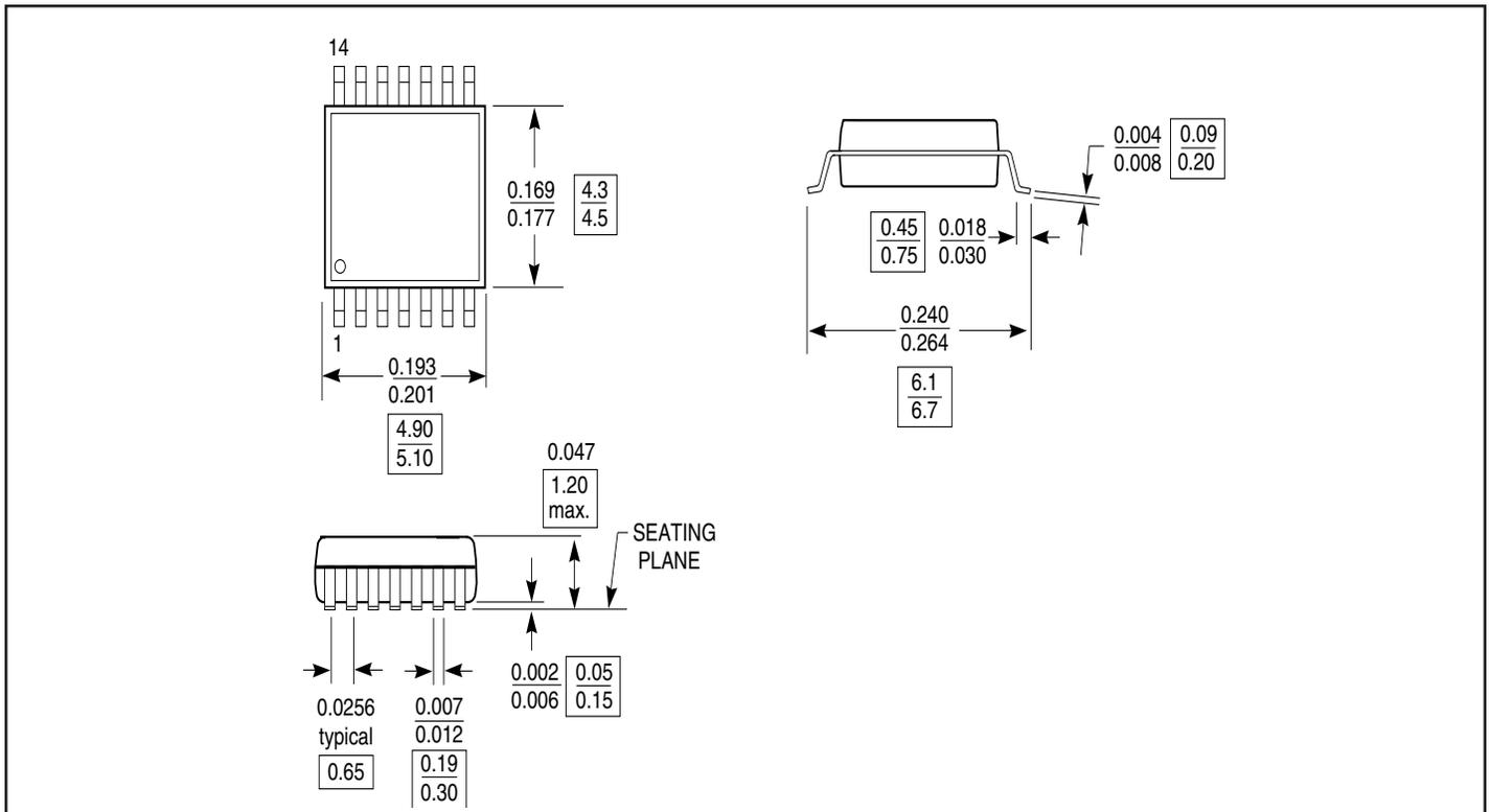
**Packaging Mechanical: 14-Pin SOIC (W)**
