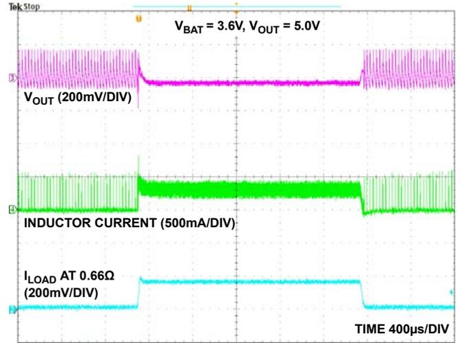
FIGURE 12. LOAD TRANSIENT RESPONSE (20mA TO 250mA)
