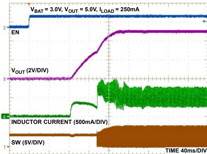
FIGURE 9. START-UP AFTER ENABLE ( $I_{LOAD} = 250mA$ )
