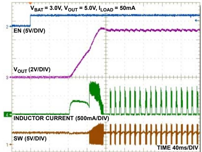
FIGURE 10. START-UP AFTER ENABLE ( $I_{LOAD} = 50mA$ )
