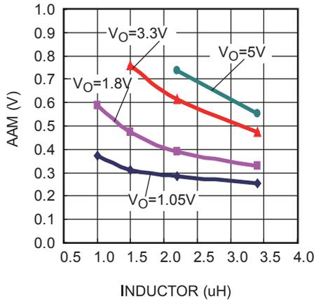
**Figure 5— AAM Selection for Common Output Voltages (VIN=5V-24V)**
