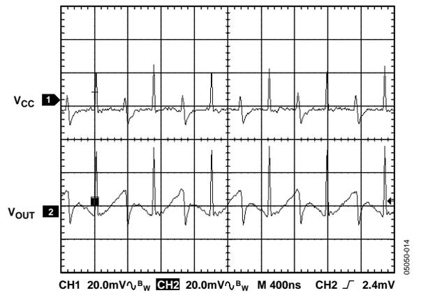
Figure 13. 2x Mode Operating Waveforms
