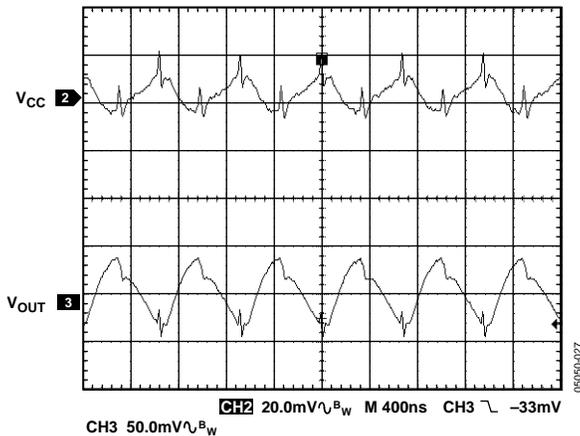
Figure 27. 1.5× Mode Operation, Four LEDs with 20 mA/LED at V<sub>CC</sub> = 3.6 V, with a 1 μF V<sub>CC</sub> Decoupling Capacitor
