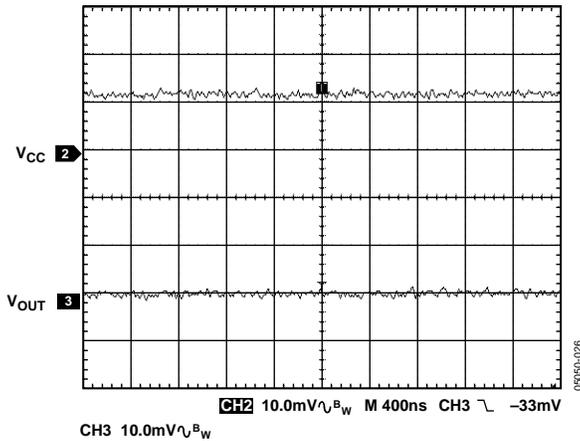
Figure 26. 1× Mode Operation, Four LEDs with 20 mA/LED at V<sub>CC</sub> = 5.0 V, with a 1 μF V<sub>CC</sub> Decoupling Capacitor
