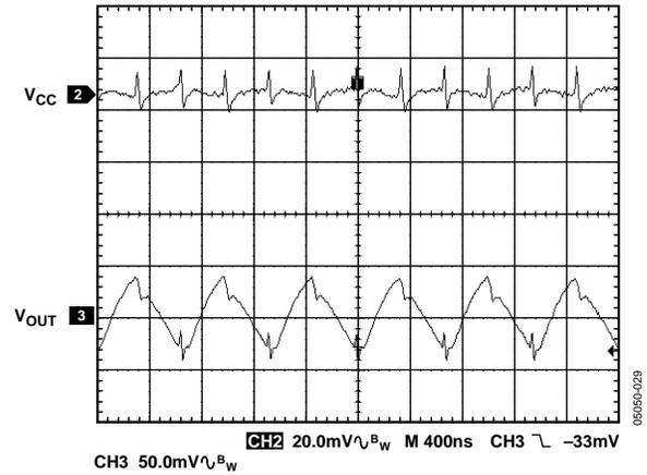
Figure 29. 1.5× Mode Operation, Four LEDs with 20 mA/LED at V<sub>CC</sub> = 3.6 V, with a 4.7 μF V<sub>CC</sub> Decoupling Capacitor
