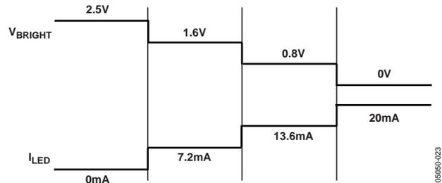
Figure 22. PWM Brightness Control Application Diagram Using a DC Voltage Applied to V<sub>BRIGHT</sub>
