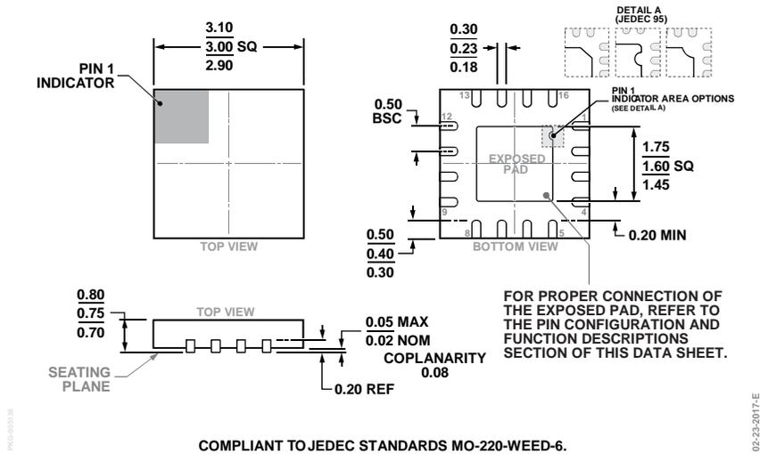
Figure 31. 16-Lead Lead Frame Chip Scale Package [LF CSP]
