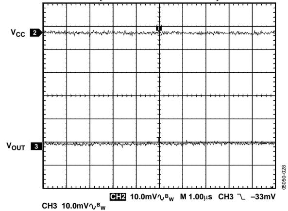
Figure 28. 1× Mode Operation, Four LEDs with 20 mA/LED at V<sub>CC</sub> = 5.0 V, with a 4.7 μF V<sub>CC</sub> Decoupling Capacitor
