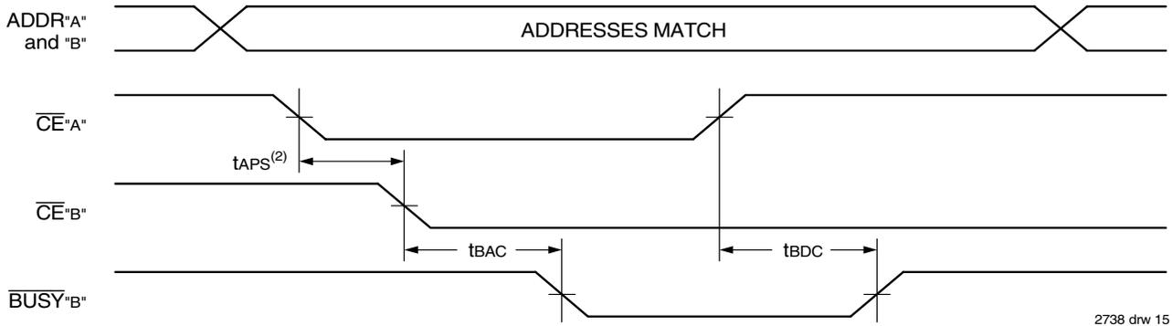
**Waveform of  $\overline{\text{BUSY}}$  Arbitration Cycle Controlled by Address Match Timing<sup>(1)</sup> ( $\text{M}/\overline{\text{S}} = \text{VIH}$ )**
